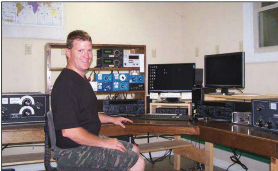
Scott Dickson, W5WZ, from Calhoun, Ouachita Parish, Louisiana, with his SO2R station. He utilizes a pair of ICE 419B bandpass filters, as well as a full complement of coax stub filters. The ICE filters are between the transceivers and the legal-limit amplifiers. The coax stub filters are installed on the output side of the WXØB SixPack.
