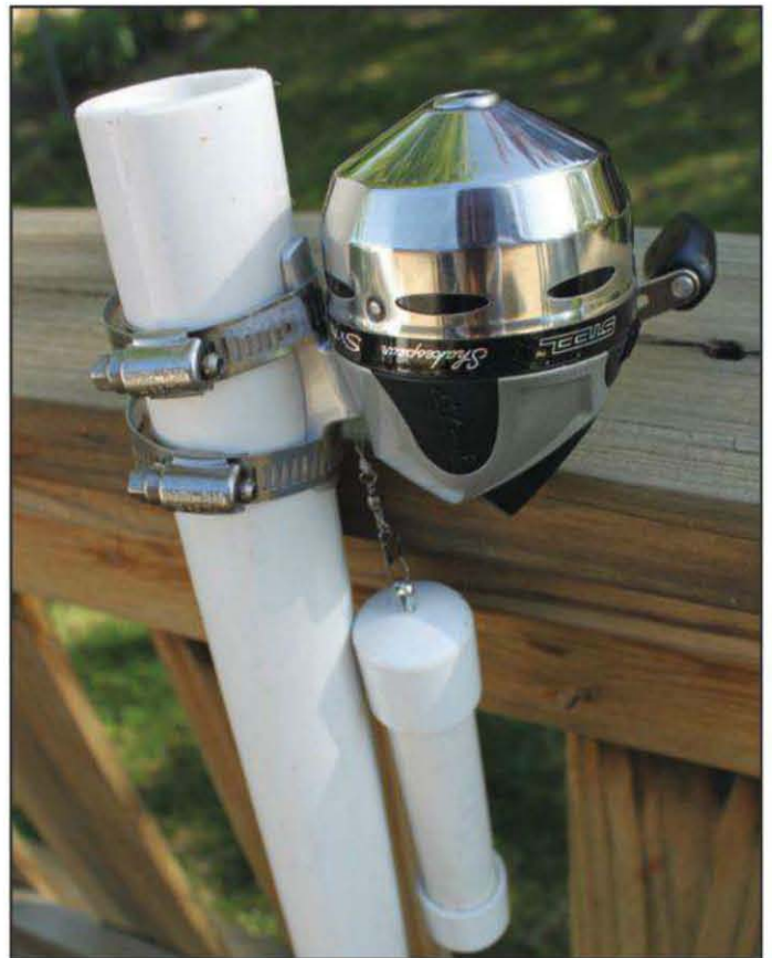
Photo C- Closeup view of fishing reel (not included with antenna launcher kit) and projectile.
