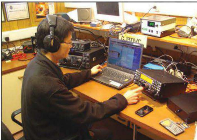
Kazunori Watanabe, JK3GAD, operating at GJ3DVC on the Isle of Jersey. Note the microHAM MK2R+ above the left transceiver to accommodate smooth SO2R operation.
