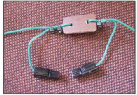
Photo E— A link dipole is a multi-band antenna with different band segments switched in and out by manually attaching or detaching different antenna segments.
