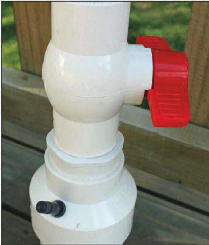
Photo B- Closeup of air fill valve on the JARC Antenna Launcher and the large hand valve used to launch the projectile (see text for details). A video demo of the launcher can be viewed at http://bit.ly/Hsxcco .
