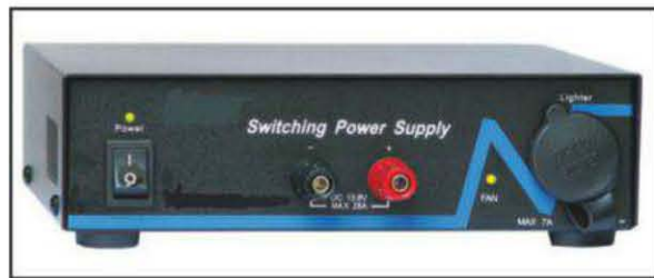
Photo B— There is also the MFJ-4128 switching power supply at $84.95. It weighs in at four pounds but can provide outputs of 28 amps maximum and 25 amps continuously at 13.8 VDC, more than enough to power your average HF, VHF, or UHF transceiver.
