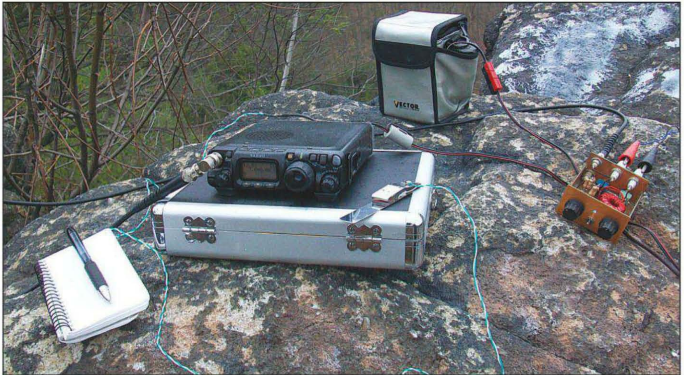
Photo B— K3NG's outdoor shack: a Yaesu FT-817, straight key, and BLT tuner. (Photo by Eliza Good)
