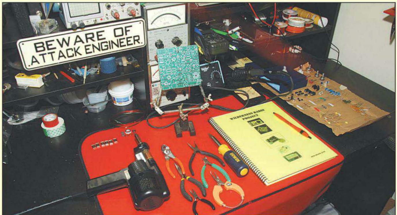
This is my workbench. It’s “sorta’ clean,” meaning I can see the simulated wood-grain top of the bench! Actually, this is about as neat as it gets. The red pad is an anti-static pad that I use on which I use to build to prevent electro-static discharge (ESD) damage to components and circuit boards. Tools are arranged for easy access, and the yellow manual is on the right side of the building area. The big black “gun”-looking device is a desoldering gun, a must for removing soldered parts on a circuit board.
