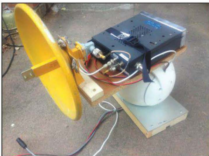
Photo 5– Brian Yee, W6BY, called his unit the “Spaceball.” It is an antenna positioner unit for azimuth and elevation, controlled by an Apple iPhone. (Photo by Brian Yee, W6BY)
