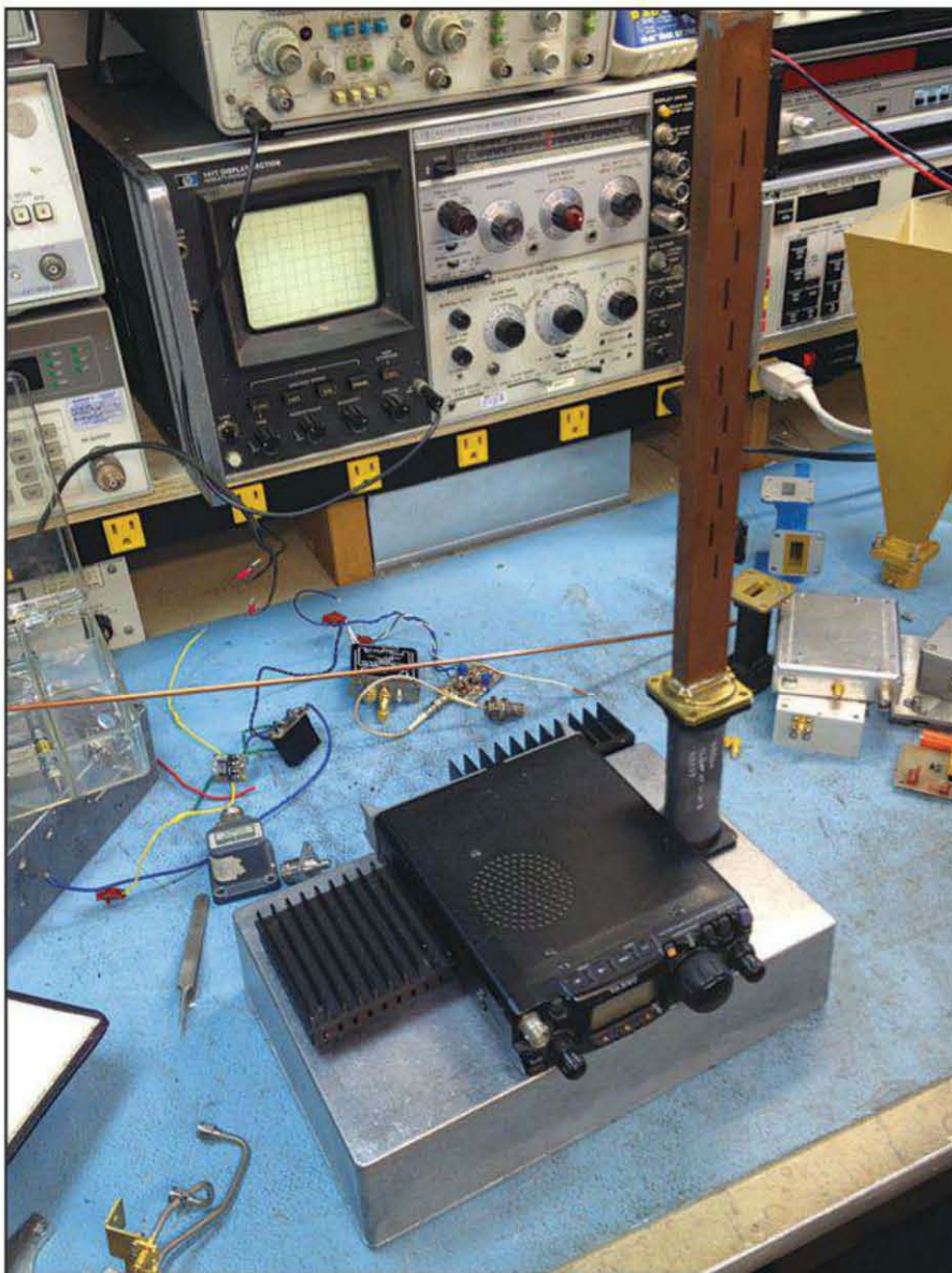
Photo 2— Dennis Kidder, W6DQ, is building this 10-GHz transverter system from a kit as well as surplus parts. The unit is "modular" to simplify upgrades and repairs. Frequency multiplication to the microwave bands, filters and transceiver basics will be taught with the microwave gear. (Photo by Dennis Kidder, W6DQ)
