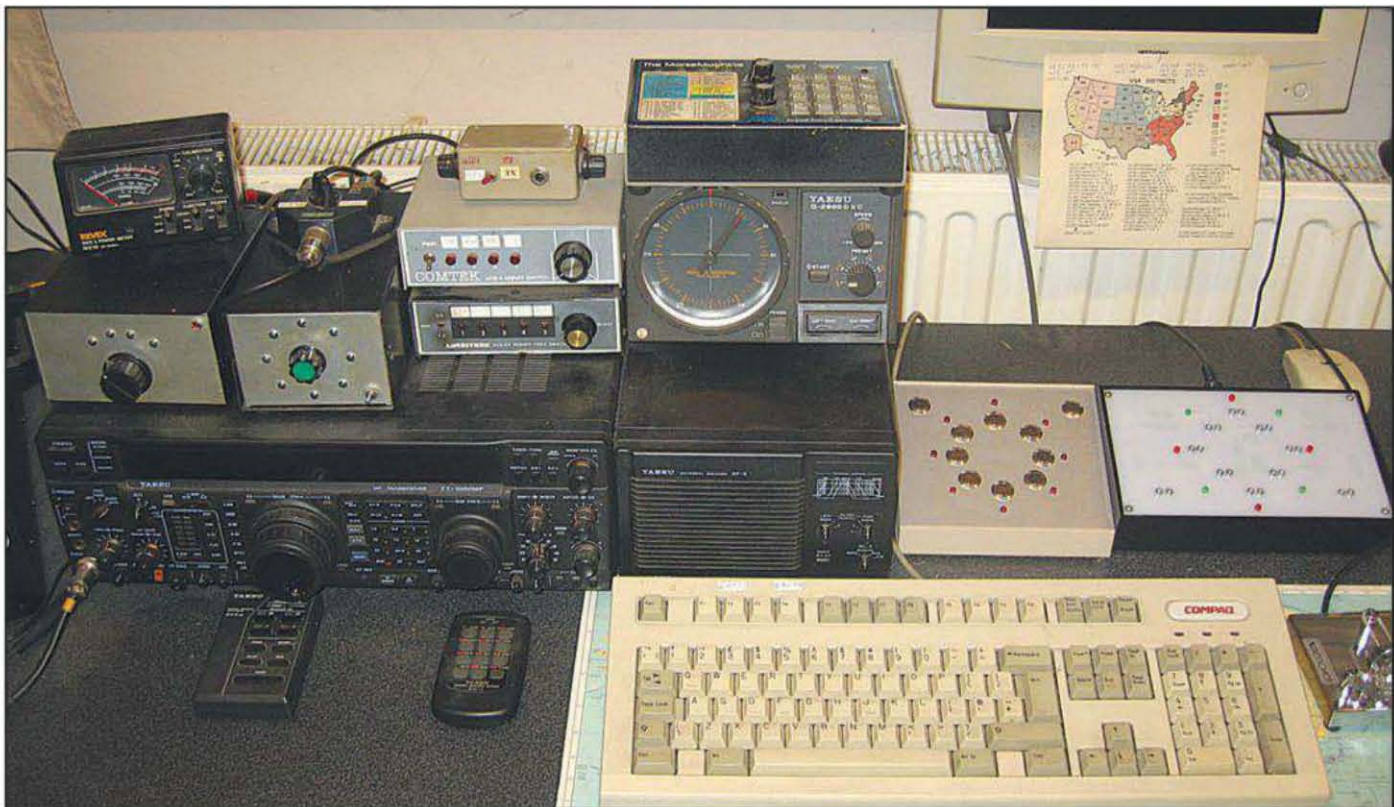
Photo E— Overview of the different switchboxes. On top (middle) of the FT-1000MP radio is the old rotary switch version (to the left of that is the homebrew K9AY control box). To the right-hand side of the speaker are the two new versions: first the pushbutton version, followed by the touch-button switchbox.
