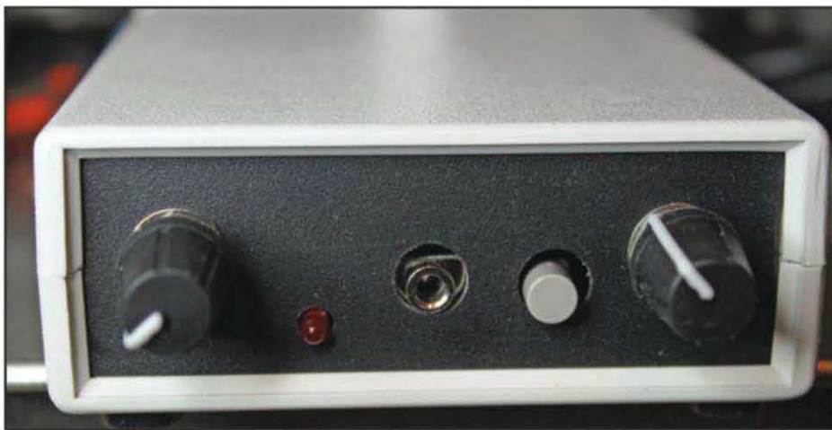
Front panel of the CW Scrubber before controls are labeled.
