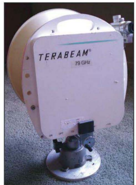
Photo 3— A pair of 79-GHz transverters will be shown by Tony Long, KC6QHP. It is housed in a surplus point-to-point wireless link chassis and dish antenna unit. (Photo by Tony Long, KC6QHP)
