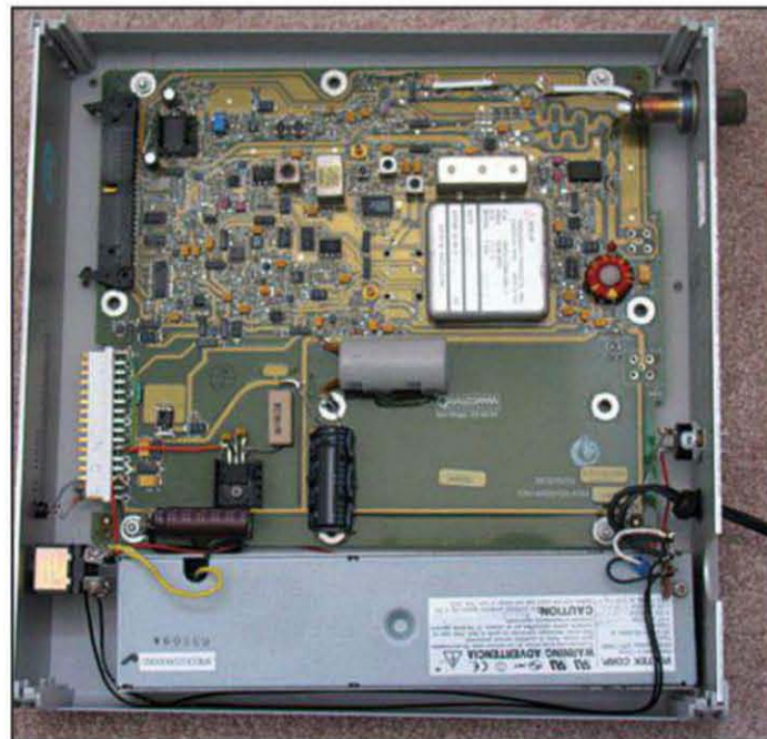
Photo 6– One of the few non-interactive displays in our booth. The “Magic 1152 Board” is a modified frequency synthesizer unit, generating 1152 MHz. This demo will describe the importance of and practical uses for harmonic radio energy.
