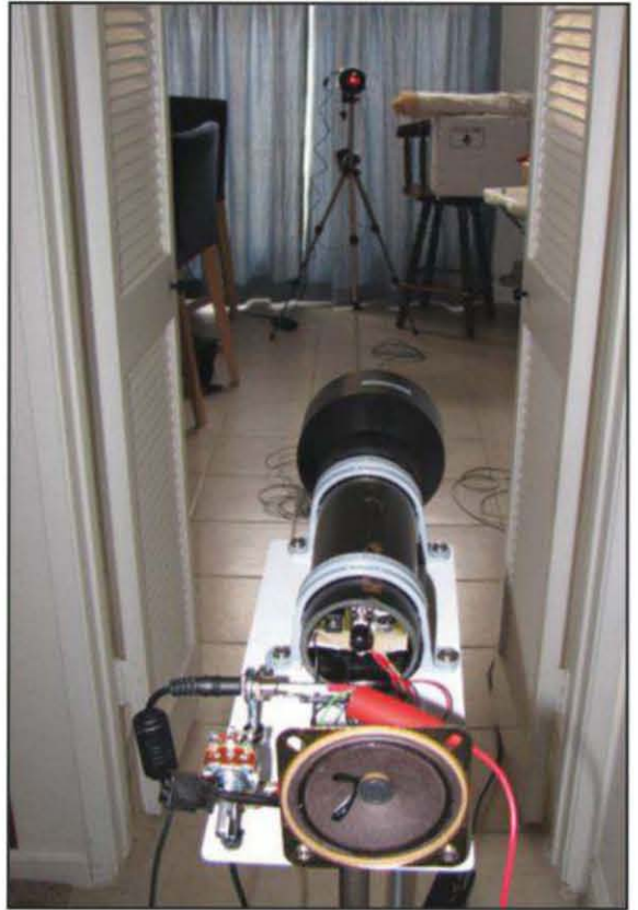
Photo. 1— This is a picture of my full-duplex laser communicators under test in my dining room. Visitors will learn about full- versus half-duplex, pulse-width modulation and other concepts.
