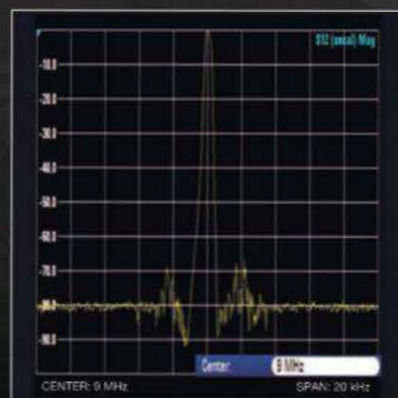
Characteristics of the Crystal Roofing Filter (300 Hz)
