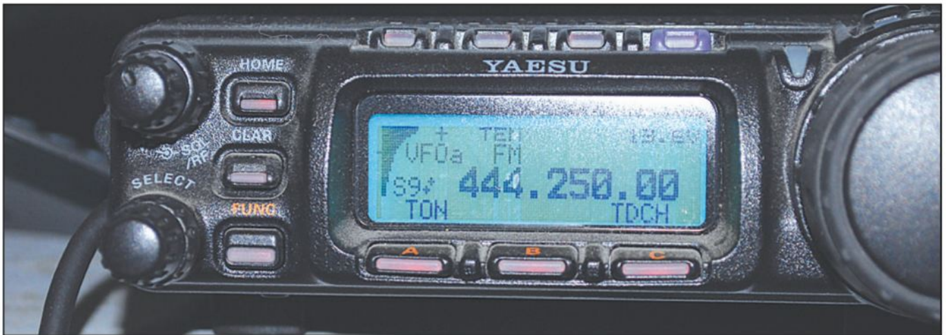
Photo B— A Yaesu FT-857 S-meter showing a signal of S-9+. (Photos B–D by KOØZ)
