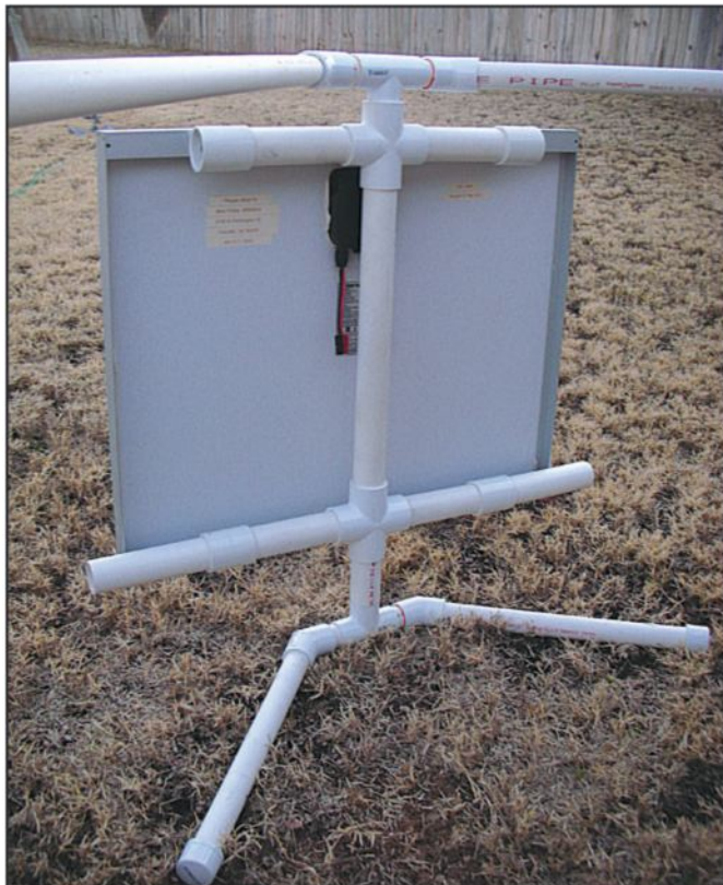
Photo K– Panel mounted on the stand and the upper hub attached. The assembly is ready to stand up on its legs.
