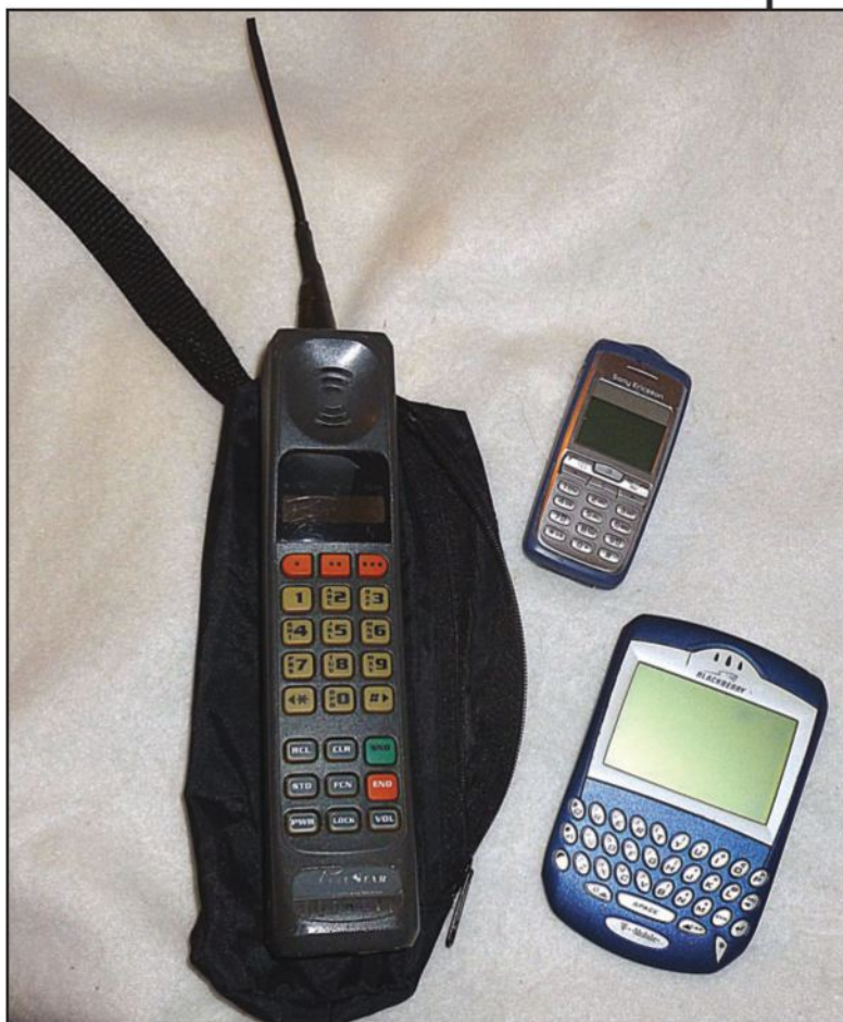
Photo A— Phone technology through the years has evolved to give us much smaller phones with very low-powered transmitters. This requires very sensitive and very low-noise receivers at cell sites.
