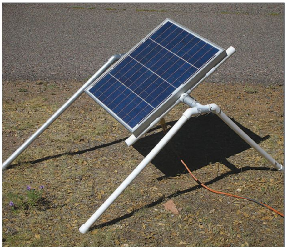
Photo I— The solar tracking stand set up in its summer configuration to capture the most sunlight.
