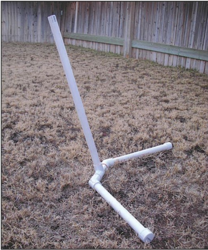
Photo J– The stand ready for the solar panel spindle to slip over the top. Stand on the lower legs to prevent the panel from toppling over onto the ground.
