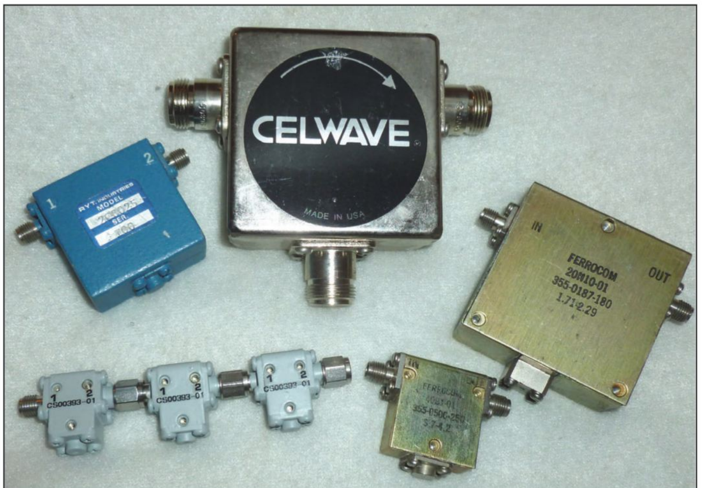
Photo C— Ferrite circulators permit RF to flow in only one direction, but are subject to noise-inducing saturation if over-driven.
