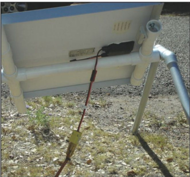
Photo R— The author uses a standard outdoor extension cord as a power cable, along with adapters at each end to convert the AC plug and socket to DC PowerPole® connectors. See text for important details.
