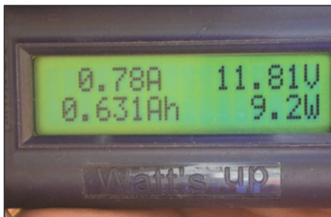
Photo P– The power drops by 74% to about 9 watts when the panel is shadowed 10%. A little shadowing has a big effect on PV panel output.
