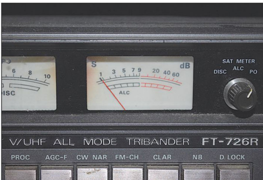
Photo D— Yaesu FT-726R with an analog S-meter.
