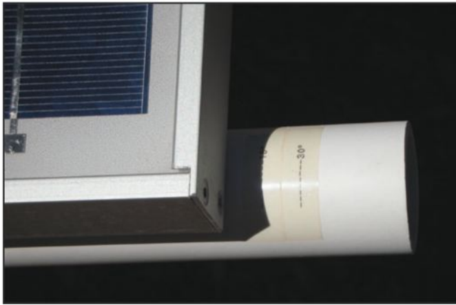
Photo Q— Markings for sun angles of 15 and 30 degrees allow the user to determine when it is time to move the solar panel to its next position.
