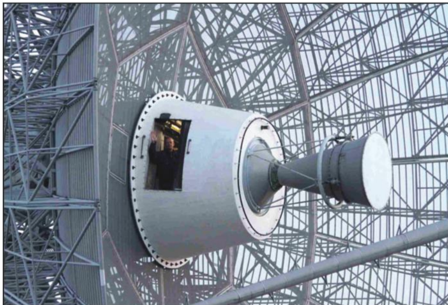
Photo 6— SM6GXV in the compartment of the Onsala 25-meter dish where TX/RX is attached to the feed. SM6CKU photo.
