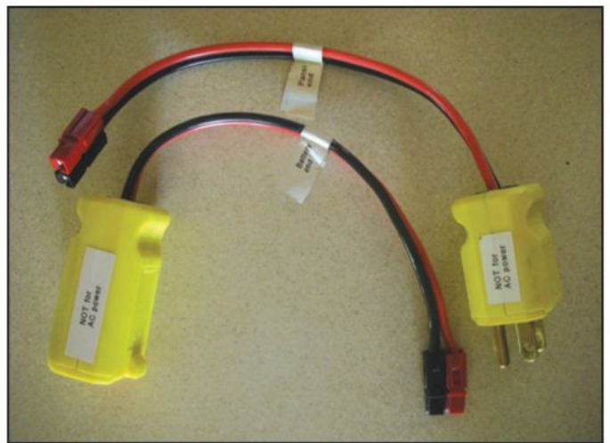
Photo S— Adapters to use a standard utility power cord to conduct the DC power from your PV panel to your charge controller.
