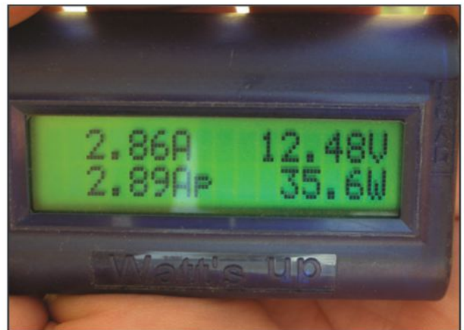
Photo N– Power output for author's unshaded panel is about 36 watts.
