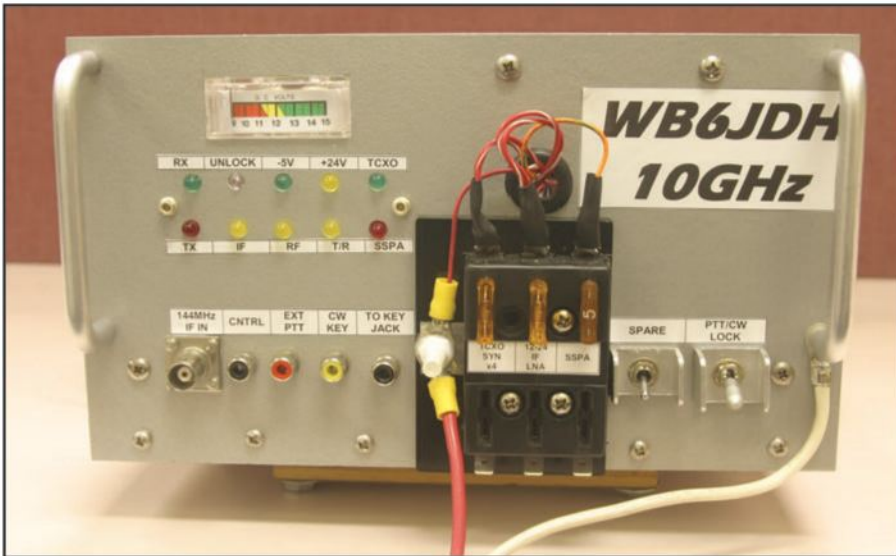
Figure 2. Surplus material and previously exotic parts like microwave mixers are easier to obtain these days. This X-Band system has a receiver noise figure of 0.7 dB, with transmit power of 900 mW measured at the antenna port. An 18-inch reflector is attached to the front of the chassis box with machine screws.
