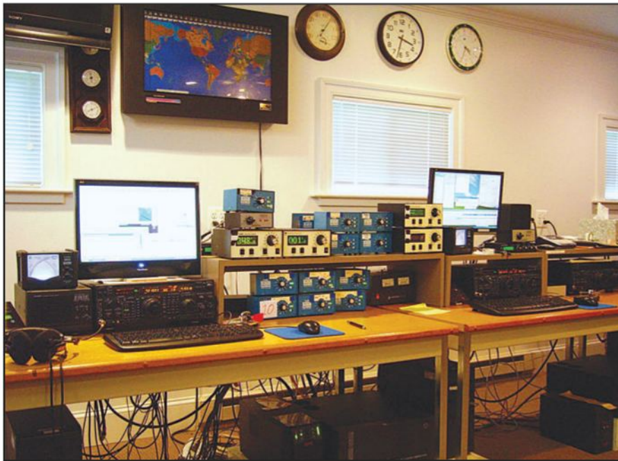
Photo B. Here are two of the three remote operating positions at K4VV. At least one operator is always on duty to deal with technical hiccups. The station can be configured from single-operator to multi-multi. (Photos courtesy of Mike Lonneke, W0YR)
