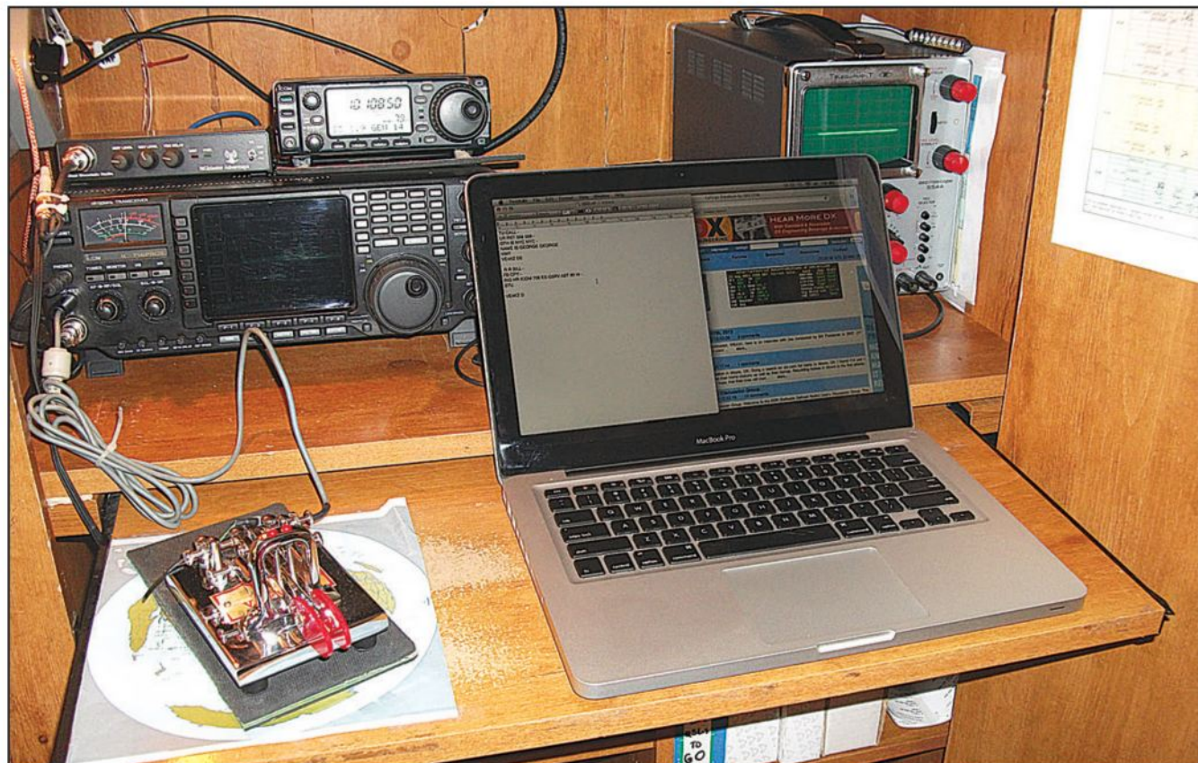
Photo D. The main operating shelf with the two transceivers and the oscilloscope used to monitor transceiver and amplifier output sampled at the input to the AMU.
