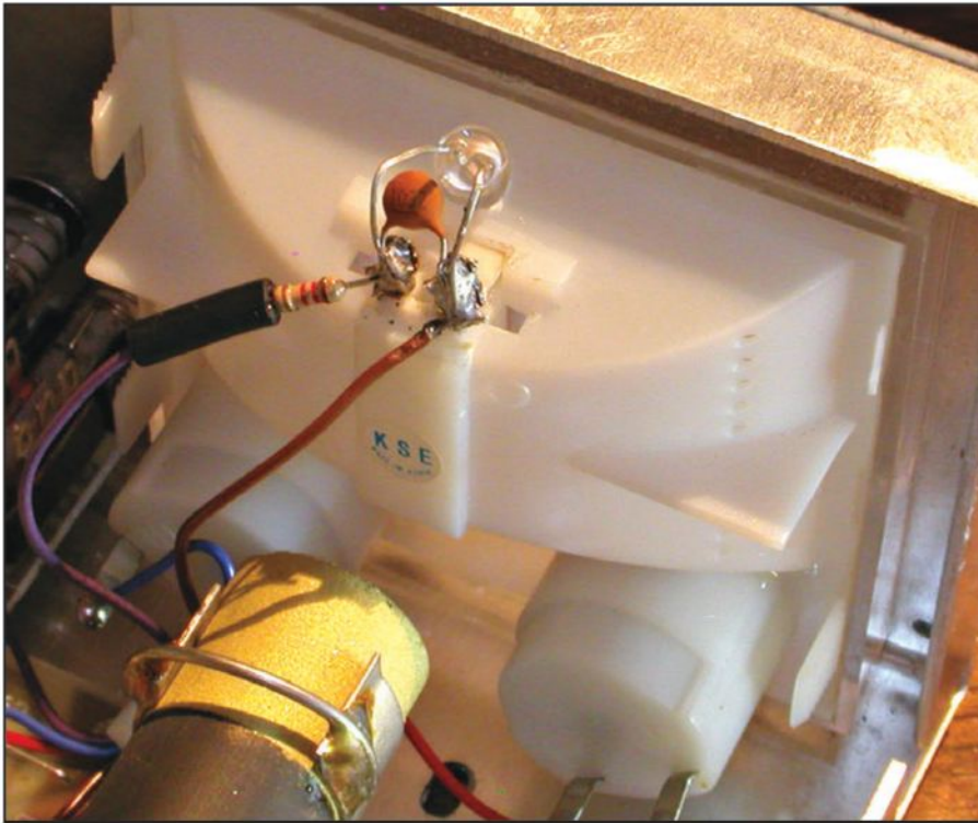
Photo F. A close-up of the meter's plastic housing shows the LED pressed through the newly-drilled hole—like an ostrich with its head in the sand. A piece of discarded black wire insulation covers the exposed resistor lead in the purple 12-V DC line. The brown wire goes to ground. The round disc-ceramic capacitor across the tabs in the background is apparently for bypassing RF to ground. It was part of the original incandescent circuitry, and we opted to leave it there.
