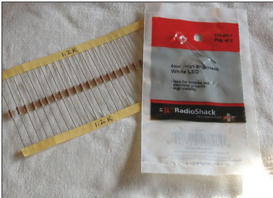
Photo B. Only two parts are needed to add luminescence to any 12-V DC-powered project: a 1.2K-ohm resistor and an LED. A package of brown, red, red resistors was pulled from the K16SN junk box, while the LED was obtained from RadioShack®.
