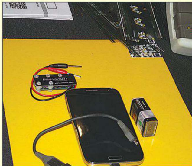
The Voltset Mini voltmeter works with an Android smartphone to provide users with a credit-card sized voltmeter.
