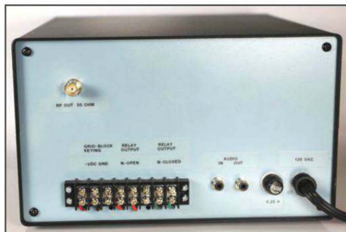
Photo C. Rear view of the VFO, showing connections for keying, relays, and audio.
