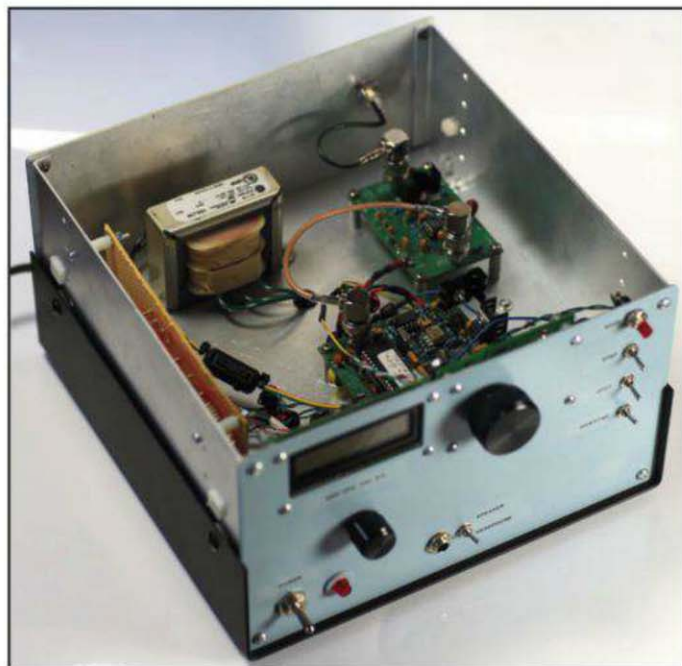
Photo A. The DDS VFO (Version 2) is intended to be a nearly plug-and-play replacement for the classic (but very drifty) Heathkit HG-10 VFO. It also provides voltages and switching needed for use with multiple receivers. (Photos courtesy of Joe Havrilla, N3DHD)
