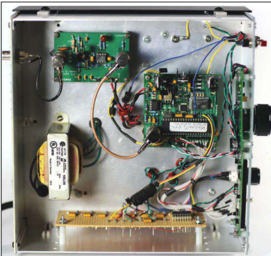
Photo D. Top view of the DDS VFO. Note the transformer for the built-in power supply (one difference from the classic HG-10, which got its power from the transmitter).
