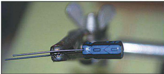
Photo E. An electrolytic (polarized) capacitor. Notice the marking indicating negative and that the negative lead is shorter than the positive lead.
