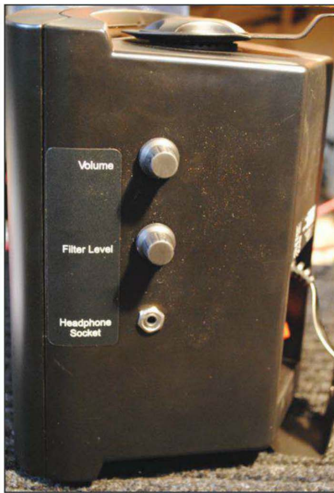
Photo C. Side view, showing volume and filter level controls, along with a headphone socket if you want to get the benefits of audio DSP while using a headset.
