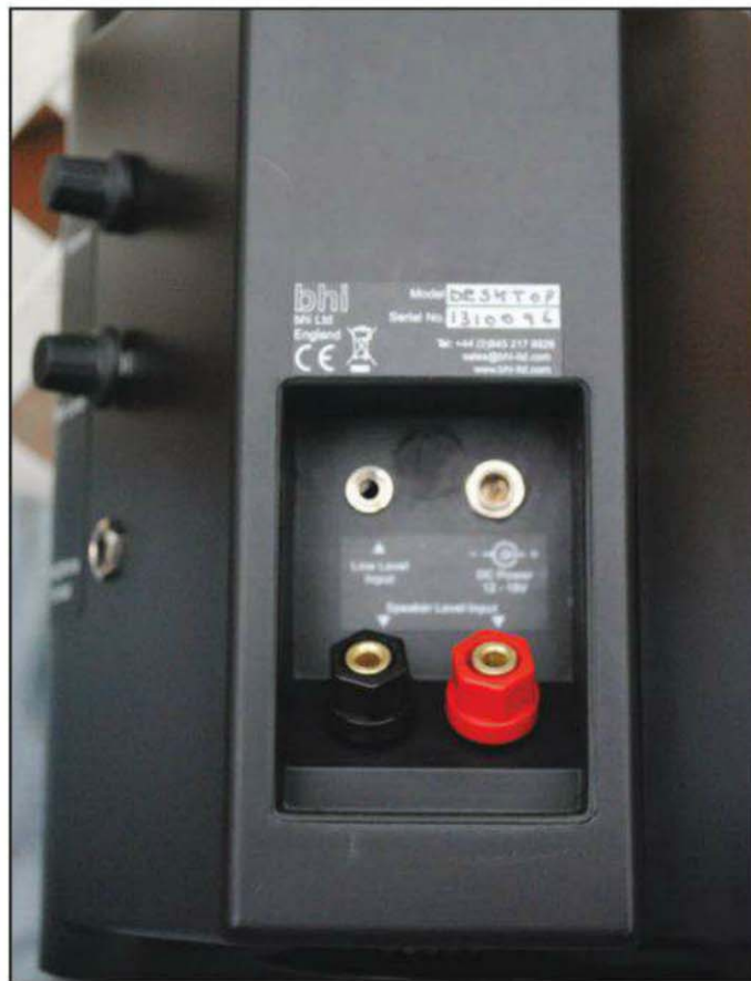
Photo D. Rear view showing speaker level inputs on the bottom row of connectors, with line level input at upper left and power connector at upper right.
