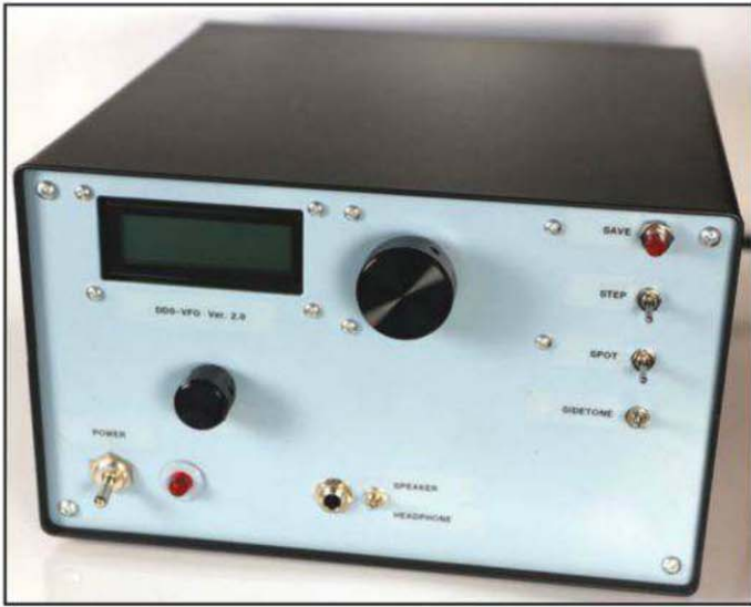
Photo B. Front view of K6CTW's DDS (direct digital synthesis) VFO for his classic Heathkit DX-60 transmitter.
