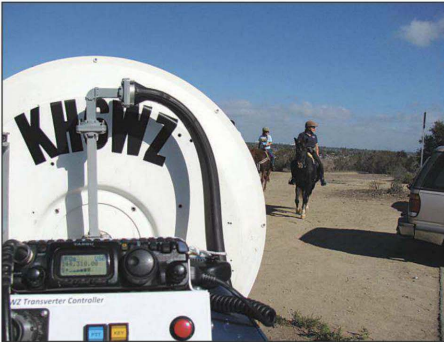
Photo B. A 10-GHz transverter system can be quite compact and yet have very good performance. This was my first operating location, Huntington Beach, CA DM03xq.
