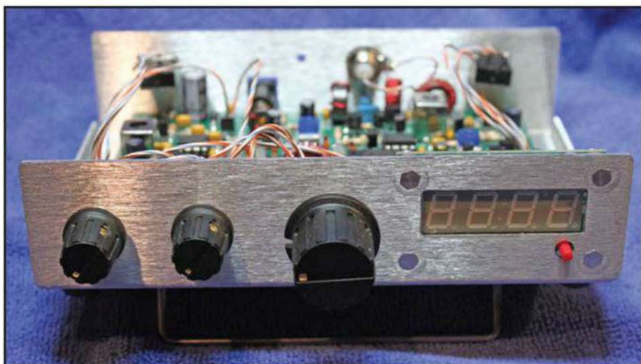
Inside look at the front panel of the Survivor featuring the Digital Dial kit on the left. ↓
