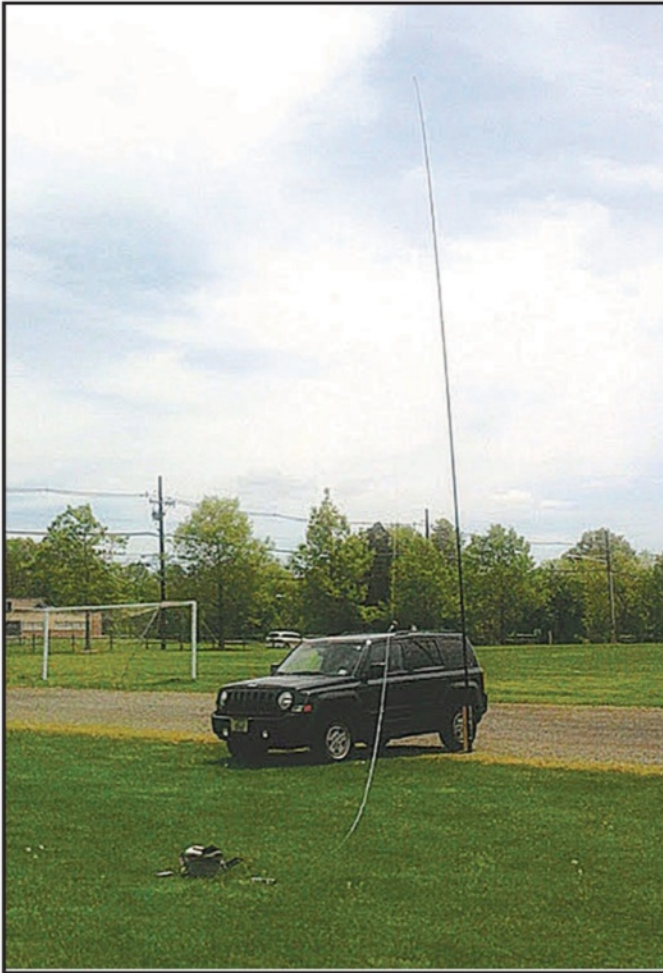
Photo B. No picnic table? Try operating from your car. In this photo, we see a quick-setup antenna supported by a mast with a baseplate that sits underneath a tire.
