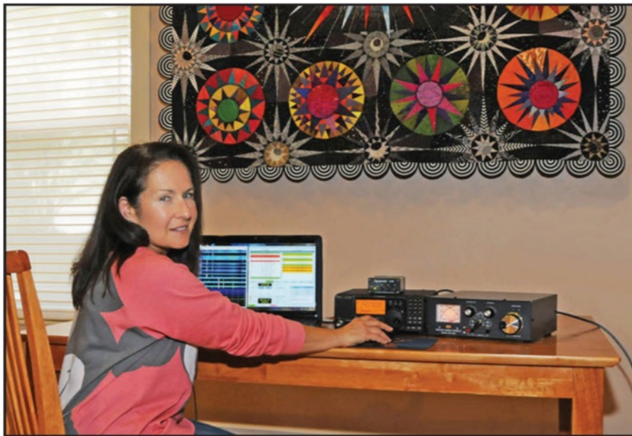
Photo B. Shirly Regis, W9OMG, operating JT9 at 5 watts with great results from her home in North Florida using an ICOM IC-718 and a temporary vertical antenna.
