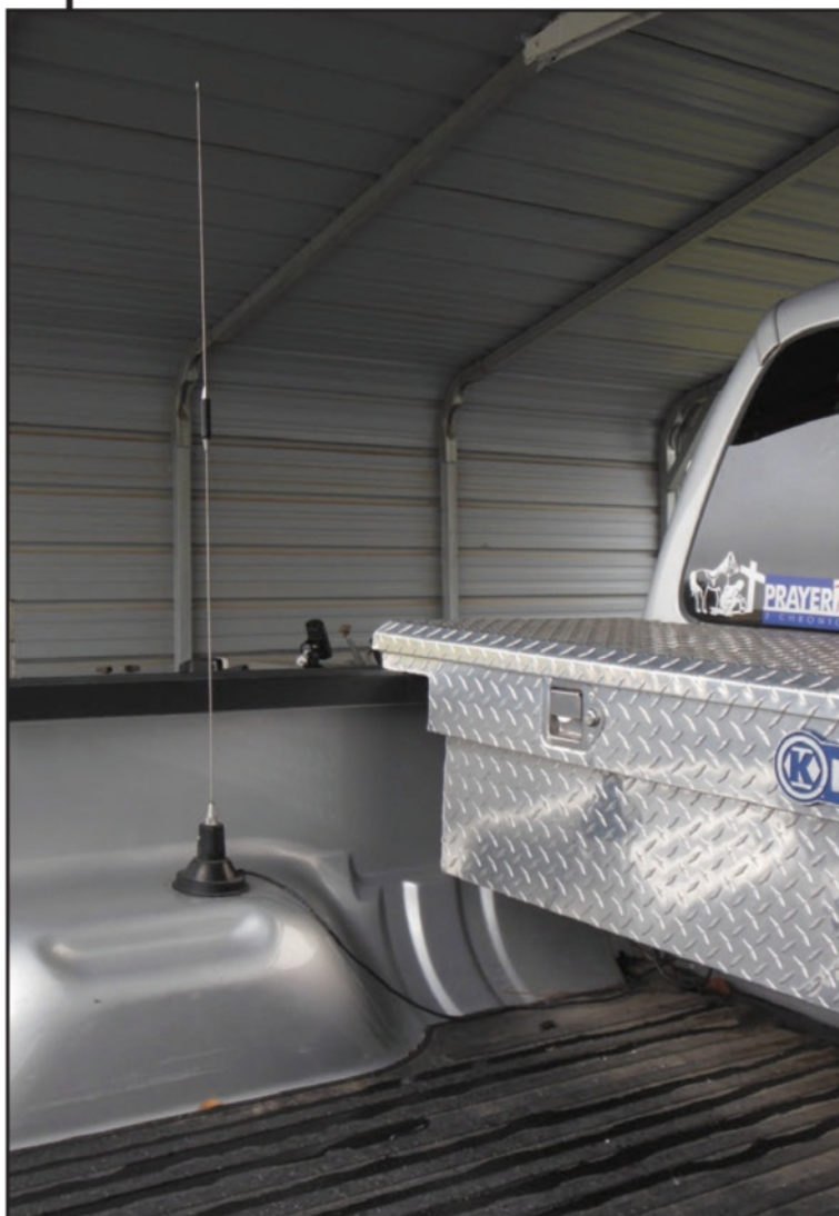
Photo 1. Simple installation of magnetic mount dual-band on the wheel well.
