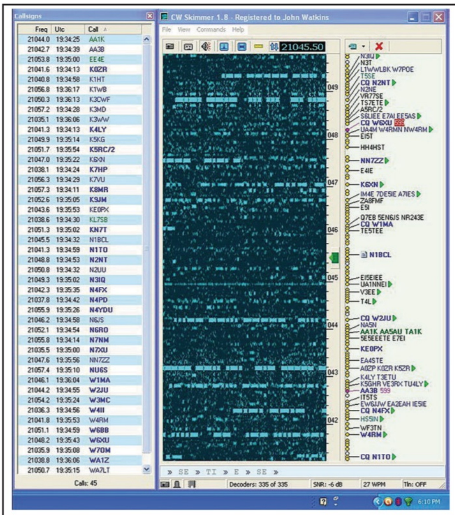
Fig. 1. Screen capture of CW Skimmer running on the right half of the screen. Taken during the heat of Sweepstakes action, you can see the list of stations that have been identified by the skimmer. They are sorted alphabetically by callsign.
