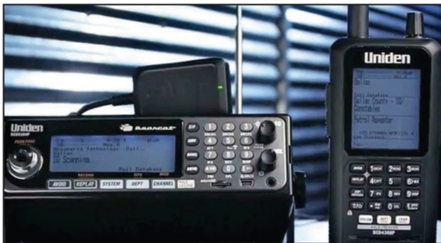
Photo A. Uniden's new BCD536HP, left, and BCD436HP scanners take the HomePatrol concept to a whole new dimension. New features and integration opportunities are all over this radio! (Internet screen grab)
