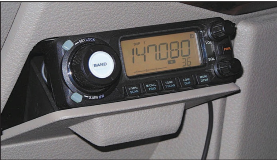
Photo 3. Control head lying on the ashtray door with the door spring holding it in place.
