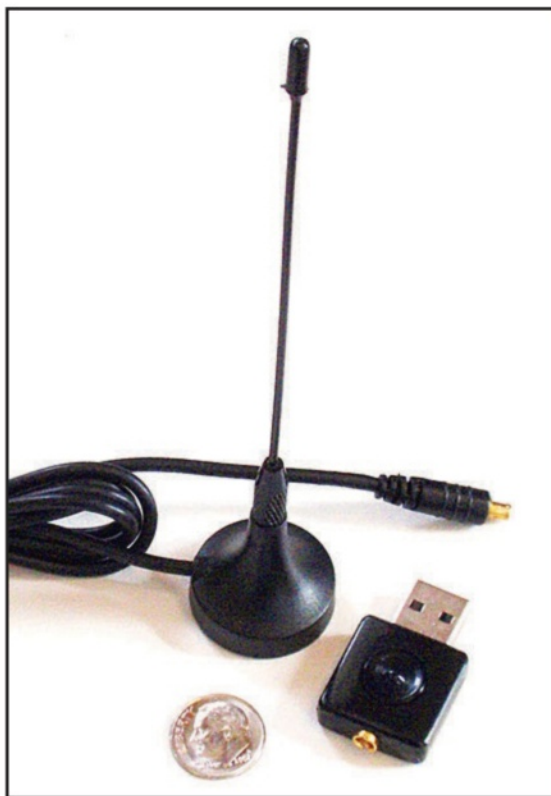
Fig. 1. The USB Dongle and unmodified antenna. The dime is there for scale. This particular unit receives from 52 to 2202 MHz, with a gap between 1102 and 12324 MHz. The antenna is only useful for the end connector that mates to the Dongle.
