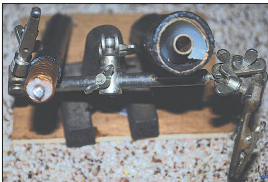
Photo D. Some examples of 1/2-inch hardline (left) and 7/8-inch hardline (right). WS9V uses 1 1/4-inch hardline in his repeater system.
