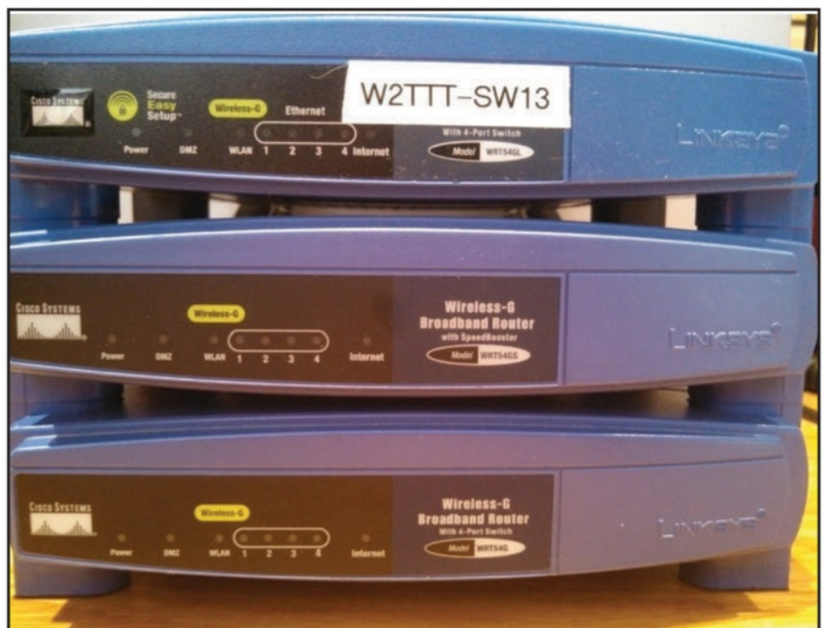
Photo A. Three different models of Linksys routers (from top, WRT54GL, WRT54GS and WRT54G) that are ideal for use as nodes in Broadband/Hamnet (HSMM-MESH) networks.
