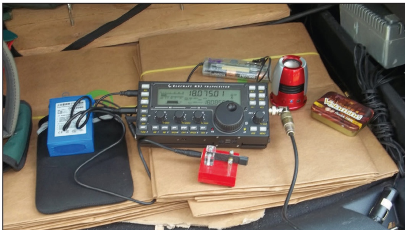
Photo E. The author's lunchtime-portable QRP station, built around his Elecraft KX-3 transceiver.
