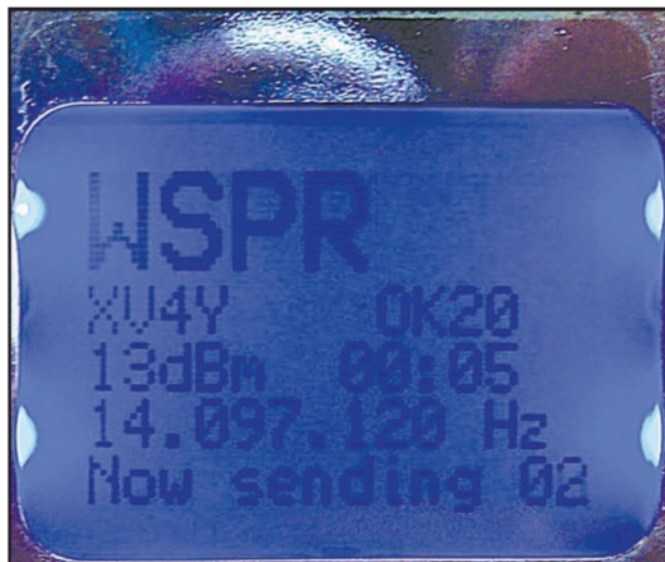
Photo A. Screen of the author's WSPR beacon while transmitting a Weak Signal Propagation Reporter signal.
