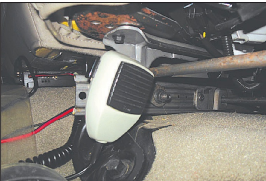
Photo 4. Microphone in its nesting place under the seat. The power wires can be seen behind the mic going to the main body.
