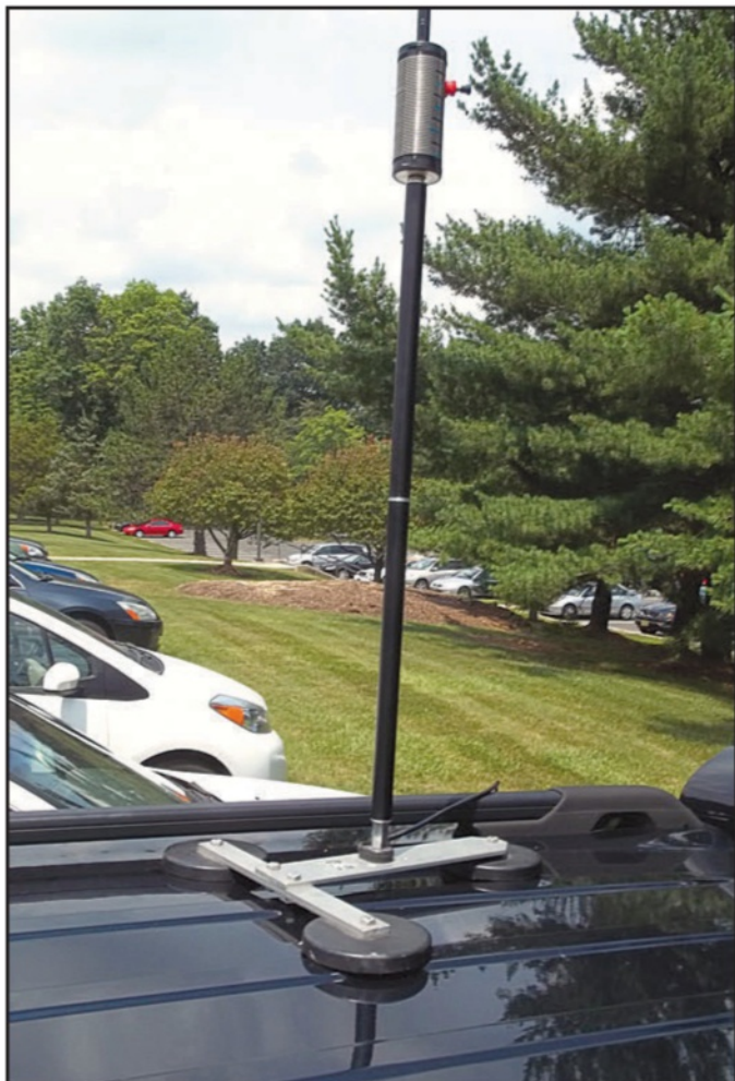
Photo D. A Buddistick attached to a heavy-duty magnet mount can be a very effective antenna that's quick to set up and tear down. Also, no counterpoise is needed as long as your vehicle has a metal roof.
