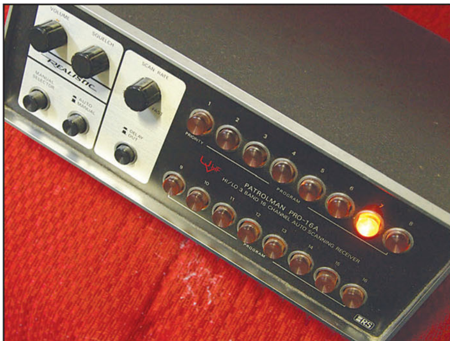
Manufactured by Realistic between 1976 and 1977, the RadioShack® PRO16A VHF/UHF scanner would be a great listening post addition even today. Its 16 channels can be set to cover frequencies from 30 to 50, 148-174, and 450-512 MHz — spectrum that is rich with activity.
