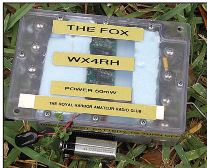
Some clubs have a "foxbox" that is used for every foxhunt, whoever hides it. This 50-milliwatt transmitter awaits members of the Royal Harbor Amateur Radio Club in Tavares, Florida during Foxhunting Weekend. (Photo courtesy Ted Luebbers, K1AYZ)
