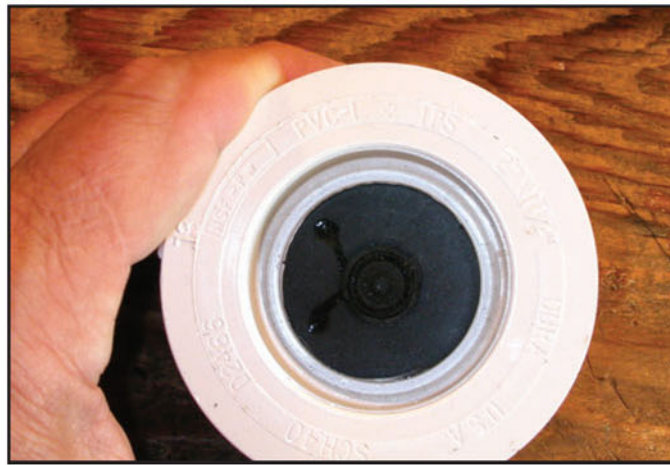
Here's how the 2-inch diameter speaker looks from the 1-and-a-quarter-inch side of the PVC coupler.
