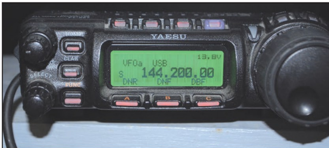
Photo A. A Yaesu FT-857 is an example of an all-mode rig covering HF, VHF, and UHF.
