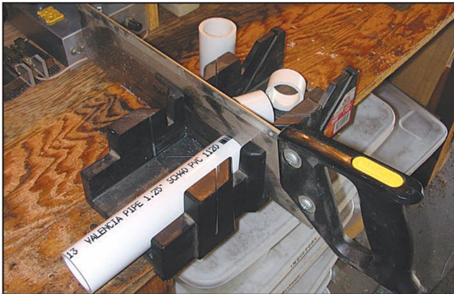
The cut-and-try method of scientific experimentation was used to find the optimum length of PVC pipe for resonance at a 630-Hz audio tone at K16SN. A mitre board and hobby saw made the job neat and easy.
