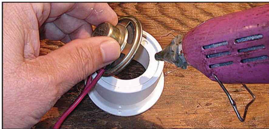
A hot-glue gun was used to apply the adhesive needed to hold the 2-inch-diameter speaker in place at the base of the PVC coupler. This 2-inch to 1-and-a-quarter-inch PVC pipe coupler was the perfect housing to mount both the speaker and the 1-and-a-quarter-inch PVC speaker cavity.
