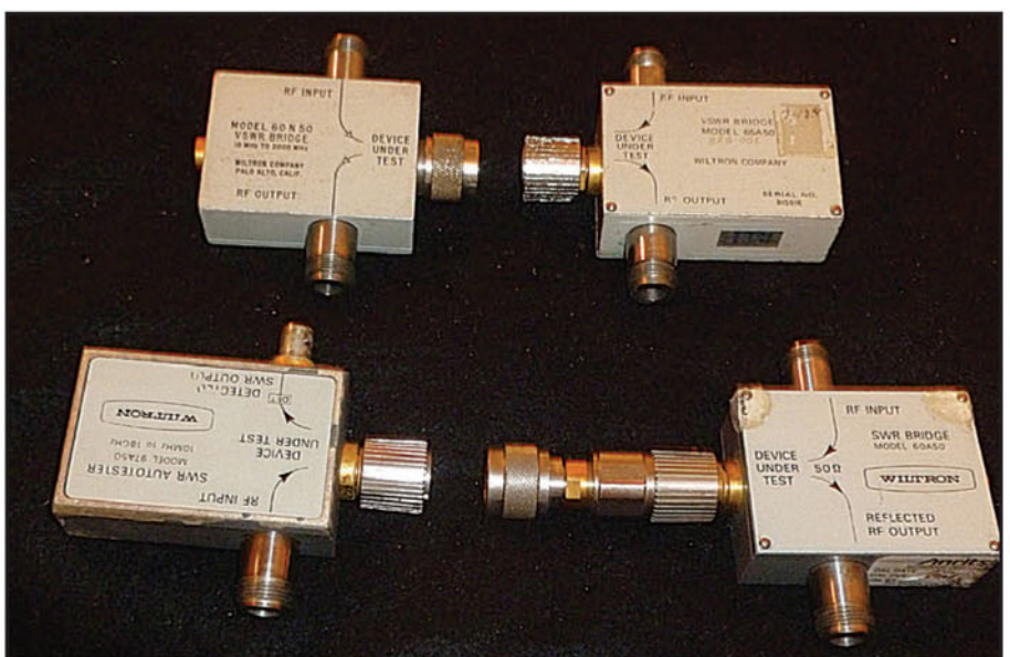
Photo F. Resistive bridges for measuring SWR
