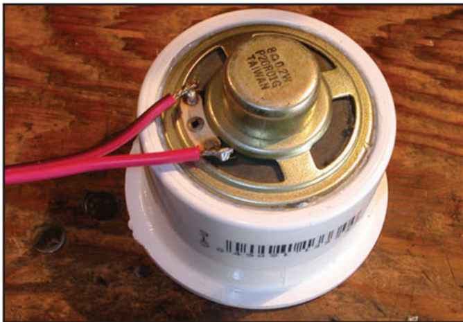
Once the 2-inch-diameter speaker was glued in place, standard audio speaker wire was used to create the link between the audio source and the resonant speaker.
