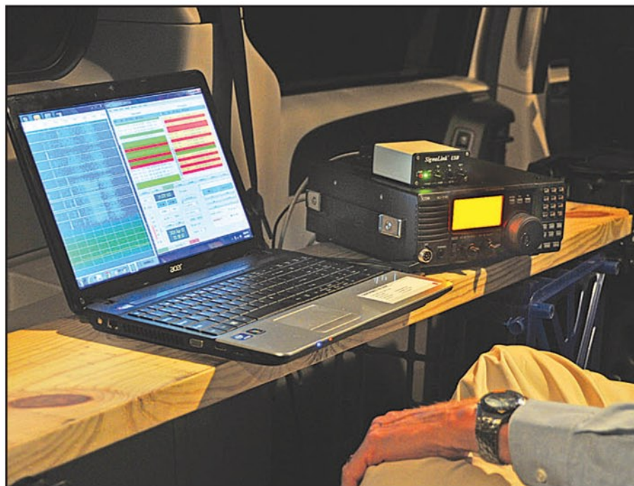
Photo C. A waterfall display full of JT9 signals is a good start for portable operating.
