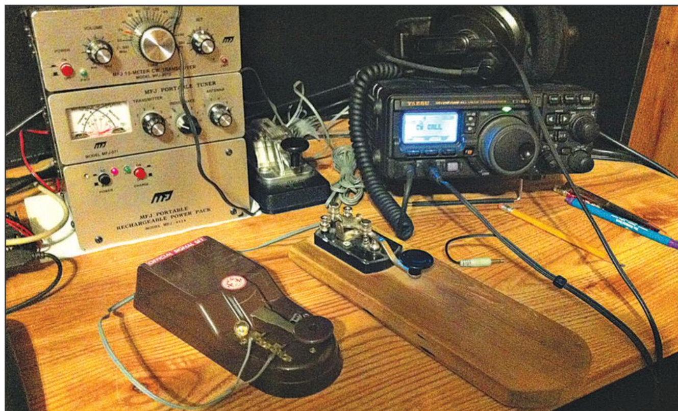
Figure 7. The Boy Scout straight key in action.
