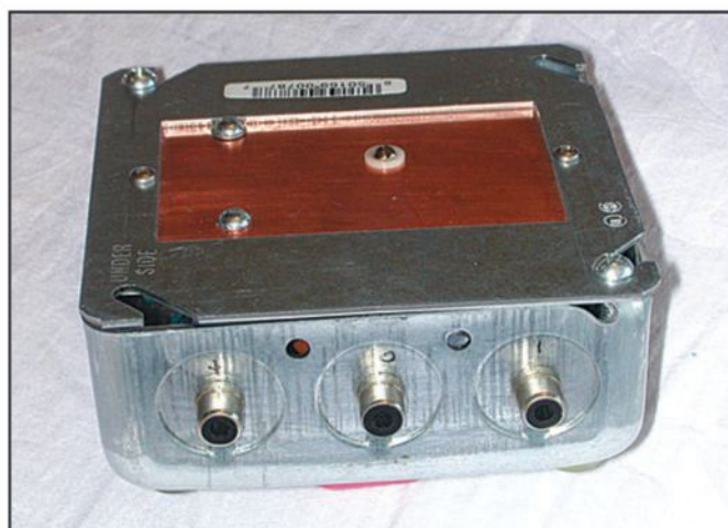
RCA-style phono jacks were mounted on the Miniboosts' back panel for, from left, 12V B+ power, Miniboosts RF output, and transceiver input drive.
