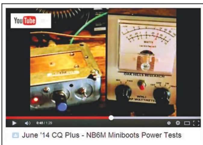
A short video on the YouTube CQ Channel shows the 2014 NB6M Miniboosts' power output with just 850mW of RF drive from a NorCal-40A transceiver. WATCH and LISTEN: < http://youtu.be/Goiz0q8qnWY >.
