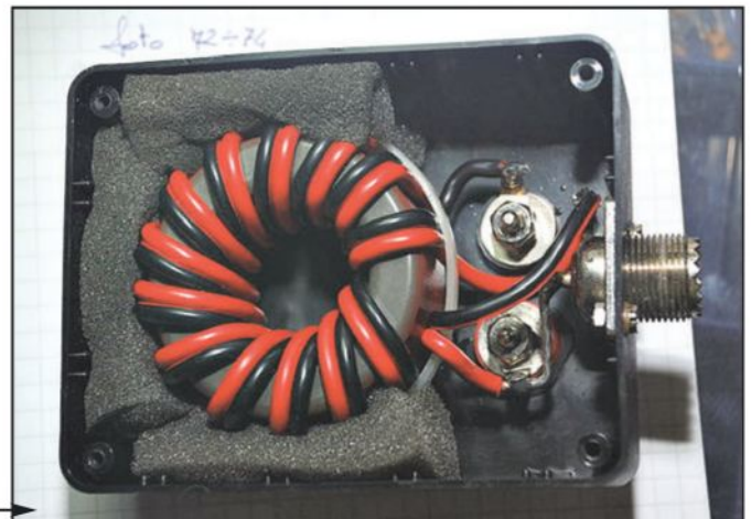
Photo B. A toroid wrapped with insulated wire is the heart of this 4:1 voltage balun. (Courtesy of Wikimedia Commons)
