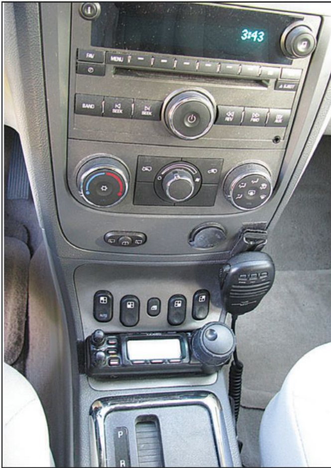
The HHR's interior is a challenge, but WØRMS found a spot that was "just right" for a control head and microphone mount. The speaker is also in a good location. Note how everything is located away from airbag deployment zones.
