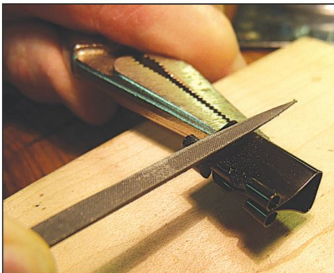
Photo C. Modifying the clip by filing the loops that hold the wires in place.
