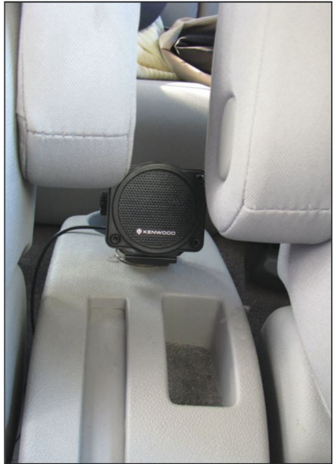
The HHR's interior is a challenge, but WØRMS found a spot that was "just right" for a control head and microphone mount. The speaker is also in a good location. Note how everything is located away from airbag deployment zones.
