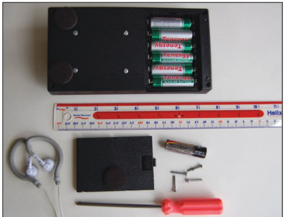
Photo C. Six AA batteries provide all the power this mini-QRP rig needs. Earbuds (lower left) and an antenna are all that are needed for a complete portable station.
