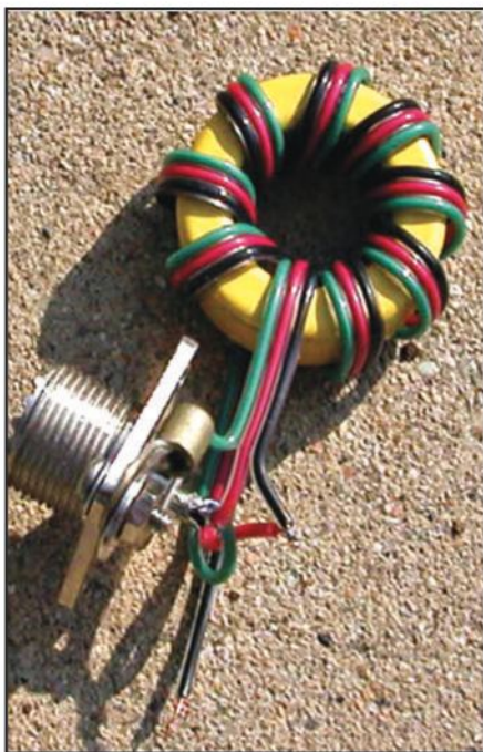
Photo D. If you want to go bare bones for a 9:1 unun, leave out the enclosure and other hardware. It can be as primitive as this — and still work!
