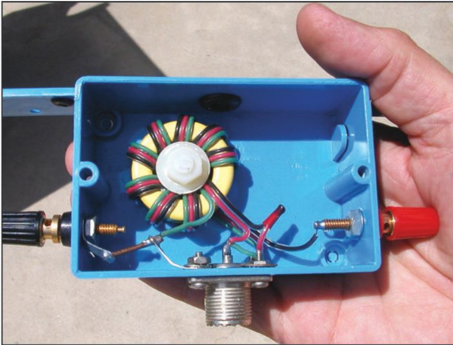
Photo B. With the barest minimum of parts, it is possible to nicely match the 50-ohm output of your transceiver and antenna tuner to a much higher impedance end-fed wire. It's all possible with the 9:1 unun.
