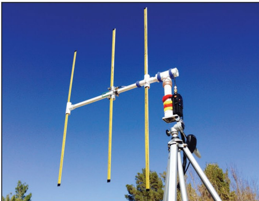
Photo F. RDF tape measure antenna oriented for vertical polarization. It may be rotated for horizontal polarization.
