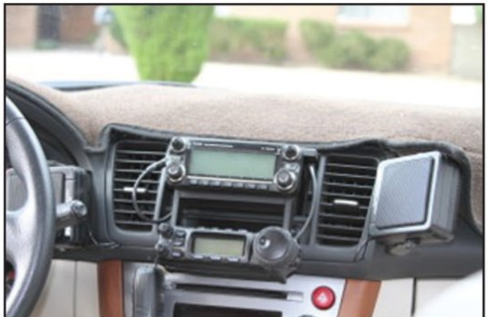
KD7TMX linked two control heads to fit onto the dash of his vehicle. The results speak for themselves in a very nice design that looks like it came from the factory.
