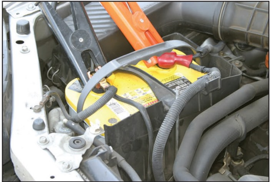
Photo B. A modified set of possibly unreliable jumper cables were used at KH6WZ while roving in the past. A safer and more secure solution was needed.
