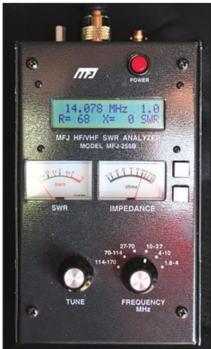
Photo B. The antenna on the van roof is tuned for a perfect match on the 20-meter JT9 frequency.
