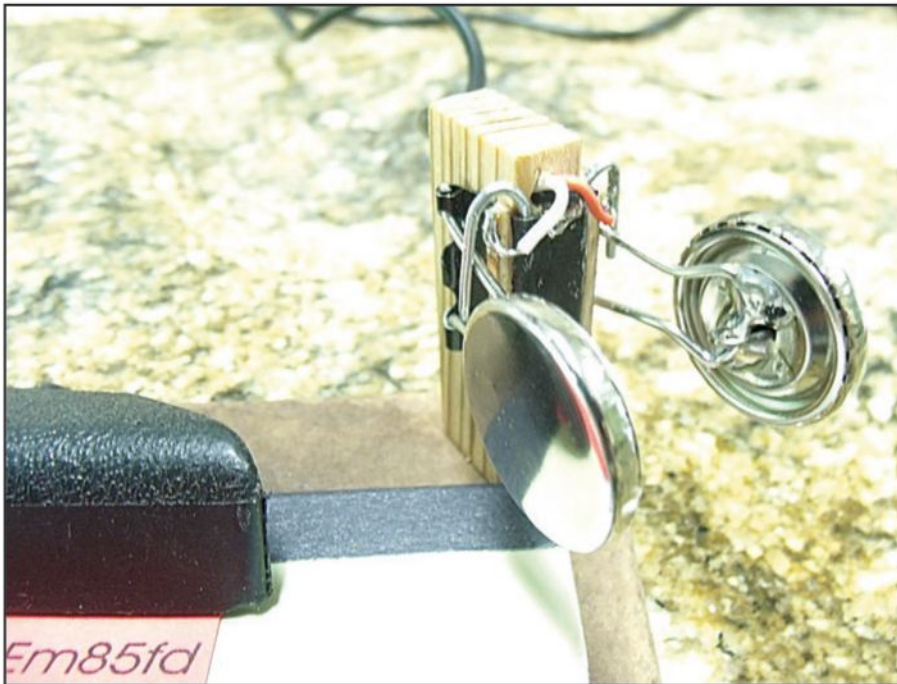
Photo B. The completed paddle mounted to a clipboard ... an idea suggested by Carlton Haycock, K2CMH.
