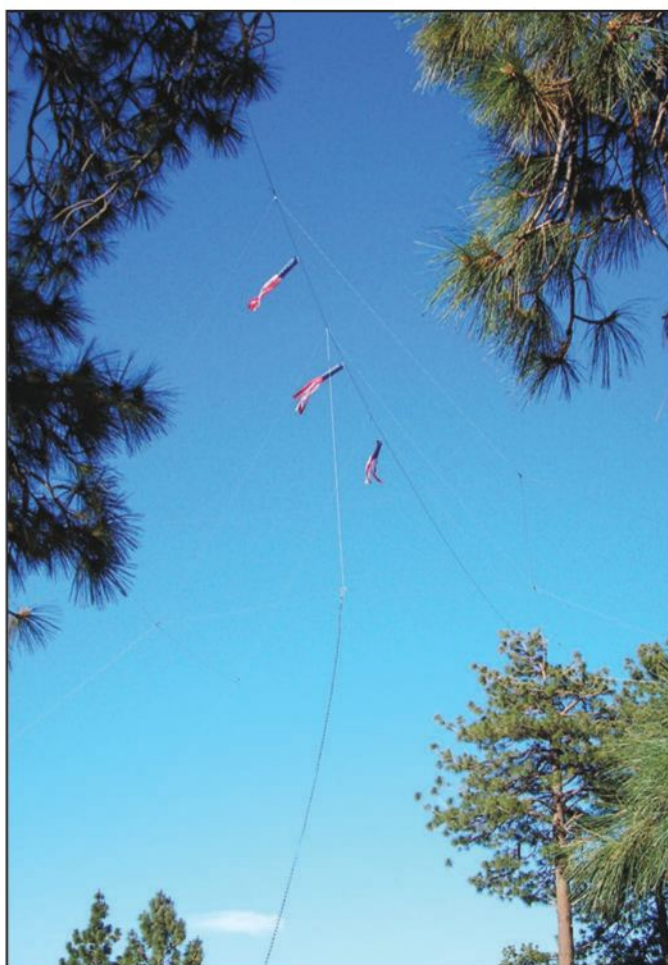
The Zuni Loop Mountain Expeditionary Force's 20-meter delta loop beam strikes a beautiful pose against the California sky, a wonderful antenna when not threatened by an out-of-control wildfire.
