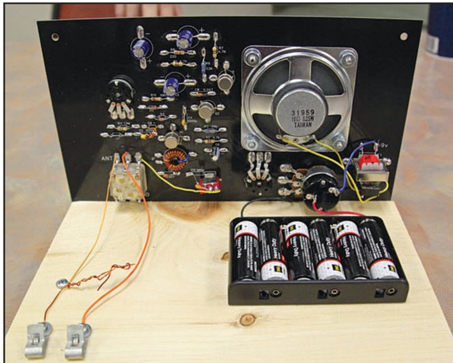
The wiring side of the Ozark Patrol front panel. All parts solder to pads that are pre-mounted on the board.
