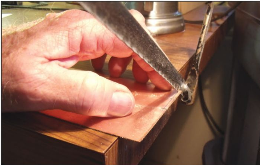
Photo F. Cutting the circuit board strips. It's best to cross-cut first, before cutting lengthwise.
