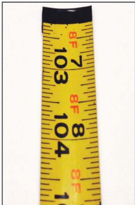
Photo B. Tip of element with black vinyl electrical tape for safety.
