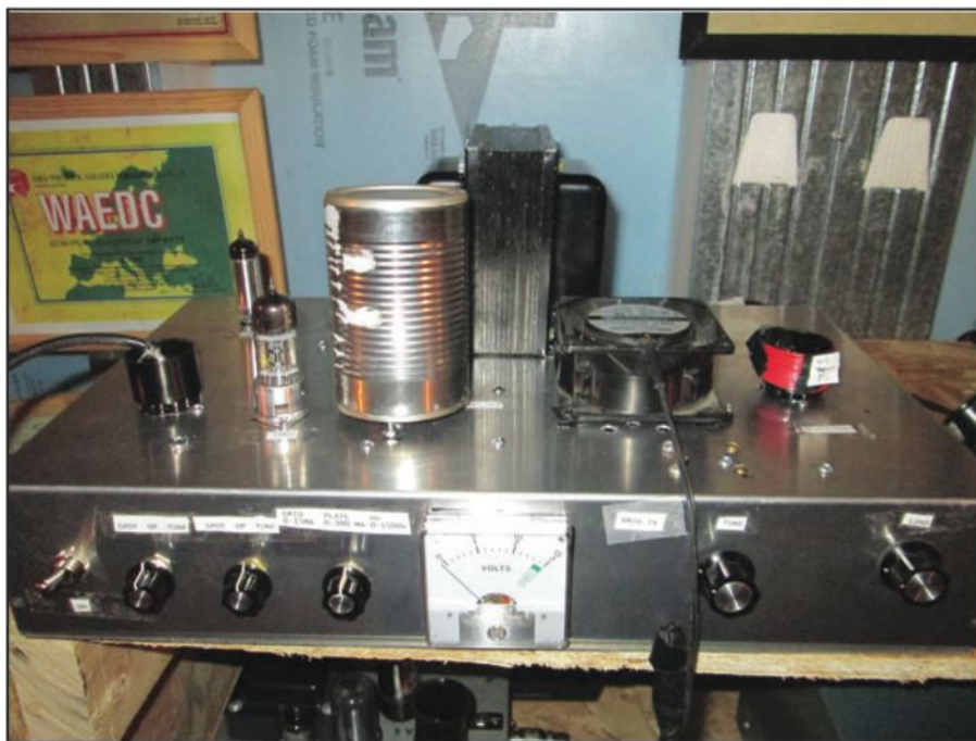
Photo A. Front view of K3MD's “Inexpensive 75-Watt Transmitter,” modified from an ARRL Handbook design of the 1960s and '70s. Note empty veggie can to left of center, shielding the grid coil.
