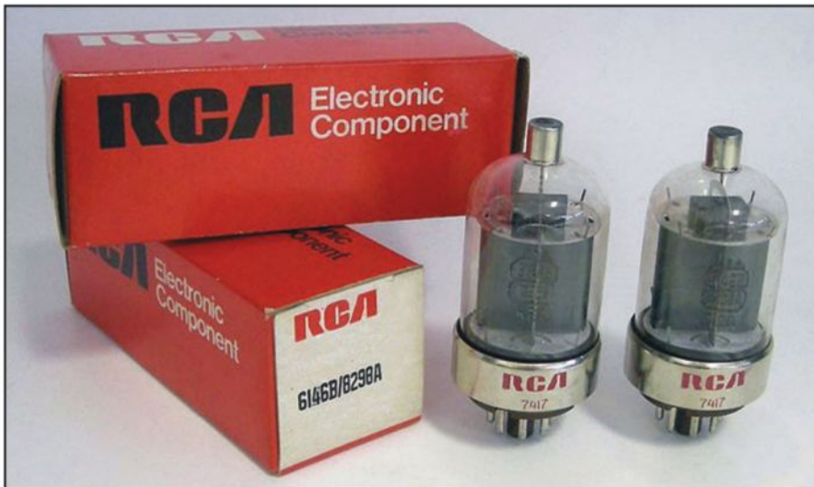
Photo B. A pair of 6146s were the big-time power brokers in the Maestro Audio Power Amplifier circuit featured in the November 1952 edition of Audio Engineering . (Courtesy of Wikimedia Commons)
