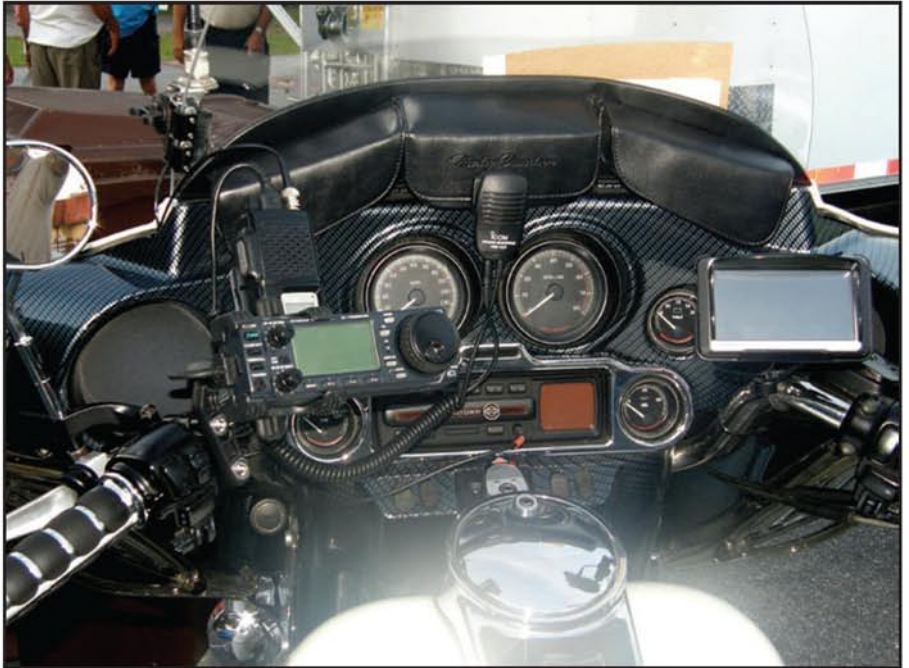
A view from the driver's seat of N4ELI's trike shows his ICOM 706 transceiver which operates on HF, VHF, and UHF.
