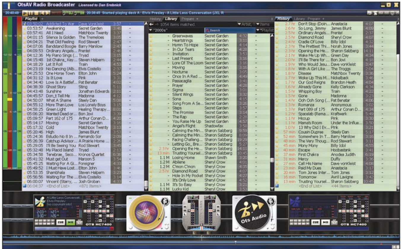
Photo A. Here's what OtsAV Radio Broadcaster looks like. The list on the left is the current playlist. In the middle is the music library and on the right is the history of what was played so far. The decks are on the bottom and the turntable icons can be used for club-like effects, such as scratches. (Internet screen grab)
