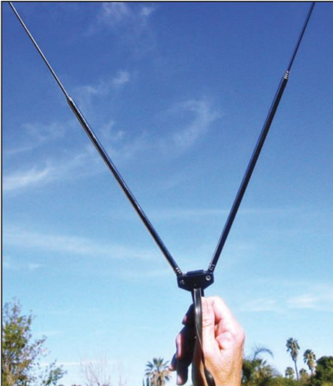
Photo A. Long-forgotten TV rabbit ears are perfect candidates for making a simple, an effective VHF or UHF antenna—of both. It's just the kind of antenna you might need in an emergency. (Courtesy of K16SN)
