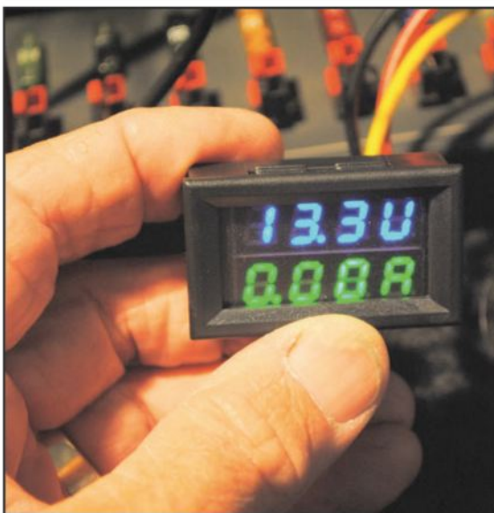
Photo B. Radio City also offers a combination voltage and current meter.
