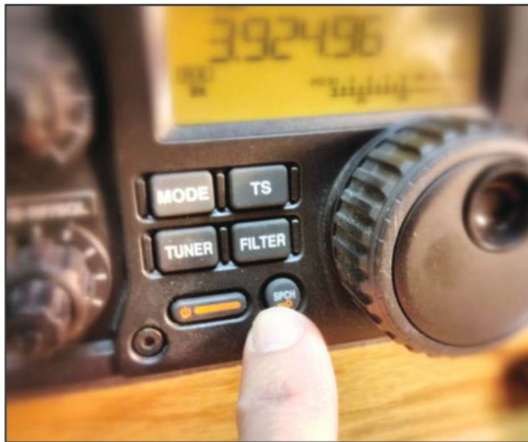
The press of a button on the ICOM IC-7200 and the radio speaks the signal strength and the frequency displayed on the readout.
