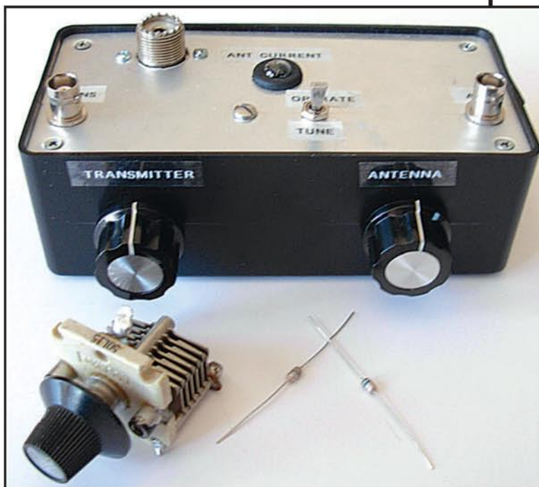
Photo A. KD9SB's 20-meter tuner. For ease of construction, Gary used the molded .56 microhenry inductors shown with the tuner.
