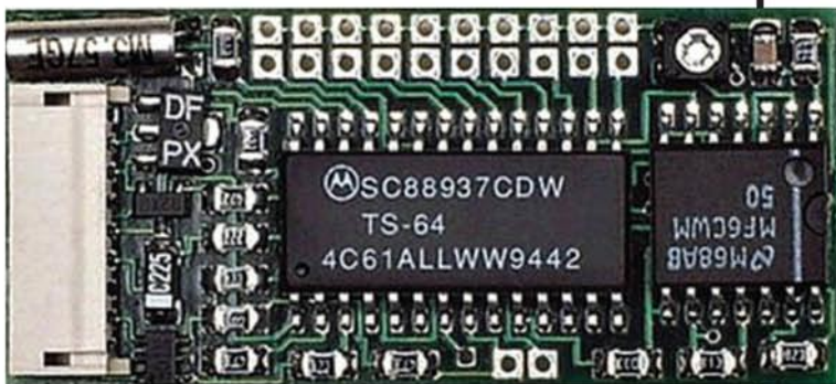
Photo A. "Using something like the TS-64WDS" from Communications Specialists, writes WA3UVV, "you attach the encoding signal to your transmitted audio and pull the decoder input from your receiver's pre-processed audio." (Internet screen grab < http://bit.ly/110Ed6s >.)
