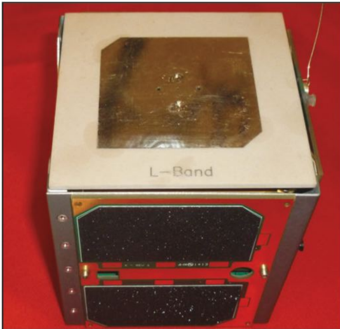
Photo C. AMSAT FOX Cubesat with L and S-Band Patch antennas.
