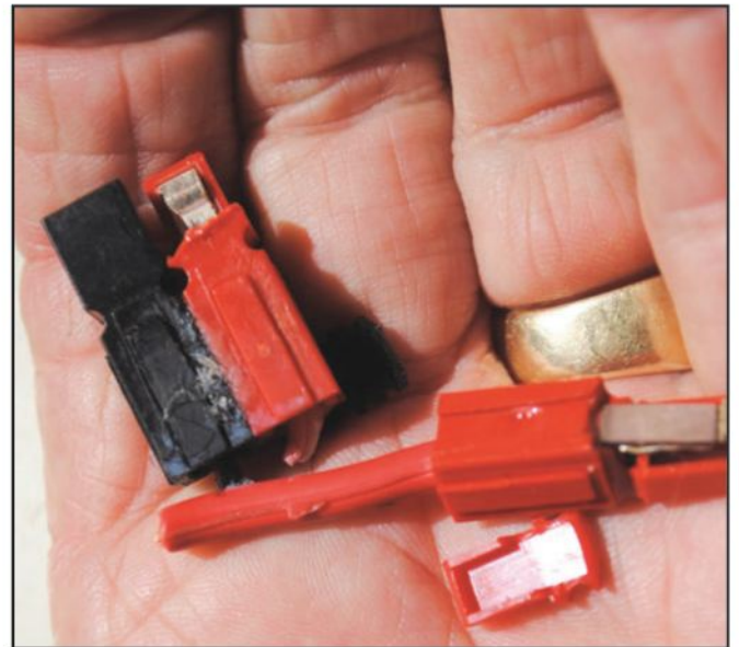
Photo F. After a year or so of constant use, PowerPoles may begin to break down. Time to replace them if they start looking like the ones in this photo.
