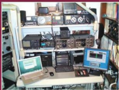
Studio A - Flex-5000A, Kenmore Twins. Palstar Tuner and Dummy Load, Yeasu FT-897D
