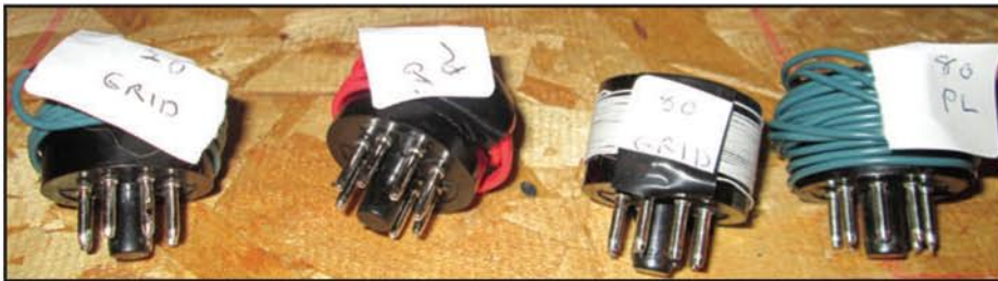
Photo G. Coils are wound on octal tube plugs to make them interchangeable for changing bands.
