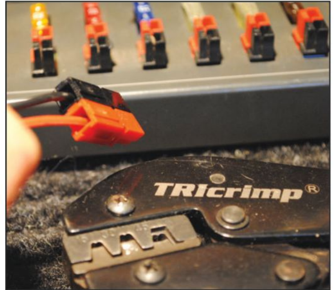
Photo E. An easy way to remember proper orientation of an Anderson PowerPole™—right, red, rear, down.
