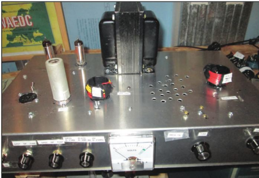
Photo B. The power transformer can come from an old tube-type TV or may be ordered online. K3MD's circuit provides two power supply options, depending on the voltage of the transformer used.
