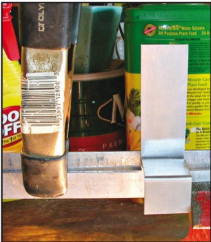
Photo H. Tightly clamping the “fold” of panels C and D between the metal bars and a vise brings the two vertical planes into one.
