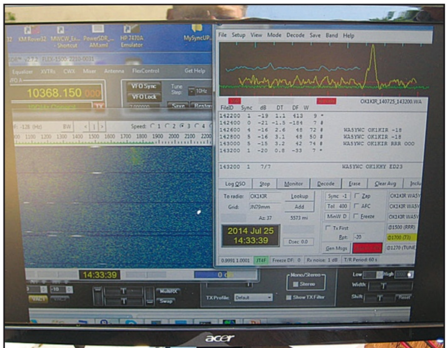
Photo E. Screen shot of OK1KIR's signal off the moon, via the JT-4 digital mode (see text for details).
