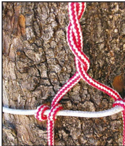
Photo E. The bulk of the remaining knot tying employs the Double Half Hitch — a nice, secure knot that can be slid for the cradle’s adjustment along the girth lines. ( WATCH AND LISTEN: How to tie it at < http://bit.ly/1vHdgb9 >. — KI6SN>)
