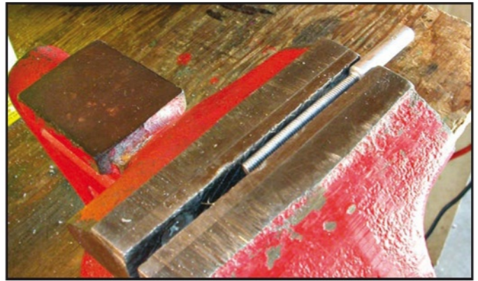
Photo O. The tuning screw is self-tapped into part of a discarded potentiometer shaft. A wood doweling will work just as well.
