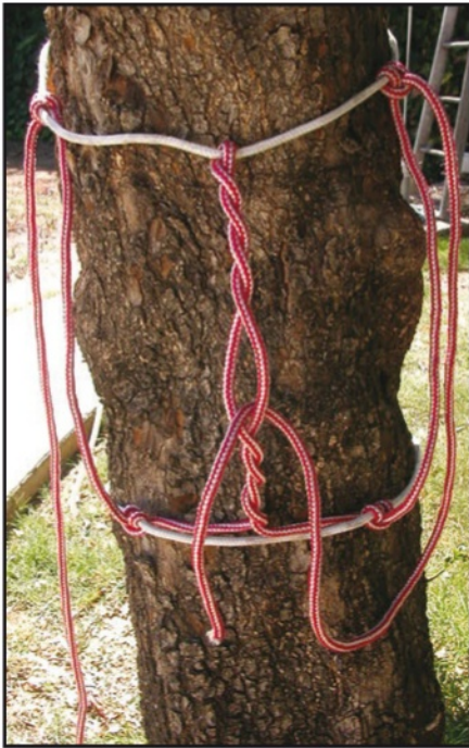
Photo F. From the Double Half Hitches on the bottom girth line, the loose ends of the red rope go vertically to the top girth line where they are secured with another set of Double Half Hitches. The loose end of one side is passed through the center loop of the twisted section. Make the same pass with the other loose end.
