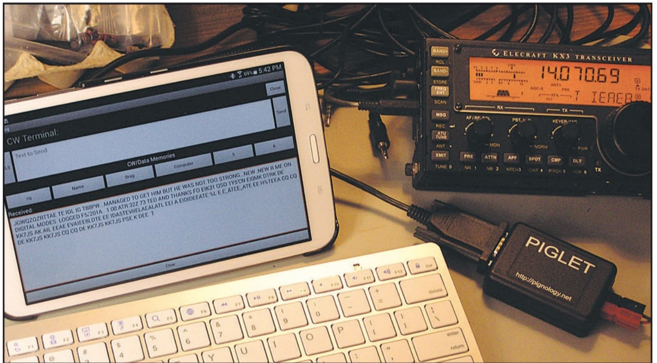
Photo C. Bluetooth keyboard connected to the Galaxy Pad, connected to the Piglet, connected to the KX3. Makes for a nice, compact digi-station.
