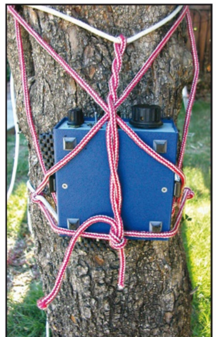
Photo I. The final step is to take the remaining red-rope ends and tie them with a simple overhand knot across the bottom part of the transceiver.
