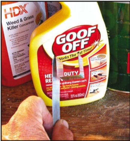
Photo G. Since the housing is made of one continuous length of aluminum, a “fold” is needed to make the center vertical plane.
