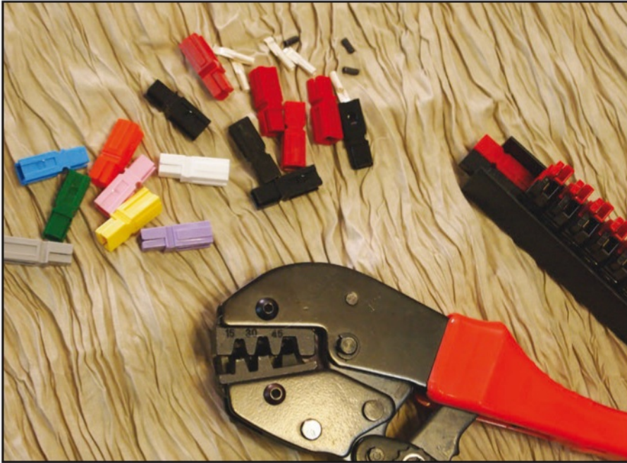
An investment in good power connections, such as the popular Anderson Power Poles, can protect your radios and accessories from being “cross polarized.” A crimping tool is the key to good connections.
