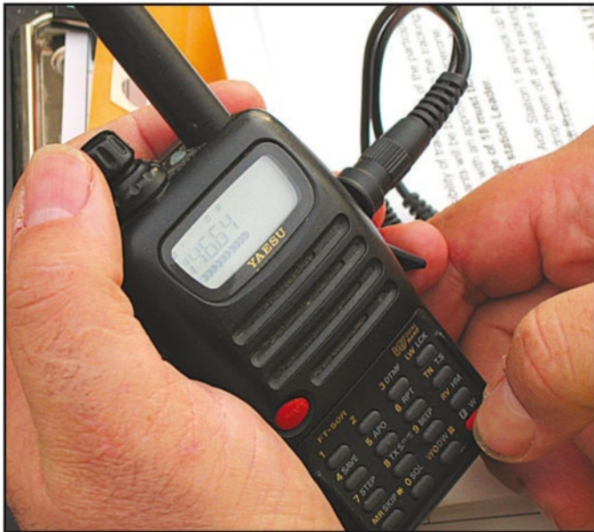
Photo D. Most new hams today begin with a does-it-all hand-held radio. Add an external antenna and 12-volt power supply to help yours put out the best signal possible.
