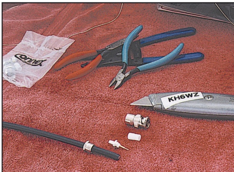
Photo 12. The BNC connector is better than a PL-259 to use at VHF and is actually easier to assemble.
