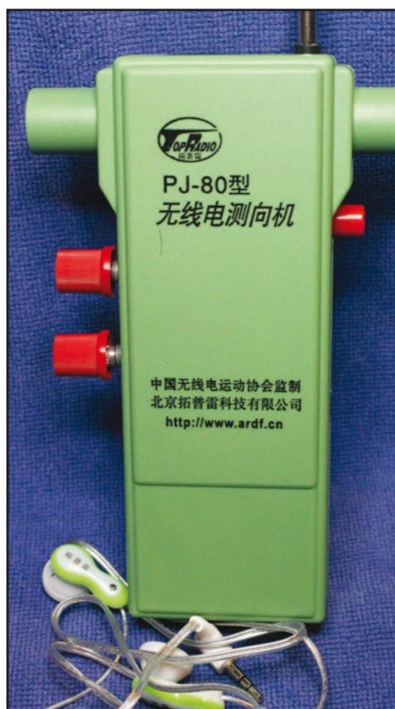
Photo B. Completed PJ80 kit ready to go foxhunting on 80 meters.
