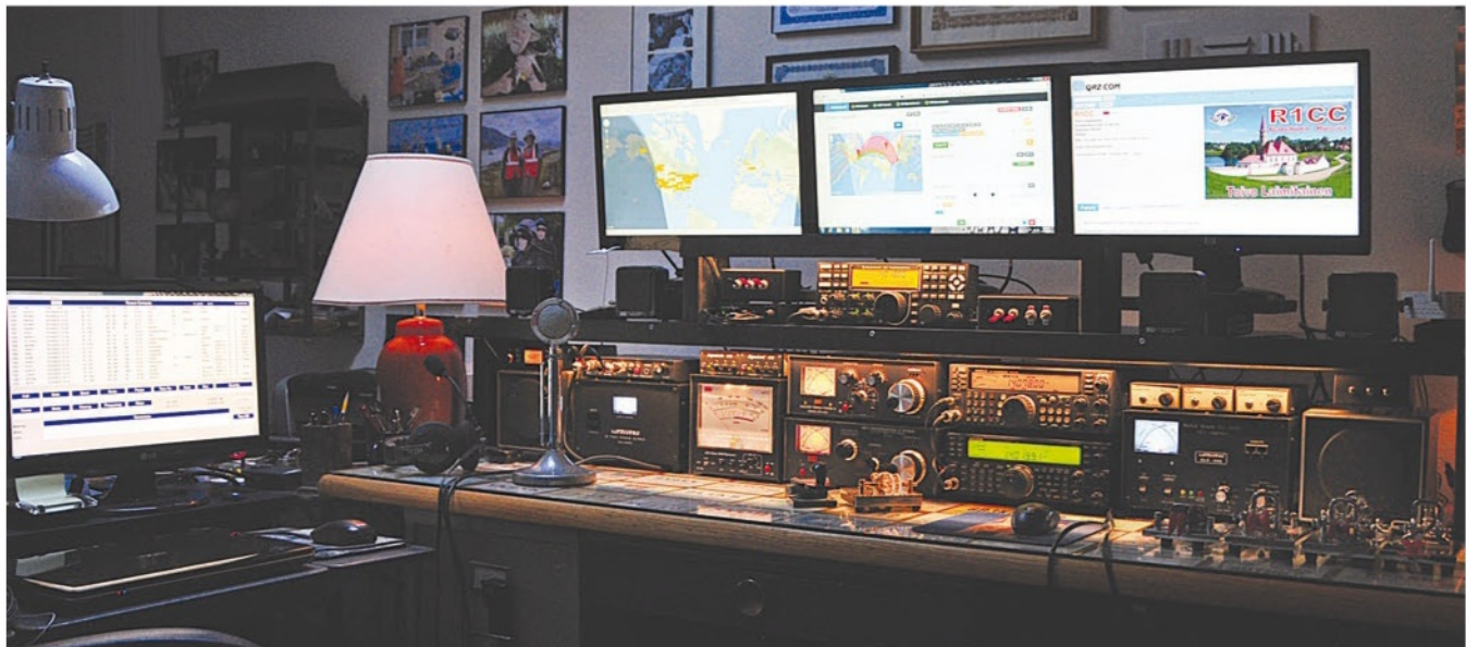
Photo B. The author's home station. The Elecraft K3 underneath the center monitor is a control head only, connected via the Internet to a complete K3 at a RemoteHamRadio station location. (W4GAL photo)
