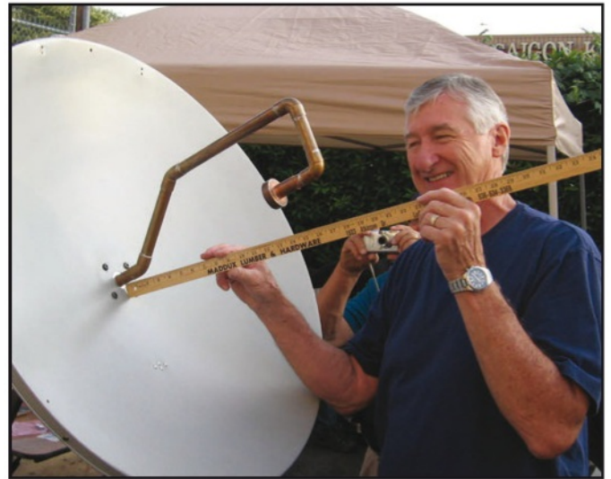
Photo C: Al's equipment was connected to a 35-inch dish and mount built by Robert Gormley, WA5YWC. Here, 'YWC checks the measurements of the shepherd's hook pipe supporting the VE4MA feed. →
