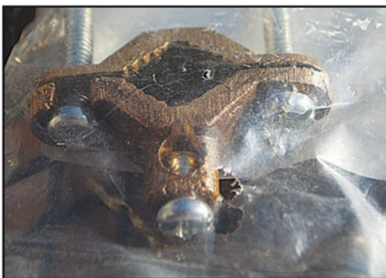
Photo A. This ground rod clamp is not rated for direct burial and can oxidize. (All photos courtesy of Ron Ochu, KO0Z)
