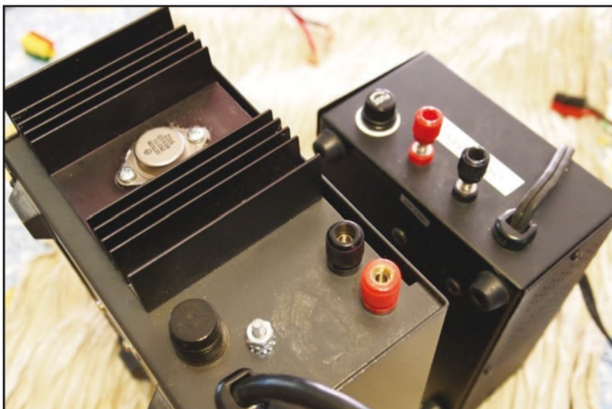
In this picture, it is easy to see how things can get confused when it comes to powering your gear. The larger power supply has its B+ terminal (red) on the right and the negative on the left. The smaller supply has its B+ on the left and negative on the right. When fiddling around on the backside of a power unit, it's best not to assume anything about which binding post is which.
