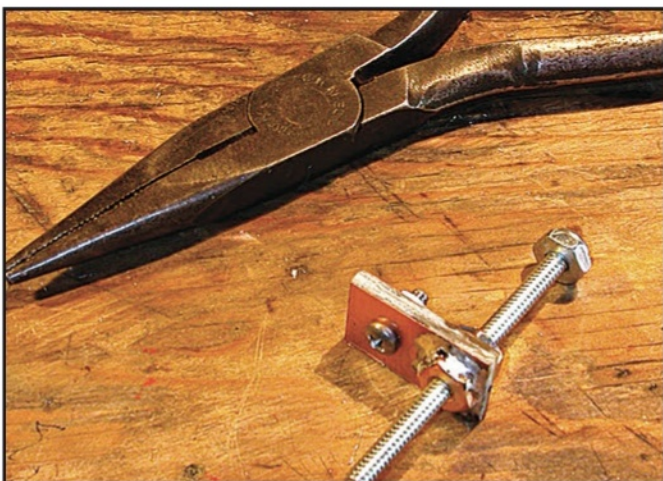
Photo N. To assure mechanical stability, small pieces of PC board and brass nuts are aligned with the tuning staff — ultimately holding it securely in place.
