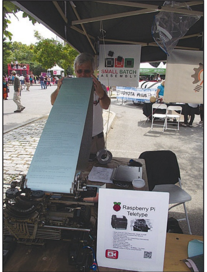
Photo L. That's Bob, NØHFV, rolling up the printout from his Raspberry Pi teletype, combining old and new by using a Raspberry Pi microcomputer to control an old Model 15 Teletype machine.
