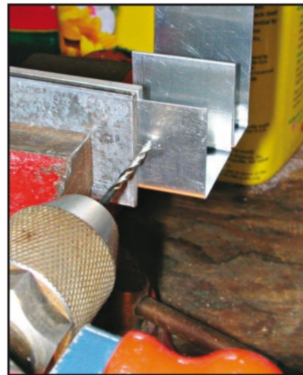
Photo J. Next in the process is drilling holes to mount the coil. Start on the back, panel A. You might want to use a hand drill for the smaller holes in place of a power drill.
