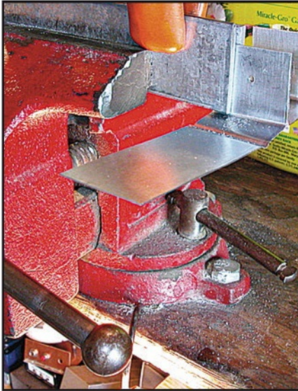
Photo L. To drill the hole through panels C and D it is necessary to "unbend" panel A.
