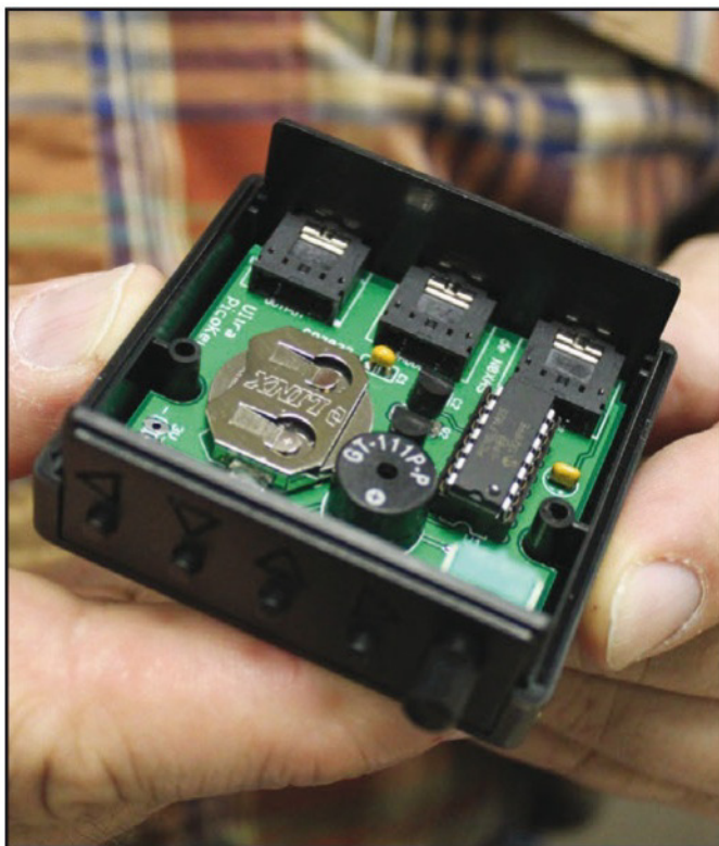
Photo E. A closeup of the Ultra PicoKeyer kit in the case.
