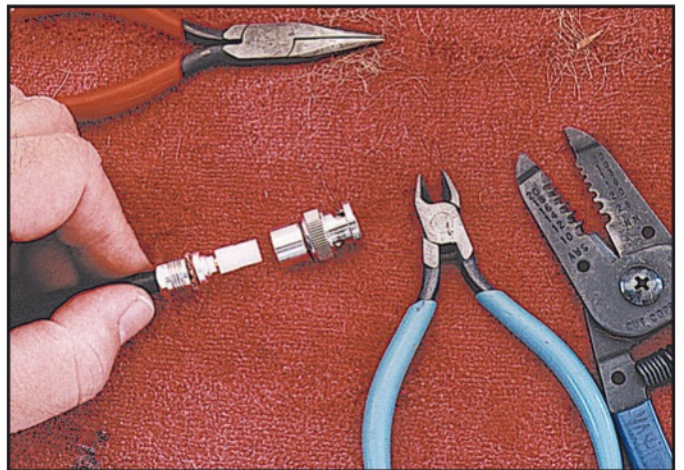
Photo 15. After soldering and checking for shorts, slide the shell onto the assembly. Hold the cable and connector body still with a wrench while you turn the locknut. Try not to twist the connector body, since that may twist the wires inside the connector.
