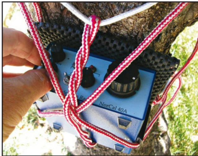
Photo H. Before sliding the Double Half-Hitch knots to tighten the lashing along the girth lines, position your radio in the cradle, with protective material between its surface and the bark, to allow free access to the controls. It may look cumbersome, but it's not.
