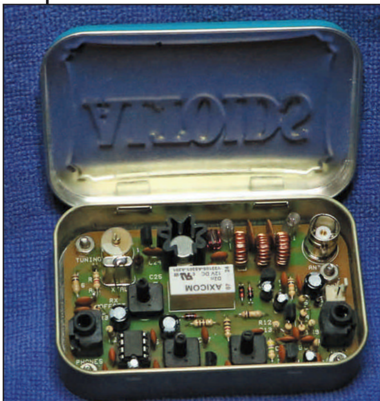
Photo A. The Kanga FOXX-3 transceiver kit mounted in an Altoids® tin.
