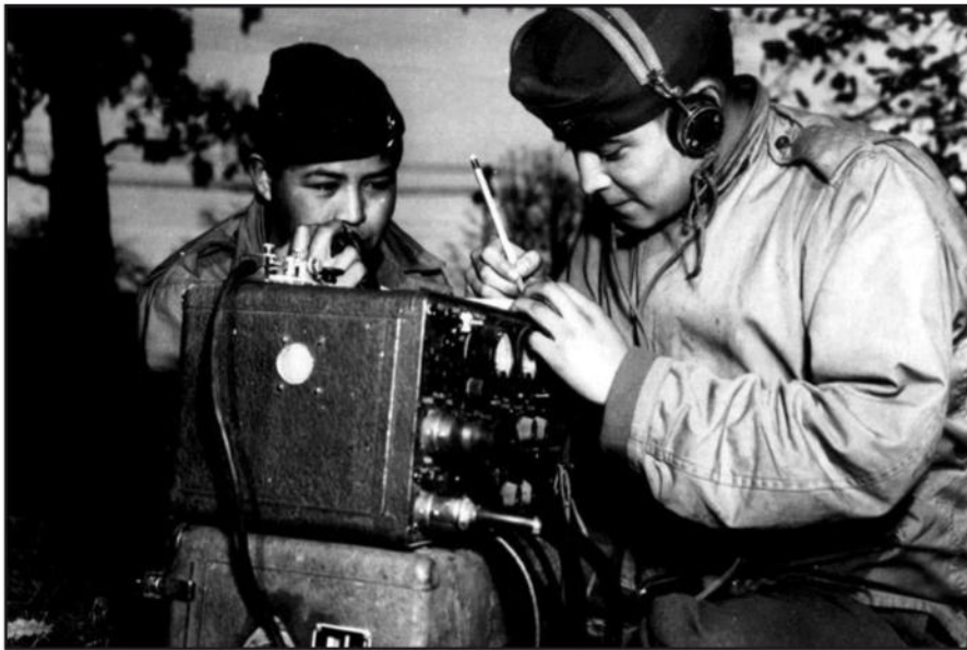
Photo D. In addition to a rifle, ammo, water, and rations, Code Talkers packed the TBY-2, vibrator power supply, batteries, generator, and accessories. (Code Talker photos courtesy of <a href="http://www.navy-radio.com">www.navy-radio.com</a> and <a href="http://vrhistory.com">vrhistory.com</a>; used by permission.)
