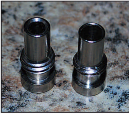
Photo C. PL-259 reducers are used to connect smaller diameter coax to a PL-259. The UG-175 (left) is used for RG-58U and a UG-176 (on the right) is used for the slightly larger diameter RG-8X coax. One can never have too many of these on hand.
