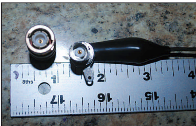
Photo D. BNC connectors: On the left is a male BNC and a chassis mount, female BNC is on the right.
