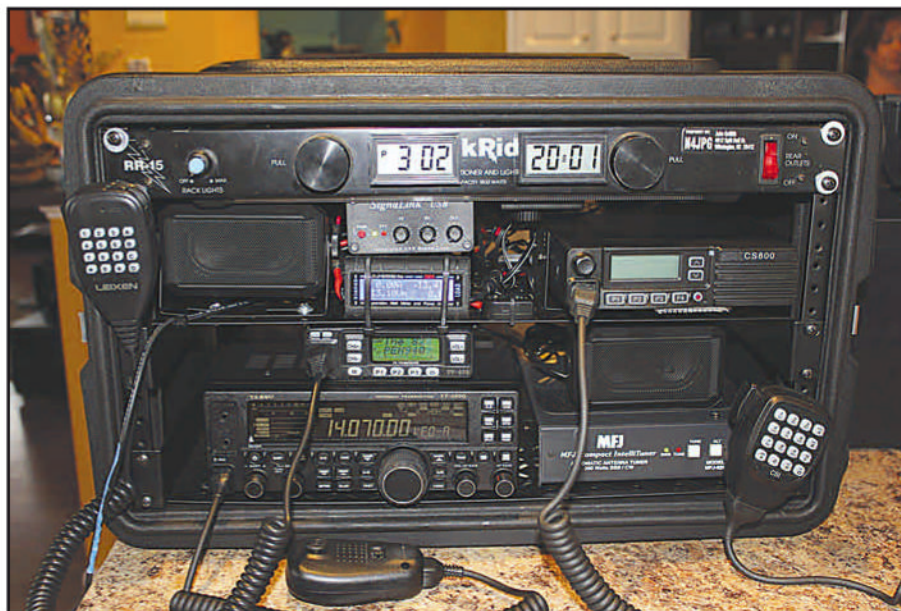
Rear and front views of N4JPG's work reveals a Go Box with HF, digital voice, and conventional analog coverage, plus support for keyboard digital modes. Of particular interest are the shelves (see text and next photo for details).
