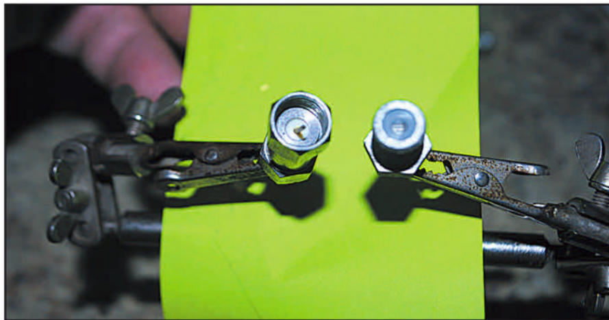
Photo G. F connectors are mostly used in video work, but they are occasionally found in ham radio applications. On the left is a male F connector with a slightly bent center pin and on the right is a female F.
