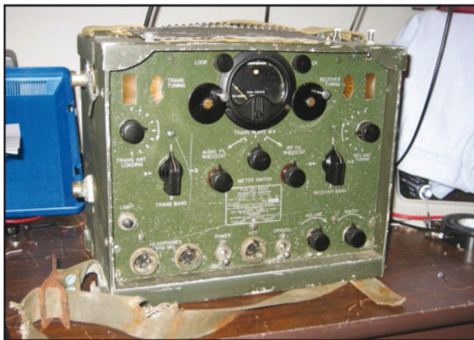
Photo E. The TBY-2 and later TBY-8 had a tuning chart and key mounted to the top, although most code talking was phone.
