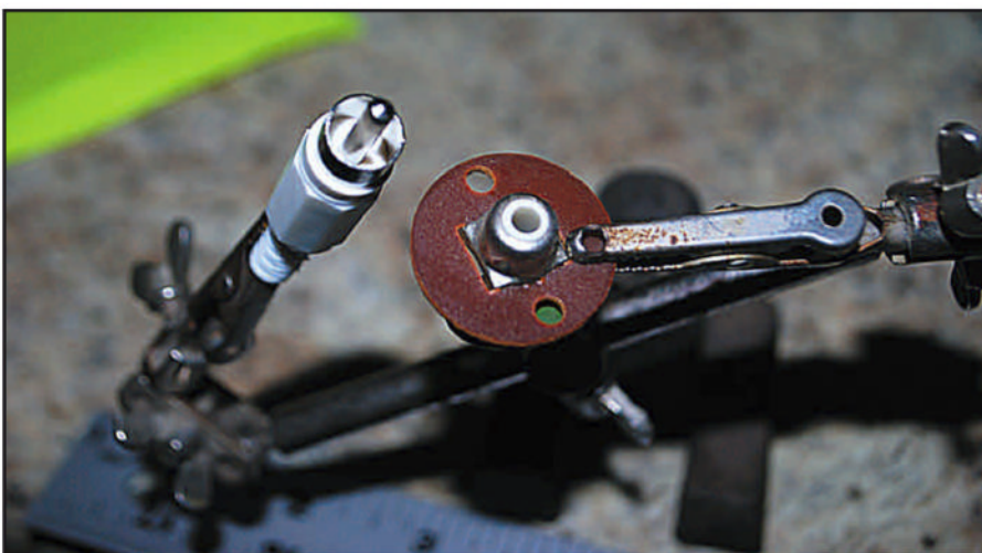
Photo H. RCA connectors can be found on older ham radio equipment and some current QRP kits. Today they are mostly used for audio-visual applications. On the left is a male RCA connector and on the right is a female.
