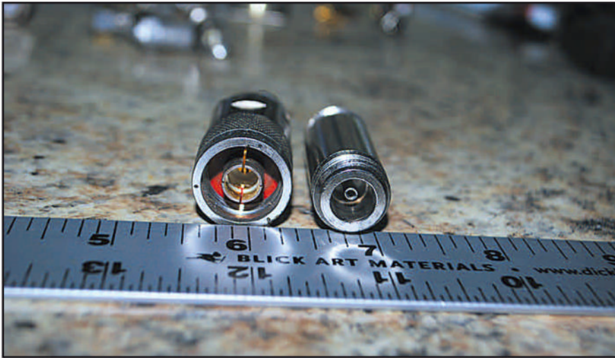
Photo F. For serious weak-signal UHF and above work, N connectors are used. On the left is a male N connector and on the right is a female, barrel N connector.
