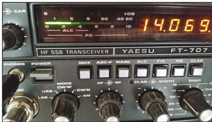
Photo C. S-meters are usually part of the AGC circuit and not all that accurate.
