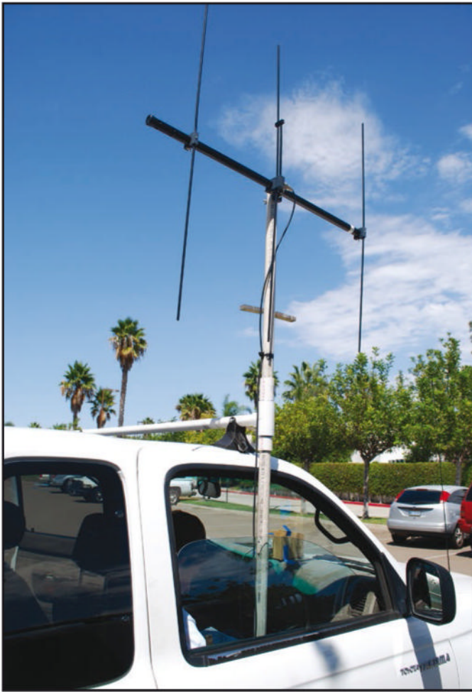
It's not difficult to mount a rotatable two-meter beam onto a vehicle to get bearings in motion. Both Yagis and cubical quads are popular for mobile T-hunting in southern California.
