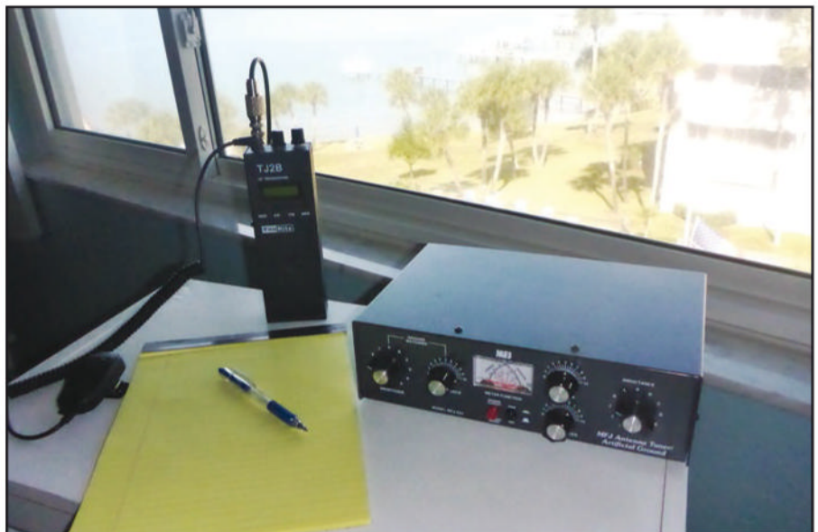
Photo C. Close-up of the TJ2B and MFJ-934 antenna tuner with artificial ground circuit.
