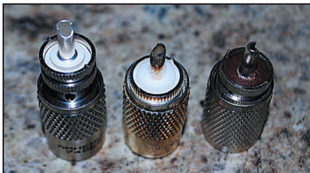
Photo B. A true Amphenol Teflon® PL-259 is on the left and an imitation Teflon connector is in the middle. The PL-259 on the right uses Bakelite as an insulator; these are great connectors, but increasingly difficult to find at hamfests.
