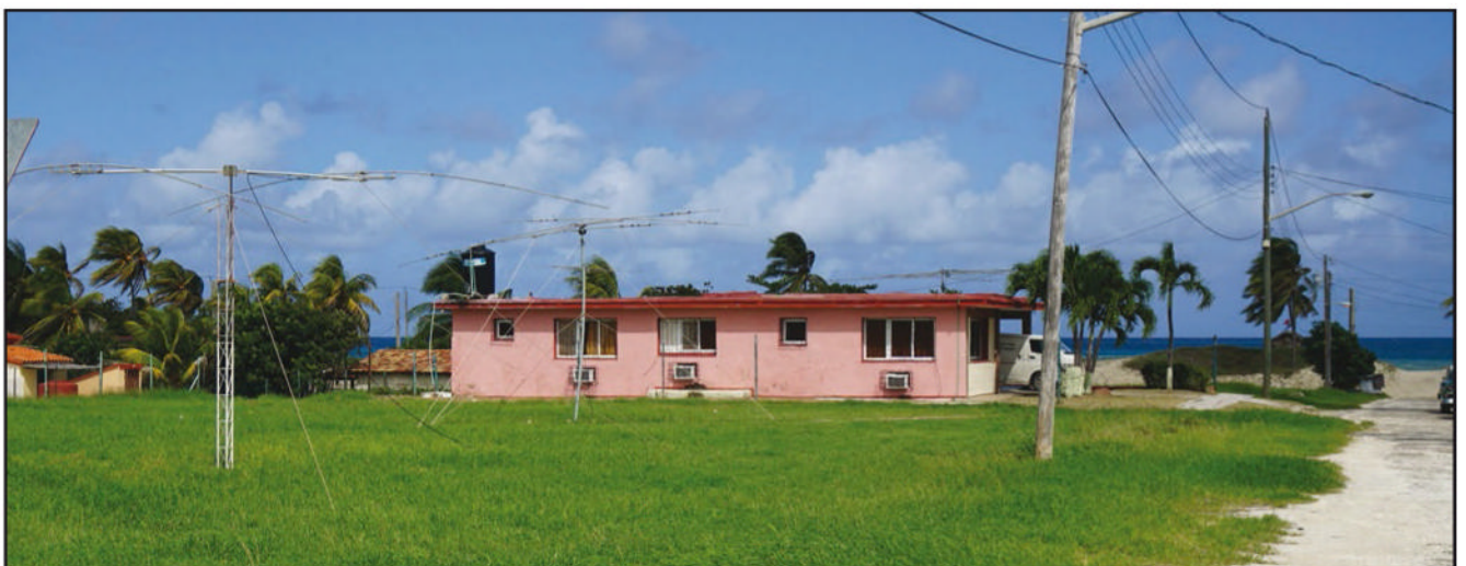
Photo C. The station was set up in a rented house with a large open area in front for antennas. A shortage of tower sections limited antenna height; beams were turned by hand, using ropes.
