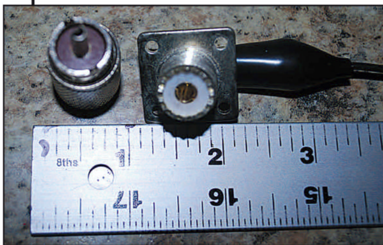
Photo A. UHF connectors, the PL-259 (male) is on the left and the SO-239 (female) is on the right. These connectors are found in most HF applications. Typically found on RG-8U coax. (All photos by KOØZ)
