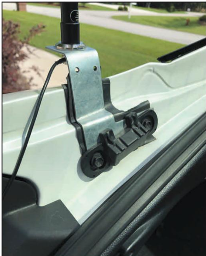
Note the rubber paint protection behind the sturdy, fabric-covered antenna mount.
