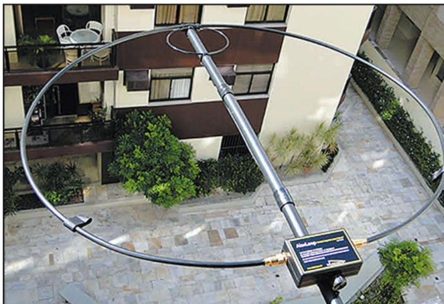
Photo C. Extremely portable and highly efficient, the AlexLoop Walkham is a magnetic loop antenna that reflects an investment of over 12 years of R&D. I highly recommend it for quick setup HF operations.
