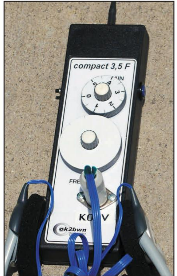
Photo A. The Compact 3.5F set sold by Jiri Marecek, OK2BWN, has a direct-conversion receiver and a short ferrite rod antenna inside the case. (Photos by the author, except as noted)
