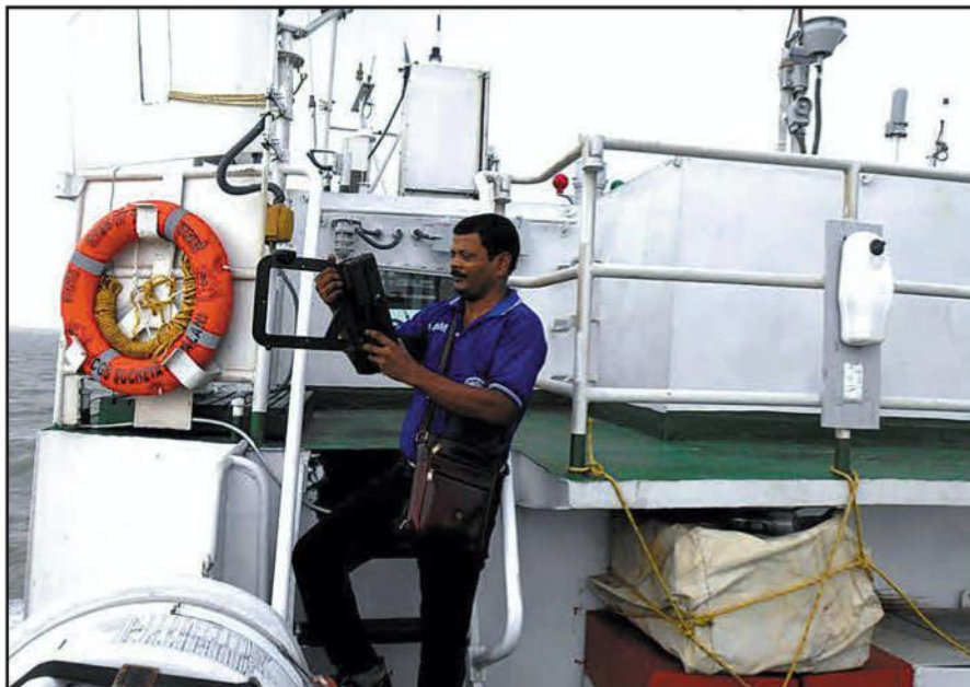
Photo D. VU2JFA checking the signals of All India Radio, Kolkata with Potomac Instruments 4100 Medium Wave Field Strength Meter.
