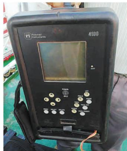
Photo E. Close-up of the Potomac PI 4100 meter. This portable laboratory-grade instrument provides direct measurement of electromagnetic field strength in the MF and low HF regions of the radio spectrum.
