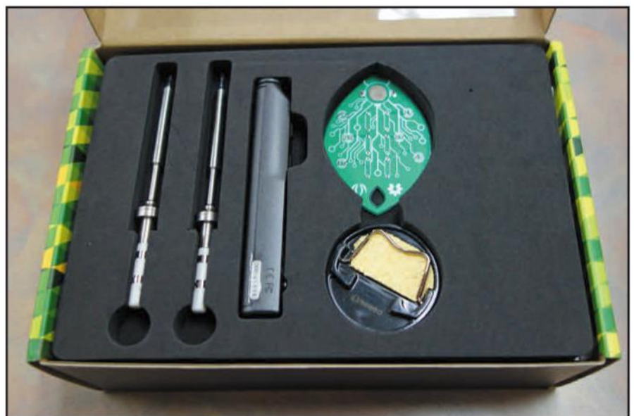
The Seeed Studio Mini Soldering Station kit in the box. The practice board is visible as are the handle and the two tips/heaters. The power supply and accessories are stored below.
