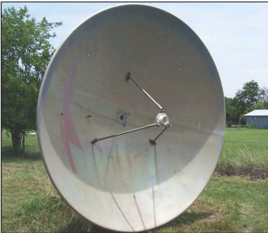
Photo B. Ten-foot dish with prime focus feed.
