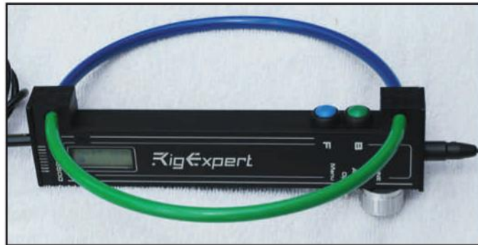
Photo G. Close-up of the FoxRex 3500 showing the dual sense pushbuttons and LCD readout.
