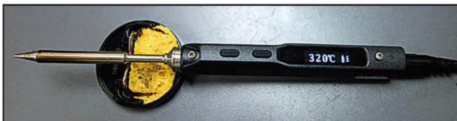
The soldering iron's digital display not only displays temperature, but also shows graphics when it goes into sleep mode, etc.
