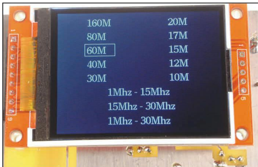
Photo D. The setup menu lets someone select any of the HF ham bands or three larger frequency ranges between 1 and 30 MHz.
