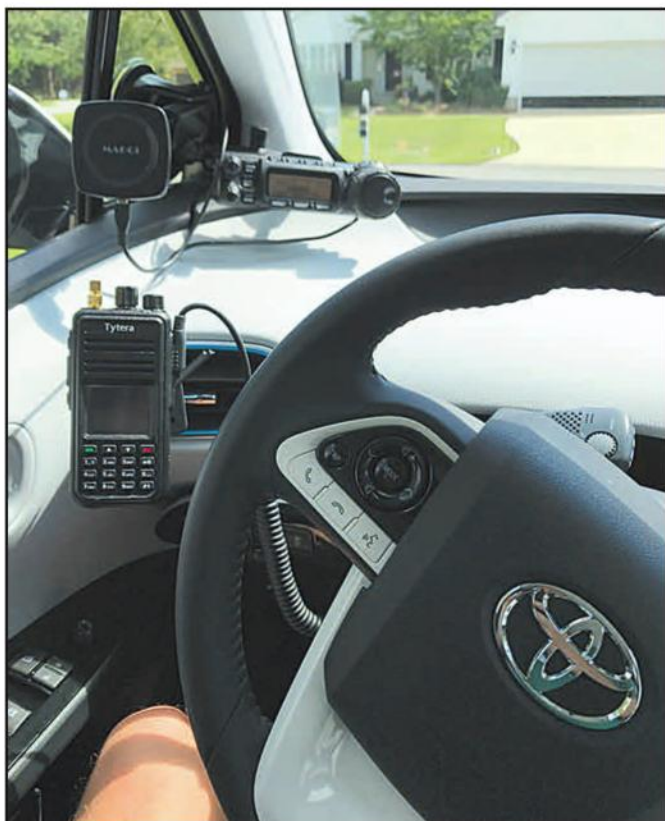
While the Prius cockpit is compact, the windshield setback offers mounting opportunities that are functional and don't interfere with driver's sight lines.
