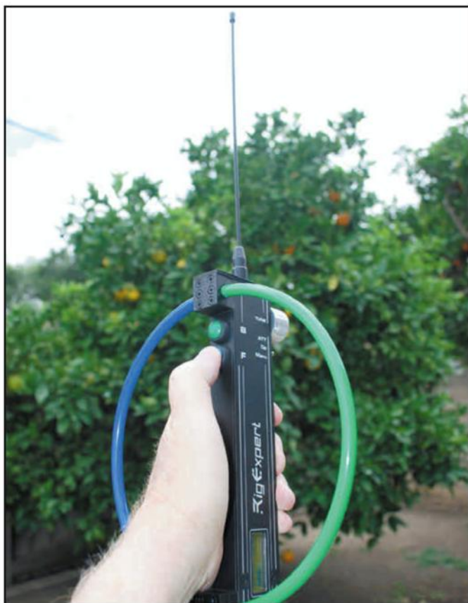
Photo E. Unlike most 80-meter ARDF sets, the FoxRex 3500 has two cardioid-pattern sense modes, each with its own pushbutton.
