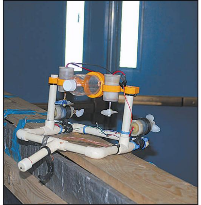
Photo F. This past school year's SeaPerch submersible ROV (Remotely Operated Vehicle).
