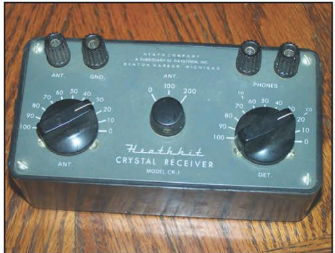
The Heathkit CR-1 crystal radio. (Photo courtesy Rob Mavis, AE6GE, of the Old Tube Radio Network <www.oldtuberadio.com>)
