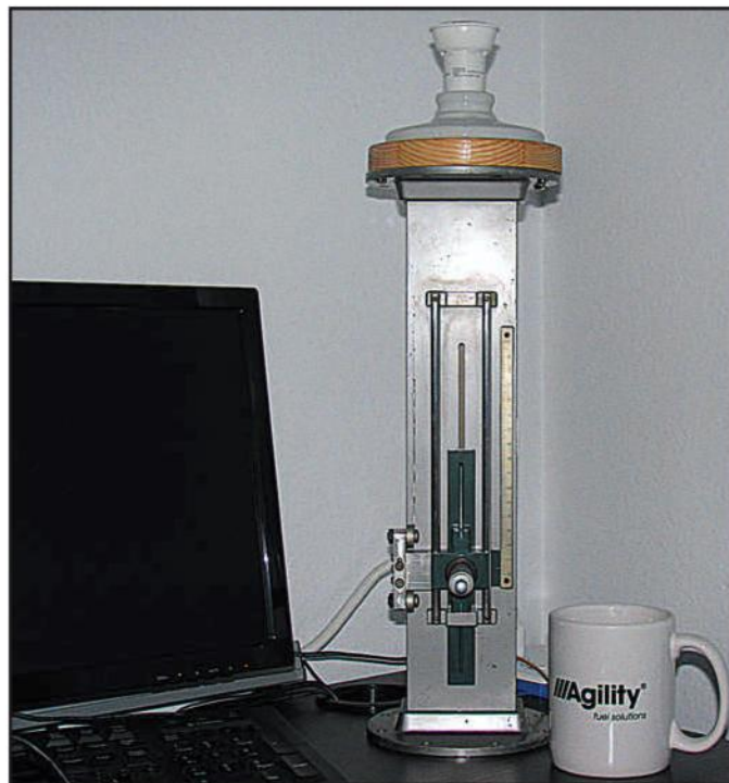
Photo G. Instead of buying a boring desk lamp, I decided to make one out of a waveguide slotted line. It is energy efficient, since an LED bulb is used.
