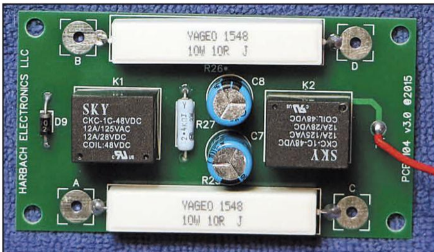
The Harbach Soft-Start kit assembled. The low parts count makes assembly of this kit easy.
