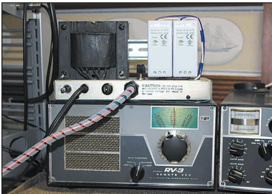
Photo B. The AC3 power supply and RV3 remote VFO were also rebuilt as part of the author's restoration project.
