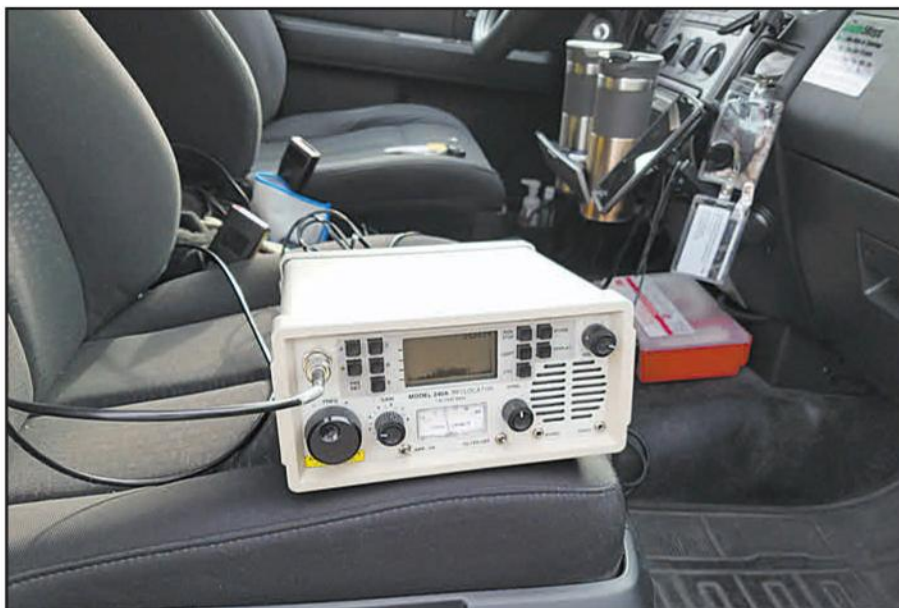
Photo E. Ameren's commercial model 240 A RFI locator operates from 1.8 to 1000 MHz. Note the RFI signature on the display.
