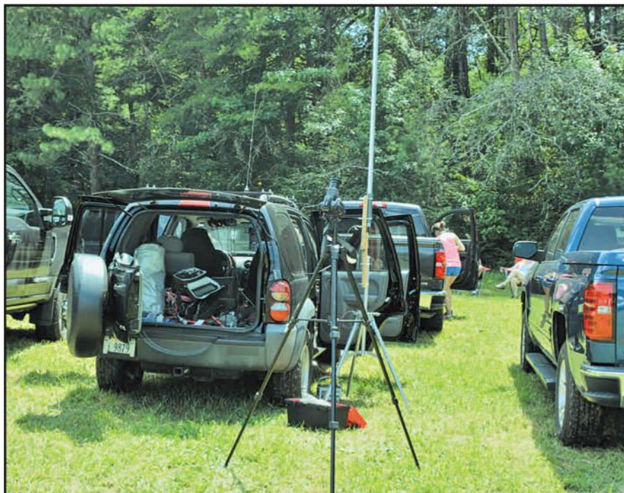
Photo I. W1IE's homebrew 20-meter vertical antenna he used during the solar eclipse party.
