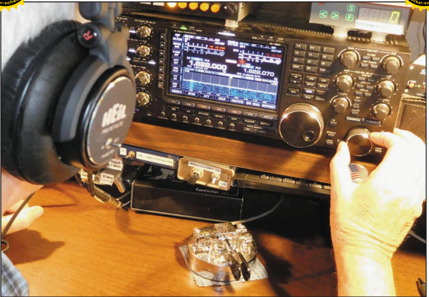
Photo A. Using a rig's dual VFO to tune in one signal at slightly different frequencies can enhance your ability to copy a weak CW signal in noise.
