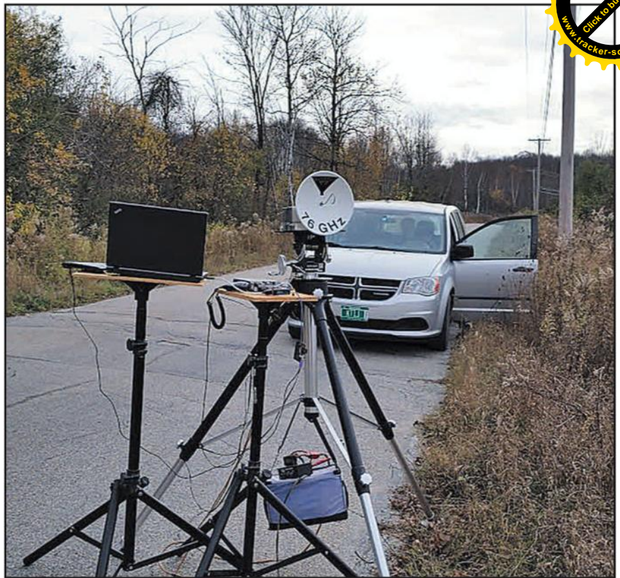
During an attempt to record a 100-kilometer QSO between the U.S. and Canada, N1JEZ set up his 78-GHz station on the side of the road.
