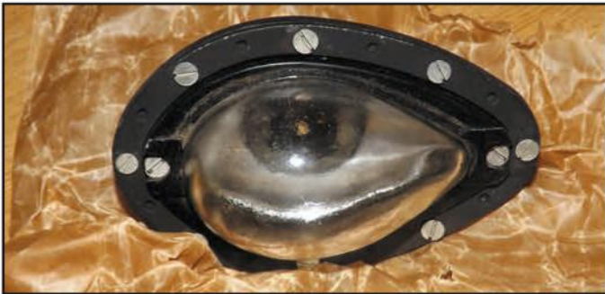
Photo H. Original identification lamp (one of two mounted on the Spitfire) operated by the key inside the cockpit.
