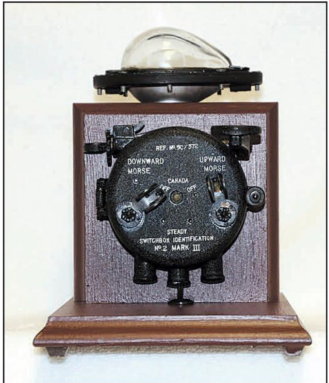
Photo I. Finished key and lamp assembly mounted; it is lit using a 12-volt DC supply.
