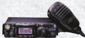
FT-891 100 watt HF + 6 meter all mode transceiver
