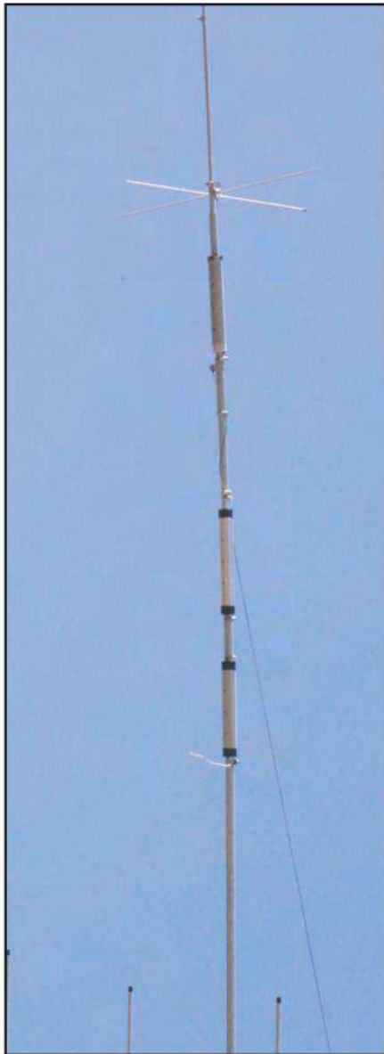
Photo E. Traps are common elements of many multiband antennas. Long-term exposure to weather extremes can cause them to become intermittent, but the fix is often quite simple.
