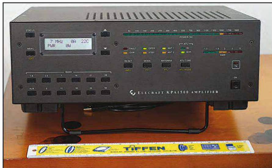
Photo A. The Elecraft KPA1500 amplifier comes in two packages, the RF deck (seen here) and a separate 220-volt power supply. (Photos by the author)
