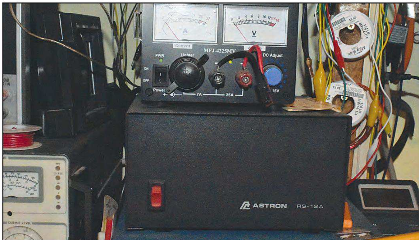
Photo B. The MFJ-4225MV switching power supply (top) is my primary workbench DC supply. It offers 22 continuous amps and variable voltage settings. Below it is an Astron RS-12 A analog power supply (without meters).
