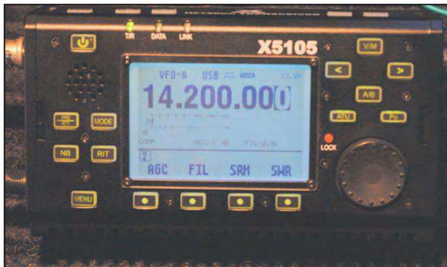
Photo A. The Xiegu X5105 portable HF/6-meter transceiver from China is marketed exclusively in the United States by MFJ Enterprises.
