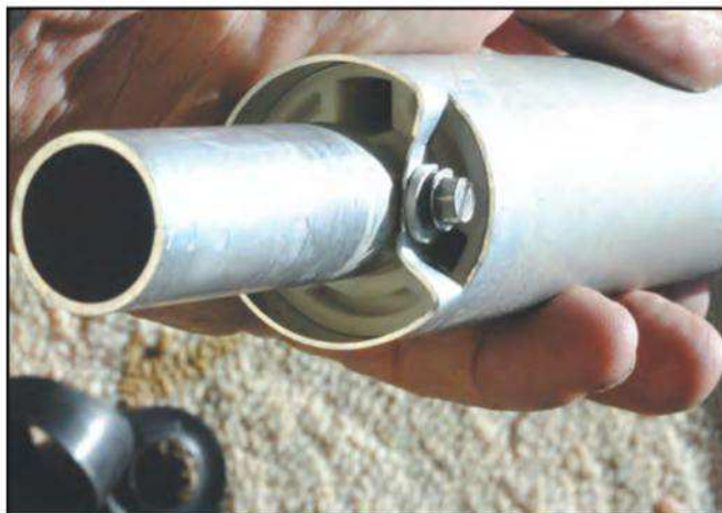
Photo F. A single sheet-metal screw — generally hidden under a rubber boot — connects the trap to the antenna element. Tightening this screw and restoring water / critter protection to the junction can often resolve a “bad trap” issue.
