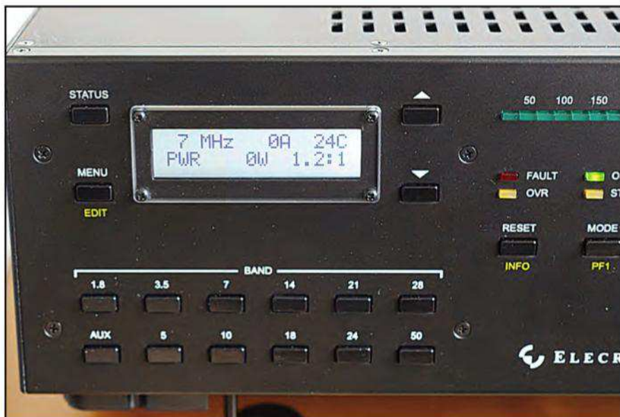
Photo D. Pushbuttons are used to select the operating band. If used with the K3 transceiver and optional KPAK3AUX connecting cable, switching the band on either unit changes the settings on both.
