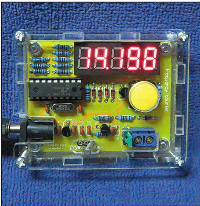
Completed crystal tester measuring a 20-meter crystal.
