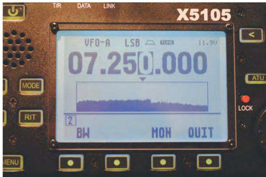
Photo D. The blue LCD display also features a graph function that can show you band activity or the SWR plot of your antenna.
