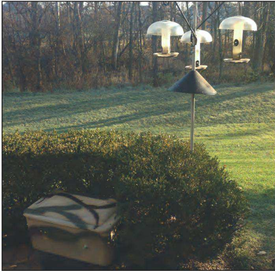
Photo B. This is W8ARE's fiberglass radiator support, showing the bird feeder and squirrel skirt in addition to the camouflaged ATU cabinet. (Courtesy of W8ARE)
