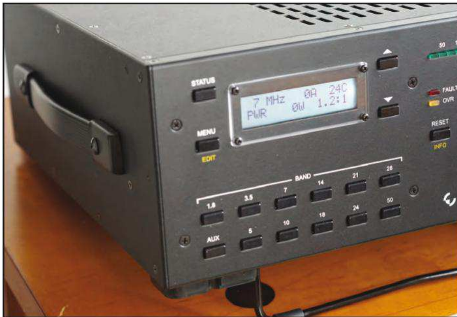
Photo B. Both the RF deck and the power supply feature carrying handles, making the units easy to lift and transport.
