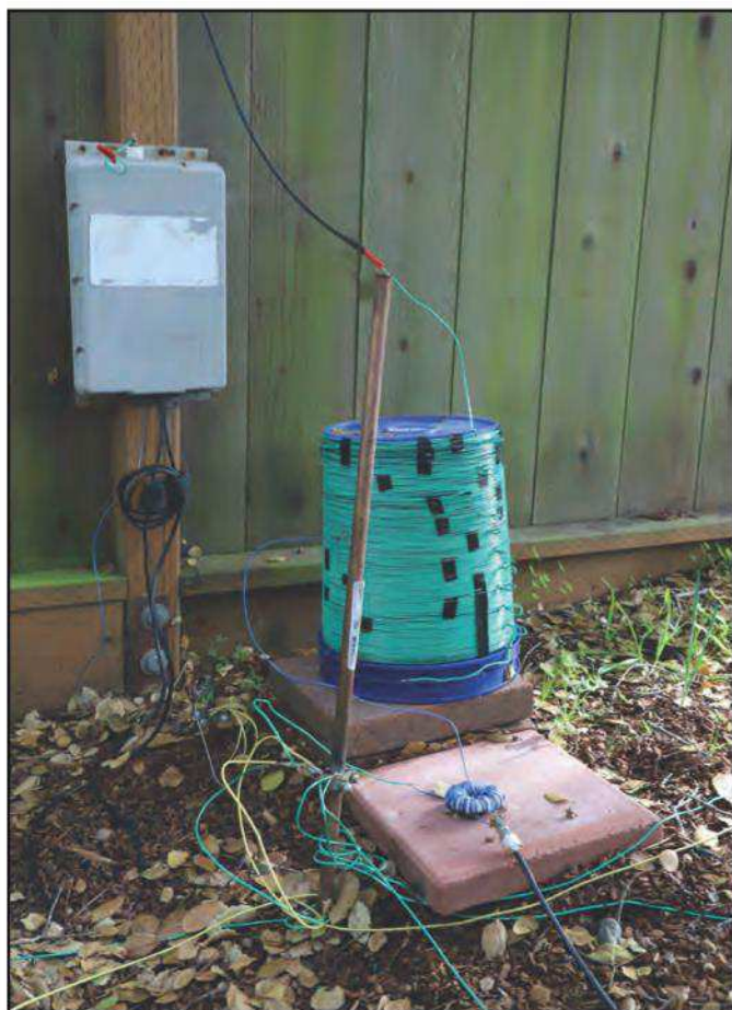
Photo C. The feed point of N1VF's 'tree' inverted-L, showing the ICOM autotuner for HF, the bucket coil for 630 meters, ground rod with radials and matching transformer for the 630-meter coil. Ben uses a Powerpole connector for the radiator to facilitate rapid spectrum changes between HF and 630 meters. (Courtesy of N1VF)
