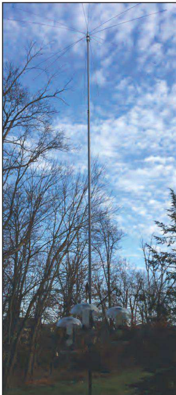
Photo A. The 19-foot, 630-meter antenna at W8ARE, complete with bird feeder and top loading spokes that resemble bird perches. (Courtesy of W8ARE)
