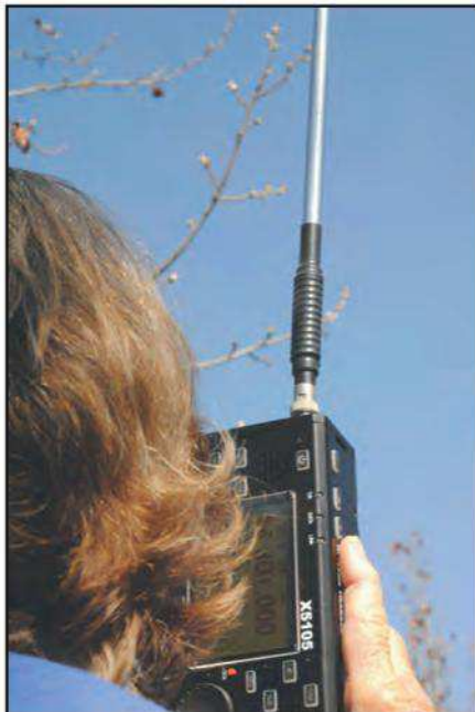
Photo B. The X5105 includes a built-in microphone and speaker for hand-held use, along with a single-band whip antenna, for self-contained portable operation. A plug-in mic is also supplied with the rig.
