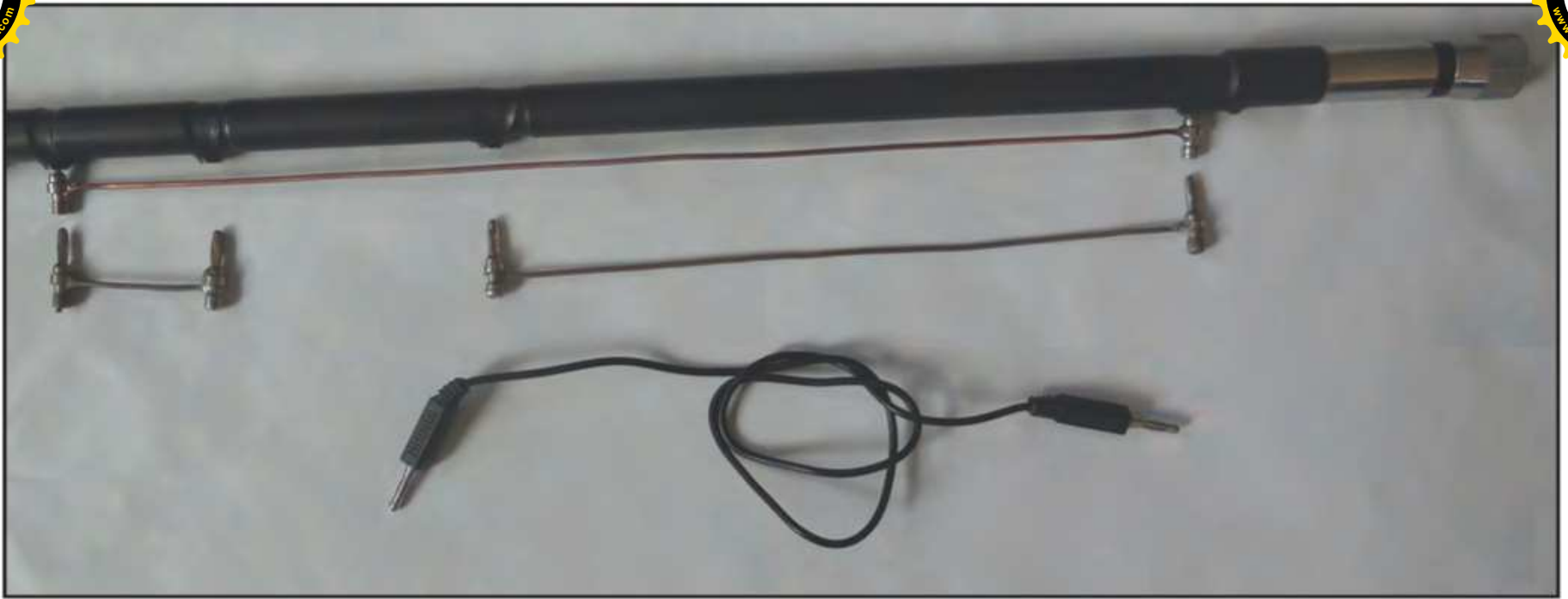
Photo B. Comparison of the antenna's supplied jumper cable (bottom in photo) with band-specific, solid-copper jumpers fabricated by the author.
