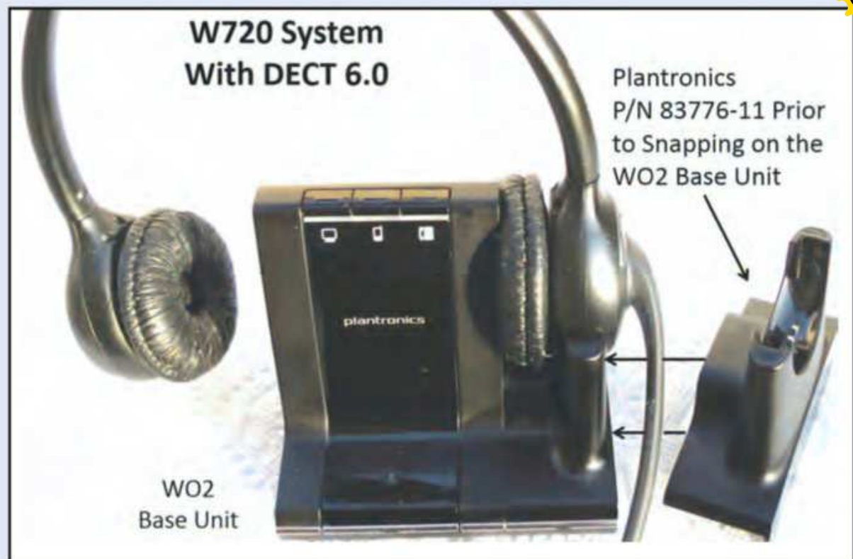
Photo B. The Plantronics WO2 wireless base unit showing the proper charging cup mounted to the right side.
