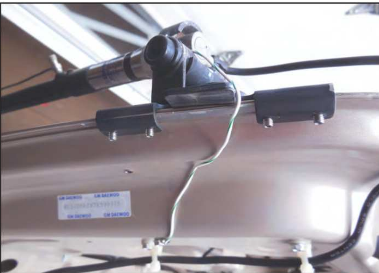
Photo E. The author also added a ground wire from the antenna base to the trunk lid to assure a good RF ground connection.
