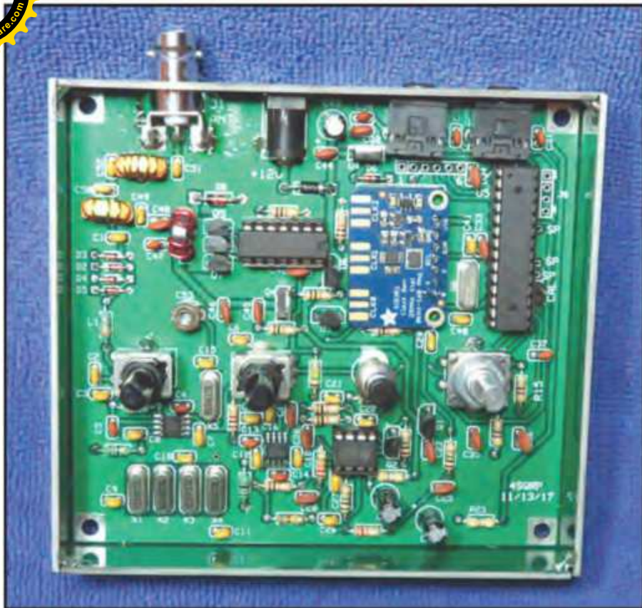
Photo D. The Hilltopper 20 assembled and ready for calibration. Note the DDS (direct digital synthesis) board at the upper right.
