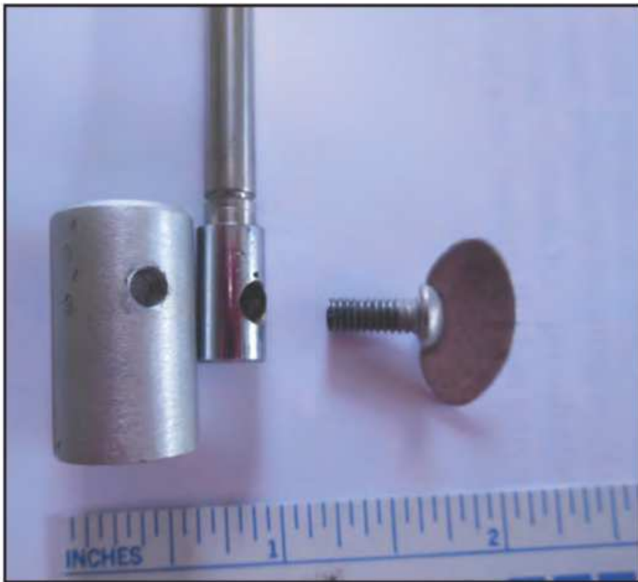
Photo C. The collar and thumbscrew with which the author replaced the Allen screw for tightening the whip. The whip length needs to be adjusted with each band change and the tiny Allen setscrew was too easy to drop and lose.
