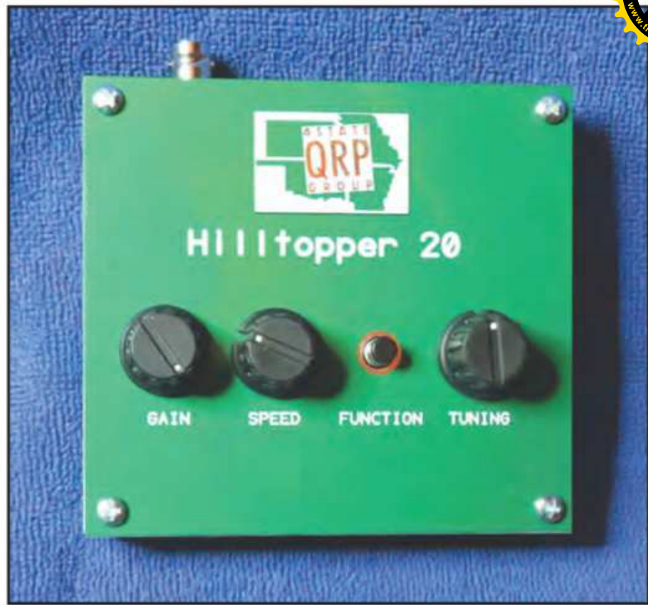
Photo E. Front panel of the finished Hilltopper 20 kit. The case is made entirely of PC board material and comes already drilled and labeled.
