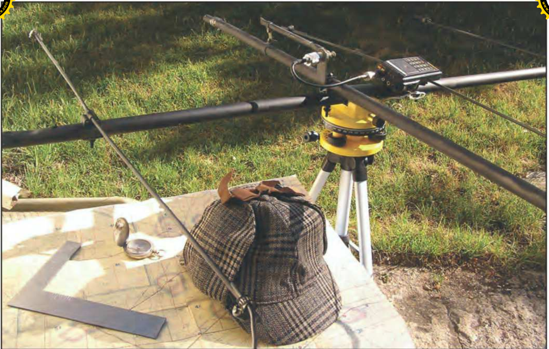
Closeup of the black Elementary Yagi on a tribrach that was used for all the direction-finding work in the 30-year T-hunt.
