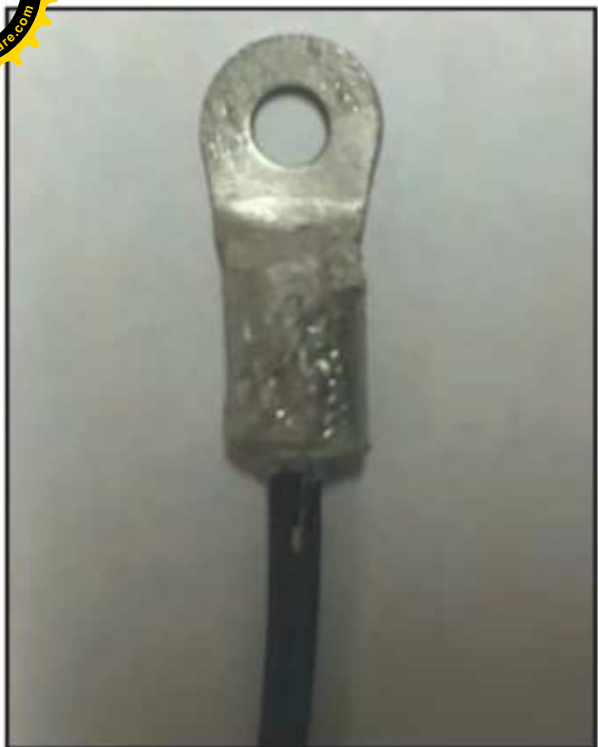
Photo D. Ring terminal with thermistor bonded inside it. The bottom of the ring is sanded and attached firmly to the transceiver (see text for details).
