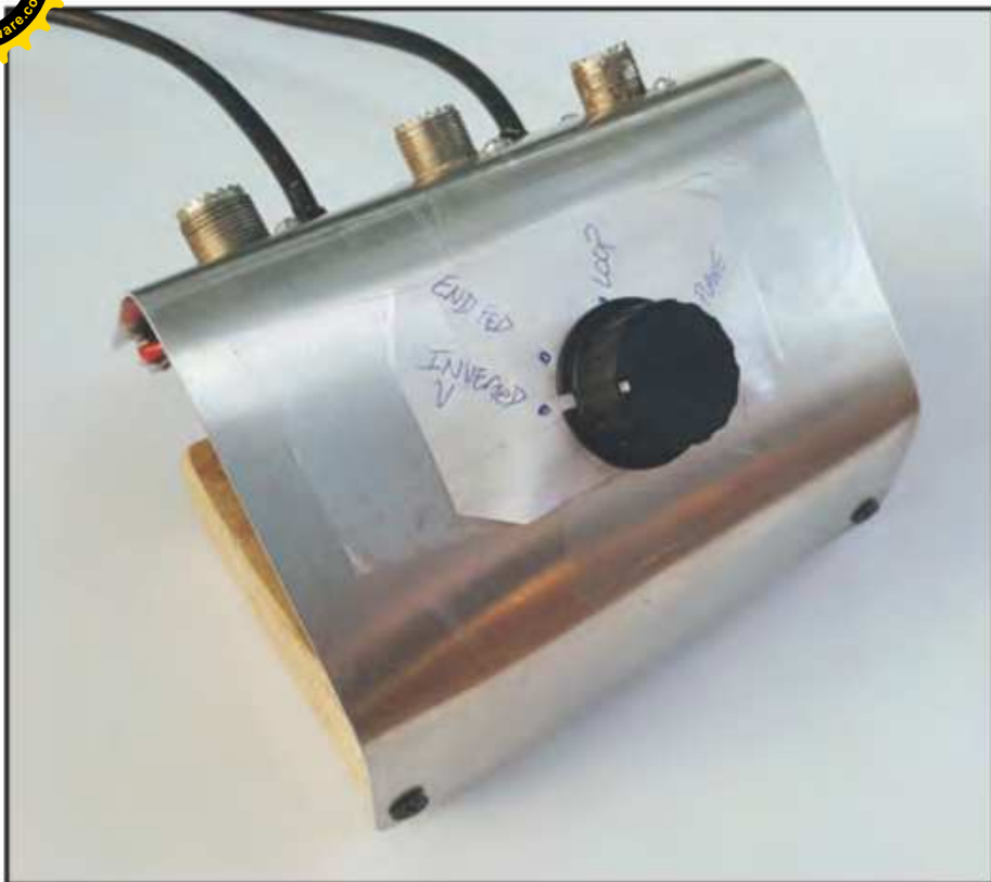
Photo B. The homebrew antenna switch I used for the showdown.
