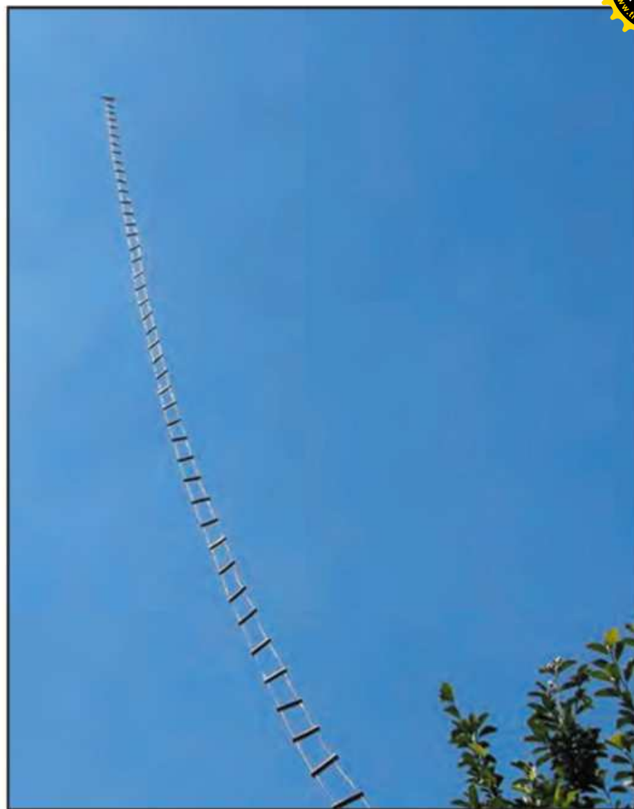
Photo B. The W8CDX (NO3M) Field Day doublet was used on HF in addition to 630 meters where it was configured as a Marconi-T vertical. This approach could be duplicated just about anywhere that has an HF dipole and feed line, whether coax or open-wire line, that can hang in free space, including Field Day sites and portable emergency activations. (Courtesy of NO3M)
