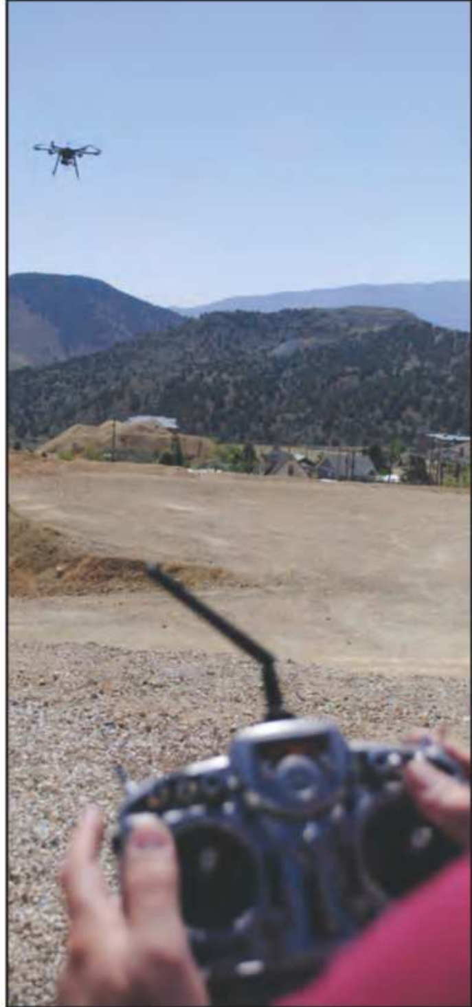
Photo G. Drones are big, but some are flying afoul of FCC frequency and power rules. Hams may operate them under Part 97 rules, but only if they operate fully within the 13- or 5-centimeter ham bands, with appropriate power levels. Drones can be great for emergency communications work.
