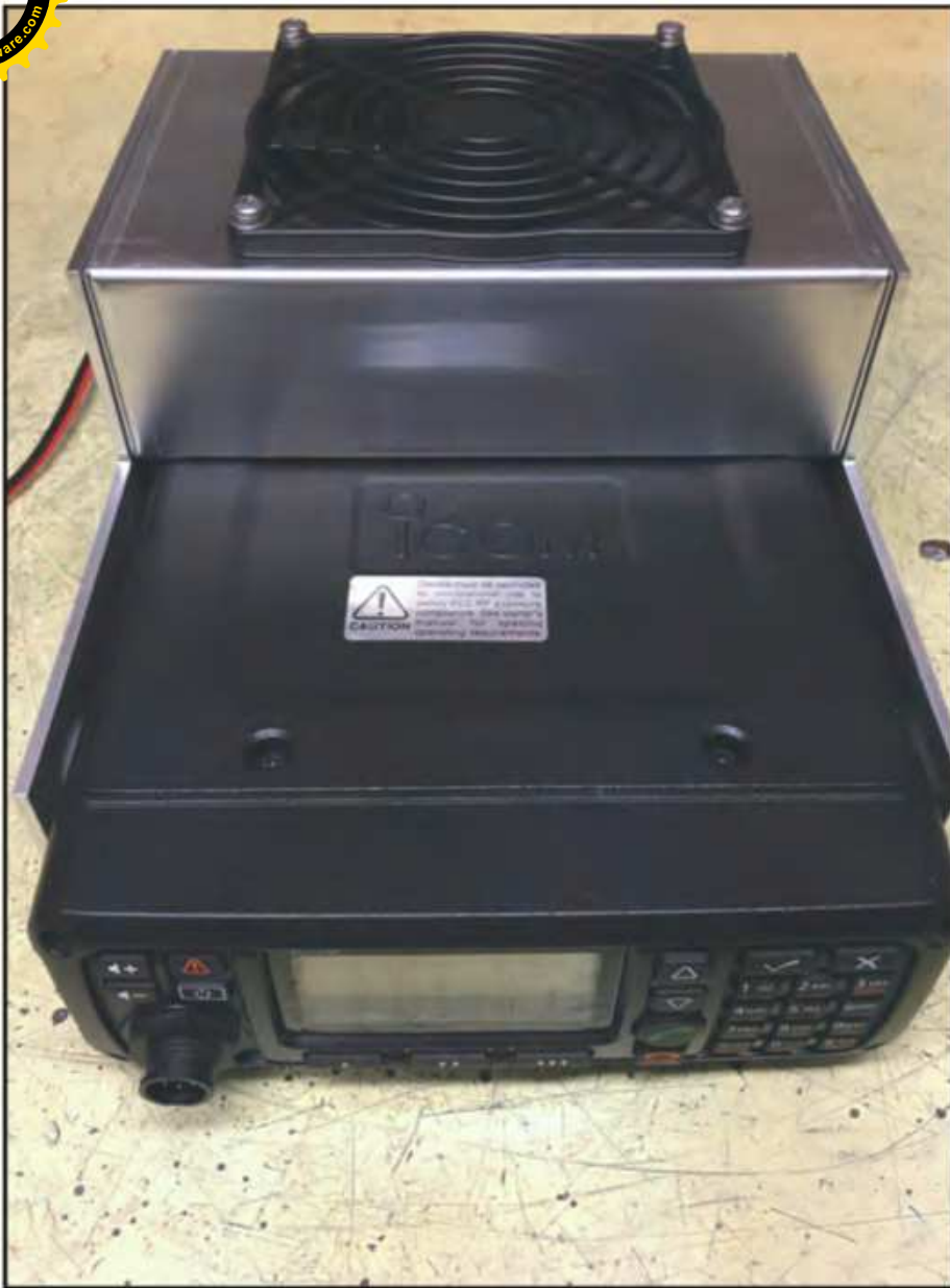
Photo B. The cooling unit is mounted on top of ICOM's F8101 land-mobile transceiver.
