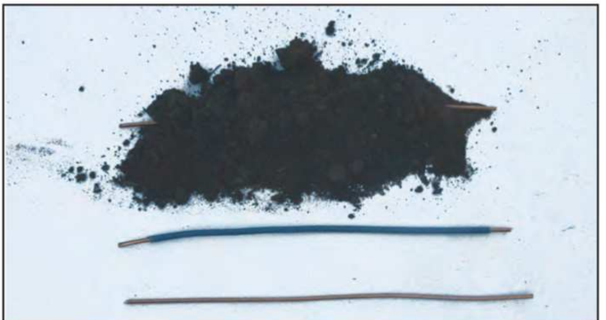
Photo B. Wire with different insulators ... air, plastic, and dirt. Do any readers have good data on ground radial currents in dirt?
