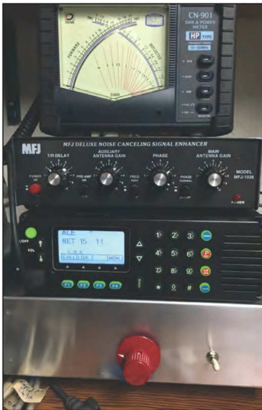
Photo A. The Micom-Z land-mobile transceiver used for ALE (automatic link establishment) service in MARS digital networks sits on top of the cooling unit.
