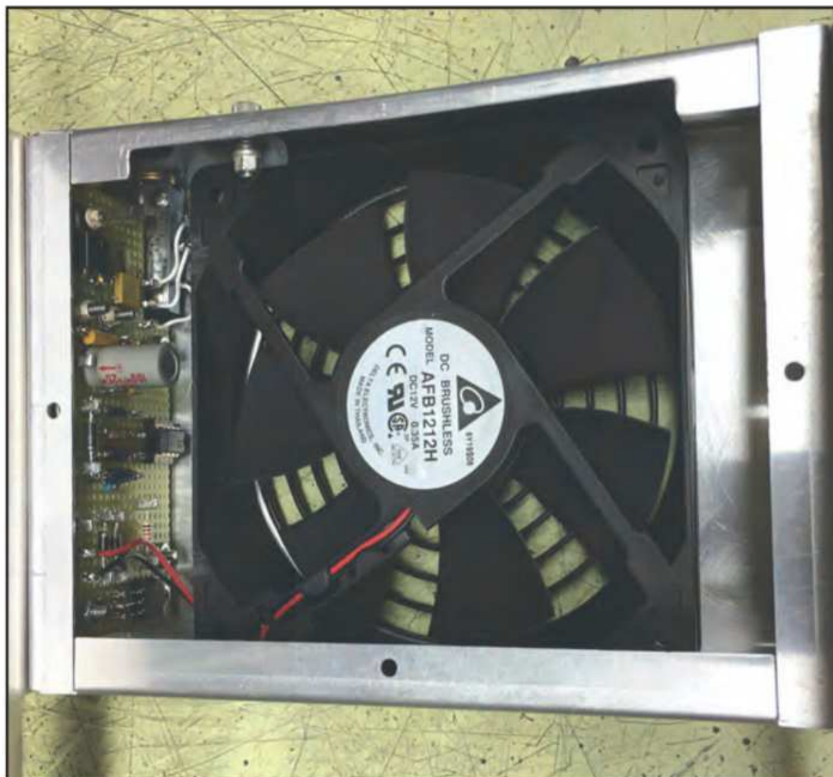
Photo F. The cooler's circuit board is mounted inside the enclosure, but out of the direct path of the airflow.
