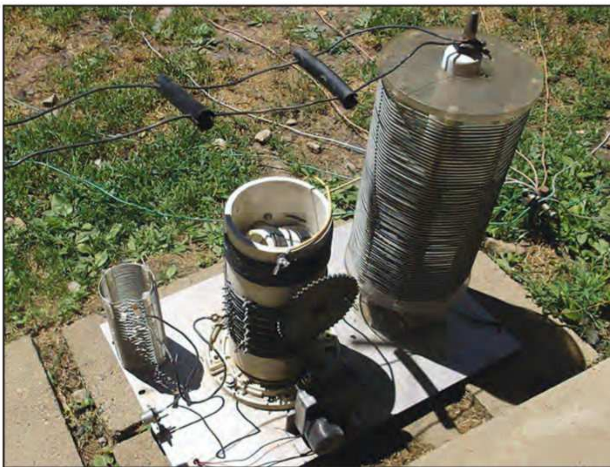
Photo C. Loading and matching for the 630-meter Marconi-T at W8CDX were accomplished by this junk box gem. A shunt match coil (left) feeds a small variometer (center) to allow frequency agility and fine adjustment. The larger coil (right) is in series with the variometer and manages the bulk of the loading. Both sides of the open-wire feed line are connected to the top of the coil. Note the minimal radials and ground rod to the right. (Courtesy of NO3M)
