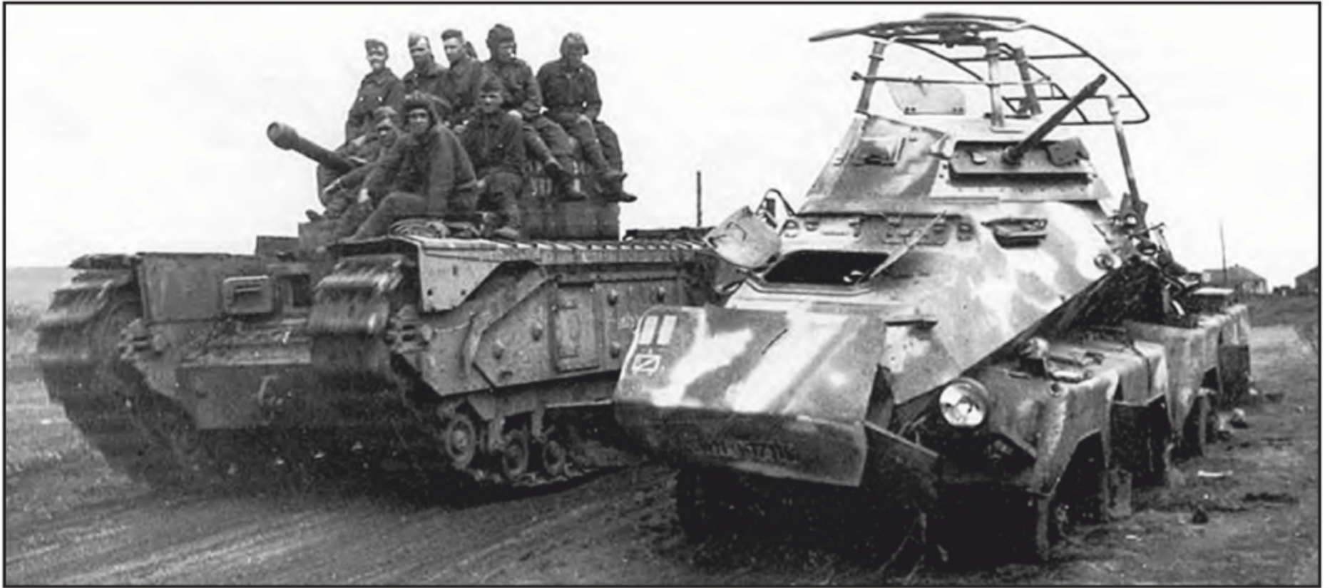
Photo A. German command vehicle on the right with NVIR loop antenna. It obviously did not survive the encounter with the Churchill tank. (Courtesy of Wikipedia.org)
