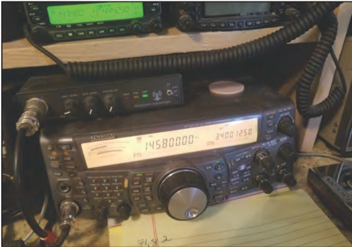
Photo H. The author's Kenwood TS 2000 X used to receive SSTV pictures. Note the West Mountain RIGblaster Advantage sitting on top of the Kenwood. (The author needs to dust off his equipment.)
