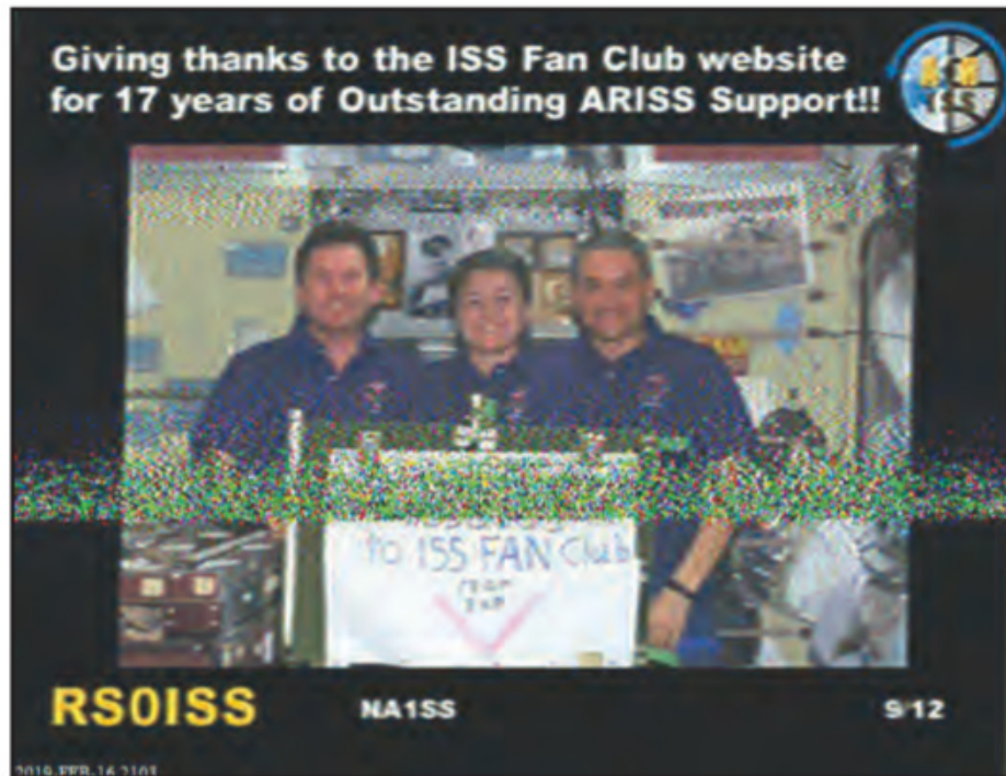
Photo E. The ISS transmitting picture 9 of 12 in February. Doppler shift, fading, and signal variations contributed to the noise (pixelated dots) on my received picture. Not a perfect picture, but still exciting to get.
