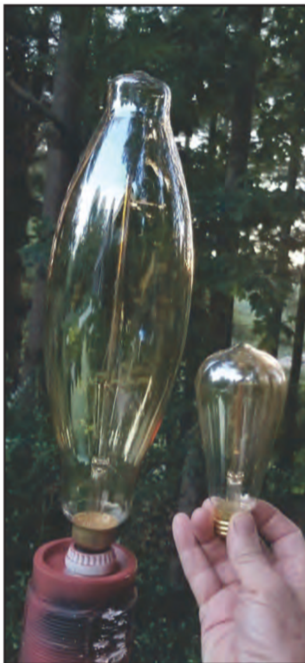
Photo A. A 100-watt Satco S2431 light bulb (left) and the Edison "squirrel cage" light bulb (right).
