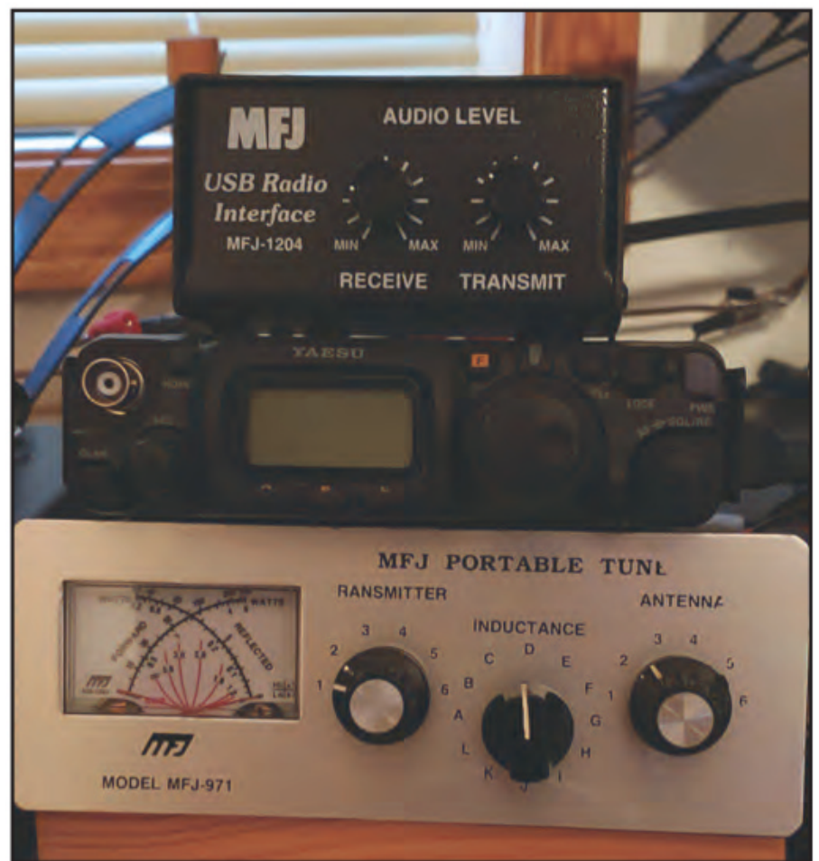
Photo A. The MFJ-1204 USB Radio Interface (top) mounted atop the Yaesu FT-817.
