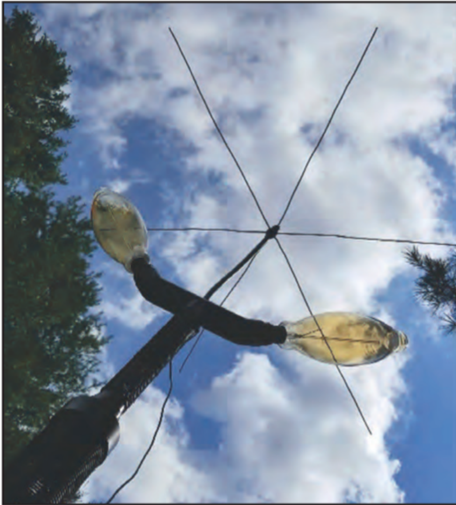
Photo C. Dual light bulb antenna and capacitance hat.
