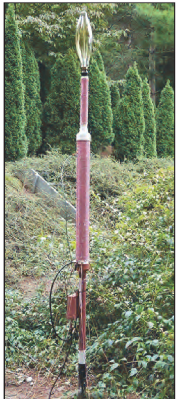
Photo B. LBA MK V Light bulb antenna.
