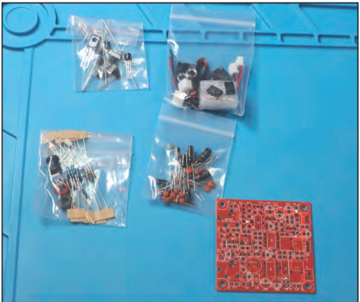
Photo B. Chinese “49er” 40-meter CW transceiver kit ready to assemble.
