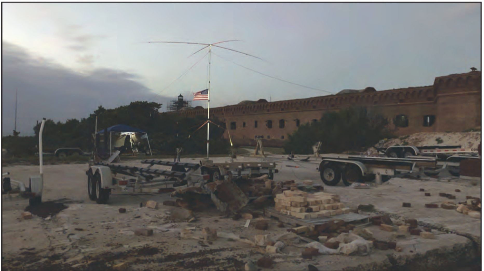
Photo A. The TN07 Engineering 20-meter X-Beam and RadioWavz 40-meter double bazooka antennas stand atop the MGS MK4-HD push-up mast with Fort Jefferson in the background. The flag is at half staff in remembrance of President George H. W. Bush. (Photos by James Lea, WX4TV)
