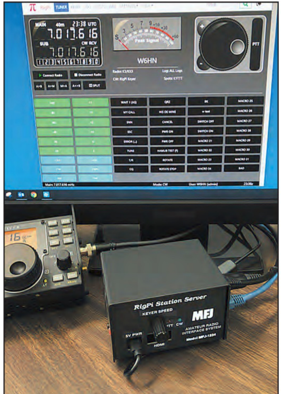
The RigPi™ in action. Here it's connected to an Elecraft KX3 along with the monitor showing RigPi Server Software in a web browser. (Courtesy of Howard Nurse)
