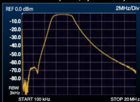
Band Pass Filter (7MHz, Span 20MHz)
