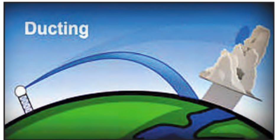
Figure 4. Temperature inversions combined with humidity can create favorable boundaries (ducts) for VHF-SHF communications.
