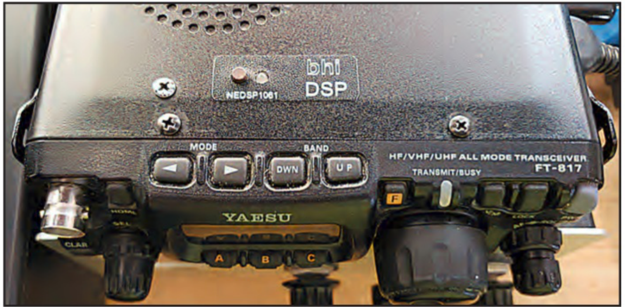
Photo E. A happy FT-817 showing off its push button switch for the noise reduction module.
