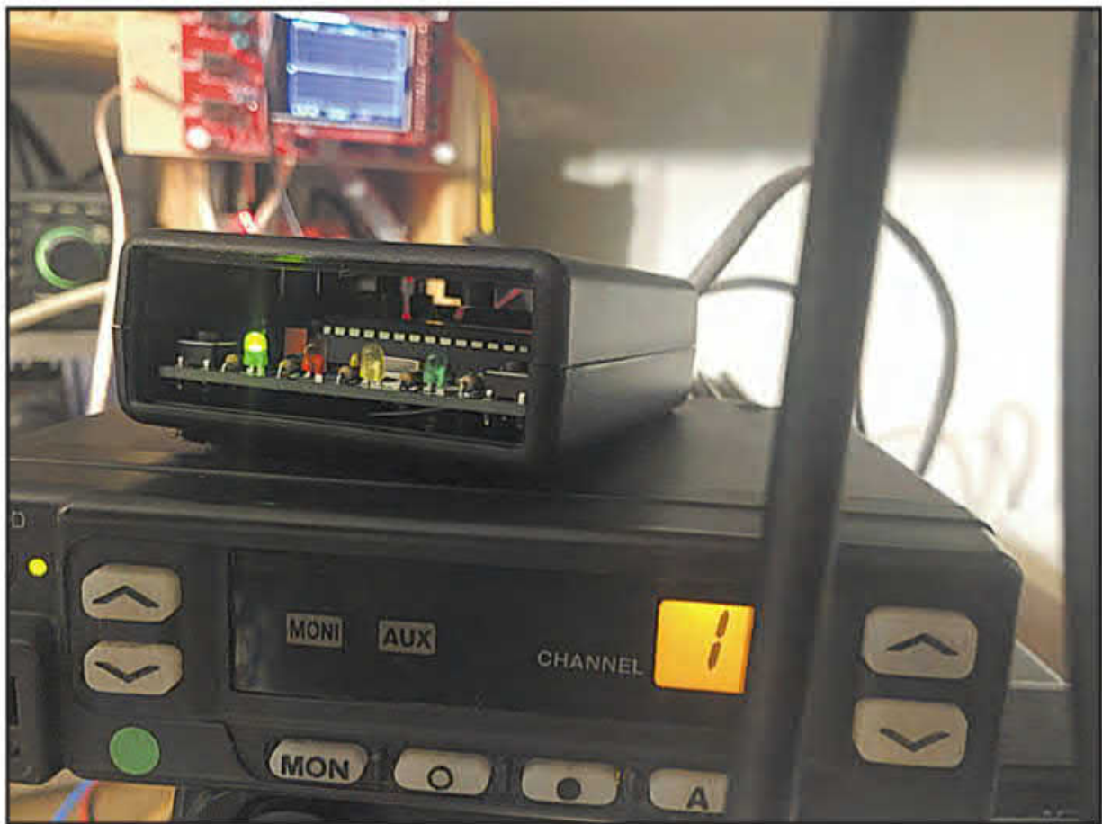
Photo A. A prototype NinoTNC, installed in a plastic case, as part of a test link at Tadd Torborg, KA2DEW's, house. The link managed over 300 bytes per second. (Courtesy of Tadd Torborg, KA2DEW)
