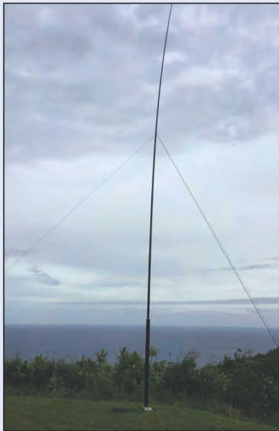
This is the 60-meter vertical used at VP6R to make nearly 1,000 FT8 QSOs on the band. Getting permission to operate on 5 MHz was a major effort! (Photo courtesy of the VP6R team)
