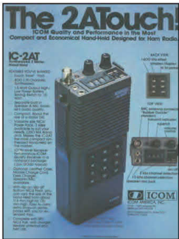
Photo L. ICOM revolutionized the VHF handheld market with the frequency-synthesized IC-2AT. The hold of crystal-control had finally been broken.
