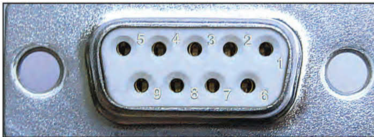
Photo B. A DE-9 female connector, the de-facto standard to interface a TNC with a data radio. My first experience with this configuration was on the TEKK KS-900 data radios. Pin 1 is data to the radio, Pin 2 is ground, Pin 4 is PTT and Pin 5 is data from the radio. (Courtesy of Wikimedia)
