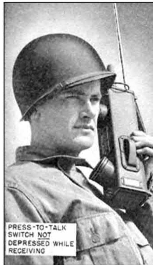
Photo A. The SCR-536 walkie-talkie was the ultimate in World War II radio miniaturization. (Public domain photo via Wikimedia Commons)
