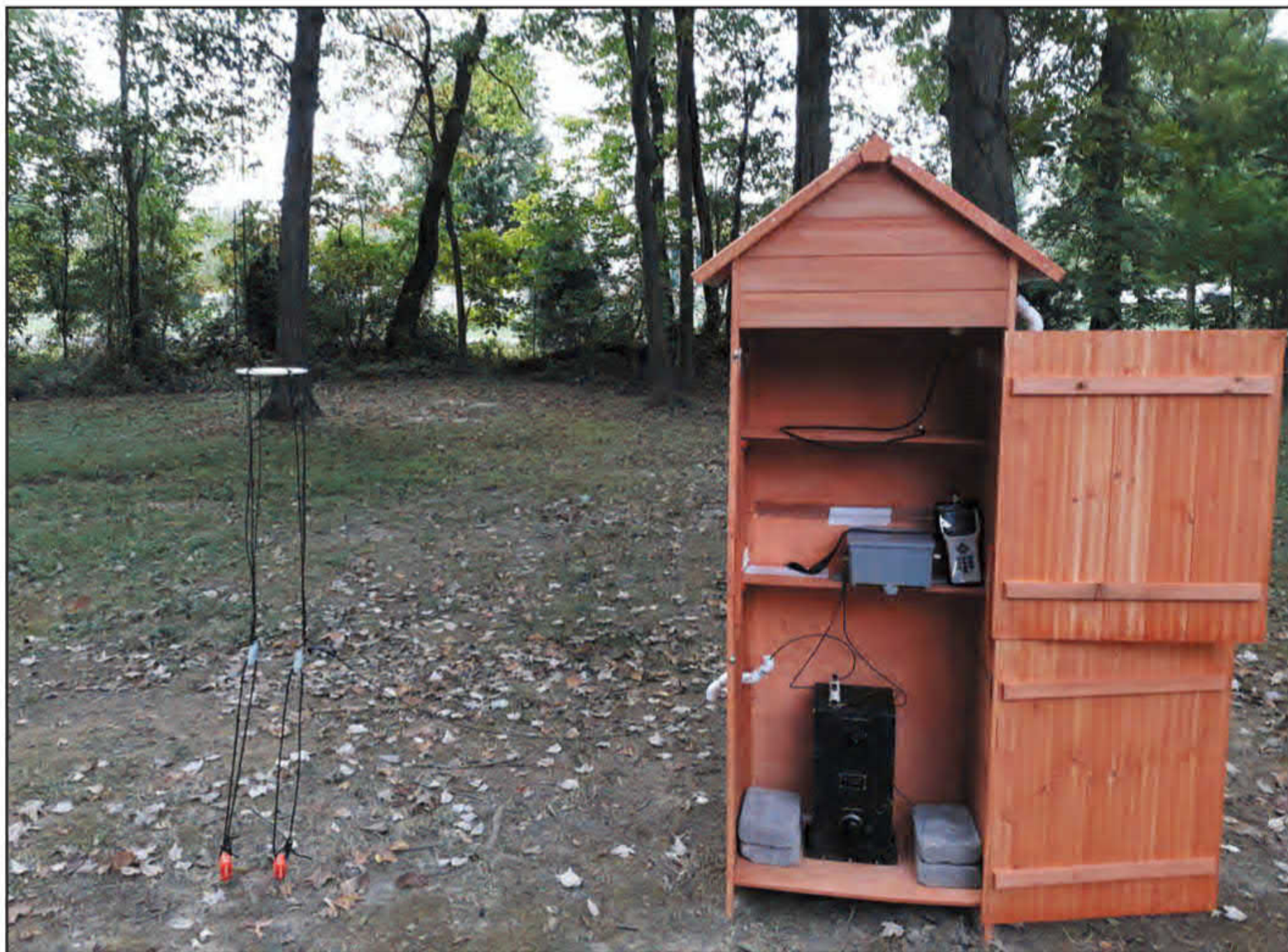
Photo L. This attractive antenna system at N9RU utilizes a 50-foot-tall tree, which supports a six-wire caged vertical with a 110-foot-long top-loading array consisting of three wires spaced 3 feet apart and fed against a radial system. A military surplus variometer resonates the system.
