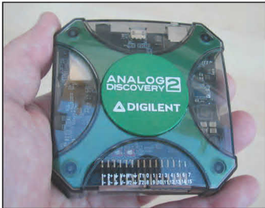
Photo J. The Analog Discovery 2, top view. This is a multi-function test instrument in a box that fits in the palm of your hand. It connects to a computer via a USB port.
