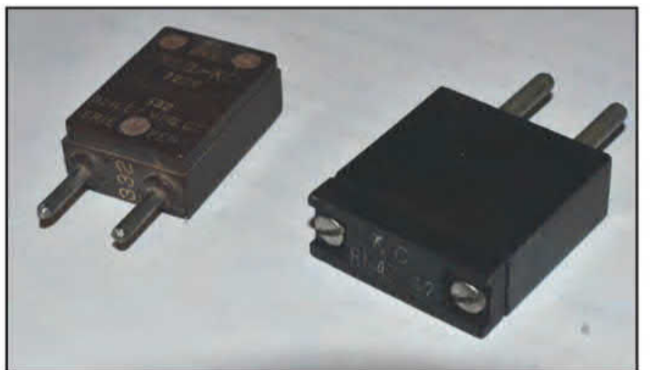
Photo D. Seventy-five years ago, crystals were the primary means of generating an RF signal. (Photo by KOØZ)
