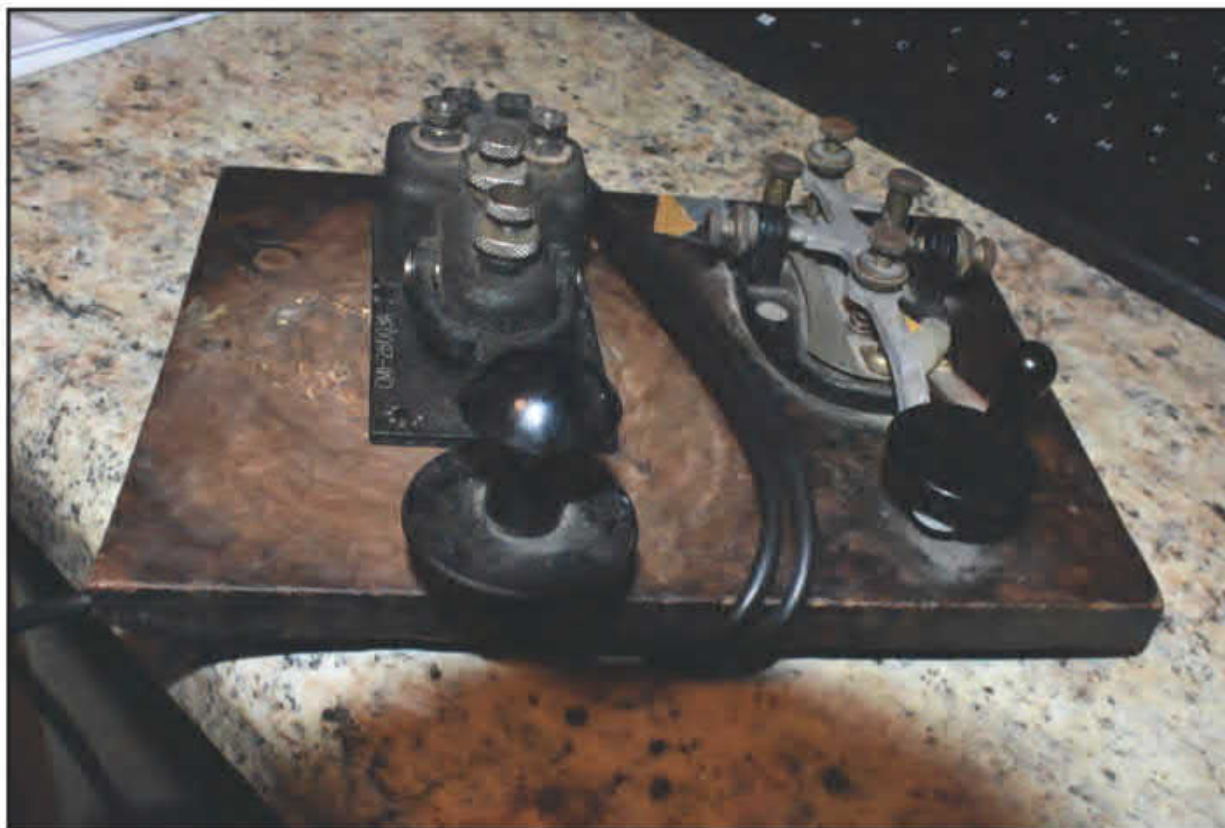
Photo E. WWII era Morse code straight keys used for sending CW. (Photo by KOØZ)
