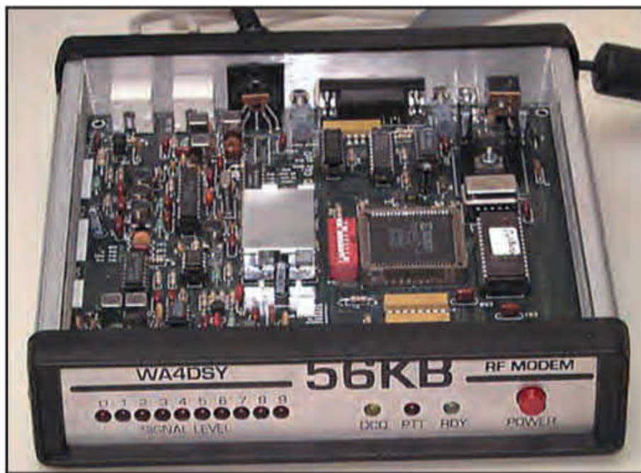
Photo D. A 56k GRAPES modem. Note that it is called an RF modem: The output was not at baseband (audio) but at around 30 MHz, requiring a transverter to place the signal on a legal frequency. This complexity was the primary challenge to its widespread use. (Courtesy of Dale Heatherington, WA4DSY)
