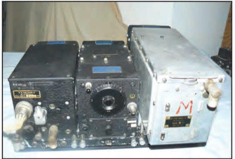
Photo C. WWII era ARC-5 military radio eventually found its way into ham shacks via electronics surplus. (Courtesy of Wikimedia Commons)
