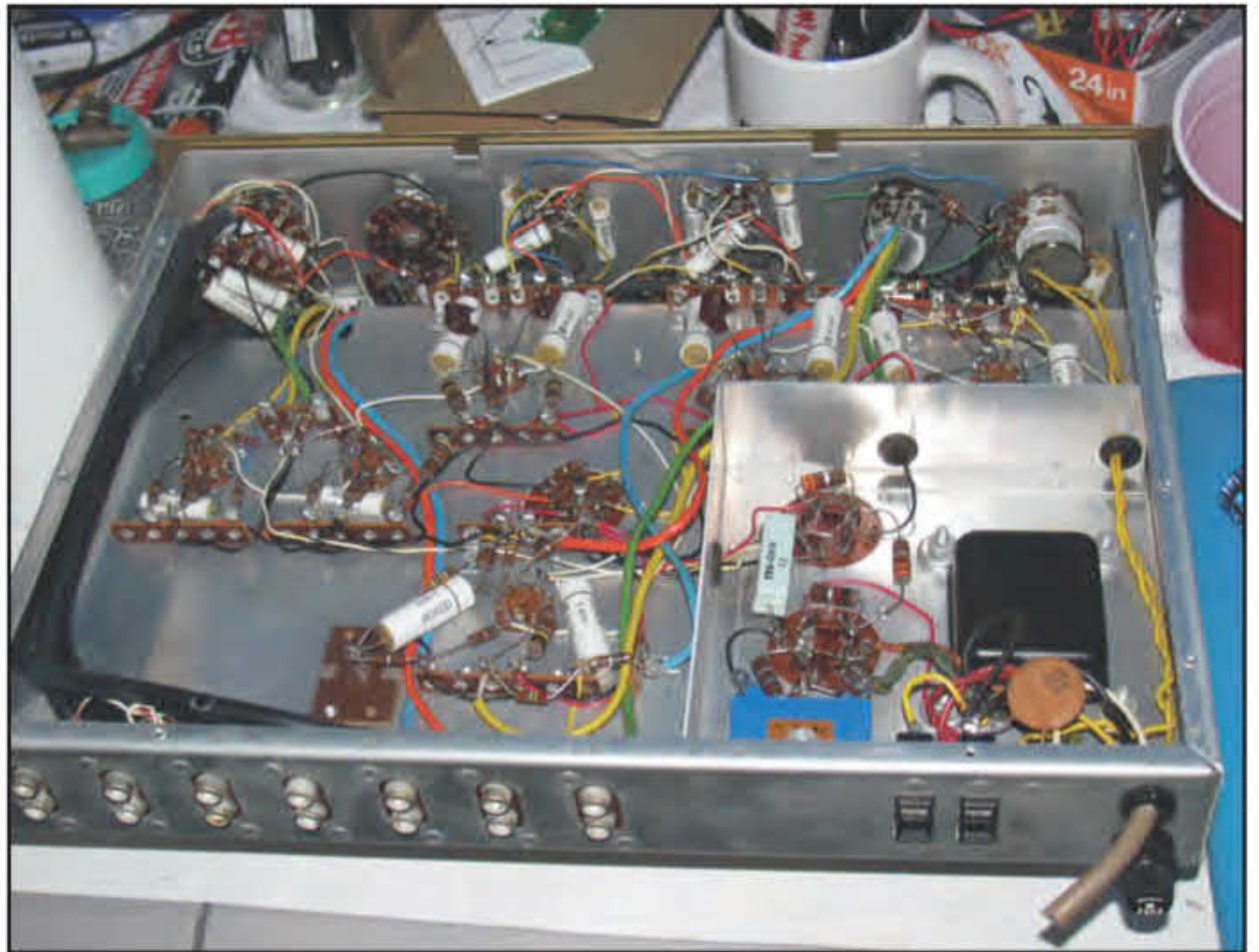
Photo A. This stereo amplifier is shown as an example of point-to-point wiring. It's very labor-intensive, compared to anything made with printed circuit board wiring.
