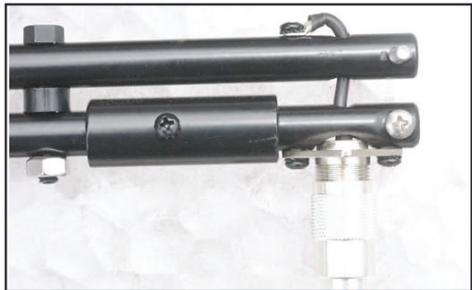
Photo G. SO-239 connector supplied with the Elk. Notice the two booms held apart with an insulator.
