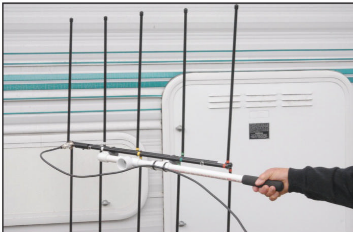
Photo D. The Elk log periodic antenna is great for hunting down noise sources on VHF and UHF.
