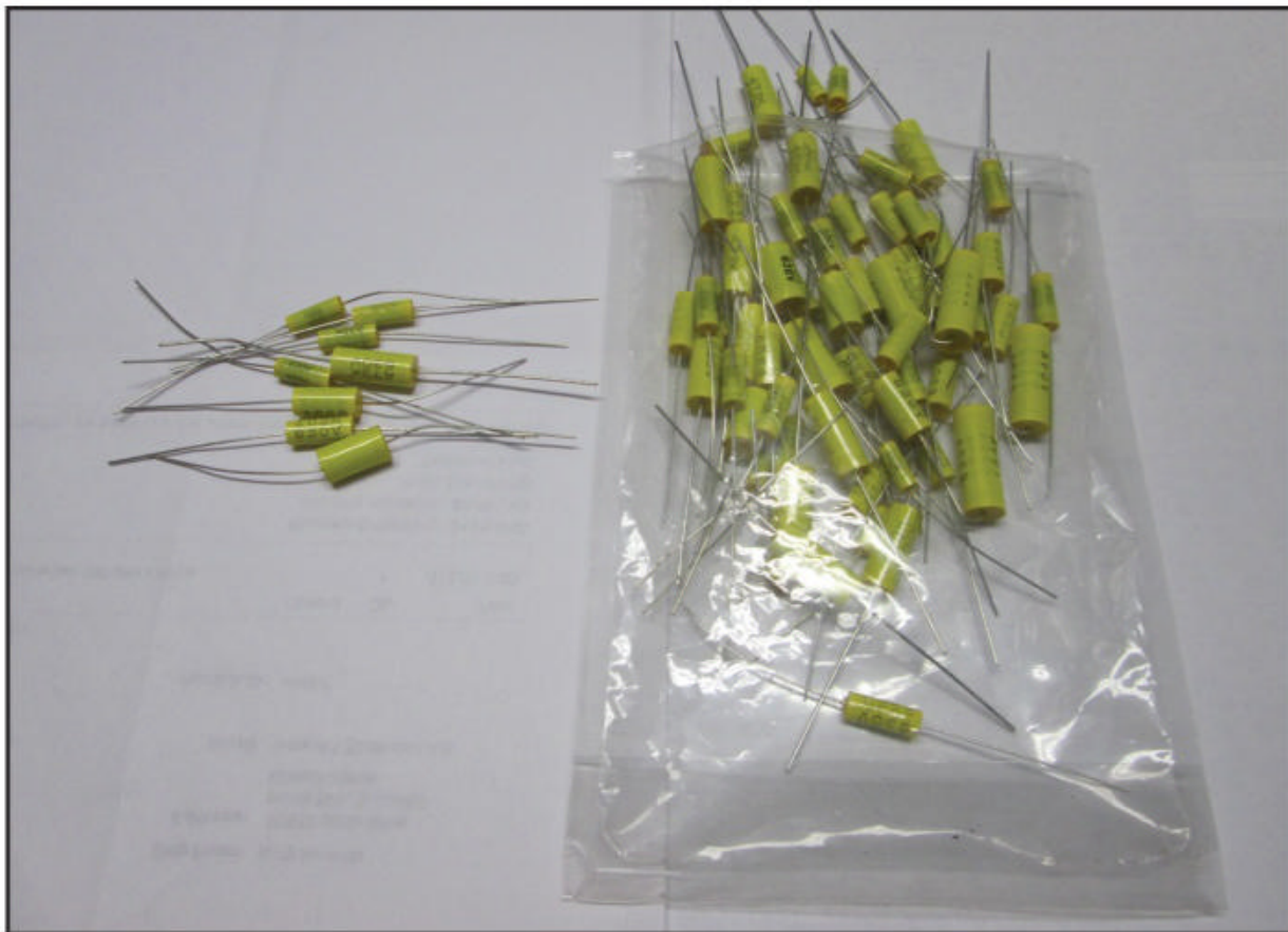
Photo B. 600-volt Mylar capacitors.
