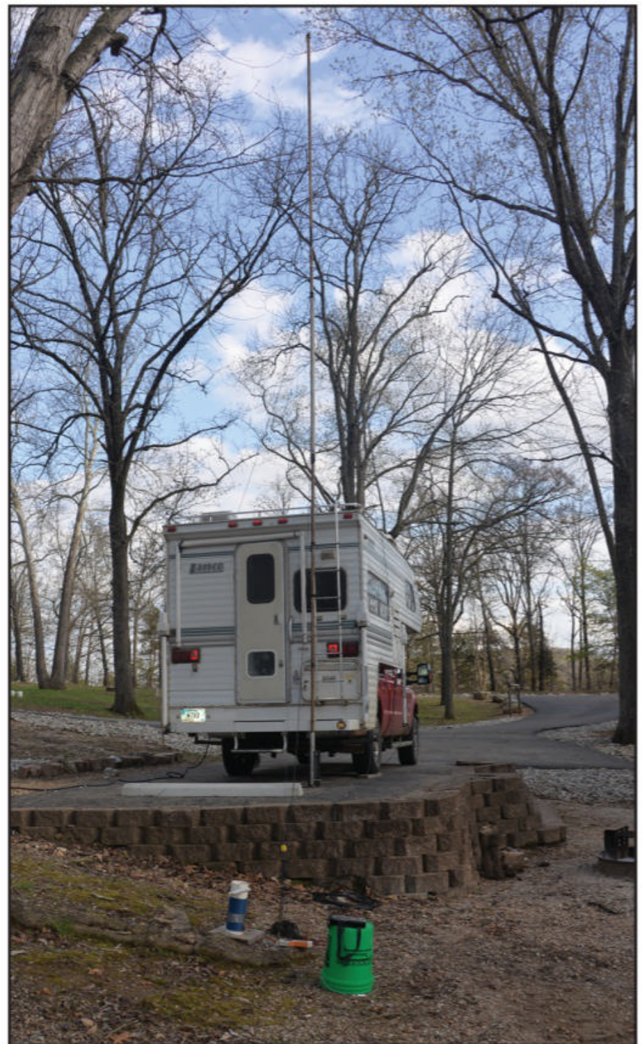
Photo D. W7XU reports that this is the, “set-up at Cricket Creek Campground in northwest Arkansas. Visible is the fiberglass mast off the back of my camper. It supported an inverted-L about 30-feet high and 100-feet horizontal. I had six radials, each 50-feet long. The loading coil is visible in the foreground.” This system netted three FST4 QSOs through very challenging noise conditions.
