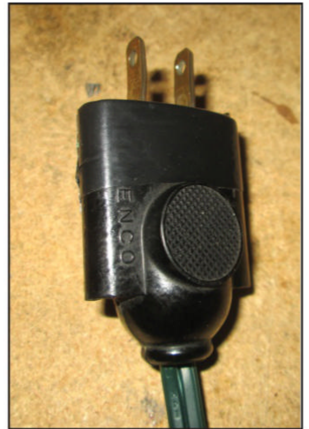
Photo E. Two-wire double-fused Heathkit or Johnson style plug.
