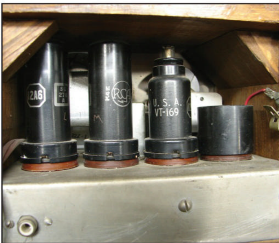
Photo F. The restored chassis reinstalled in the original builder’s homebrew wooden cabinet.
