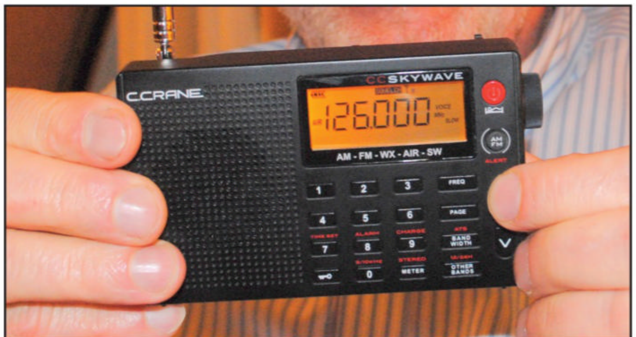
Photo C. Finding noise sources, using the CCrane receiver on AM.
