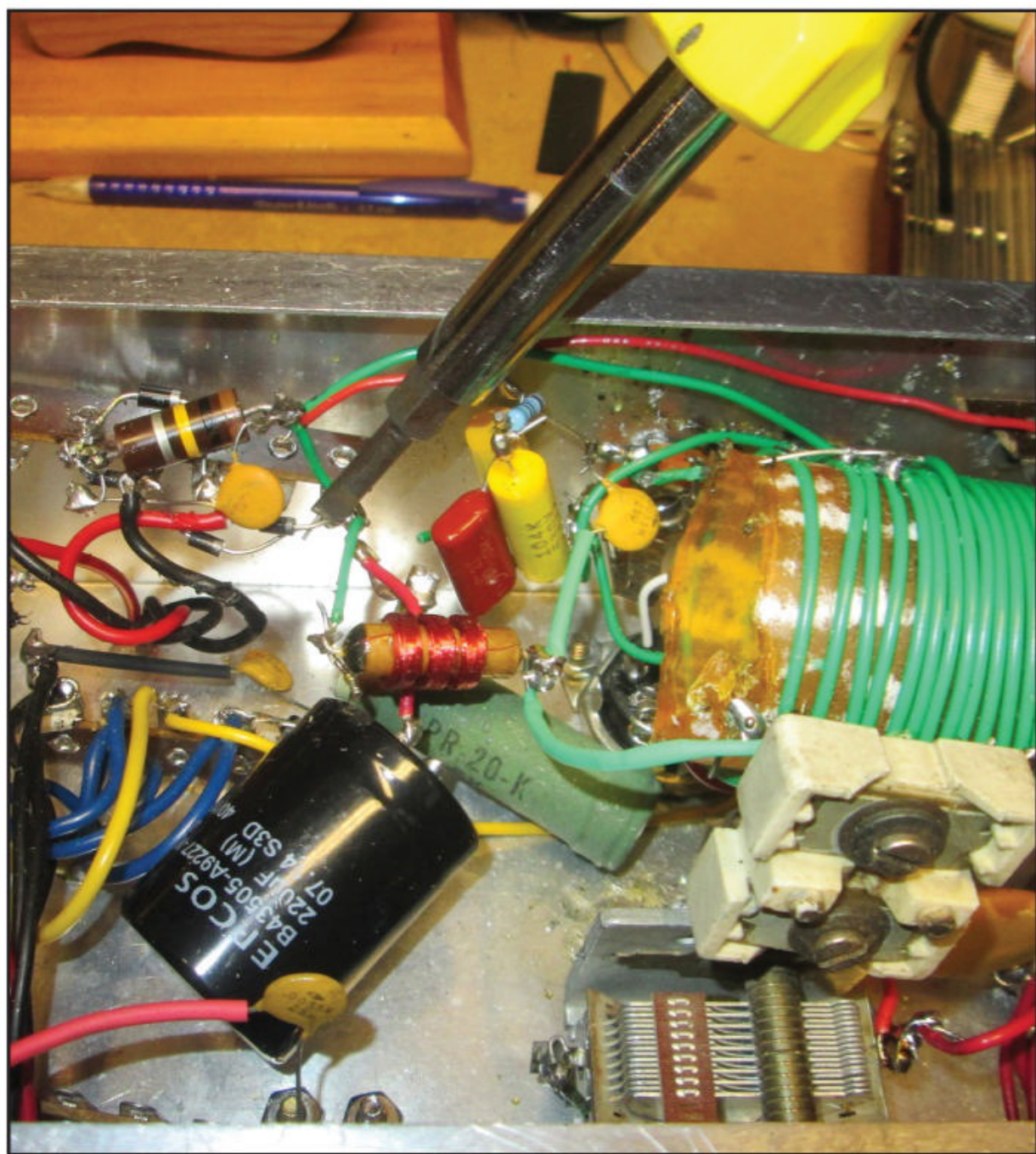
Photo C. High-voltage electrolytic discharge technique. Note that operator is insulated from metal and that the shaft of the screwdriver is touching the metal chassis.
