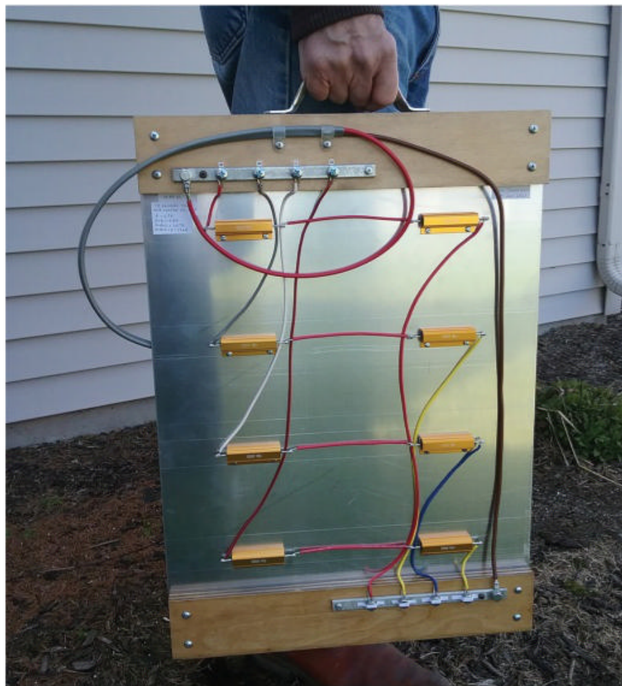
Photo A. KBØVKS's "dummy load for power supplies." The large sheet of aluminum is necessary for effective heat dissipation.
