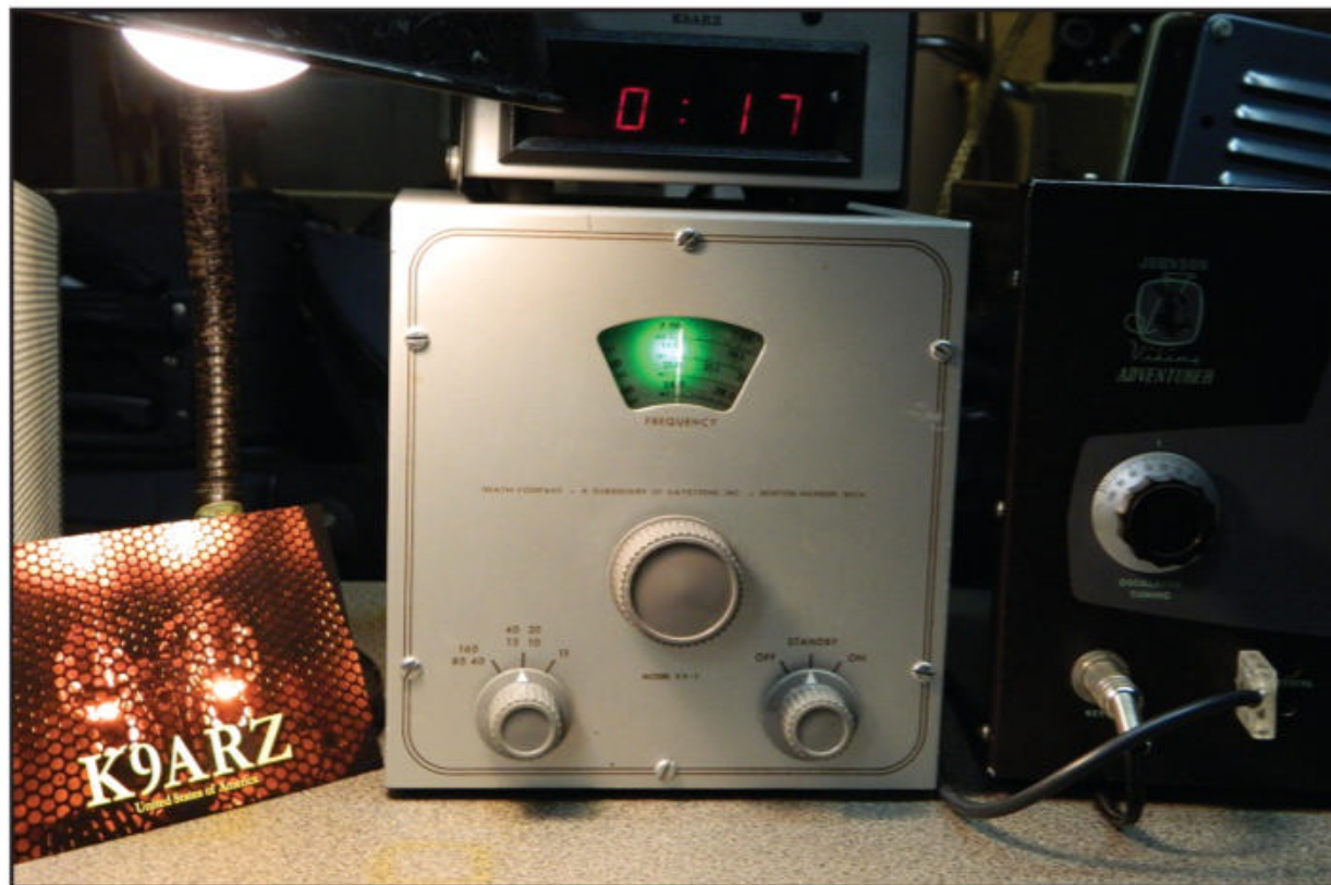
Photo B. The author's Heathkit VF-1 external VFO is currently teamed up with his classic Johnson Viking Adventurer transmitter.
