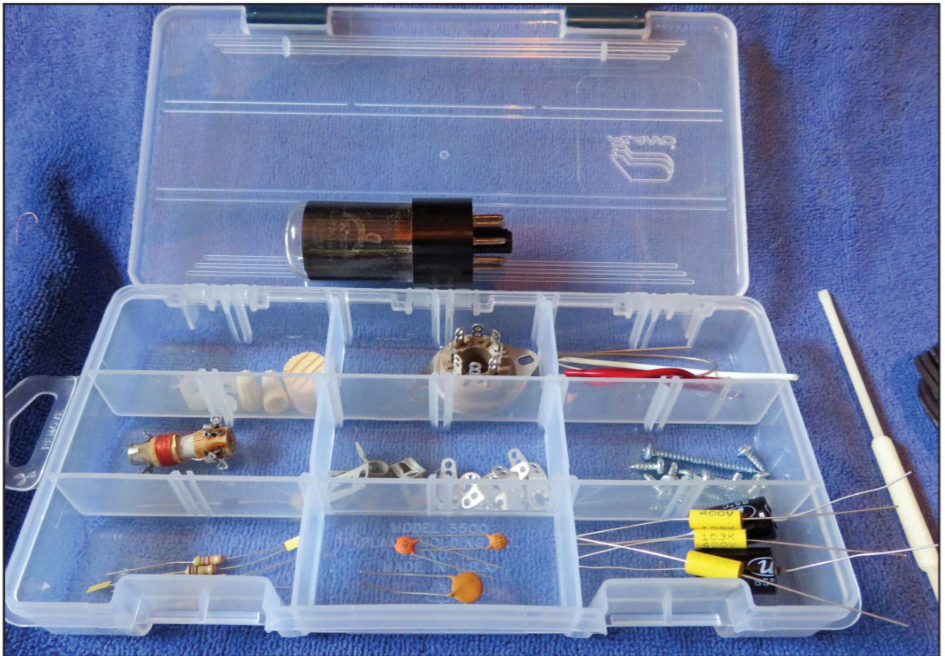
Photo A. The K-488 AM transmitter parts all sorted out and ready to assemble. The tuning tool was included in this kit, as was the 12SA7 tube.
