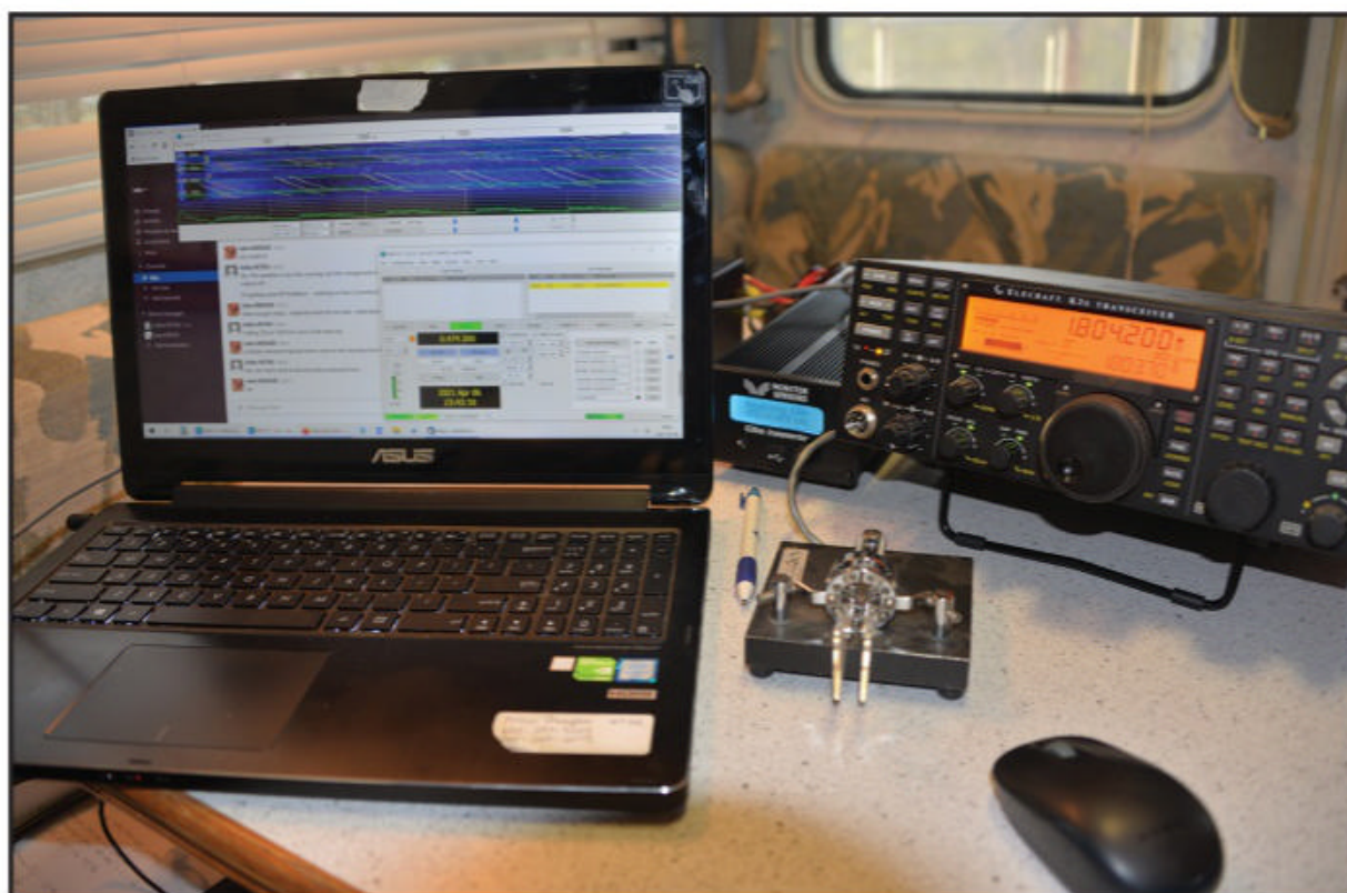
Photo C. This simple operating position made a number of 630-meter operators happy as W7XU activated two states that have until now eluded on-air activity. The Elecraft K3S used a 160-meter IF to drive a Monitor Sensors transverter. FST4 and CW were used during these operations. Note the level of local interference on the waterfall that was experienced from this site in Arkansas.
