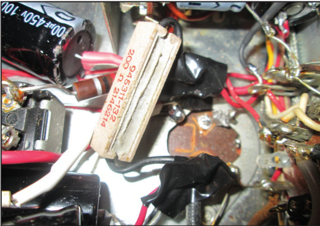
Photo D. Ugly method of replacing above-chassis multiple capacitor cans.
