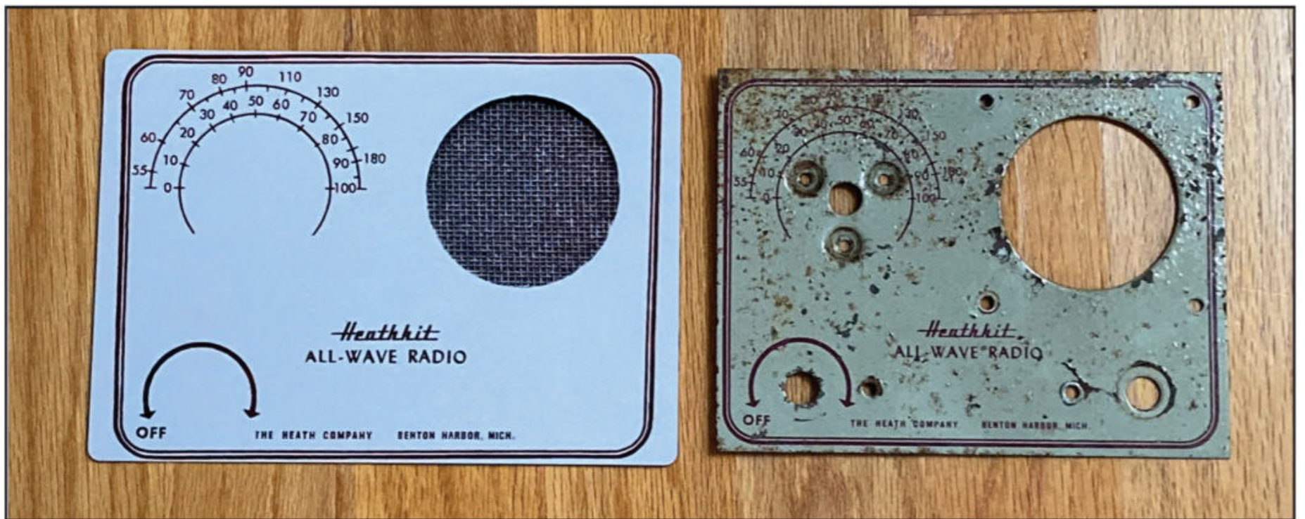
Photo E. N8RG had to recreate the front panel by taking a high-resolution photo of it, filling in the pitting and other damage pixel-by-pixel and then having the “new” image printed onto a piece of sheet aluminum.
