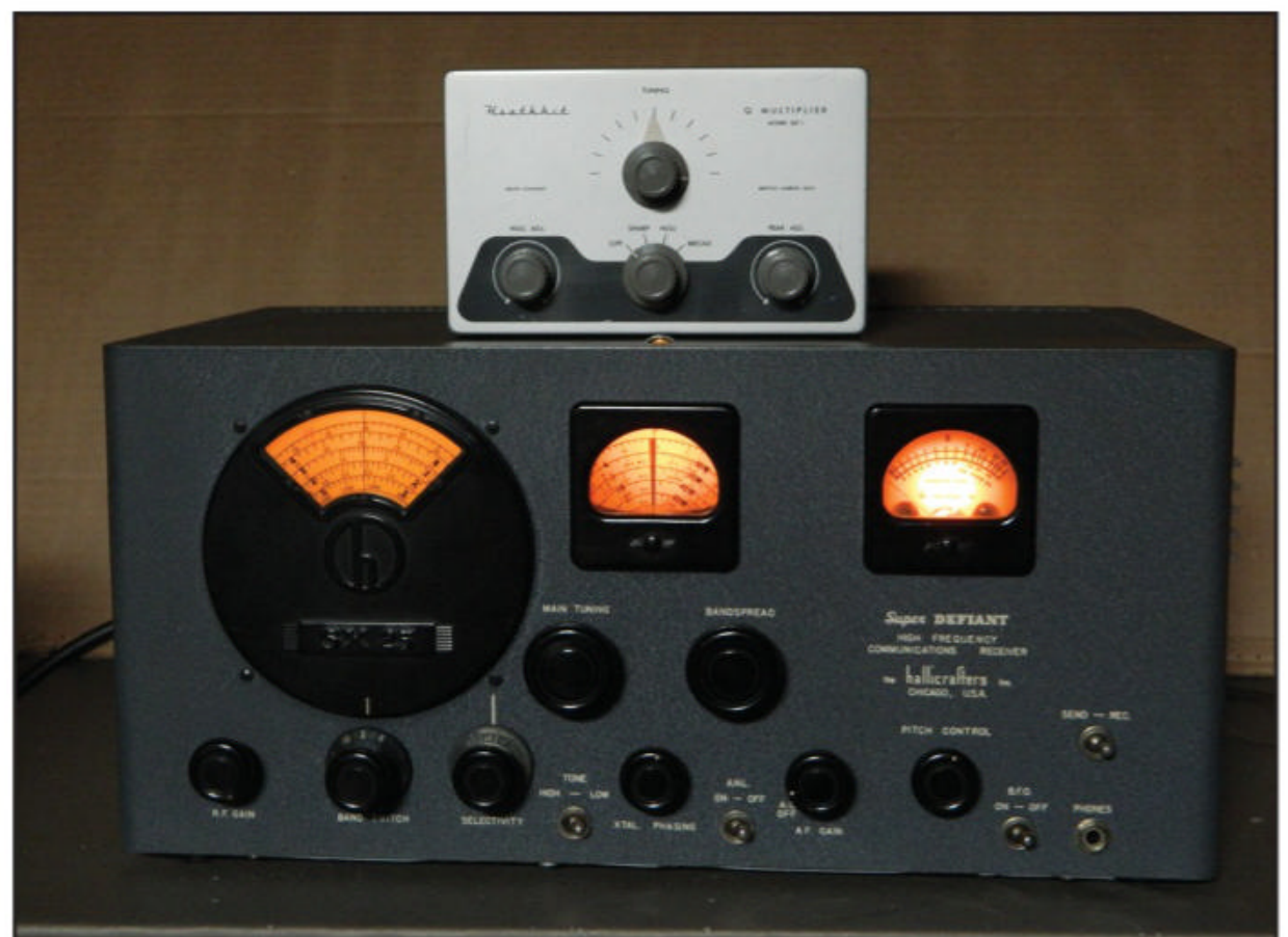
Photo A. The author’s Heathkit QF-1 Q-multiplier (top), still in use today with his Hallicrafters SX-25 receiver.
