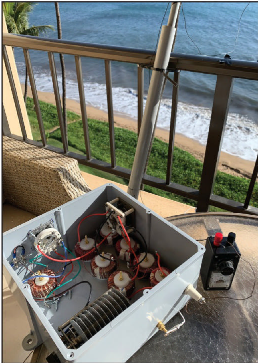
Photo A. The antenna feed point was quite close to saltwater on the sixth-floor balcony. This height above ground likely contributed to a far better system than calculations suggested on paper.
