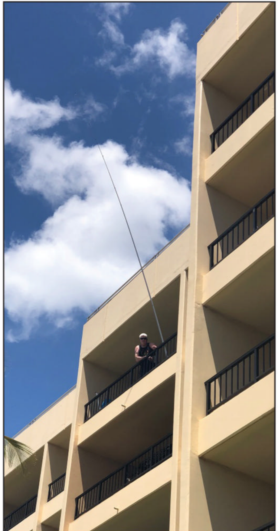
Photo B. Just because it’s not perfectly vertical does not mean it’s not a vertical antenna. KL7L’s arrangement of a sloping fiberglass pole from a balcony once again shows that successful 630-meter micro-operations are possible.
