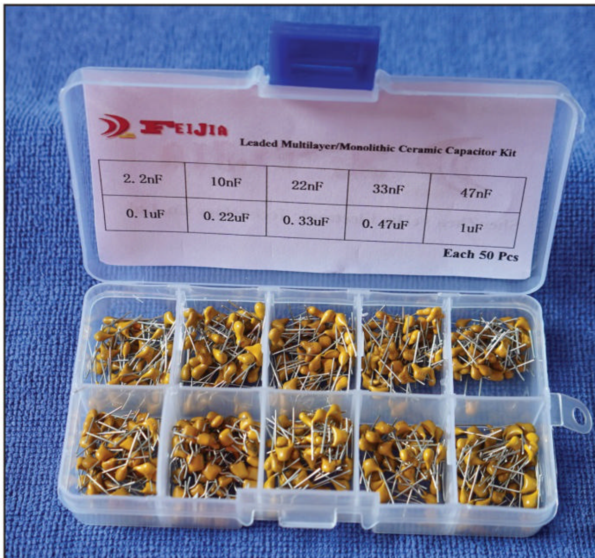
One of my capacitor assortments that made it possible to finish the kit without having to order parts to replace missing ones.
