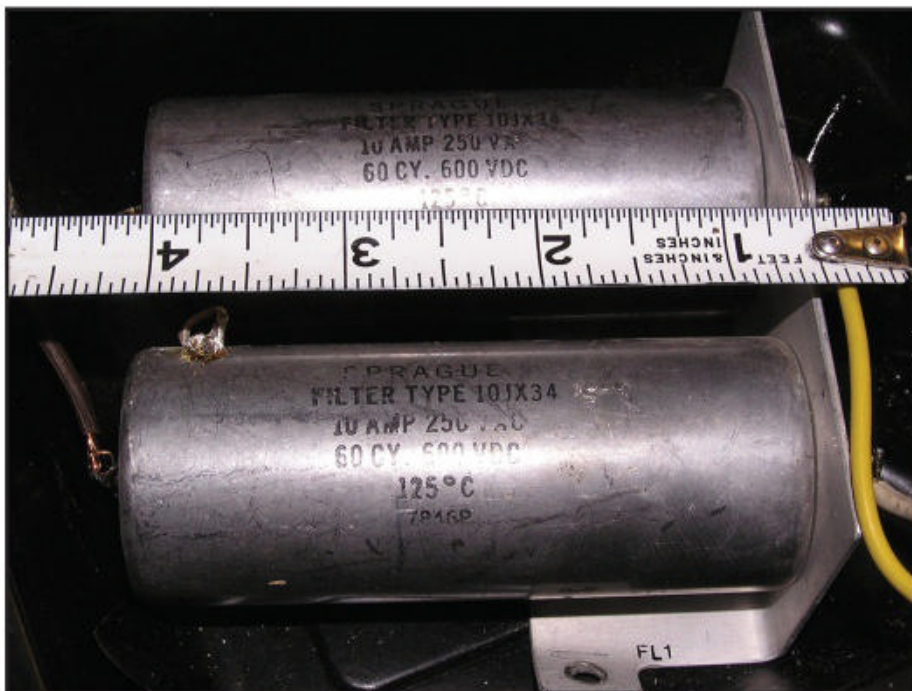
Photo D. You can also build your own filter, as Sherlock did for his battery chargers with these two big Sprague filters. See text for details and cautions when building your own.
