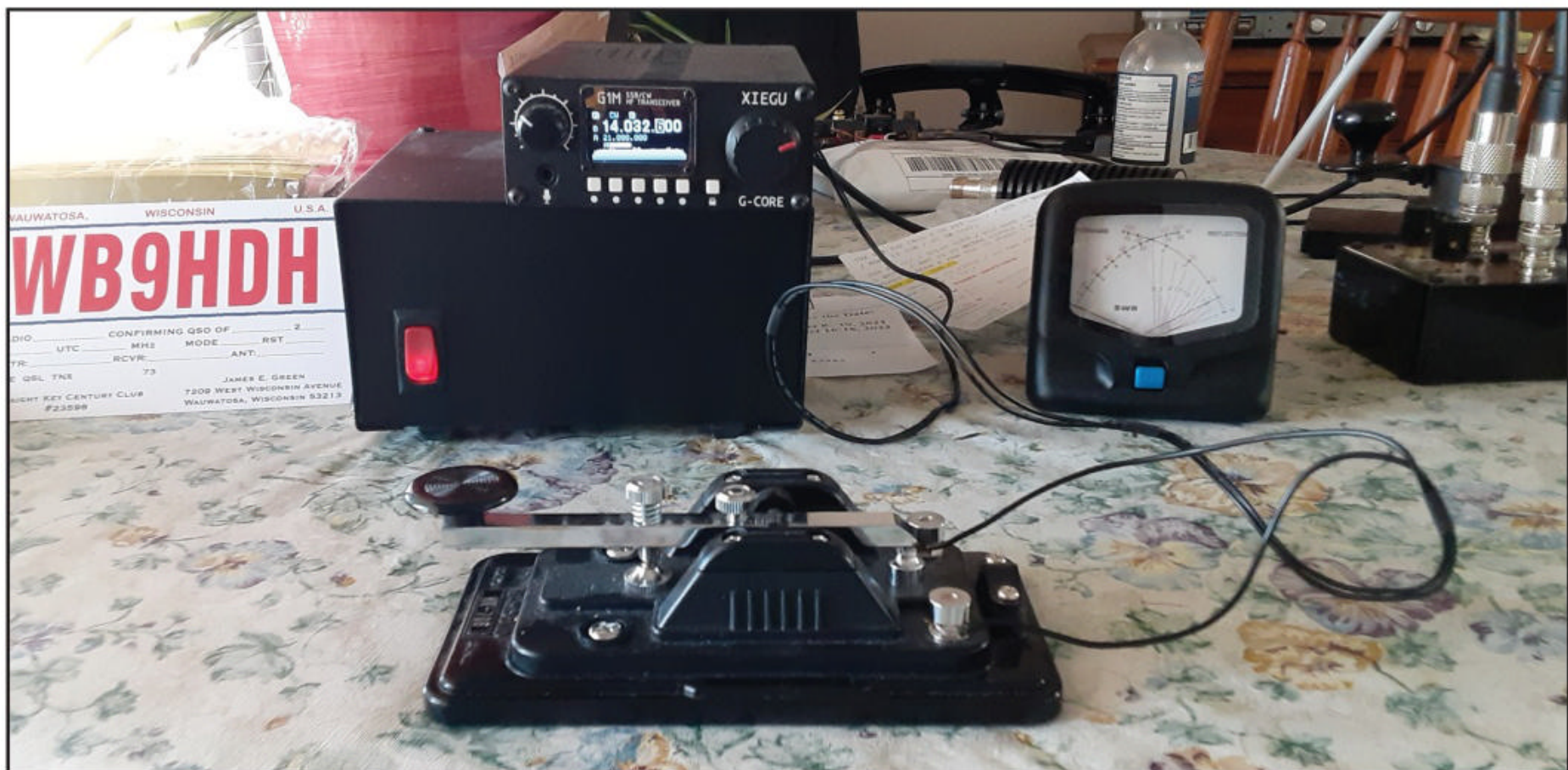
Photo B. WB9HDH station layout, featuring a Hi-Mound HK-708 telegraph key, with the Xiegu G1M QRP transceiver, power supply, and SWR meter in the background.
