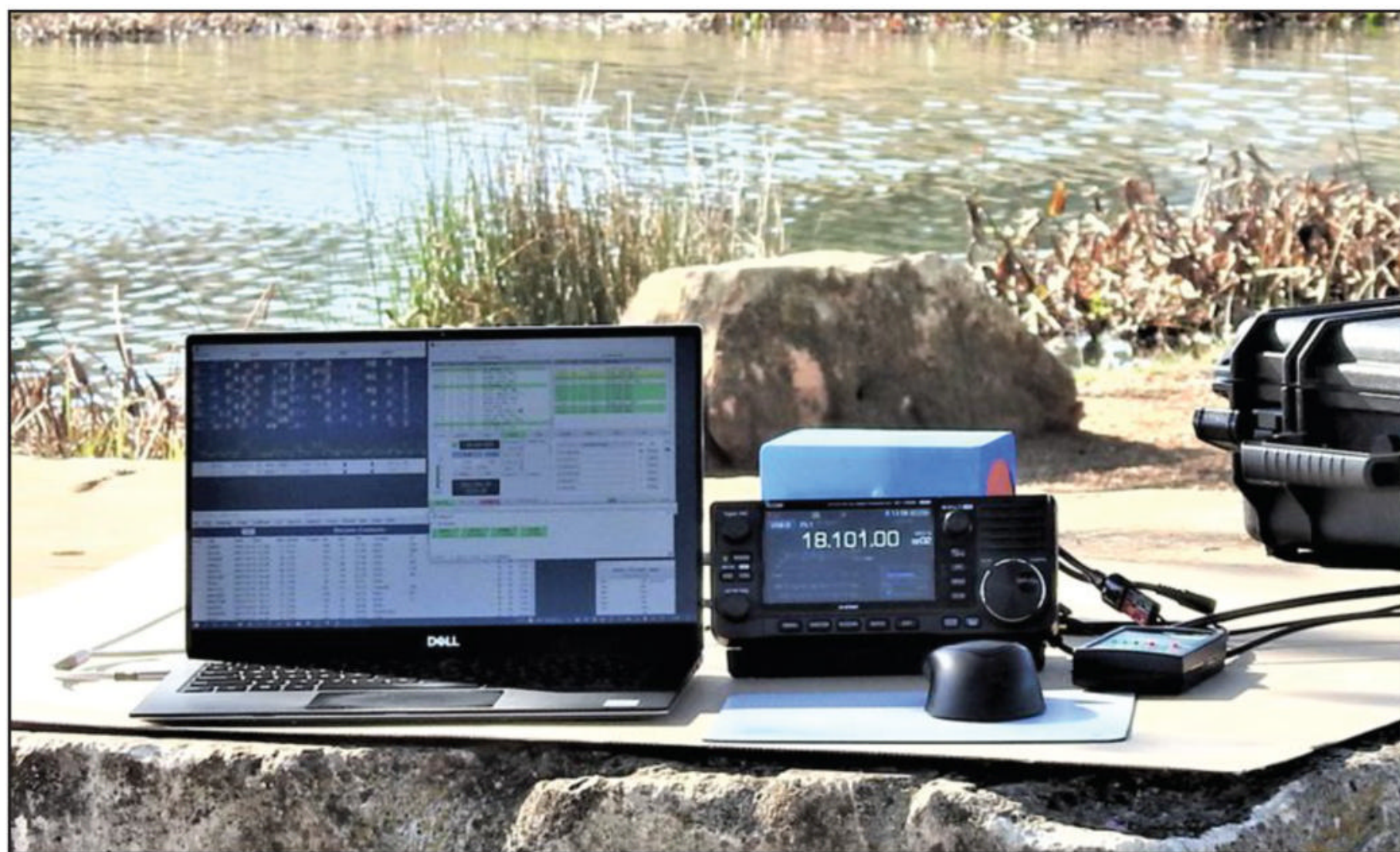
Photo A. QRP FT8 in the field (Photos / diagrams by the author except as noted)
