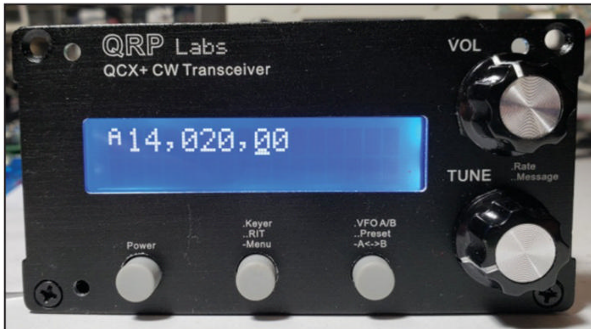
Photo A. The QCX+, a very popular CW transceiver offered by QRP Labs. (Photo from <qrp-labs.com>)
