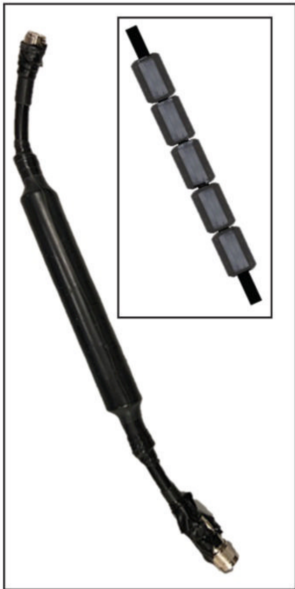
Photo H. Unnecessary inline RF choke with water-filled connectors (Inset shows construction without shrink sleeve)
