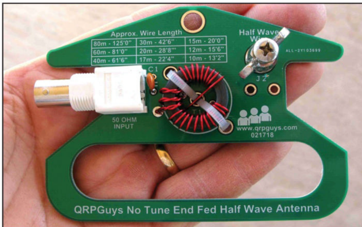
Photo B. The No Tune Half Wave Antenna by QRPGuys. You supply the wire. (Photo from <qrpguys.com>)
