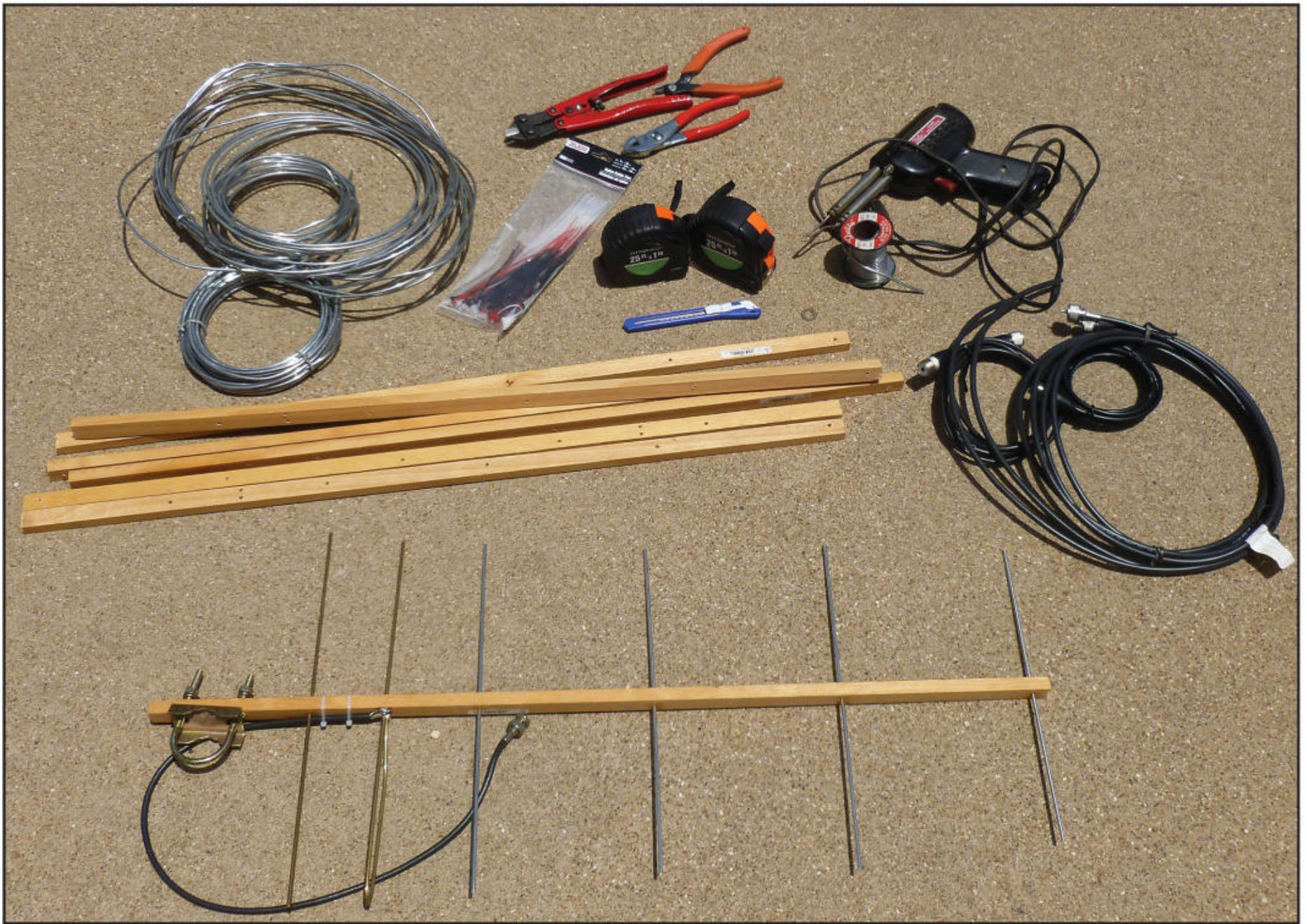
Photo B. Wood, wire, coax, and a few tools are all you need to build the Yagi shown here.
