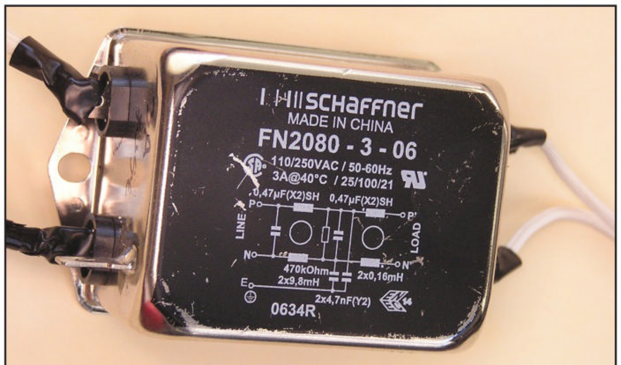
Photo B. These Schaffner power line filters are good for reducing 630-meter noise from low-current devices.
