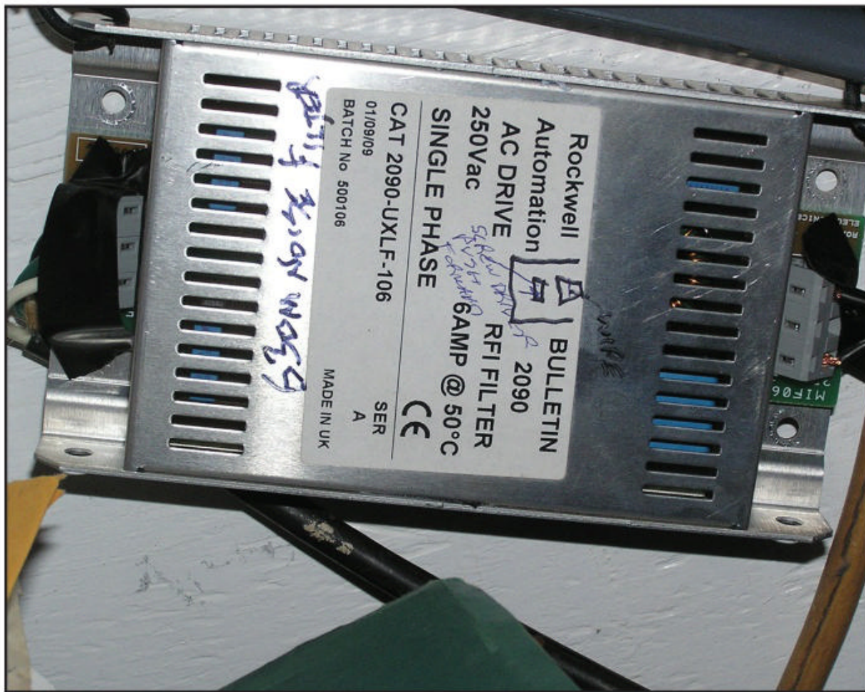
Photo C. Higher current devices, such as power supplies, need higher-rated filters, such as this 6-amp Rockwell Automation 2090.
