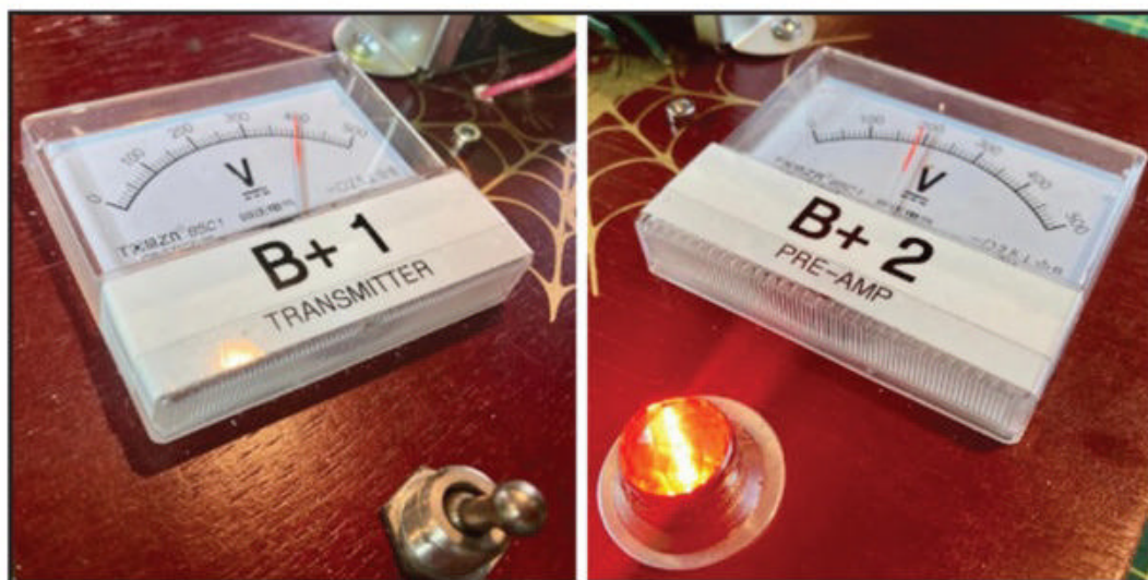
Photo G. Power meters add a new dimension to Bob Heil's Pine Board Project, which provided half the inspiration for James's project. Left: B+ No. 1 will deliver almost 400-volts DC to the transmitter. Right: B+ #2 will provide the 12AX7 tube plate with a safe voltage of 190-volts DC.
