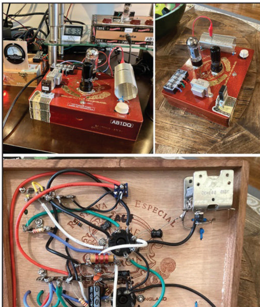
Photo I. The transmitter assembled in the cigar box.
