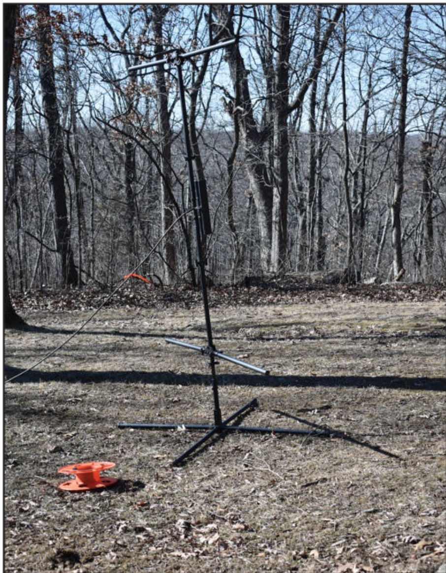
Photo G. TransWorld Basic antenna used by SLQS Winter Field Day. It covers 10, 12, 15, 17, and 20 meters.
