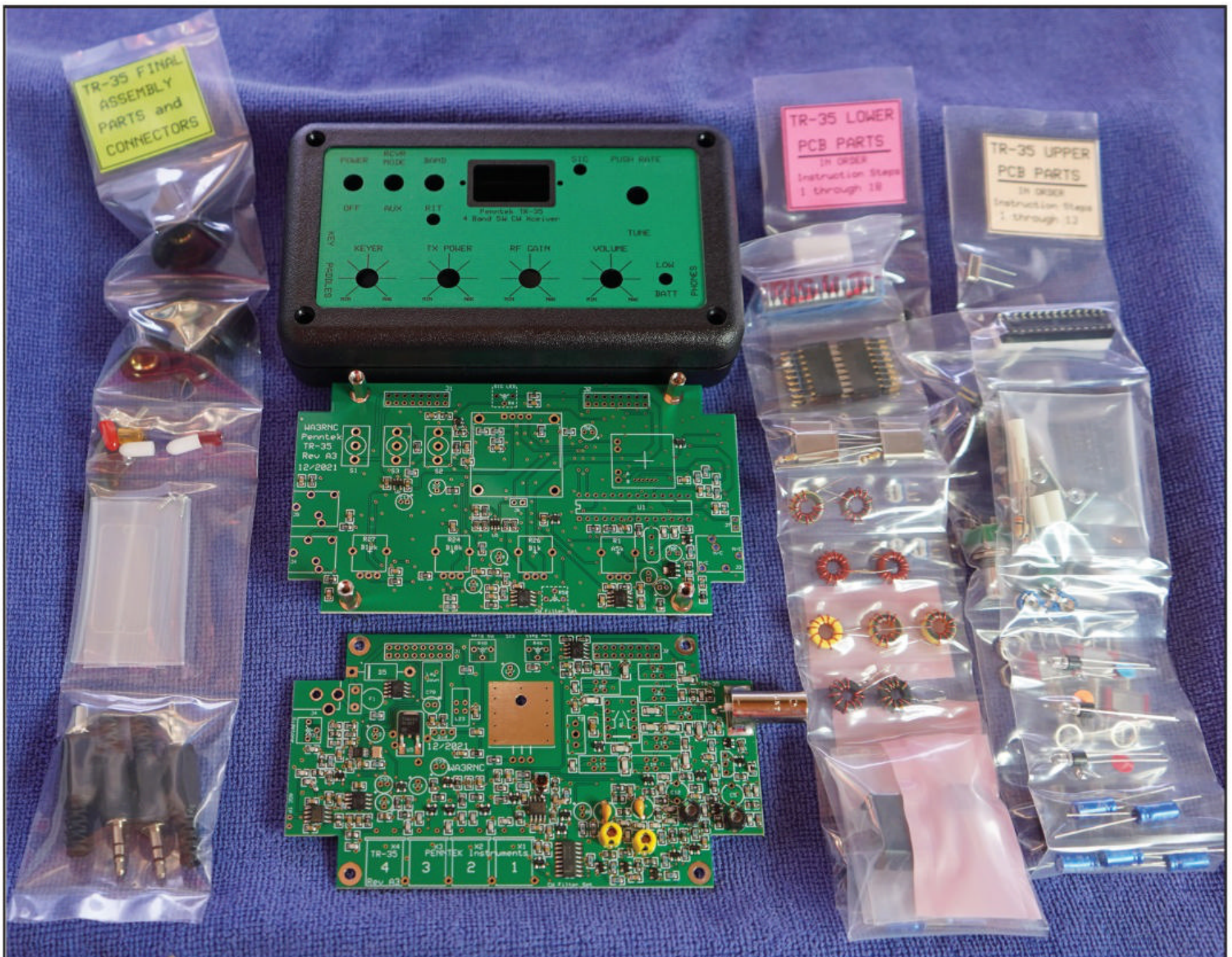
The parts for the Penntek TR-35 are pre-sorted and packaged in the order in which they are used, making the kit ready to assemble right out of the box.
