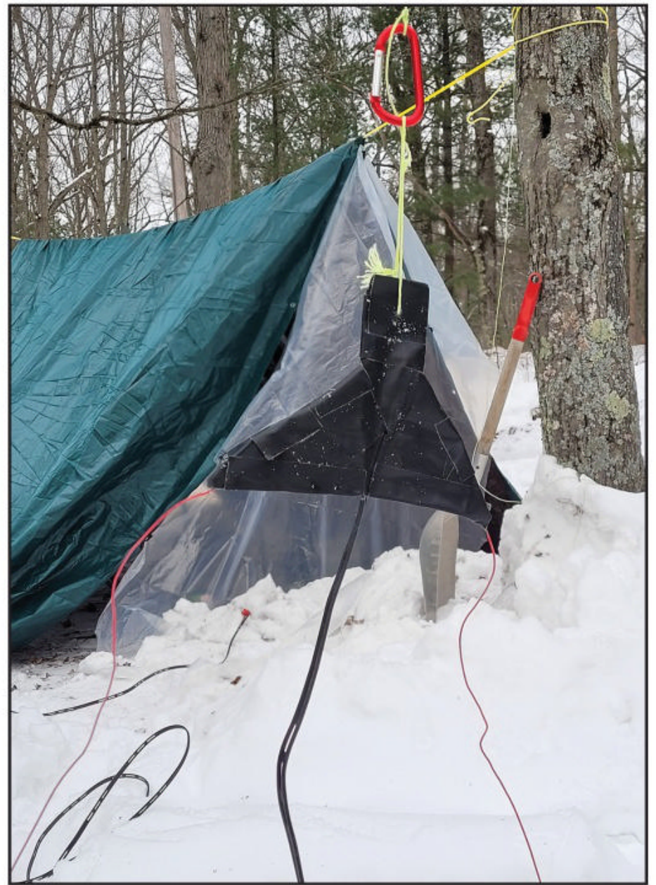
Photo D. Up and away! My 40-meter inverted-V antenna being readied for deployment.
