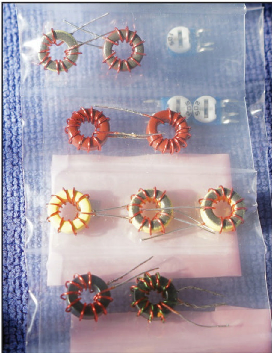
The toroids are already wound and prepared for mounting, and are packaged in the order in which they are placed on the board.
