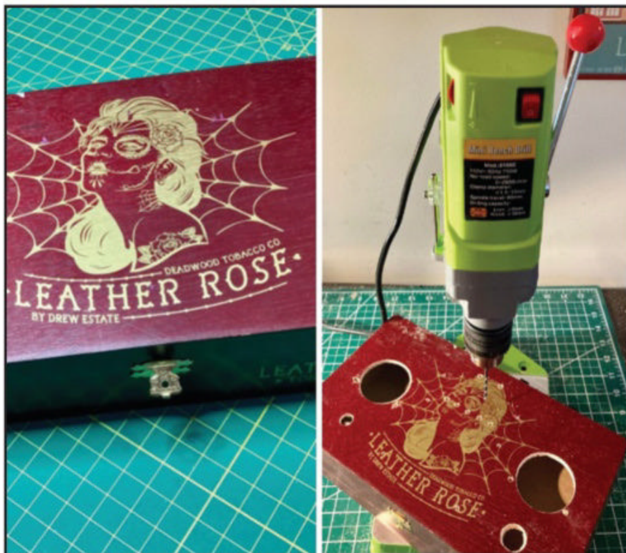
Photo E. Starting to assemble the second power supply, James drills holes in a cigar box.
