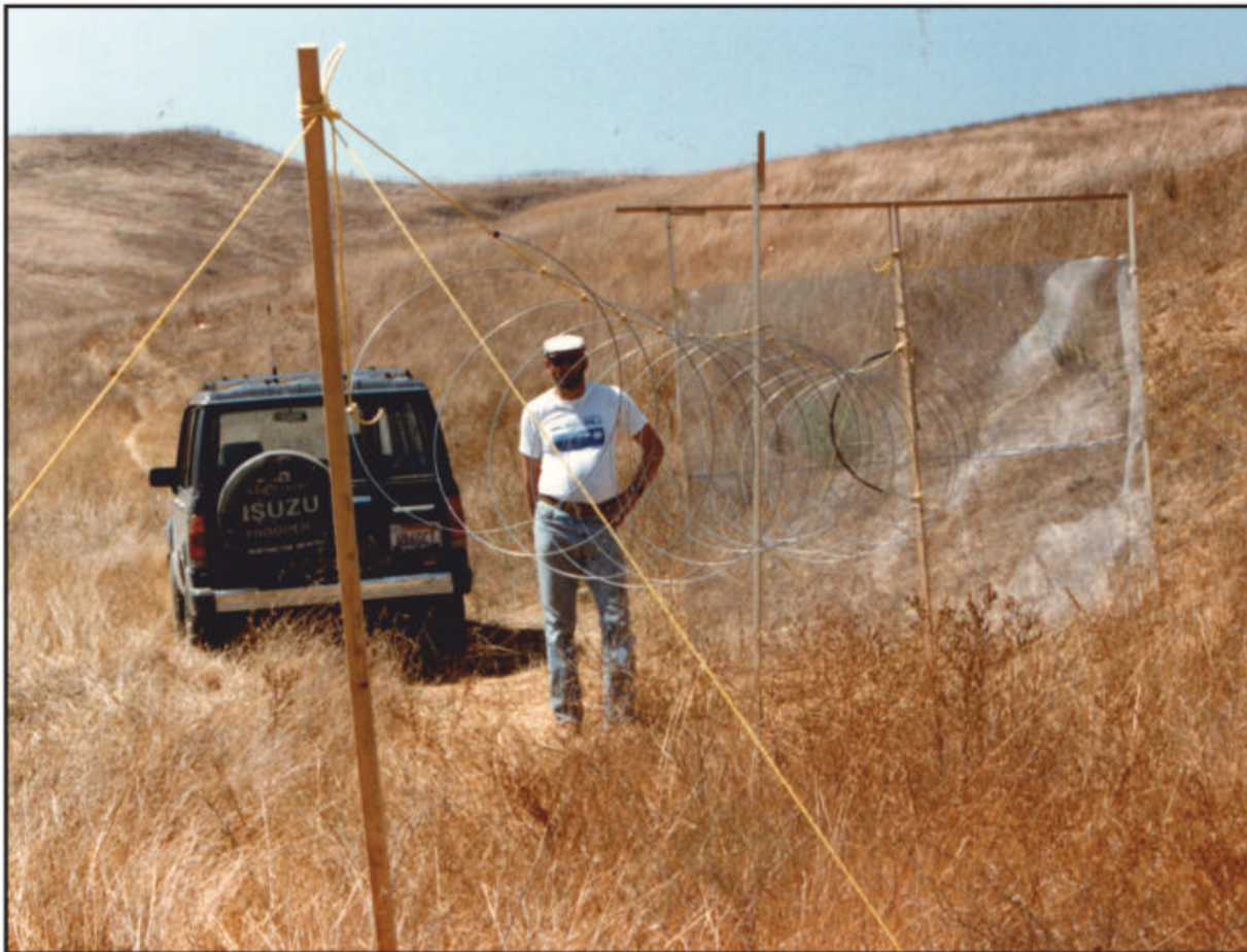
Photo B. Gary Holoubek, WB6GCT (pictured), and Tony Levand, now AA9CC, assembled this 16-foot-long circularly polarized beam with 6- x 6-foot screen reflector in a wilderness park for a Fullerton Radio Club mobile T-hunt. It shot lots of signal down the canyon, where it was several miles to the closest road. But it gave very little signal to the rear, where the approaching road came within a hundred yards. (Photo by Joe Moell, KØOV)
