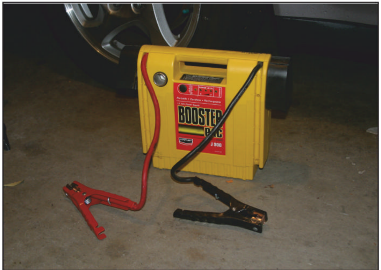
Photo B. A booster battery like this can be used to power a mobile rig temporarily as you make tests and adjustments. Do not touch the positive cable to any electrical ground!
