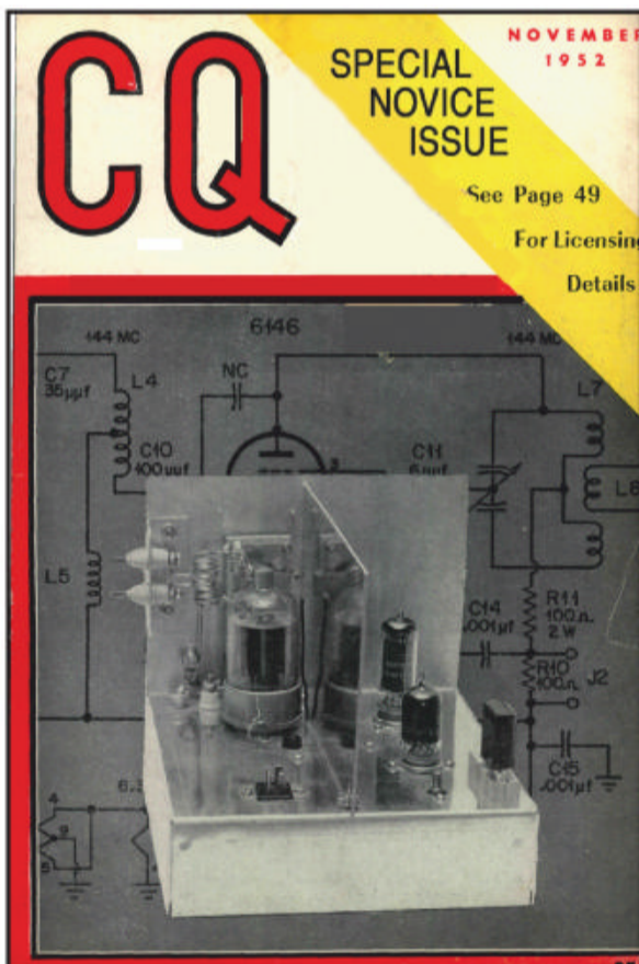
Photo A. The November 1952 issue of CQ was a "Special Novice Issue" featuring a 2-meter transmitter built around a 6146 final amplifier tube. The original Novice license included voice privileges on 2 meters.
