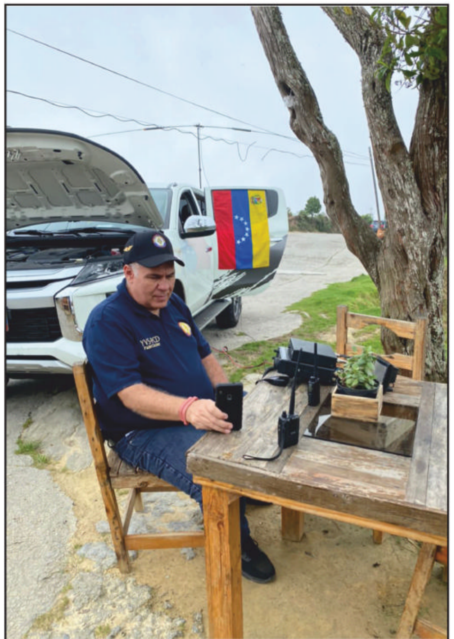
The HF portion of the portable station, getting power from the truck battery. The weather had improved by the time this photo was taken!
