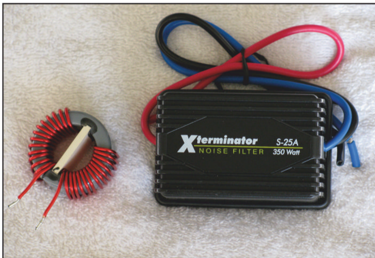
Photo D. Left: A toroid choke found in my junk box. Right: A store-bought DC line filter.
