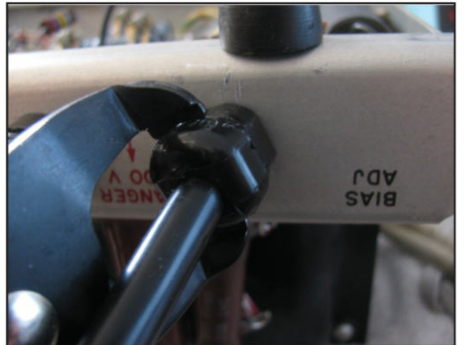
Photo J. The special grommet tool securely grips the grommet.
