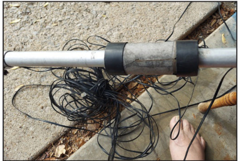
Photo B. A trap element appears to be nothing more than a can inserted between two aluminum poles. (Photos B-E by KOØZ)
