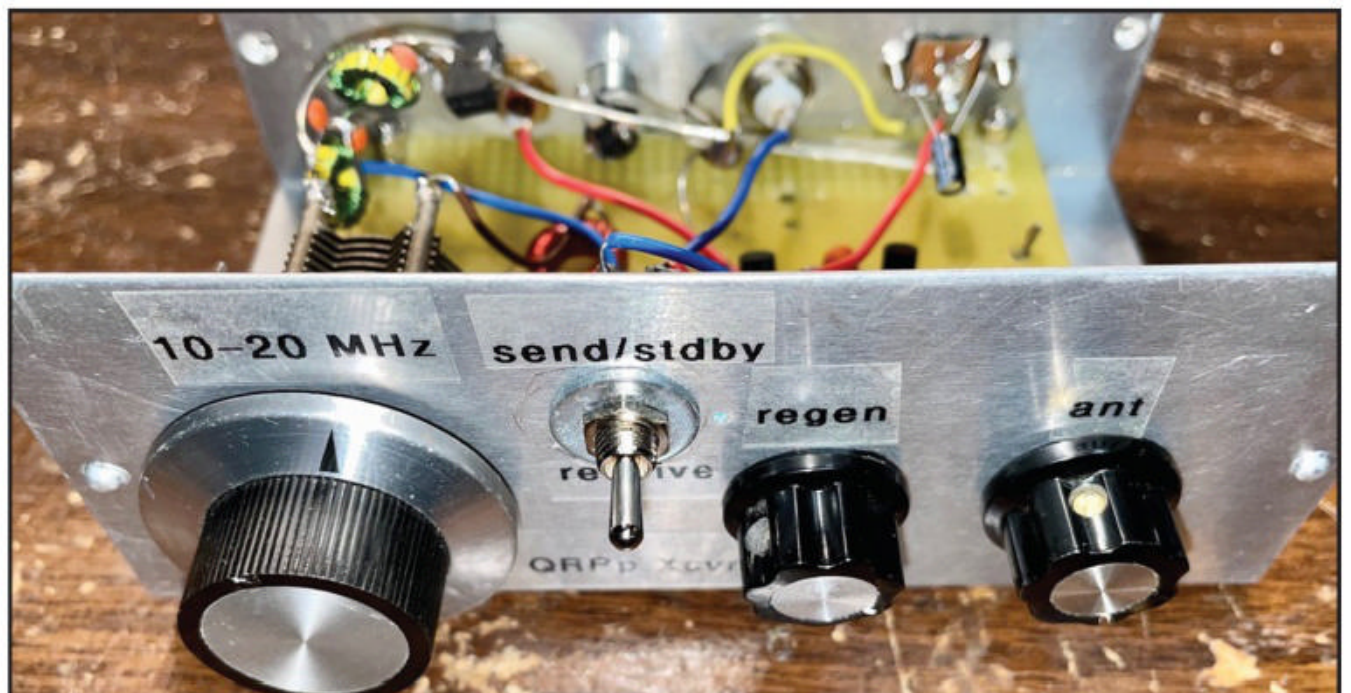
Photo G. A regenerative receiver circuit found on the internet provided the receive side of the author's original plant-powered station.
