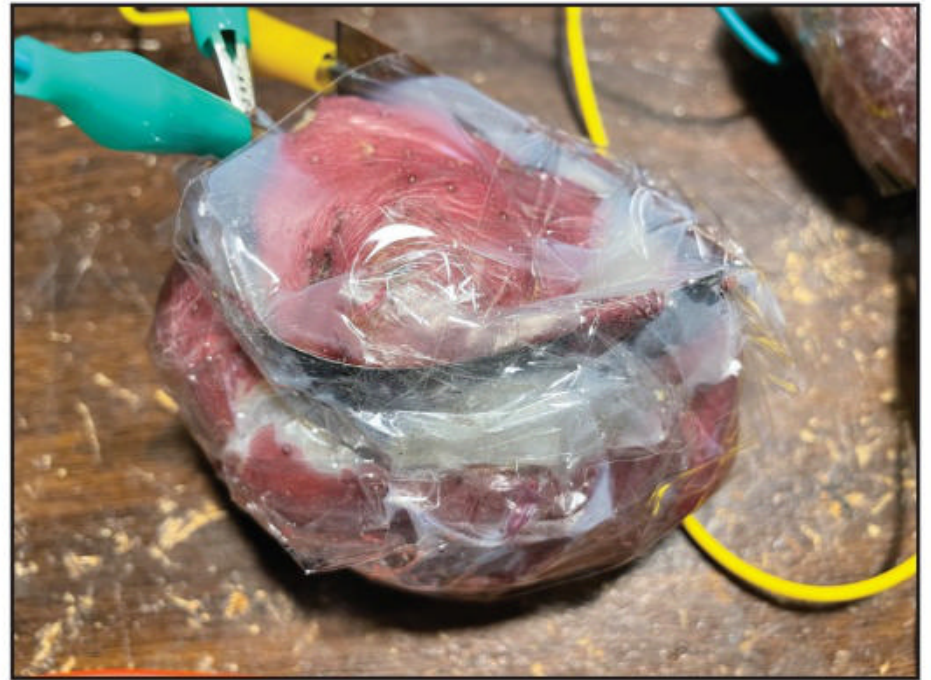
Photo C. The potato batteries were wrapped tightly in plastic tape, with the electrodes curved around them for maximum contact area.
