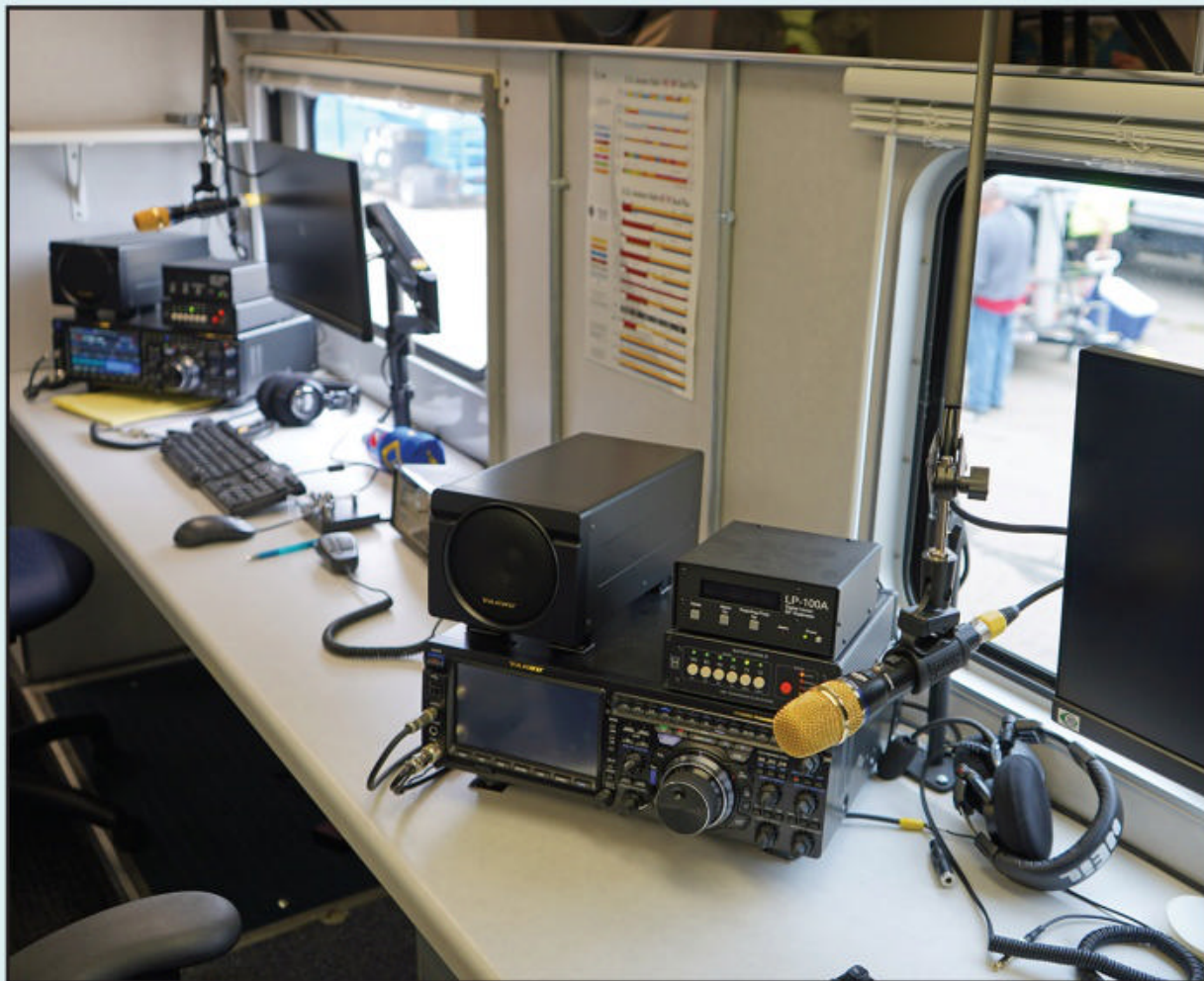
The MVRA bus is equipped with three operating positions that feature Yaesu FTDX101D radios, as well as other operating positions.
