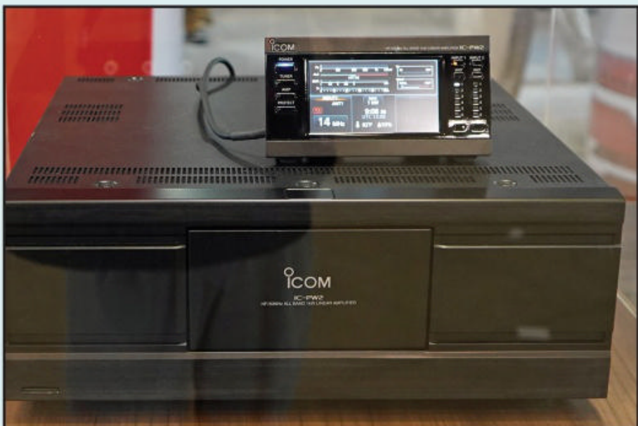
Icom's new IC-PW2 1-kilowatt, solid-state amplifier was on display. This amp will output 500 watts at 120-volts AC and 1 kilowatt at 220-volts AC power input. The amplifier does not have to take up any desktop space, being completely controlled either via your network or the removable touch-screen control panel. SO2R capability is also built in.
