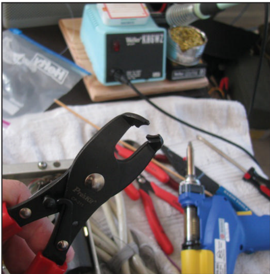
Photo H. The special tool makes removing and installing plastic strain-relief grommets safe, fast, and easy.
