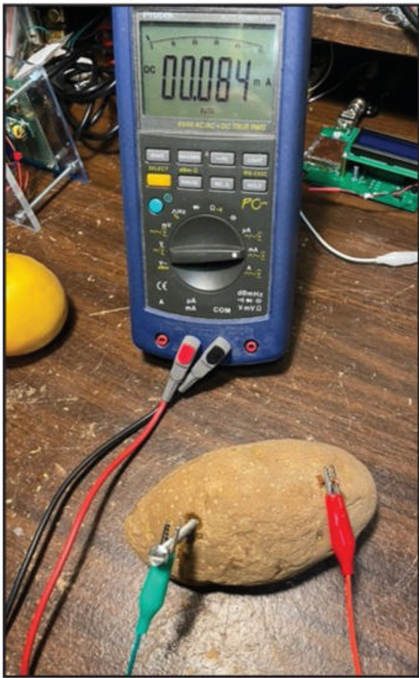
Photo B. In the initial experiment, a copper penny and a zinc-plated nail were used as the electrodes in a single raw potato. I could only get 0.084 mA of current.
