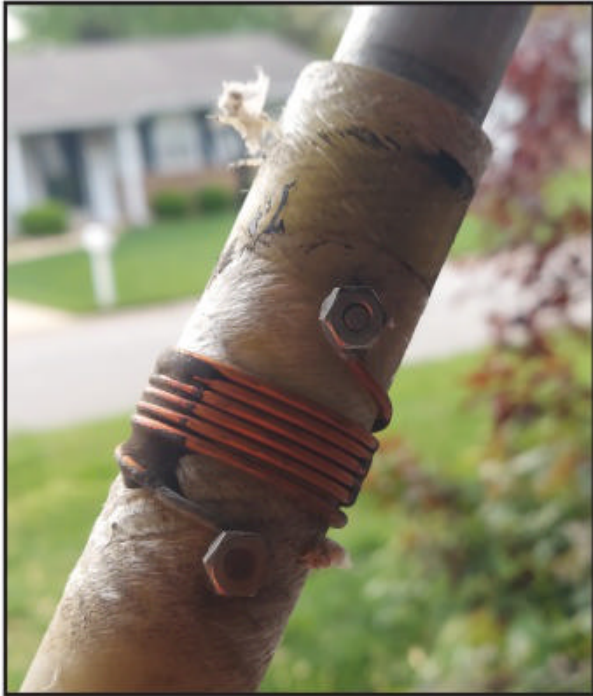
Photo C. Upon closer inspection by removing the outer metal housing (trap capacitor), an RF coil is wound on an insulator that is connected to each aluminum element.
