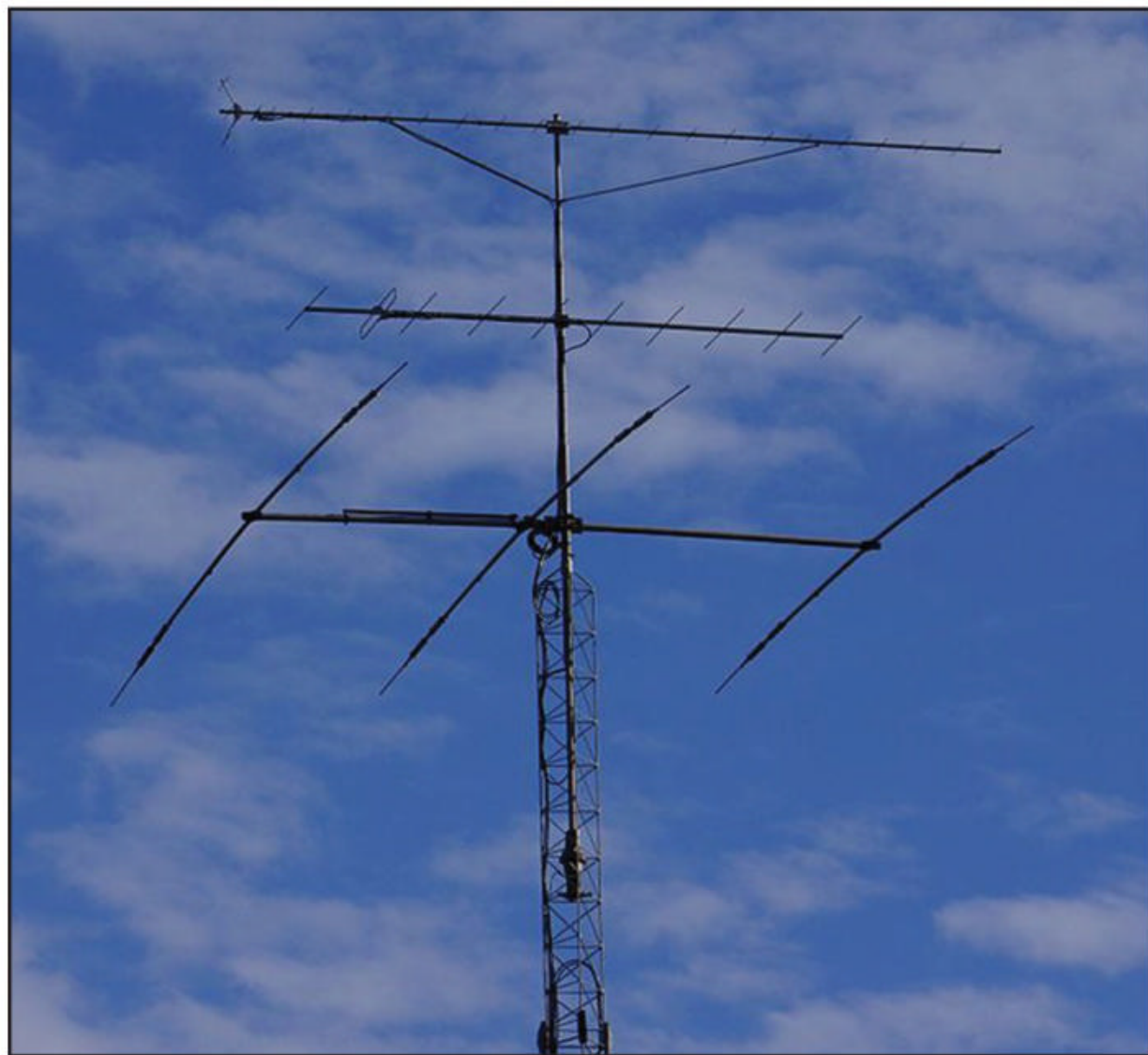
Photo A. A multi-band Yagi antenna. Note the traps in each element of the Yagi. (Courtesy of Wikimedia Commons)
