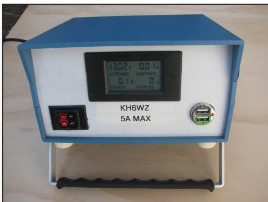
Photo N. The completed unit features a multi-function digital meter, Anderson PowerPole®, and USB output ports.
