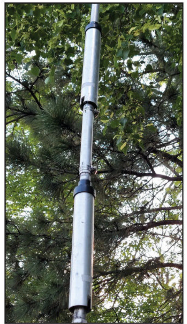
Photo E. A close up of a 14 AVQ (10-40 meter) vertical antenna trap.
