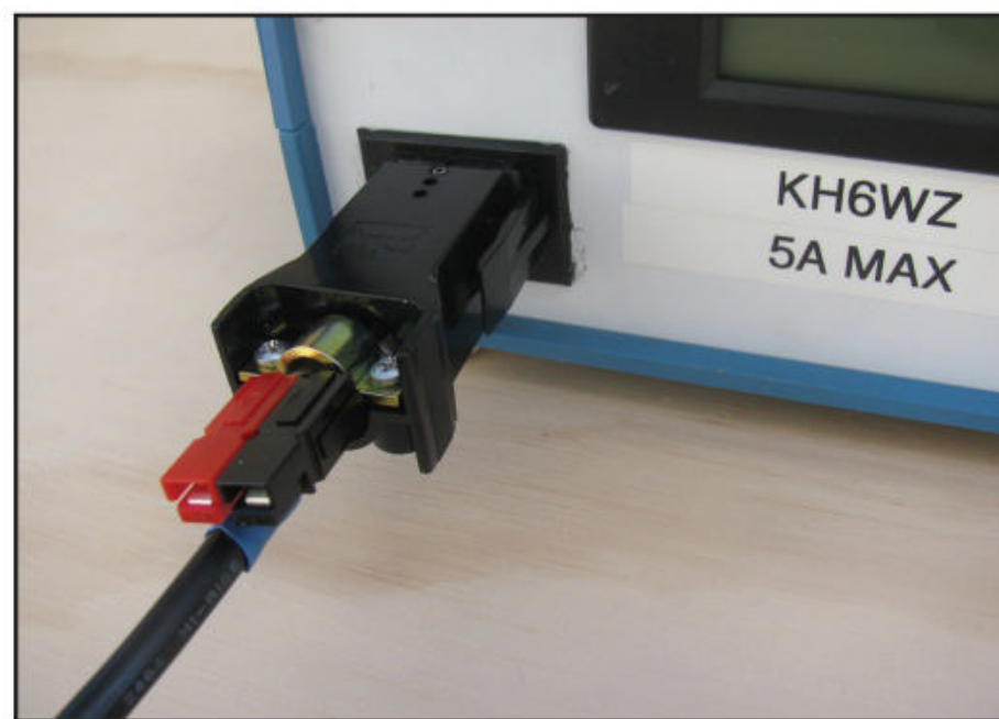
Photo O. The 12-volt output mates with the cable-mounted locking housing. An extra pair can mate with other accessories near the power supply if needed.
