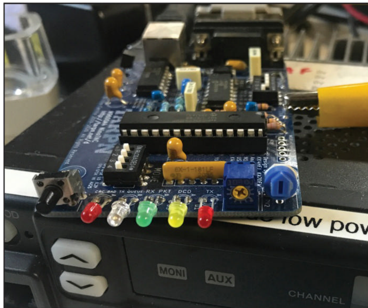
Photo D. Receive testing the Kenwood TK-762G with a NinoTNC. TXA and RXA test points on the NinoTNC, along with transmit test modes, make it easier to adjust the transmit audio level for best performance.
