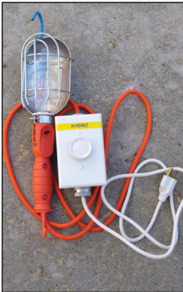
Photo L. Useful for Field Day at night: A dimmable red light for nighttime use.
