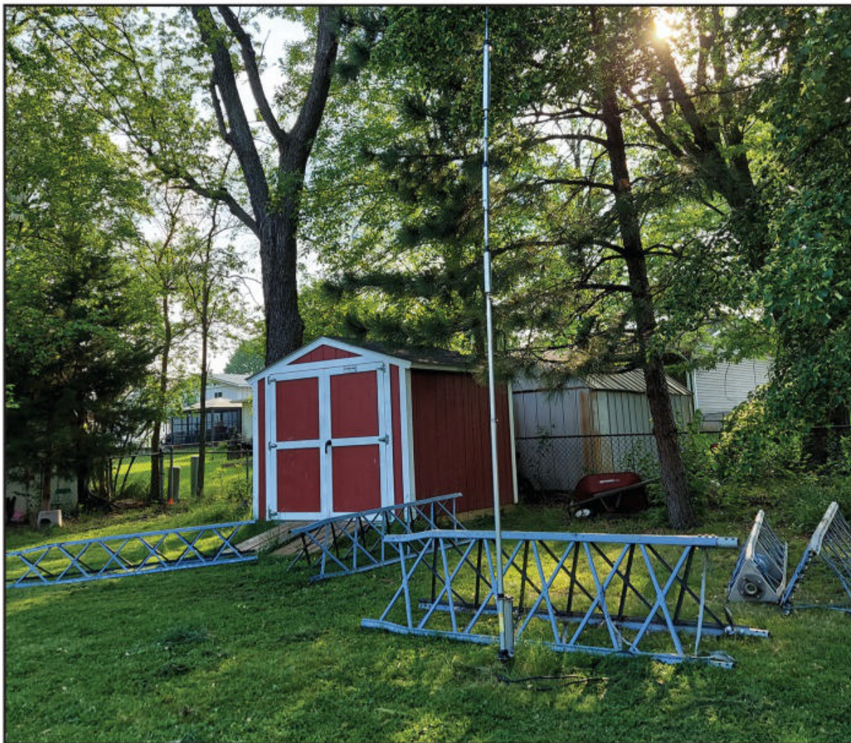
Photo D. Hy-Gain's 14 AVQ, 10-40 meters is a low maintenance, relatively low profile, efficient HF antenna.
