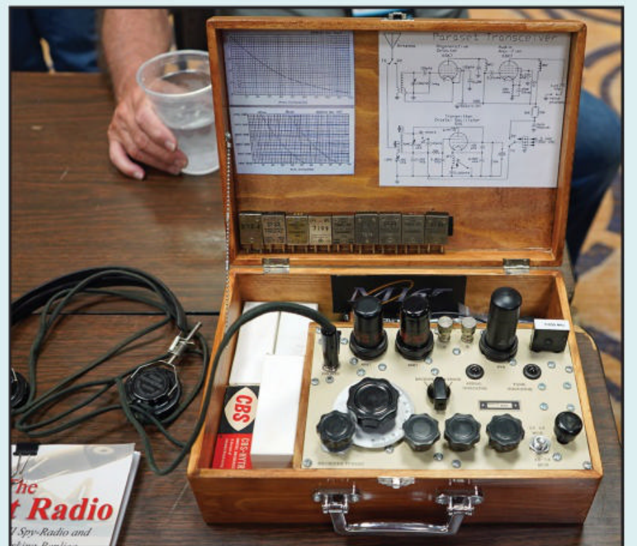
The best homebrew award at FDIM went to Gary Auchard, W0MNA, with his incredible tube-type World War II replica Paraset radio.
