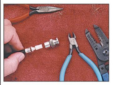
Photo 15. After soldering and checking for shorts, slide the shell onto the assembly. Hold the cable and connector body still with a wrench while you turn the locknut. Try not to twist the connector body, since that may twist
