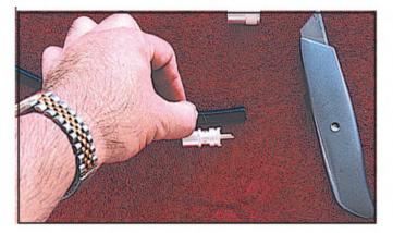
Photo 3. No need to measure. My thumb indicates where the outer jacket needs to be removed. Notice that the length of cable is slightly longer than the connector length, as indicated by the center pin.
