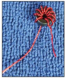
The last toroid to be mounted is a trifilar type, which requires three wires to be twisted together. The leads are then separated out, stripped, cleaned, and tested to get three parallel pairs of leads to be mounted. Be sure to do the continuity tests exactly as instructed for this vital toroid to work properly.
