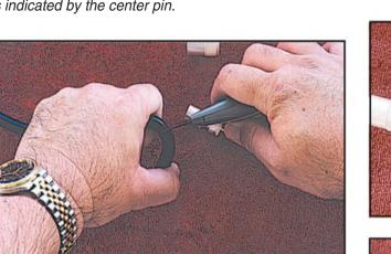
Photo 4. Carefully remove a section of the outer jacket. See text for a neat technique to prevent nicking the braid.
