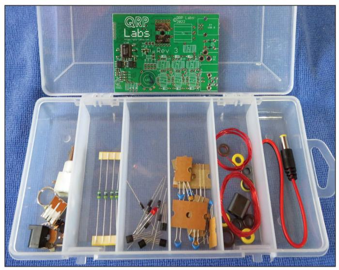
The QDX 4-band digital transceiver parts ready to assemble. Notice the low parts count, due to all the surface-mount parts already being mounted.
