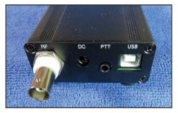
The rear of the finished QDX transceiver.
