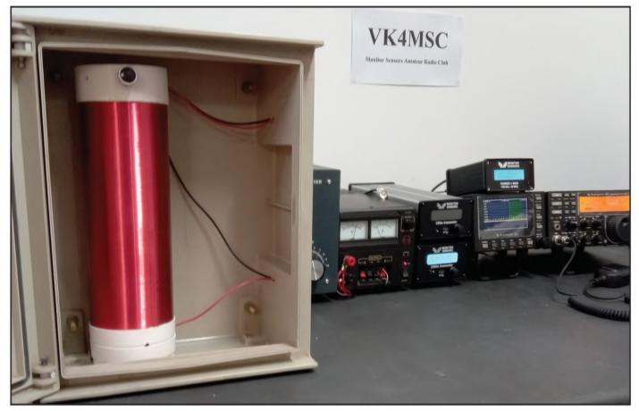
Photo D. The 8.2-milliHenry, 2200-meter loading coil for the Hustler vertical atop the VK4MSC Monitor Sensors Amateur Radio Club station.
