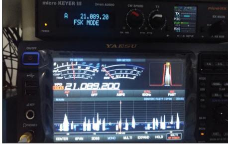
Photo C. MicroHam MKIII RTTY interface, in FSK mode. (PY2XV photo)
