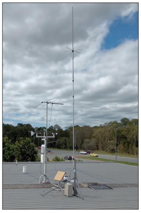
Photo C. Here is the business-end of the Hustler vertical that was adapted to 2200 meters by Roger Croft, VK4YB. The high-inductance loading coil is secured in the sealed box under the mounting bracket while the antenna is fed against a small radial field and the metal roof of the building.
