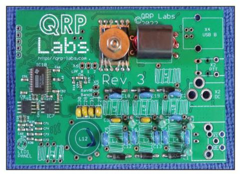
The through-hole parts are mounted and one of the toroids, T1 is mounted. I used the 3:2 ratio winding option for lower power output when running up to 12 volts to prevent damage to the output transistors.
