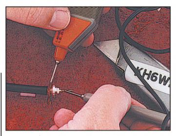
Photo 14. Check for short circuits between the center pin and shield as you assemble any connector.
