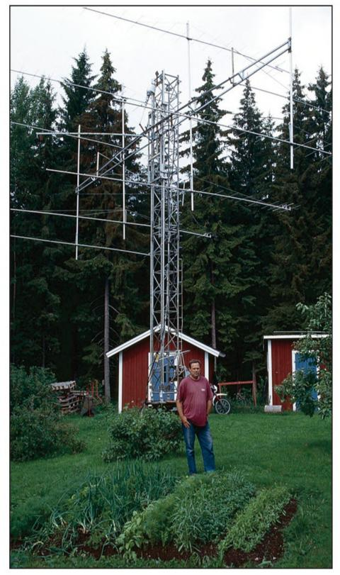
Photo A. I didn't have a photo handy of a 6-meter EME (earth-moon-earth) station, but Sverker Hedberg, SM3PWM's, 2-meter EME station gives a good idea of the resources and coax needed to build a good, EME station. EME is the ultimate satellite QSO. (Courtesy of Wikimedia Commons)
