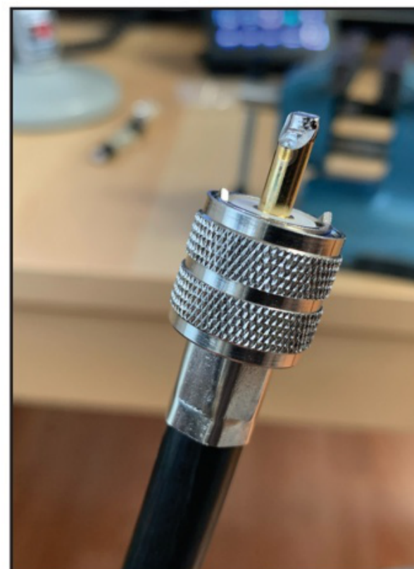
Photo F. A crimp-type PL-259 properly installed on LMR400 coax. A length of weatherproof heat shrink tubing over the crimp and outer jacket will be added as a finishing touch.
