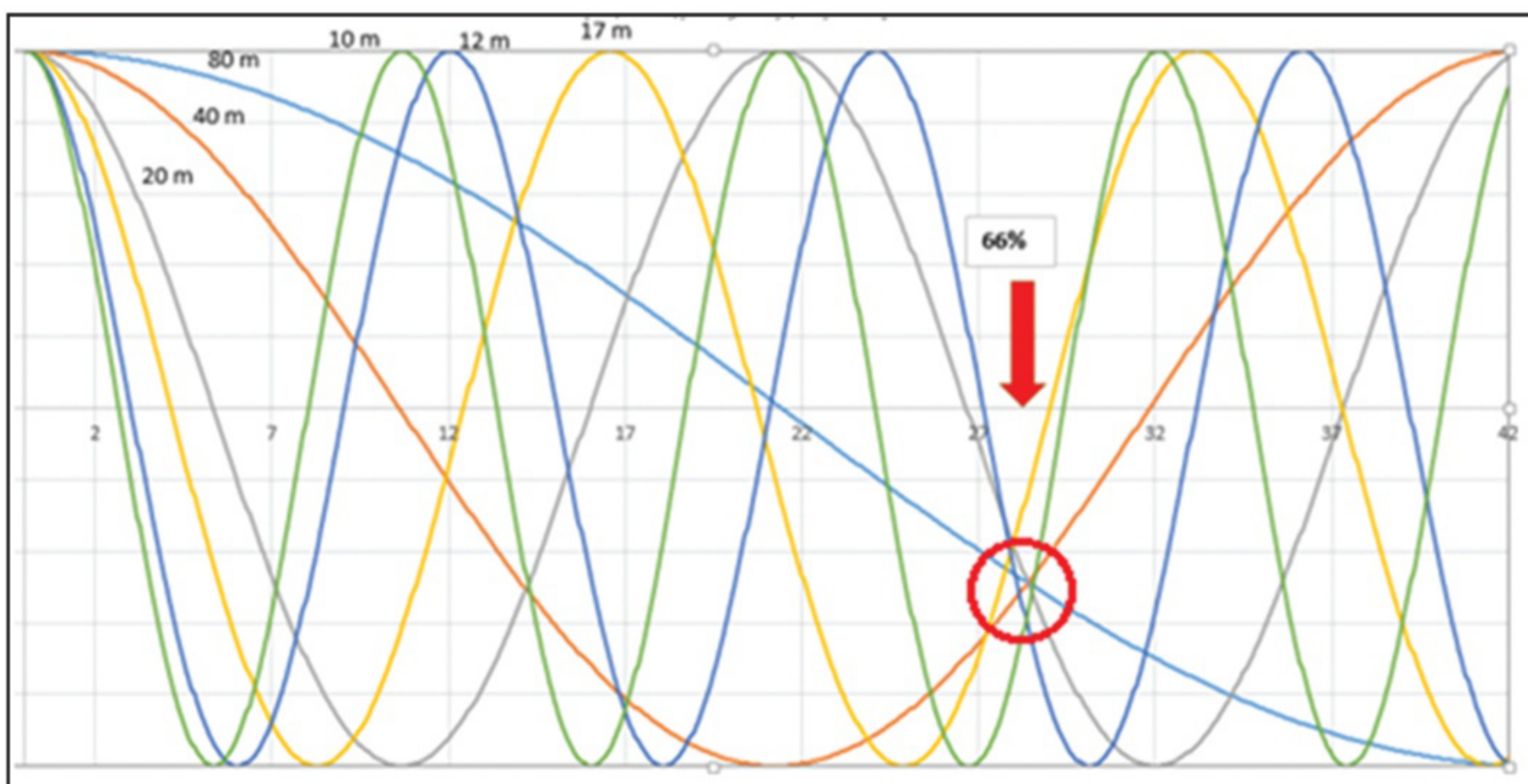
Figure 1. Windom wave distribution for amateur HF band signals on six HF bands. Note the convergence at 66% of the 80-meter length.
