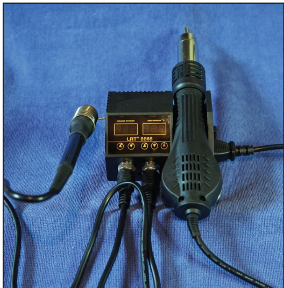
Both tools have cradles for safe storage. In addition, cradling the heat tool triggers an automatic cooldown mode. Setting the soldering iron for 300° C and the heat tool for 400° C seems to work well.
