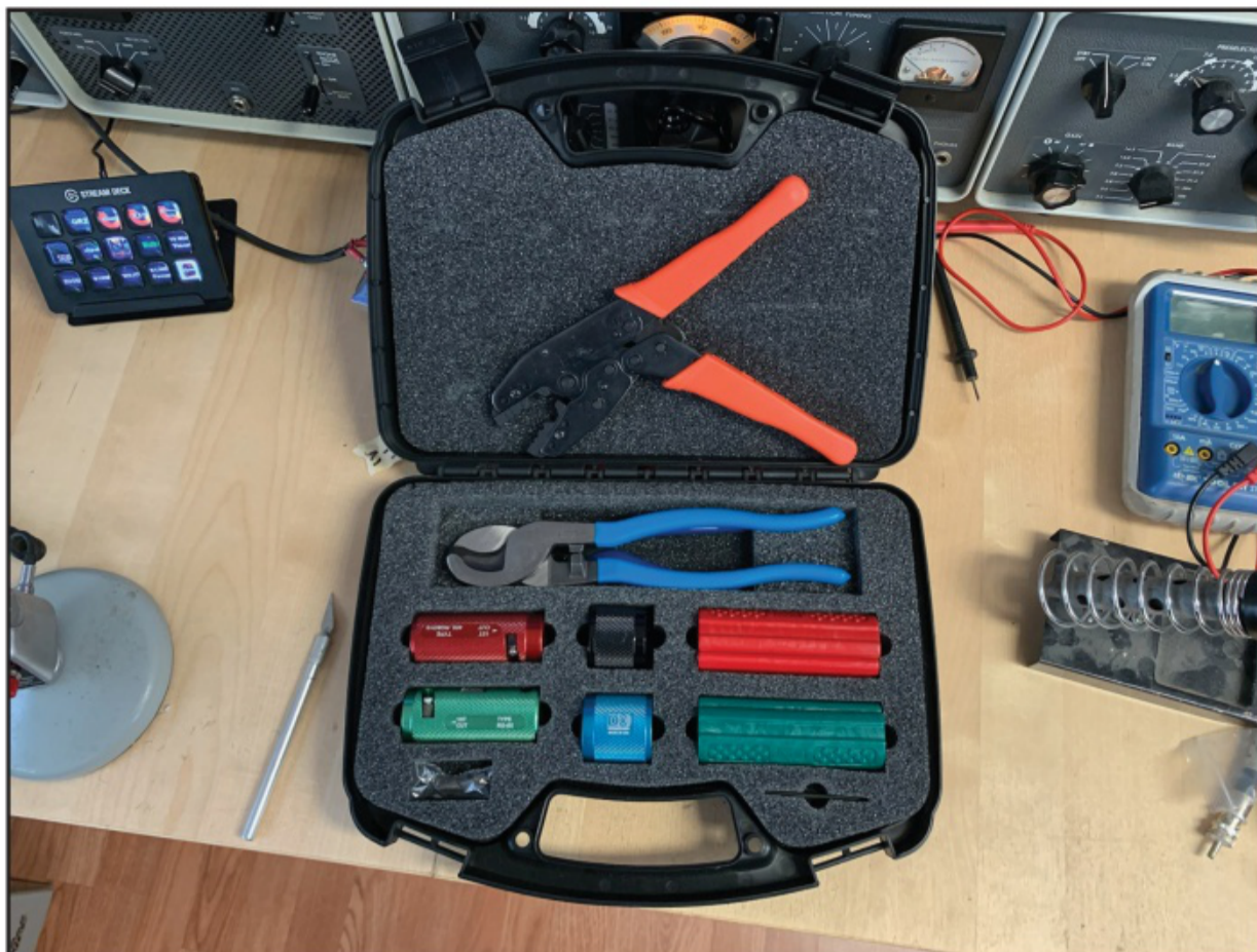
Photo E. A crimping tool kit for crimp-type coaxial connectors. The ratchet and die are the critical tools.
