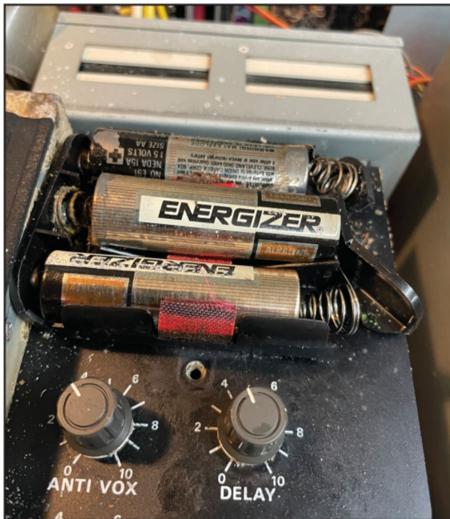
Photo B. A little-known internal battery holder made a mess of the 930 prior to restoration.
