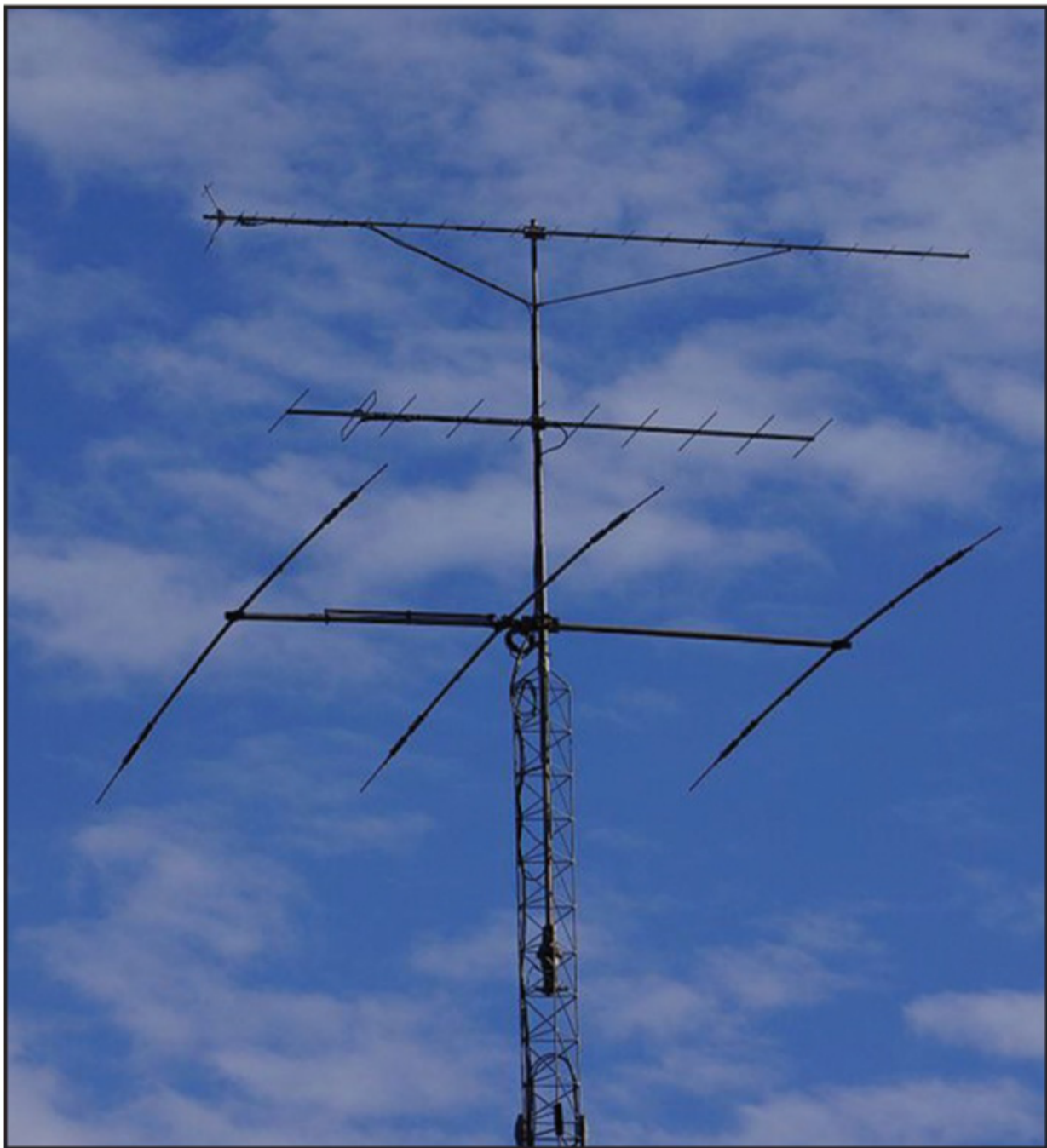
Photo A. The Yagi is a popular directional antenna. Rotor motors are used to move directional antennas. (Photos courtesy of Wikimedia Commons, except as noted)
