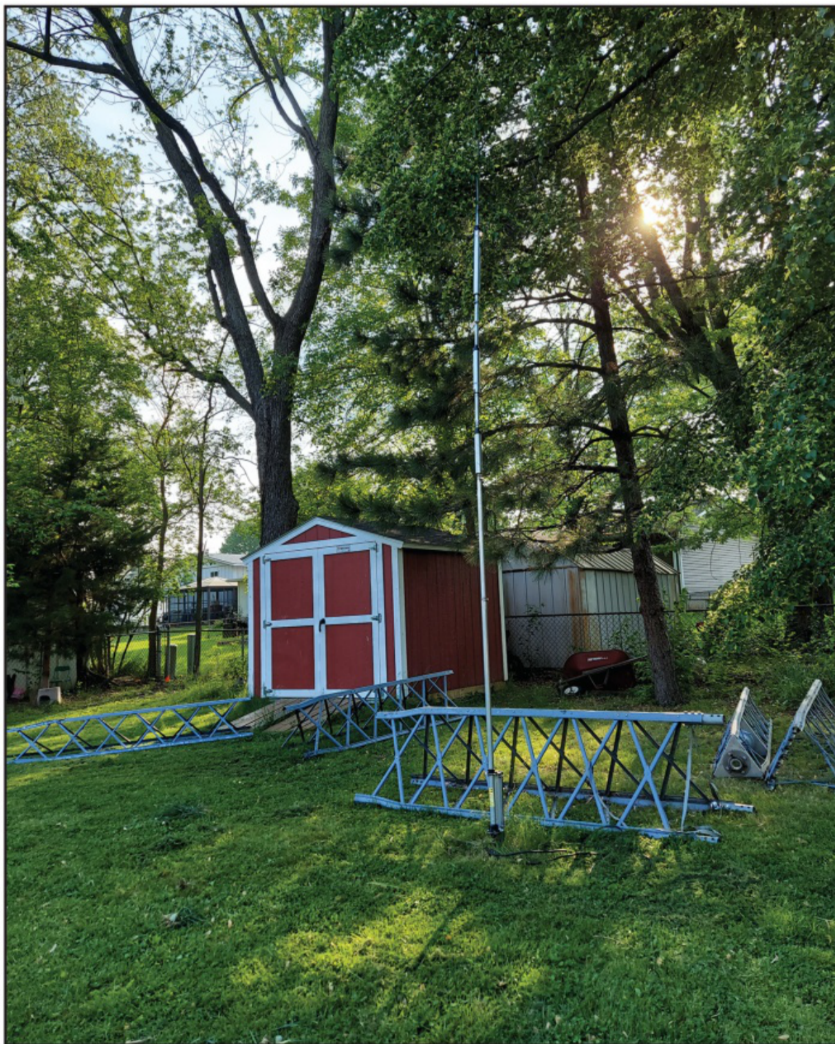
Photo C. A vertical antenna is omnidirectional. It can transmit and receive in all directions. (Photo by KOØZ)
