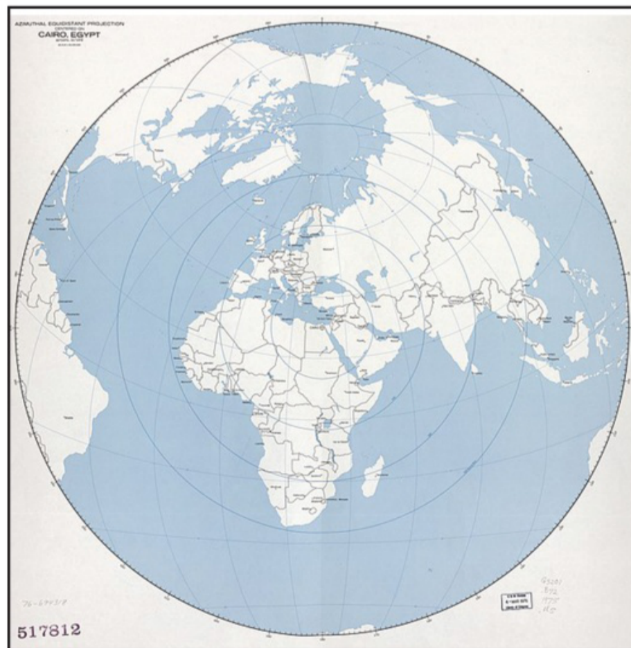
Photo E. Azimuthal (great circle) maps are ideal for showing true bearings from a central spot. This map is very useful for hams using directional HF antennas.
