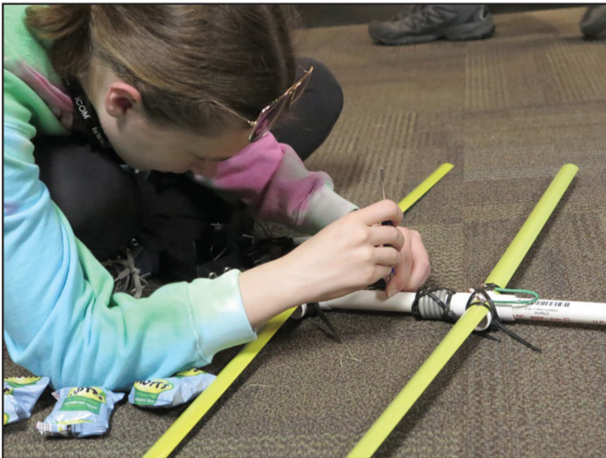
A YOTA camp participant works on her 2-meter measuring-tape Yagi antenna for foxhunting.
