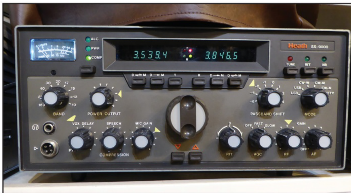
Photo B. The remake of the SS-8000 ... the Heath (not a kit) SS-9000 9-band synthesized transceiver, including 30, 17, and 12 meters. Only 350 were built. All were fully assembled and tested at the Heathkit factory in Benton Harbor, Michigan.
