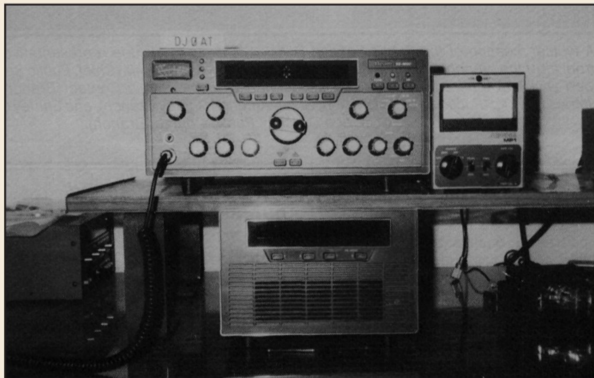
The SS-9000 on the operating table with the PS-9000 power supply below it.
