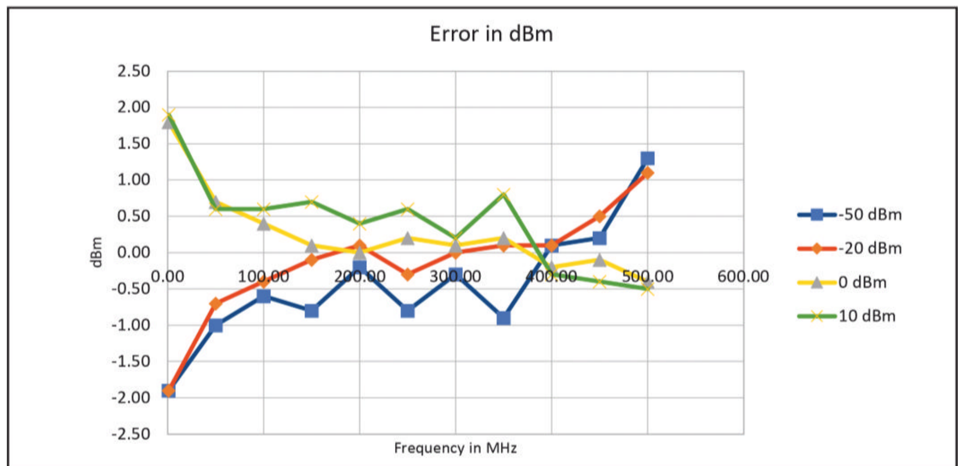
Figure 1. Measurement and error data from Tables 2 and 3 presented in graphical format. This particular meter is most accurate at VHF and low UHF frequencies.
