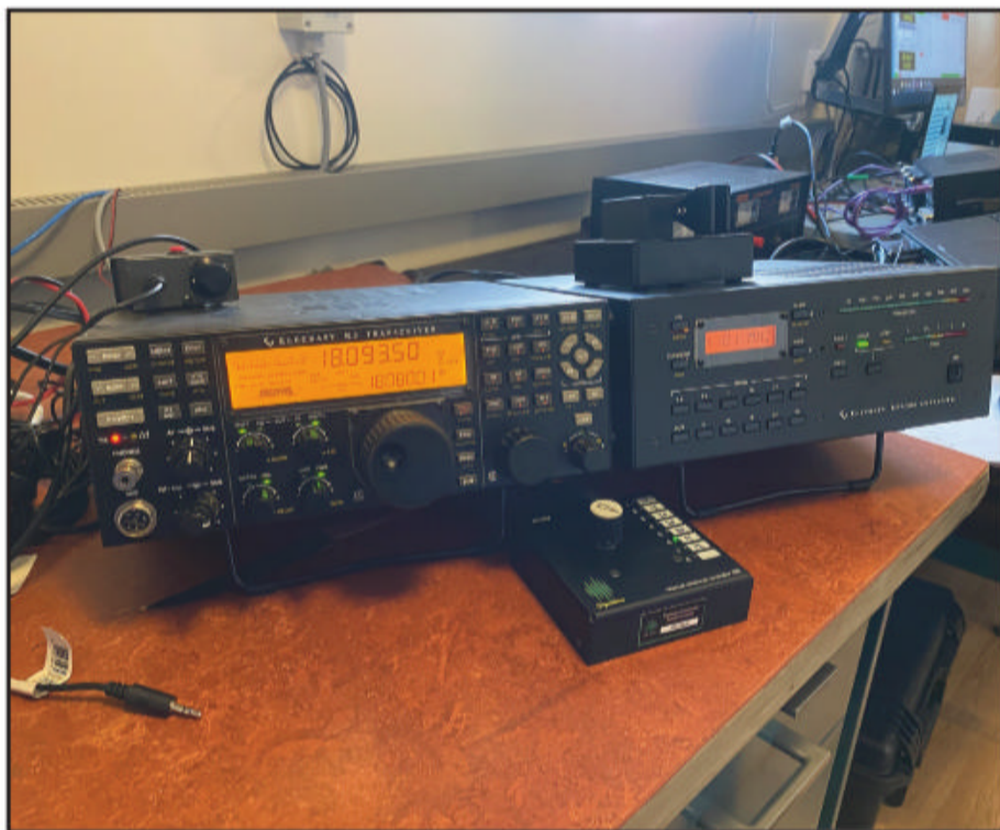
Photo D. Team members brought their own rigs – Elecraft K3s transceivers and KPA500 amplifiers.
