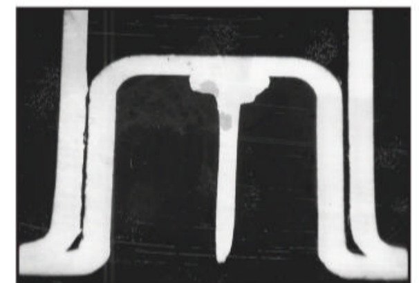
Photo D. The most reliable construction method used metallurgical "nail head" weld to the header.
