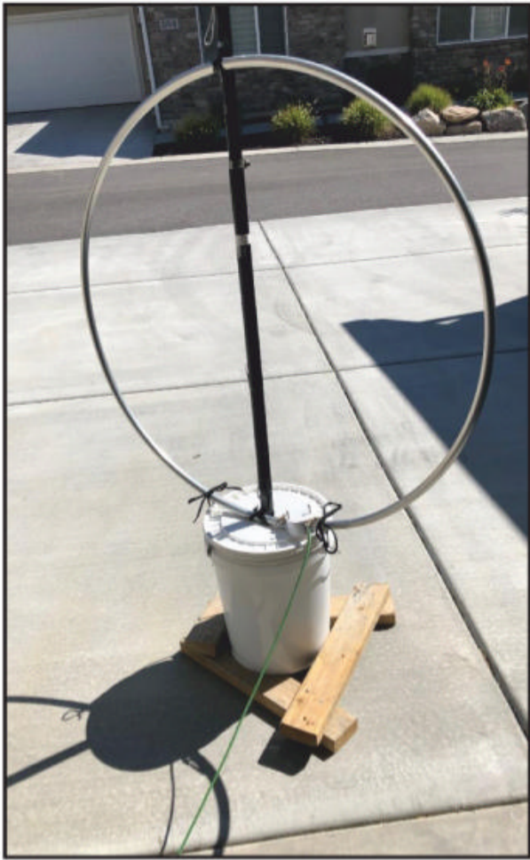
Here is WØYSE/7's Wellbrook loop sitting in the driveway of his home in a covenant-restricted neighborhood. Reports are that he has brought this loop into the garage alongside the transmitting loop and following some work on the preamp after initial testing. It seems to be hearing pretty well. (Courtesy of WØYSE)
