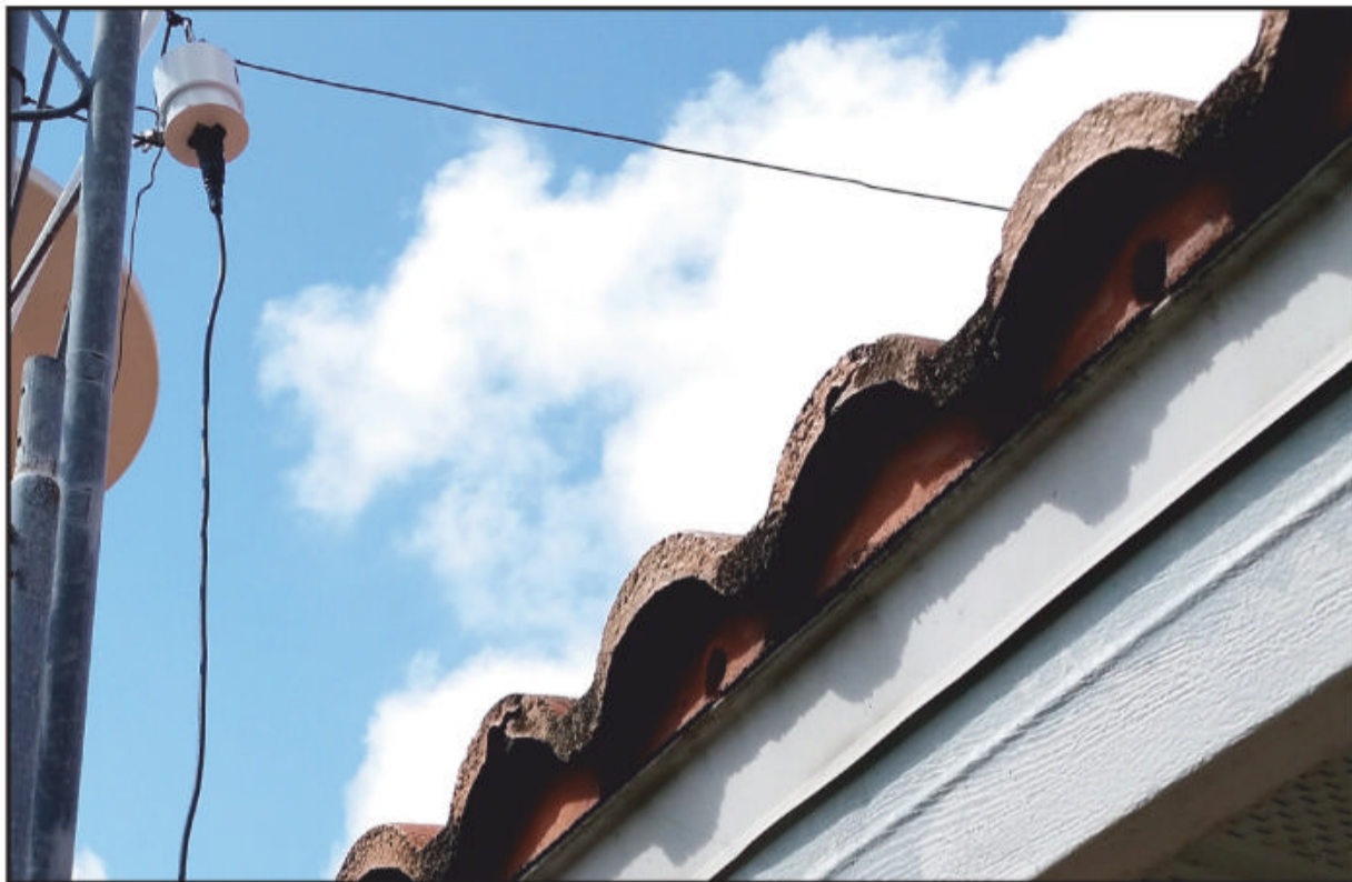
Photo D. The 9:1 unun is attached to my tower with Dacron® rope and the wire lies on the roof.
