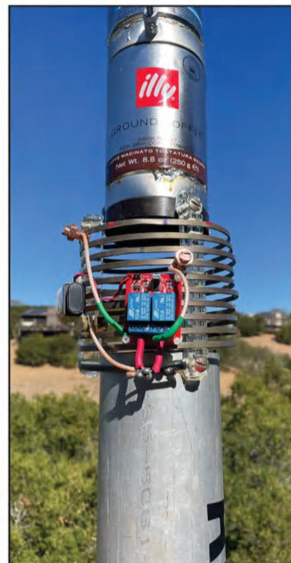
Photo I. The coil is center-mounted between the pole below and the coffee cans above. Retuning may be done by adding or removing coffee cans as well as changing taps on the coil.
