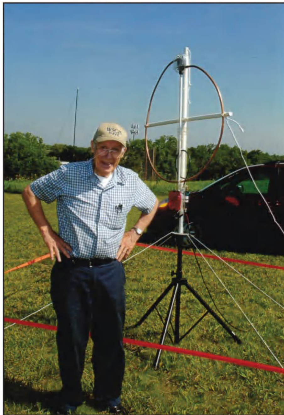
Photo A. The author at Field Day with his 100-watt magnetic loop (mag-loop) antenna, tuned with a motor-driven vacuum-variable capacitor. (Photos courtesy of the author)
