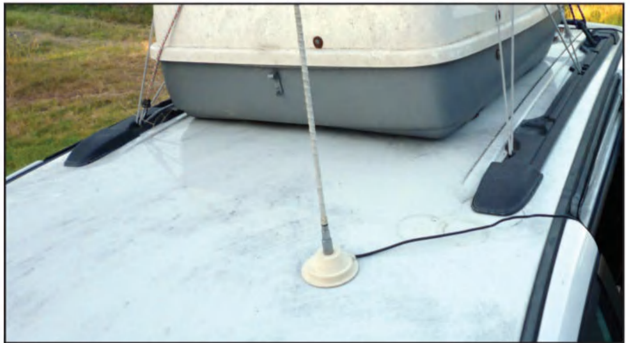
Photo B. A quarter-wave vertical over a ground plane.
