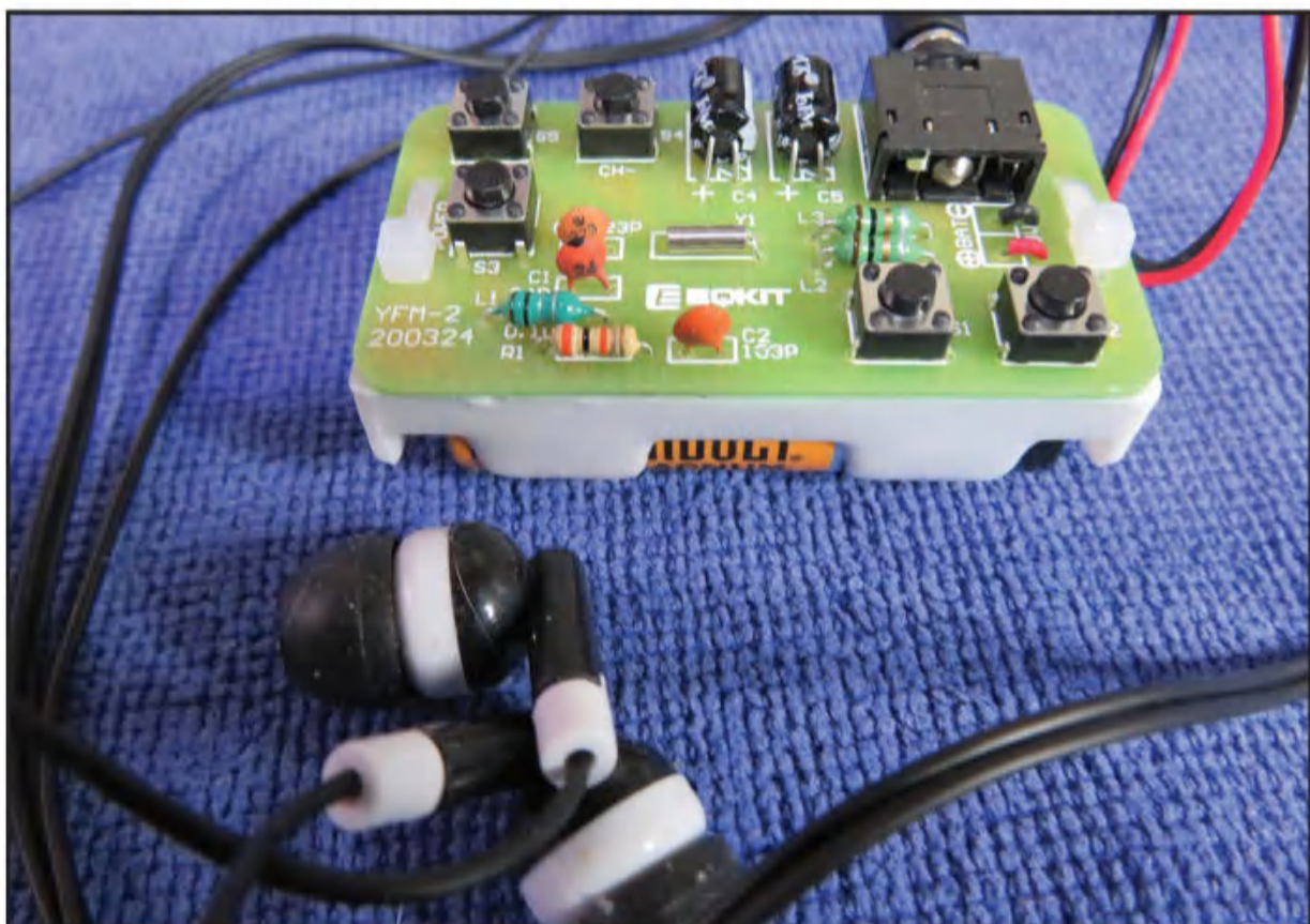
The finished FM stereo radio kit is completed and attached to the battery pack with the supplied zip ties. Ready to rock and roll!
