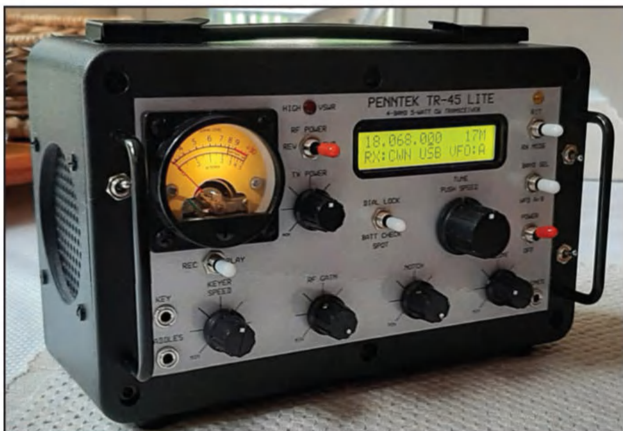
Photo C. WA3RNC’s TR-45L, a 5-band CW QRP transceiver offered in kit and built form. (Photo courtesy of <wa3rnc.com>)
