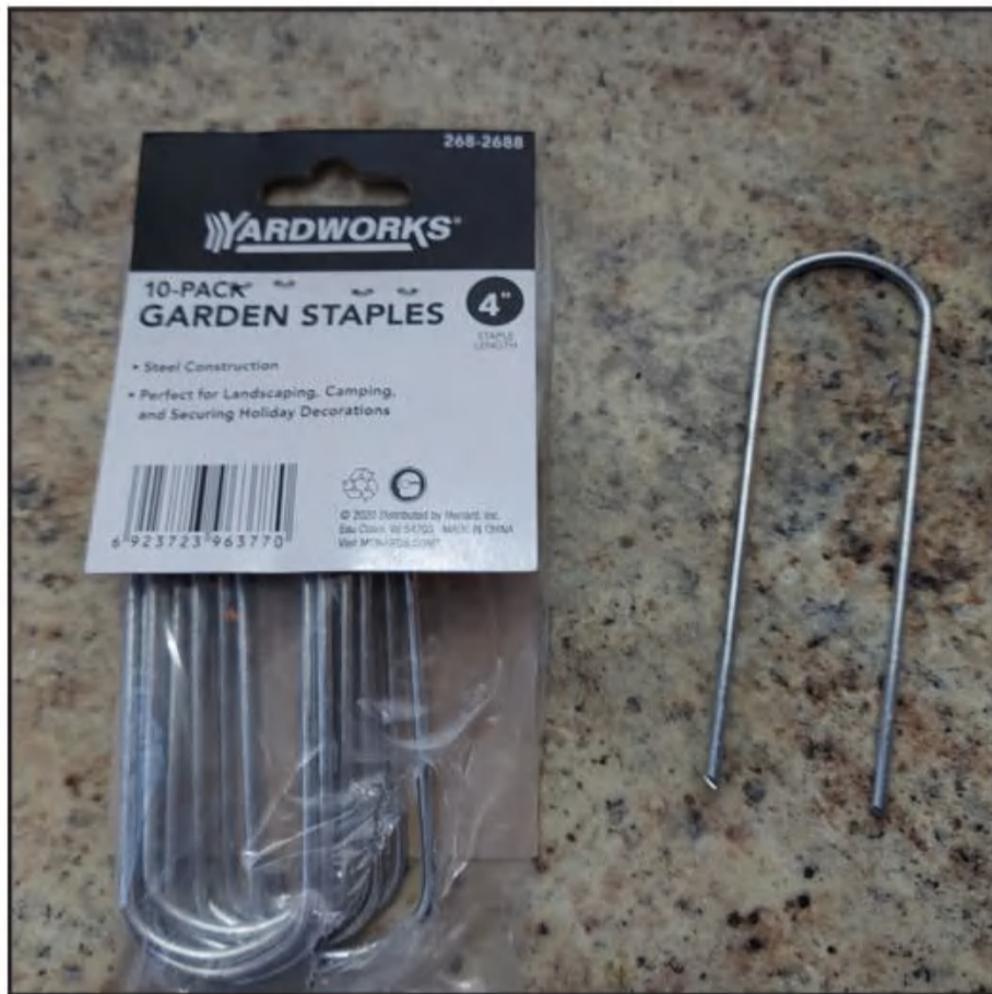
Photo A. Most hardware stores carry garden staples or yard staples in their garden department. They are about 4 inches long and they are easy to drive into the ground. They will hold a ground radial snugly to the yard. No need to bury the radial. In a few weeks, the lawn will grow over the radial and it will be "safe" to mow the lawn.
