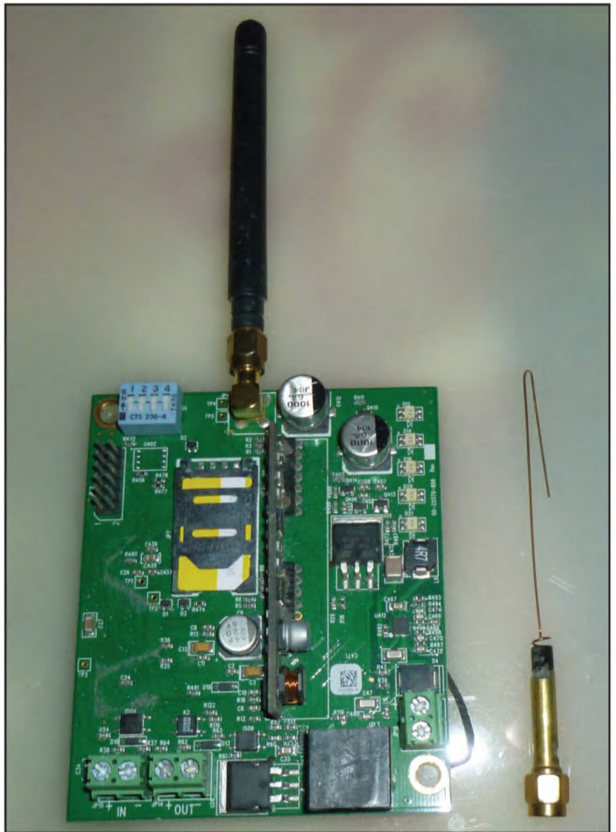
Photo D. An industrial cell phone, the type usually built into other devices.
