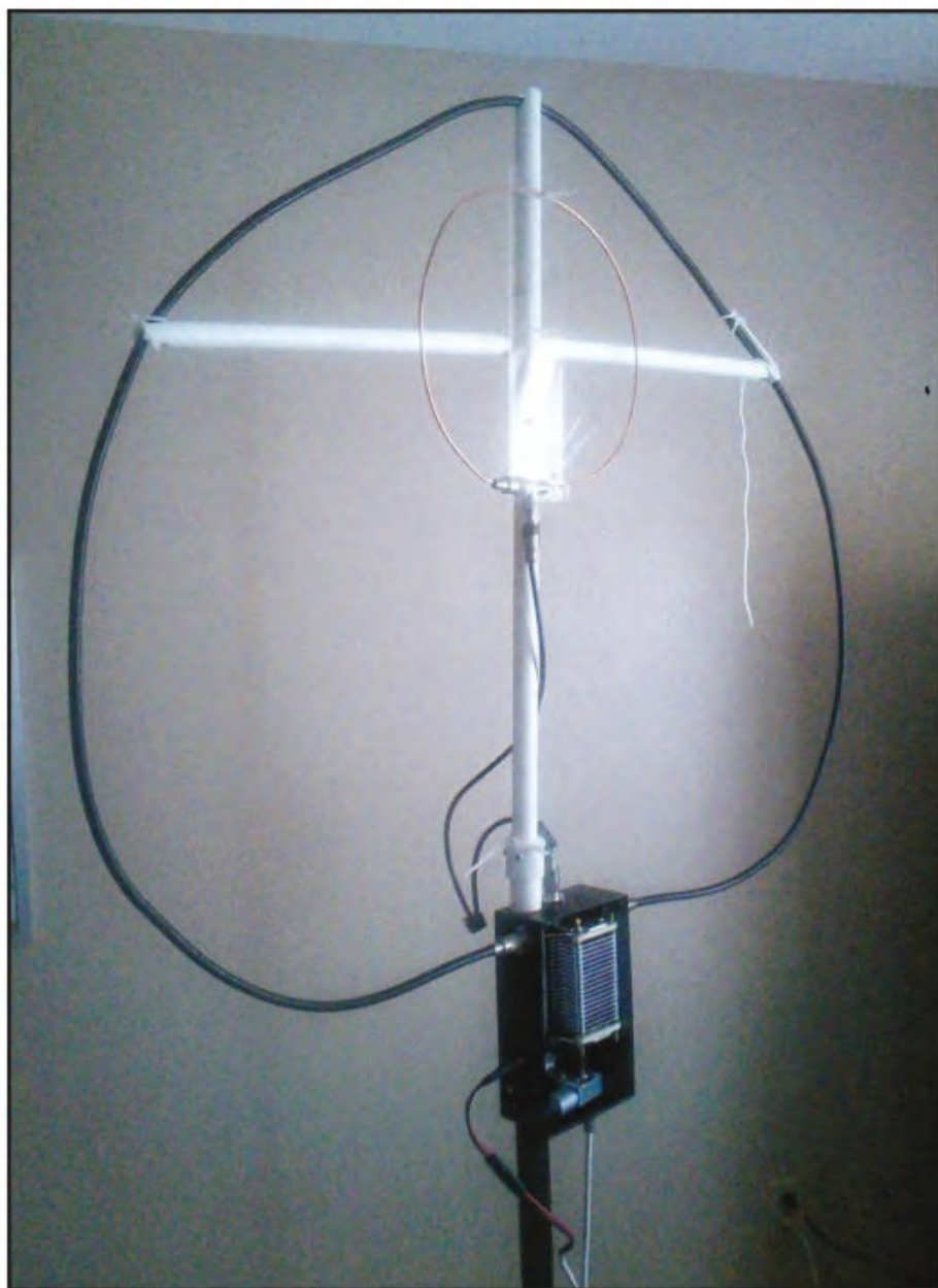
Photo F. The author's third mag-loop, using a motorized capacitor mounted inside the tuning box. The PVC tube segment is slid into the pole of a tripod.
