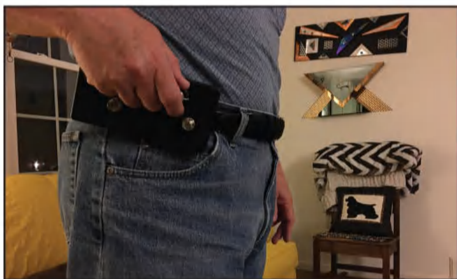
Photo B. Attenuator concept of operation. The unit is belt worn. Tuning is performed by rotating the potentiometer with one hand while holding the antenna in the other.
