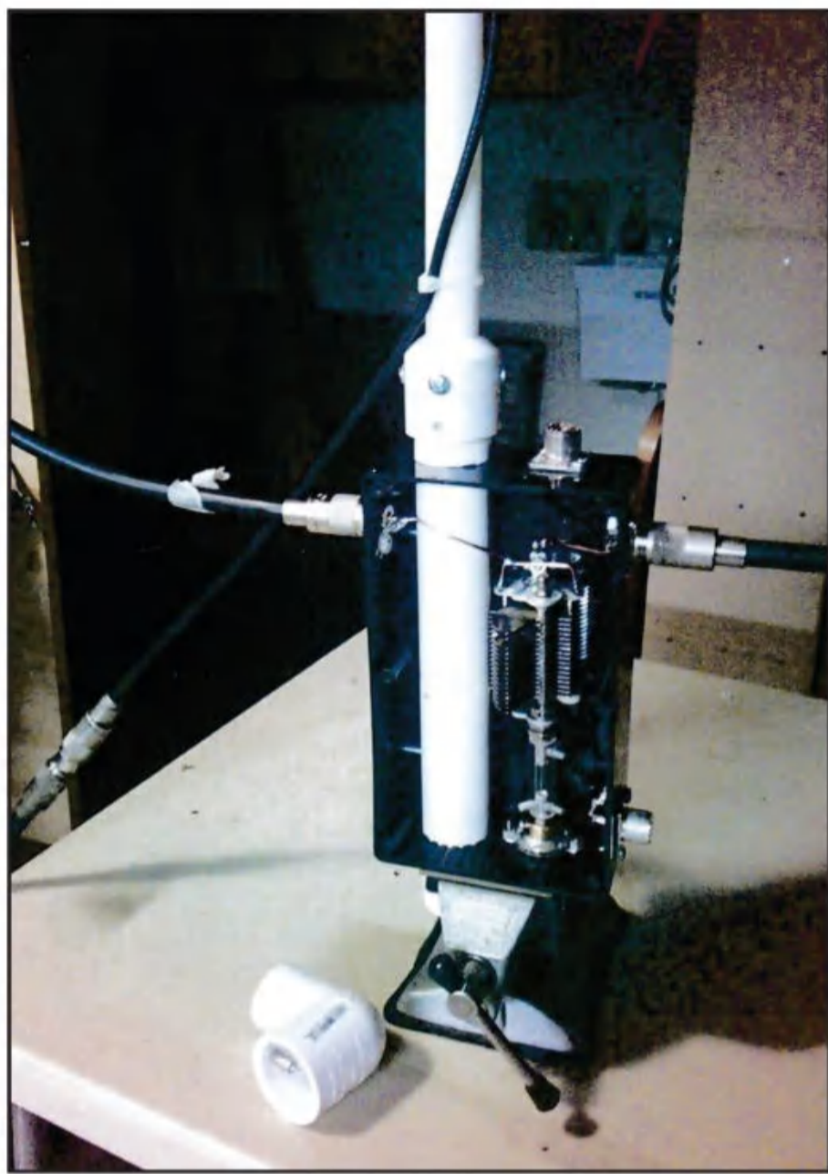
Photo C. This is the QRP mag-loop, seen here with the box in a vertical orientation. In this photo, it's held up by a small vise but would be mounted on a tripod in actual use.
