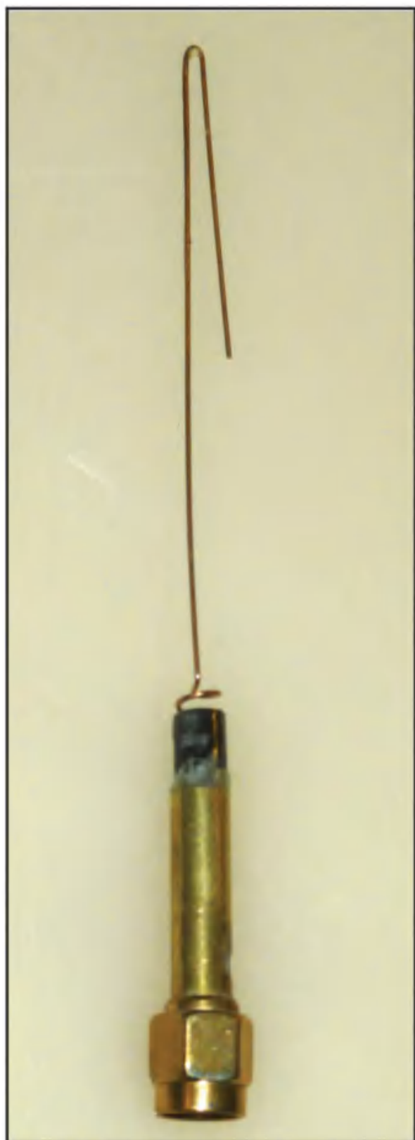
Photo E. Dual-band cell phone antenna. See text for details.
