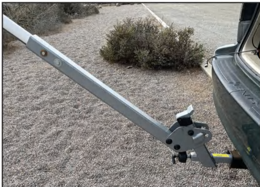
Photo G. The antenna support pole can tilt for easy attachment / detachment.
