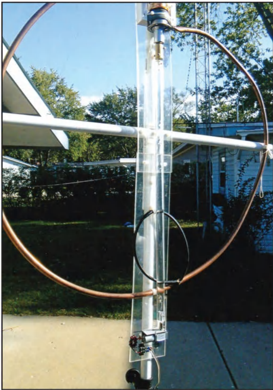
Photo B. Close-up of the 100-watt mag-loop construction. The vacuum-variable capacitor is at the top and the drive motor is at the bottom. The two are connected by a drive rod mounted on a sheet of Lucite.
