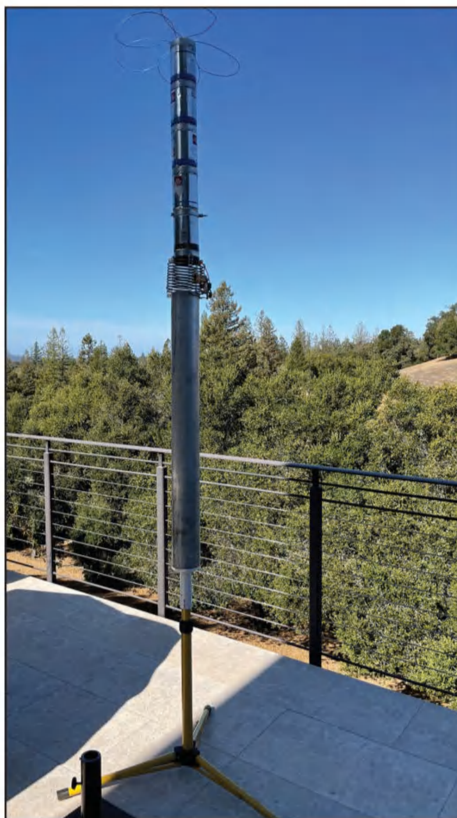
Photo H. The “Fat Man” can also stand on a tripod for operating away from a vehicle.
