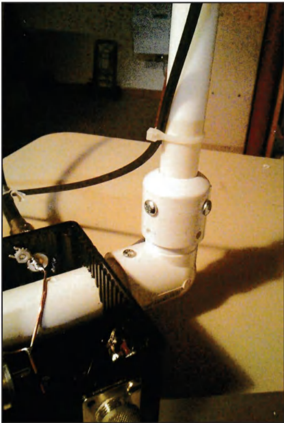
Photo D. Close-up of the PVC elbow used for operating the QRP mag-loop on a tabletop. The box is horizontal on the table and the loop support is vertical.
