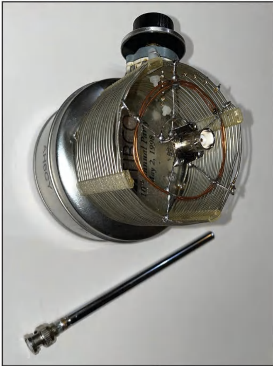
Photo B. The telescoping whip is mounted to the top of the loading coil via a BNC connector.
