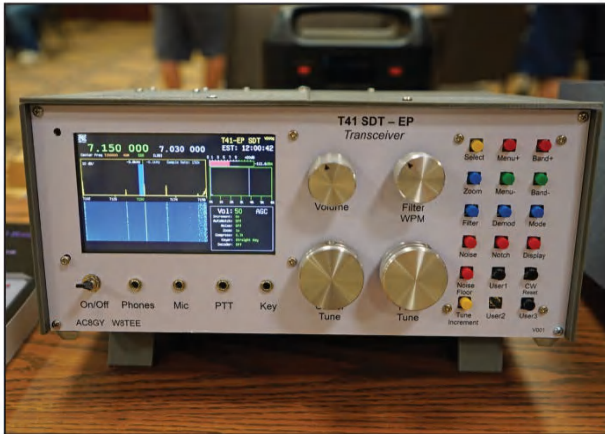
Photo B. The Four State QRP Group’s T41, a 5-band CW/SSB QRP transceiver offered in kit form. (KØNEB photo)
