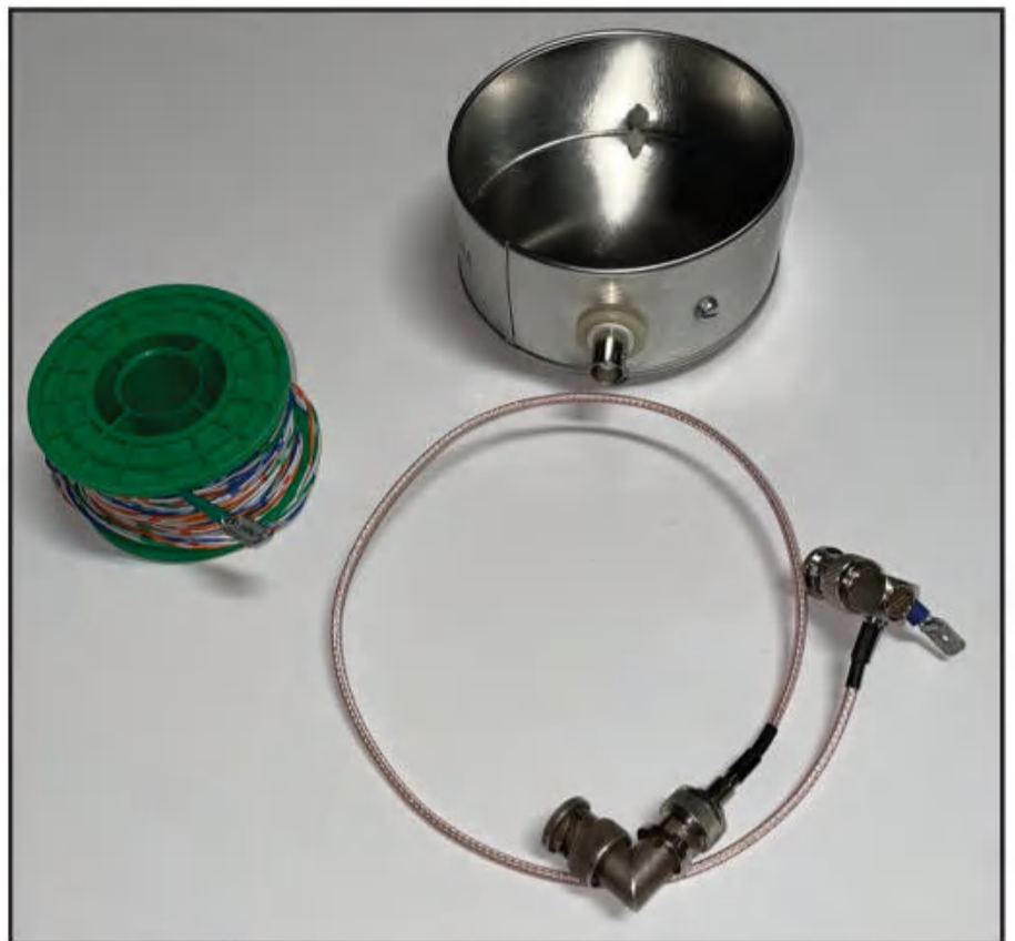
Photo D. In addition to the whip and coil assembly, the antenna system consists of a repurposed chocolate tin as a base, rolled-up radial wires, and a 3-foot-long feed line.
