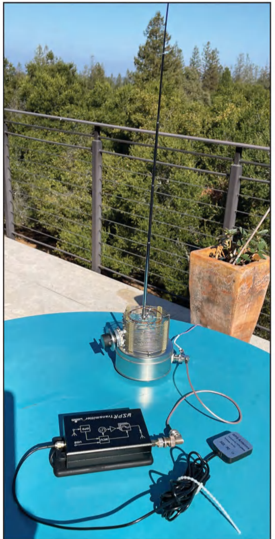
Photo A. Here I am operating WSPR with the 200-milliwatt ZachTek transmitter and the “Little Boy” antenna.
