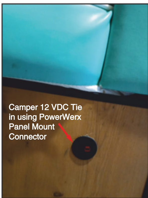
Photo G. Power cable into dinette area terminates in a PowerWerx DC connector.
