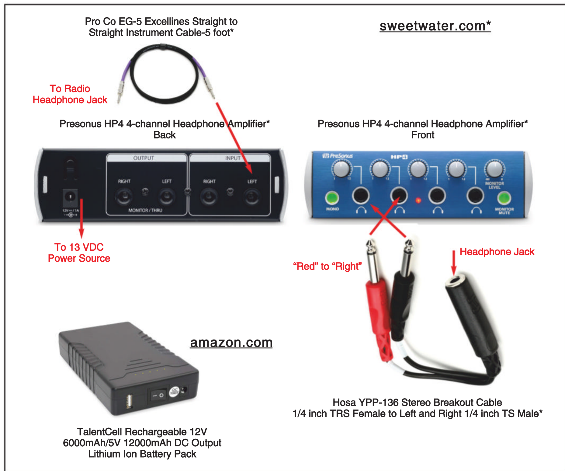
Figure 1. Headphone amplifier connection diagram
