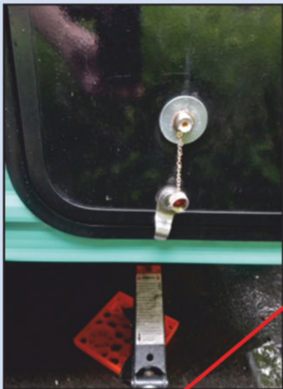
Front Right Access Door PL259 Connector with Threaded Cap
