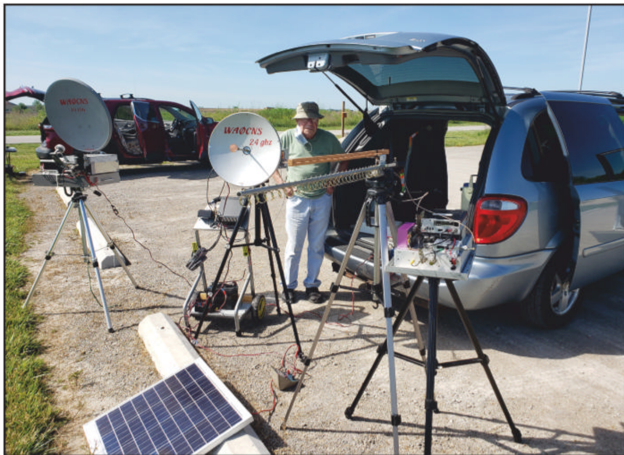
Photo G. Harry Haeusser’s, 1.2-GHz loop Yagi antennas along with some of his microwave gear on recent contest outing. (AF4JF Photo)
