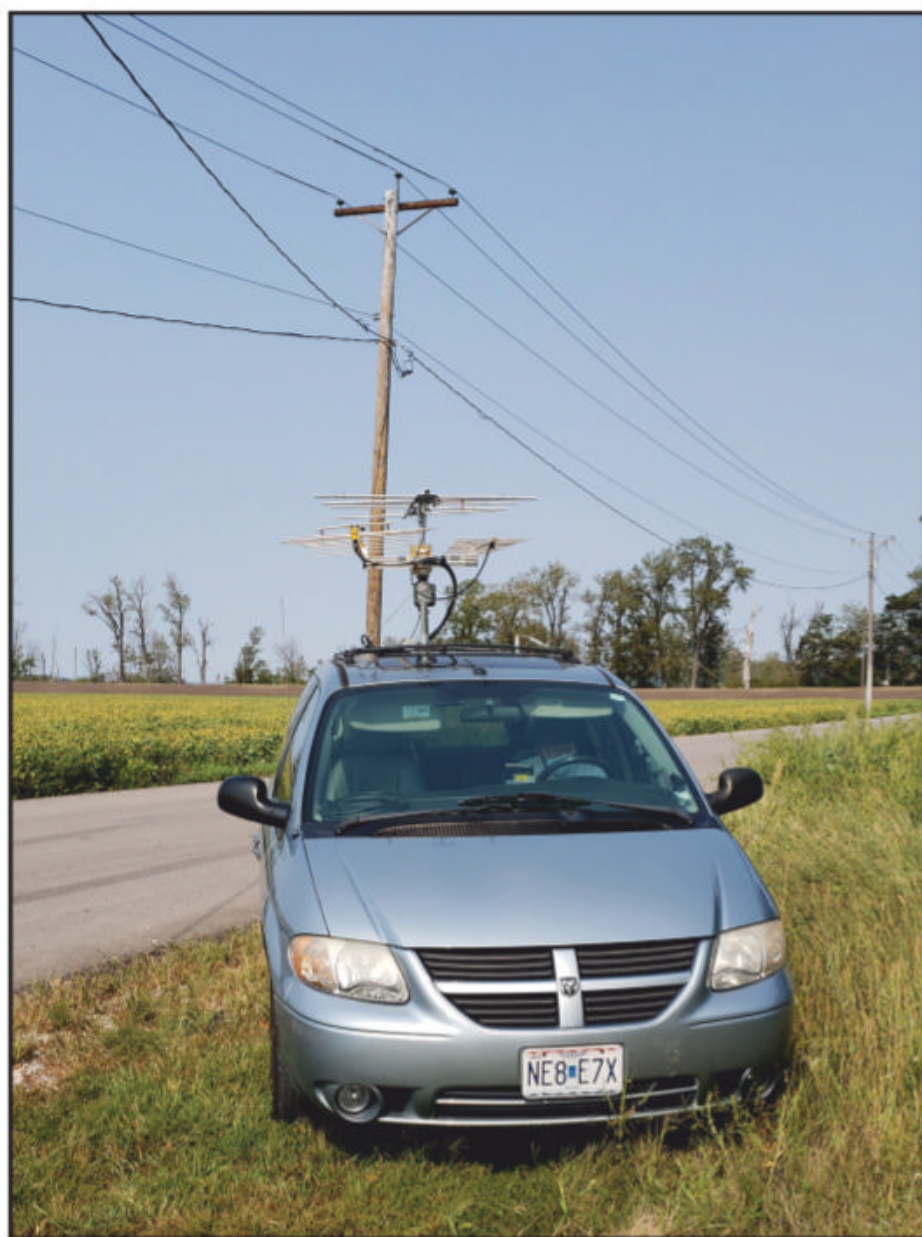
Photo F. Harry, WAØCNS, in his rover van. Note his roof-mounted 144-, 222- and 440-MHz Yagis. Harry uses a rotor to aim his Yagis when he is stationary. (Photo by Herbert Ullmann, AF4JF)
