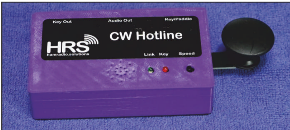
The finished CW Hotline in the 3-D printed case is assembled with the straight key option. A paddle still can be plugged in to the kit as well.
