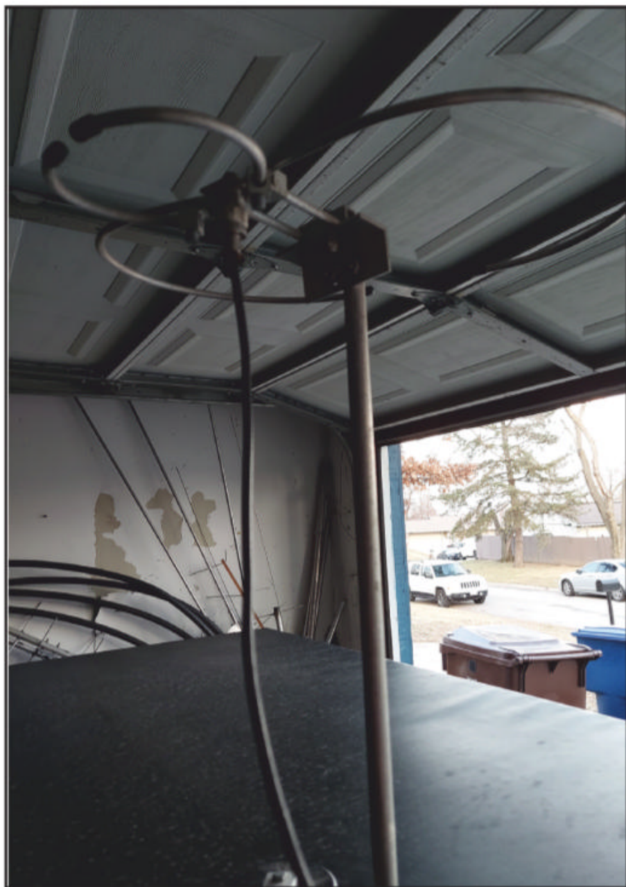
Photo E. My dual-band loop antenna with magnetic mount. This antenna has a single feedpoint, and it covers 2 meters and 70 centimeters. It is horizontally polarized.
