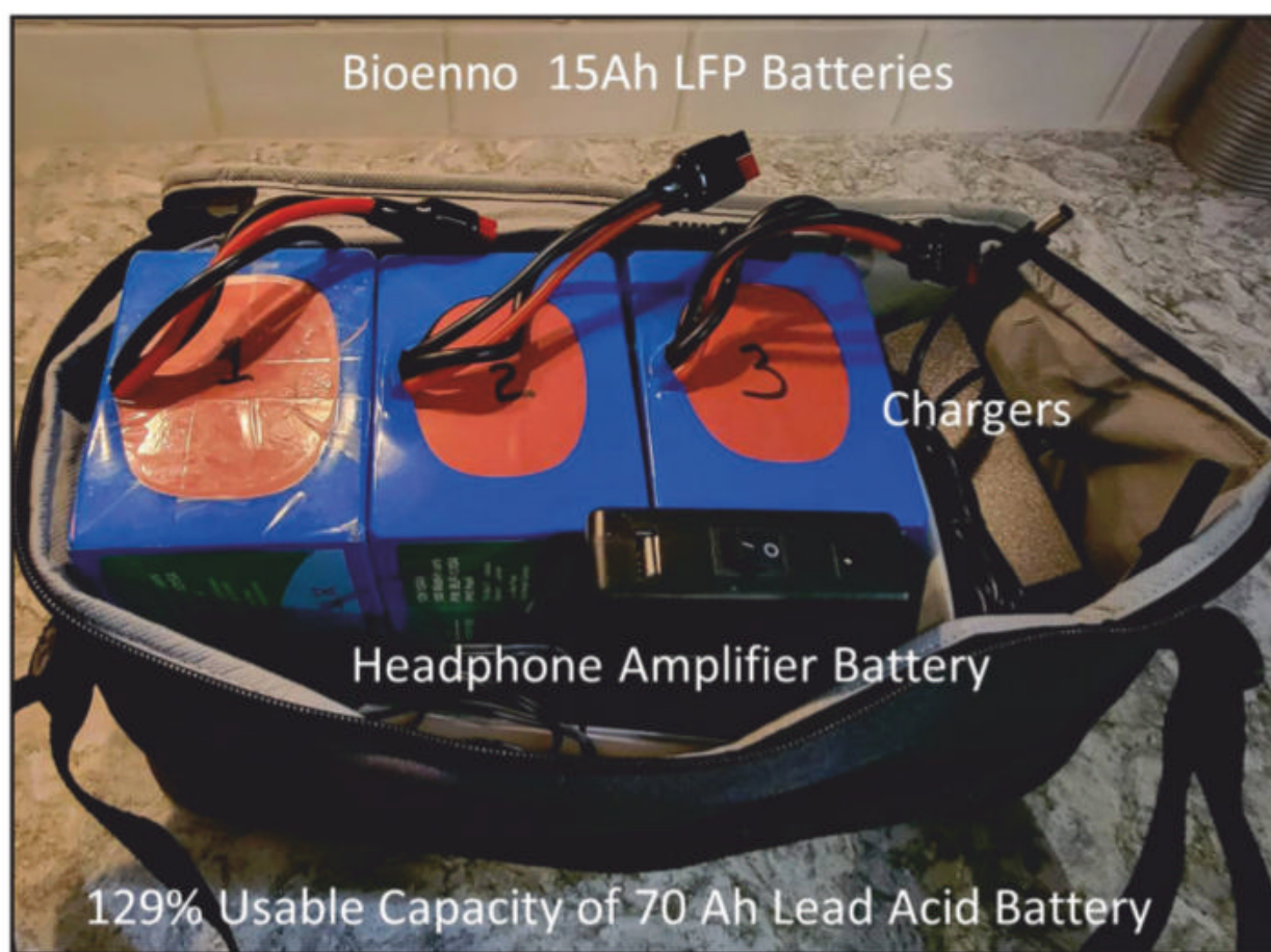
Photo A. The new power pack consists of three Bioenno 15-Ah LFP batteries.
