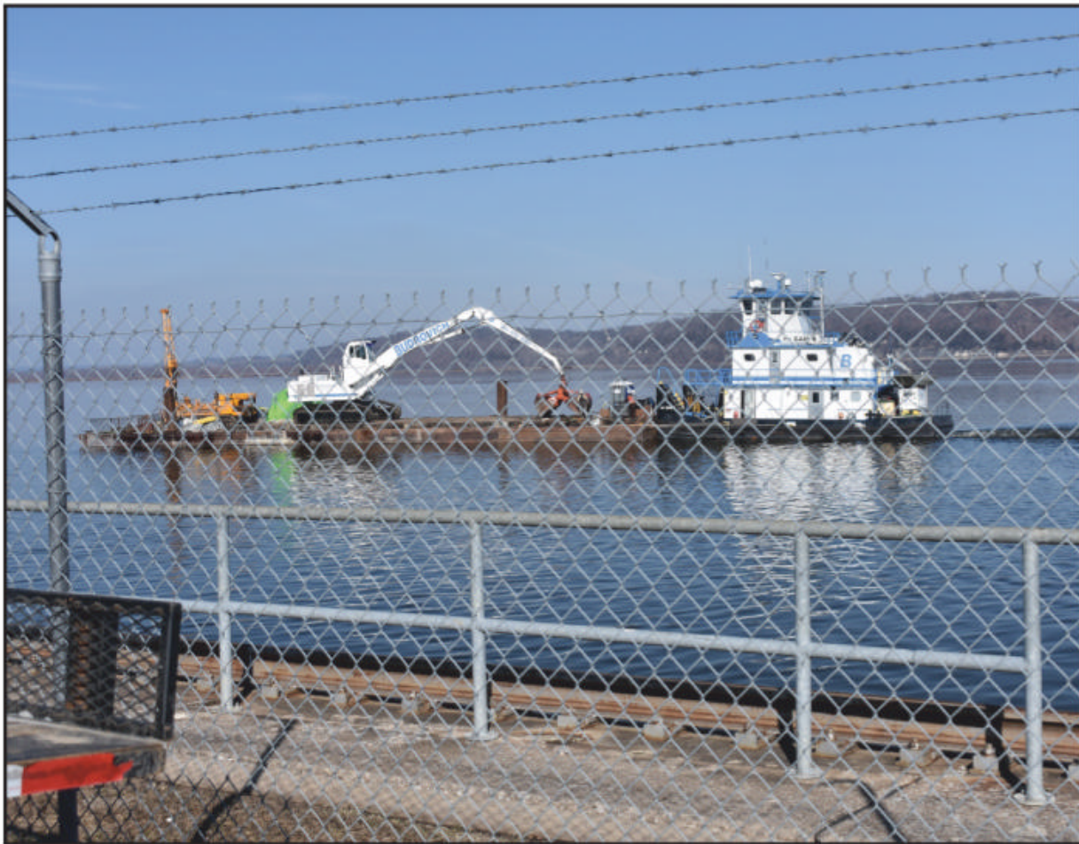
Photo D. A tow boat on the Mississippi River near Lock and Dam 25. Actually, tow boats push barges rather than tow them.
