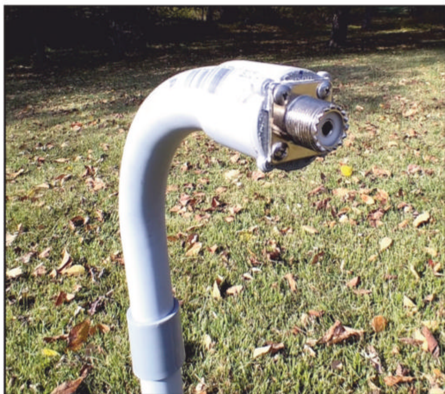
Photo E. The SO-239 connector mounted on the standoff
