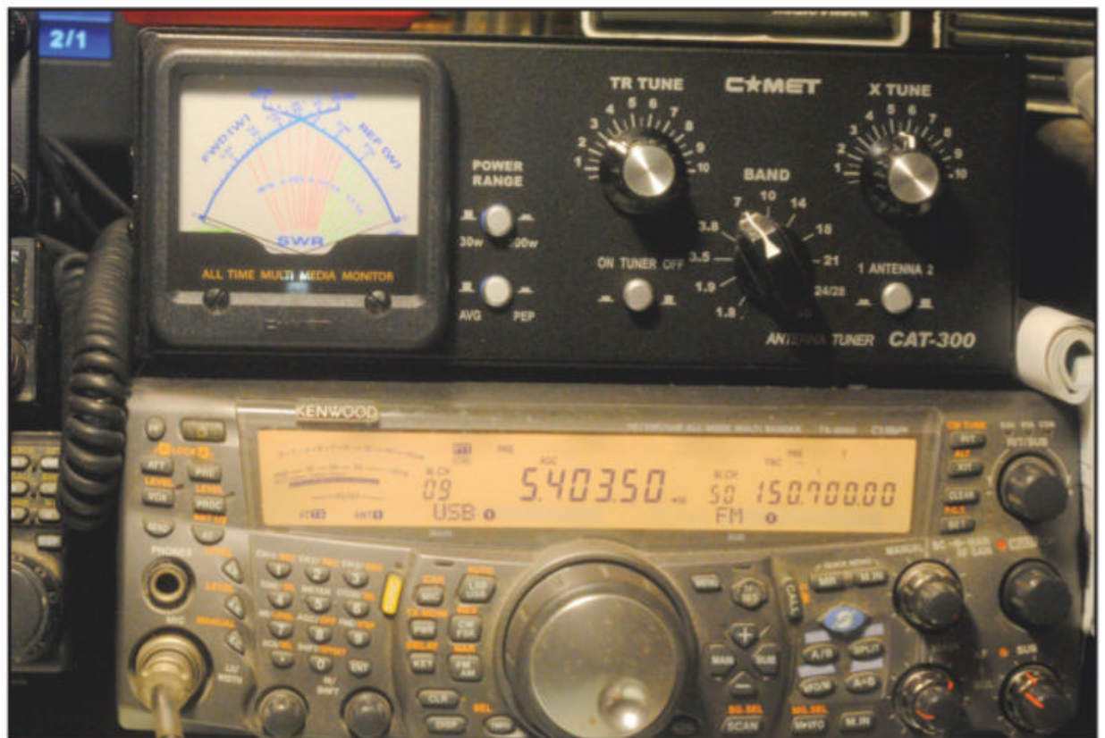
The Comet CAT-300 manual tuner easily tunes from 1.8 to 29.9 MHz and all in between.
