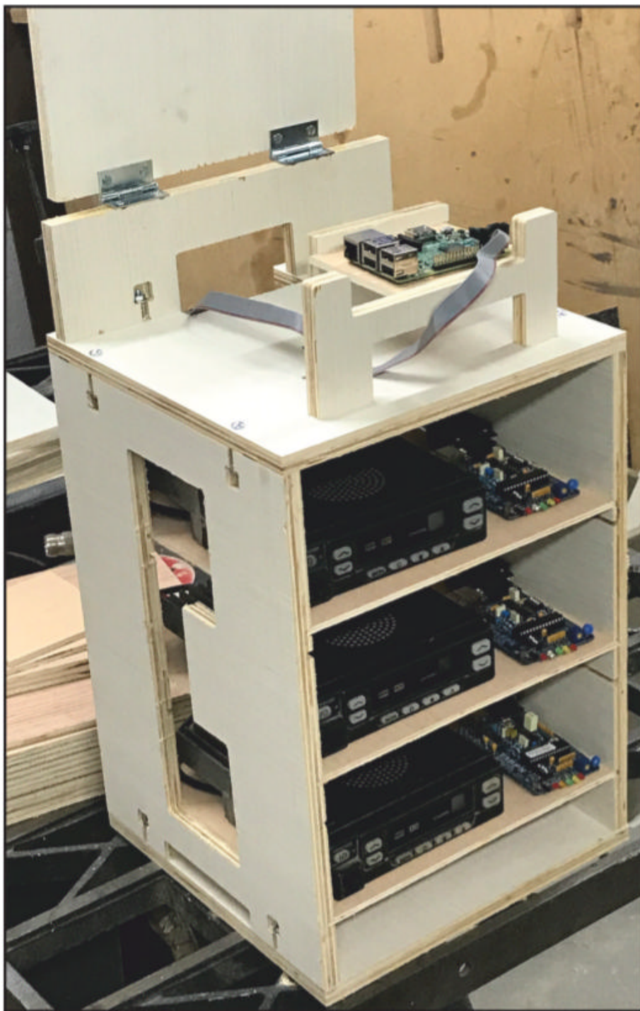
Photo A. A prototype TaddBox, designed to hold a complete three-port TARPN node (less antennas, of course). On top is the Raspberry Pi computer, and below are three radios and their associated KISS TNCs. There are some parts missing here, such as cables, power supply and backup battery (these sit on the very bottom shelf), and the Pi power supply and fuse box.
