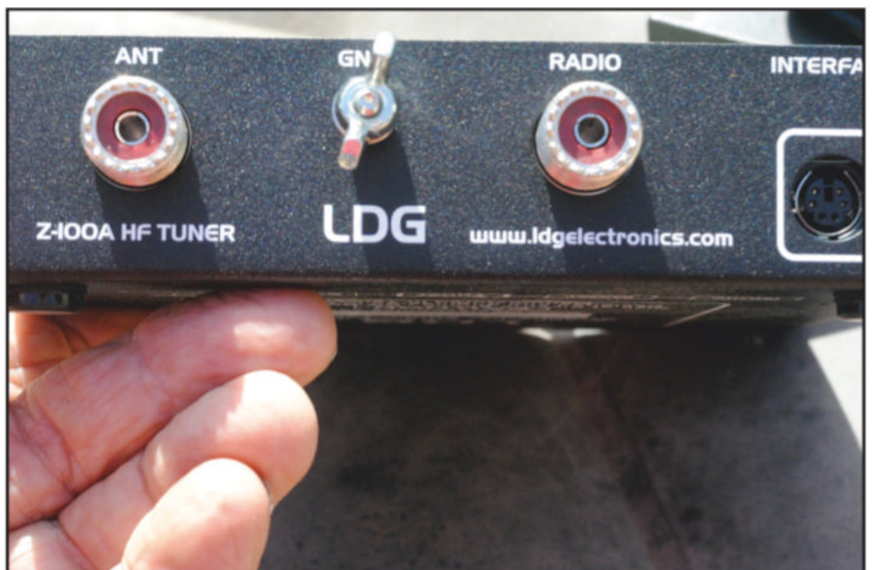
The LDG Z-100A has a coax output only to a balanced antenna system..
