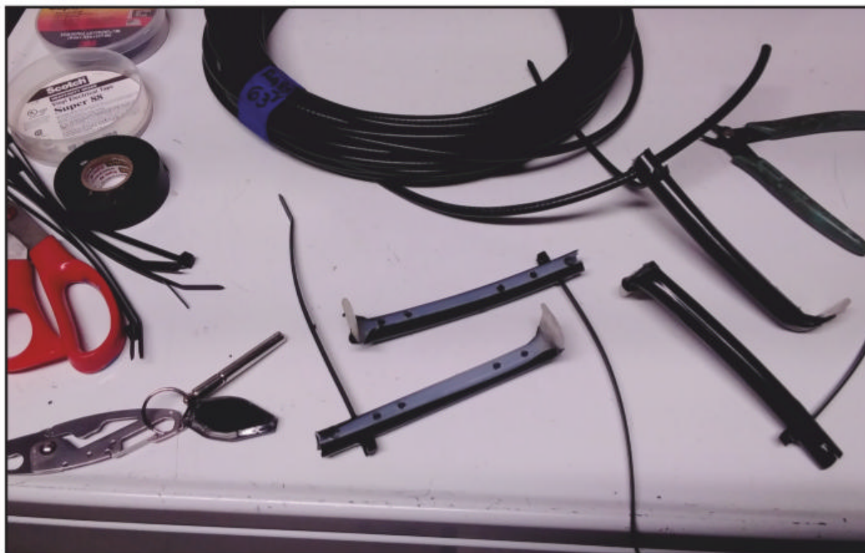
Plastic standoff insulators now replace the metallic insulators. A clamp holds the end of the insulator to the mast while the coax is tie-wrapped to the other end. These insulators only maintain spacing and do not have to support the weight as the main support is at the top of the mast. (Courtesy of W3TS)
