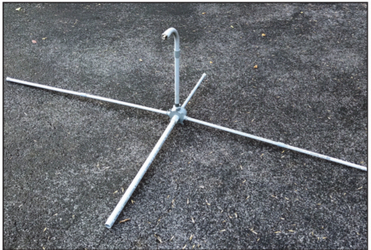
Photo D. The assembled antenna with the standoff
