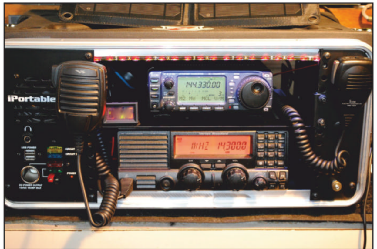
Gordo's portable SSB pack with a marine SSB on bottom working 14.300-MHz USB.
