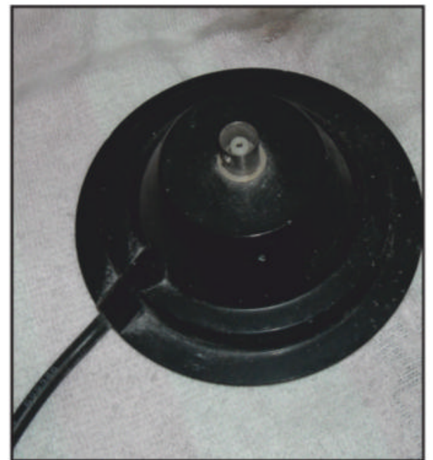
Photo D. A magnetic mount with a BNC connector can accommodate just about any antenna that also works with your handheld radio.
