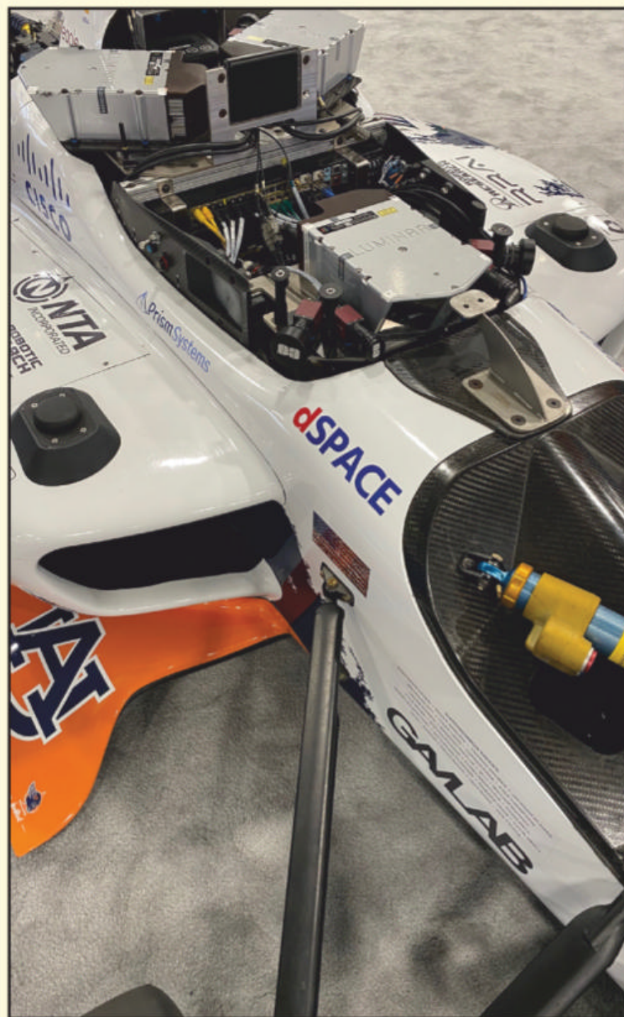
Photo O. The driver cockpit in an Indy Autonomous Challenge (IAC) racecar is filled with electronics. There is no room (nor need) for a human driver.
