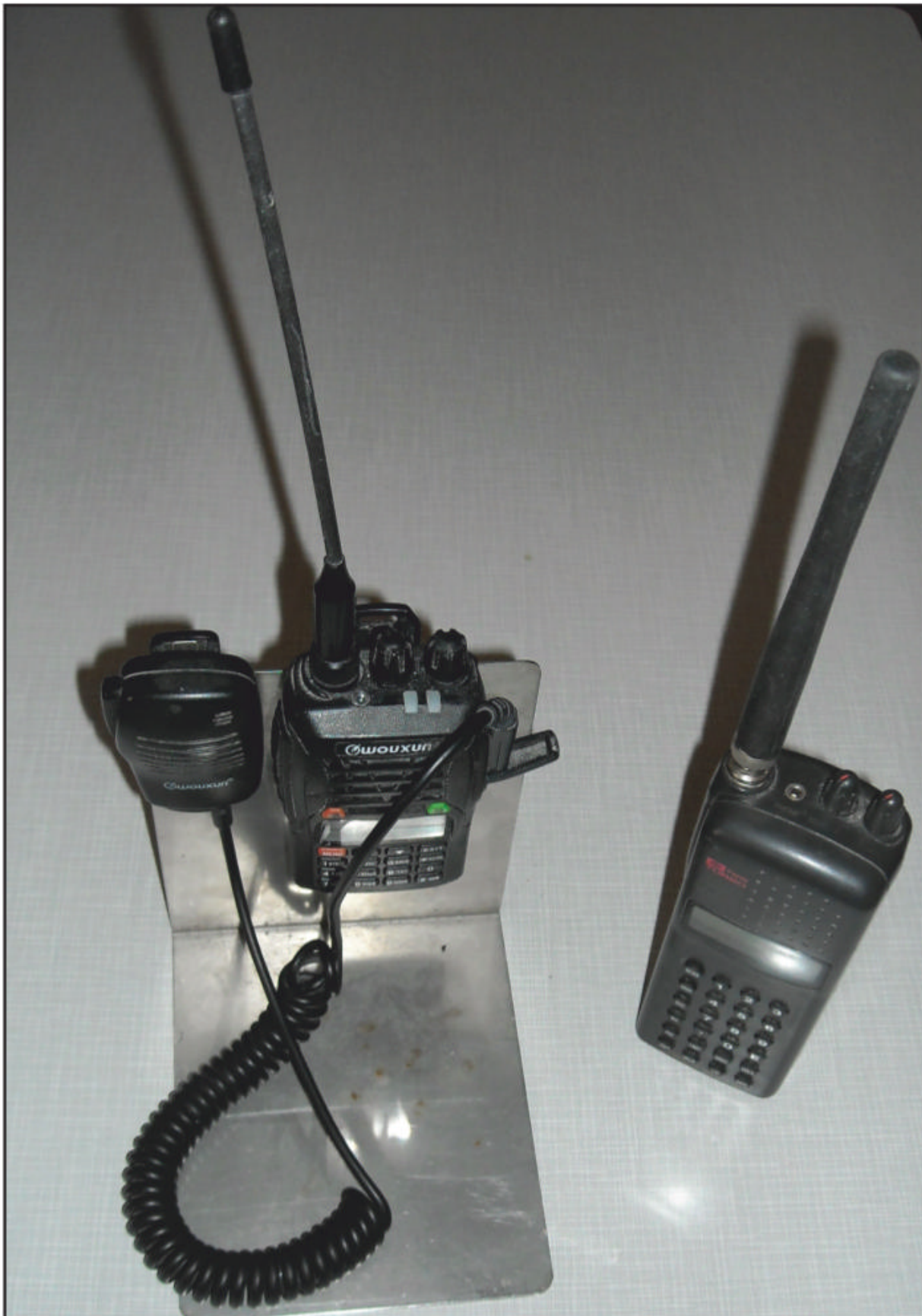
Photo C. A bent piece of scrap sheet metal can serve as a lightweight and portable stand for a handheld, especially when using it with a speaker-mic.
