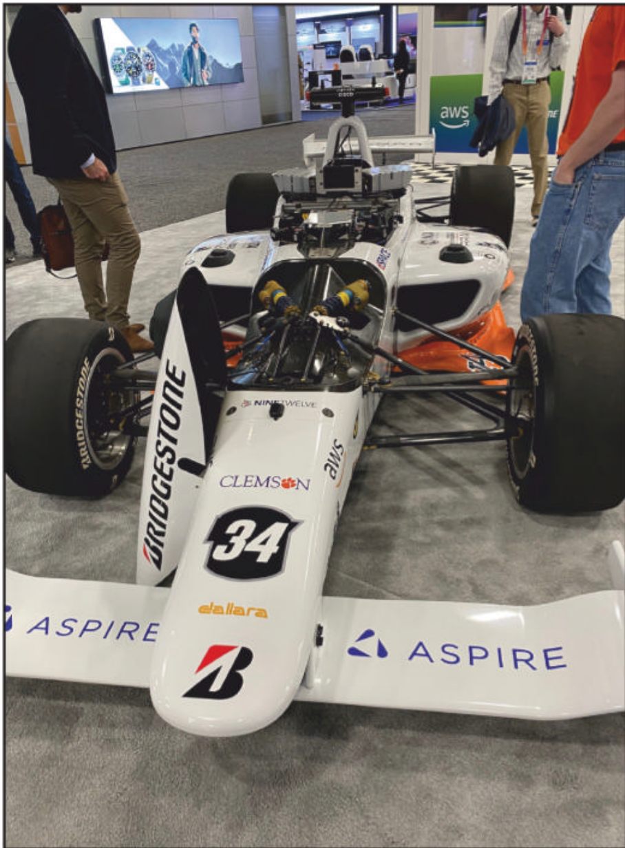
Photo F. One of the Indy Autonomous Challenge race cars. Looks just like an “ordinary” race car, but if you look closely, there is no driver seat (see sidebar for more).
