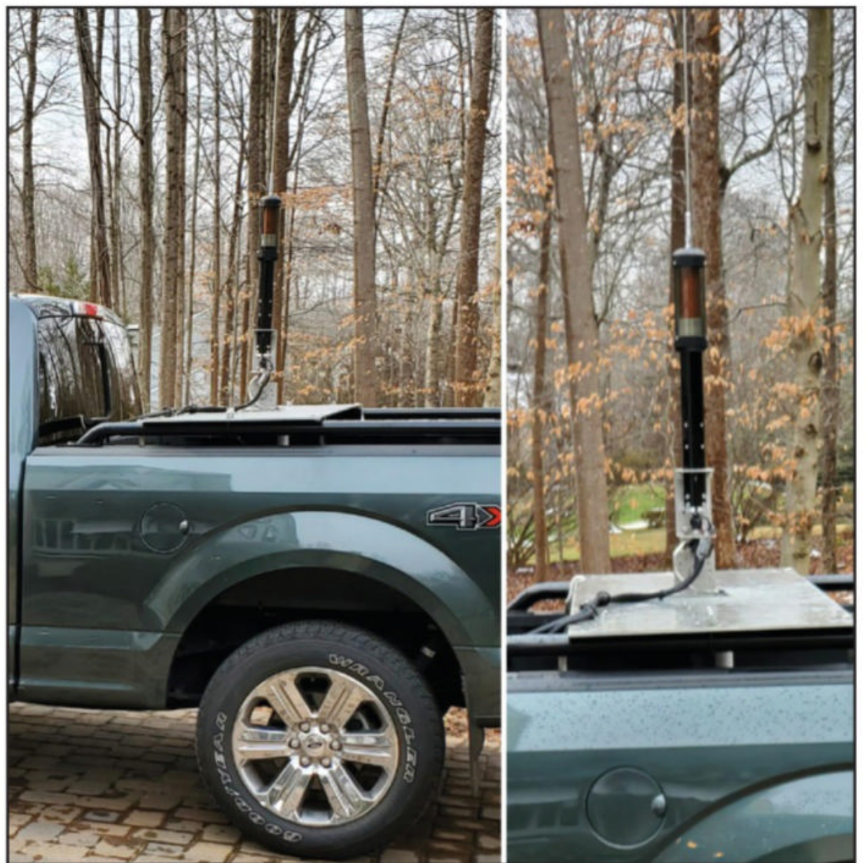
Photo G. Chip Lohman, NN4U, installed a Tarheel antenna < https://www.tarheelantennas.com > on his F-150 pickup. He also mounted the Yaesu FT-891 on a cup holder mount from < lidoradio.com >. He has an aluminum body truck that does not directly accept a magmount antenna. He solved that issue by placing a six-inch “donut” magnet on the inside of his moon roof glass with the magmount antenna attached through the glass. I would not drive with that arrangement, and would probably want a better ground plane. Things to think about.
