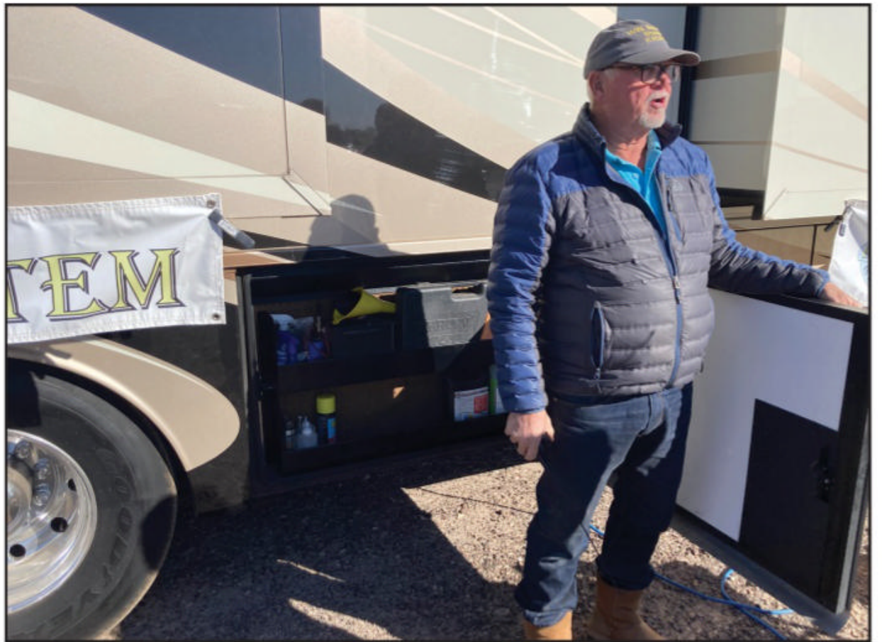
Photo A. Steve Taylor, K6UFX, of the WIN Repeater System is standing in front of the compartment where he keeps his 446.88-MHz portable repeater. The short-range repeater operates while driving down the road, allowing multiple hams traveling together to use it as they drive. The repeater is beneath the yellow funnel.
