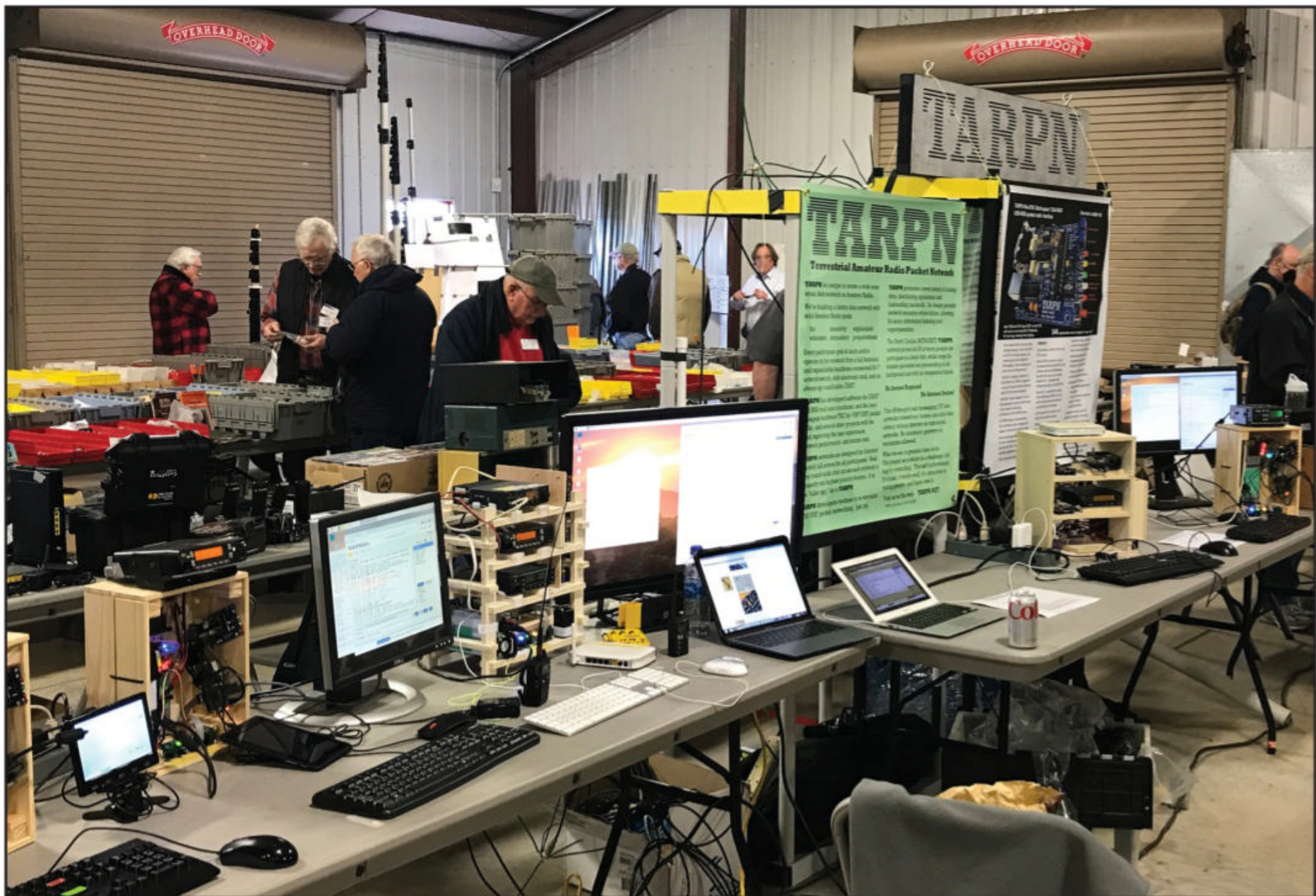
Photo C. The TARPAN network demonstration booth at the Stone Mountain (GA) hamfest in 2021. With five portable nodes, each with a computer and actual radios (using dummy loads though) attendees were able to see and hear how the network operates in real time. The same setup has been used for club meeting demonstrations and could be deployed in minutes as a functioning network in the real world.
