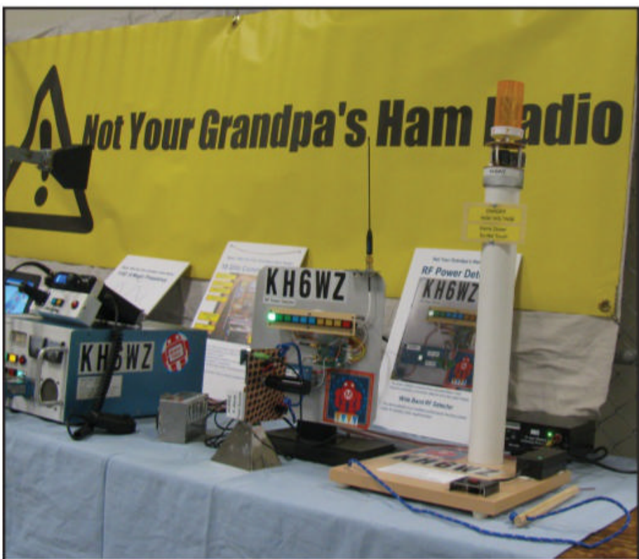
Photo D. The Mini Tesla Coil is shown on the right. A plastic medicine bottle covers the output. Holes are made so an insulated probe can be used to draw sparks and create artificial lightning.
