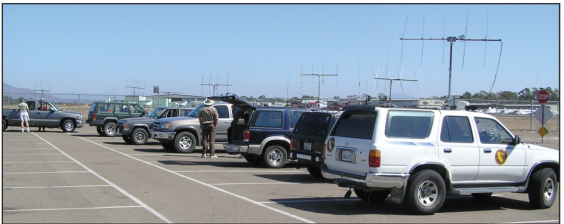
The big parking lot at Montgomery-Gibbs Executive Airport serves as starting point for many mobile transmitter hunts in the San Diego area. Most of the teams on this hunt are using rotatable two-meter quad or Yagi antennas for RDF. (Photo by Joe Moell, KØOV)
