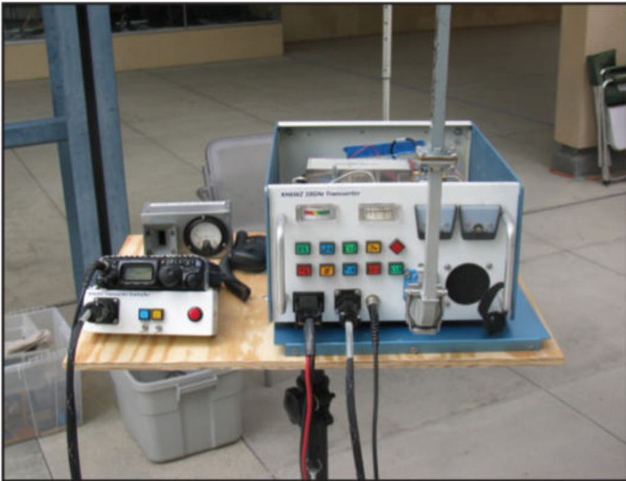
Photo C. Microwave transverter systems are ideal for demonstration stations, since the antennas are usually small and the rigs are portable. And they are a very different kind of radio.
