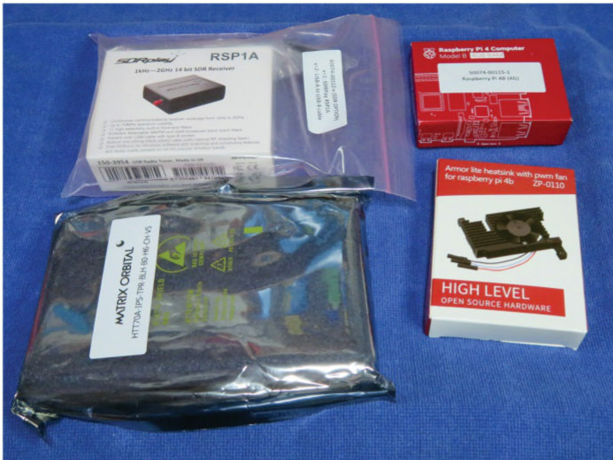
Photo G. The Raspberry Pi 4B and the heat sink, along with the SDRplay and the touch screen are also ready for assembly.
