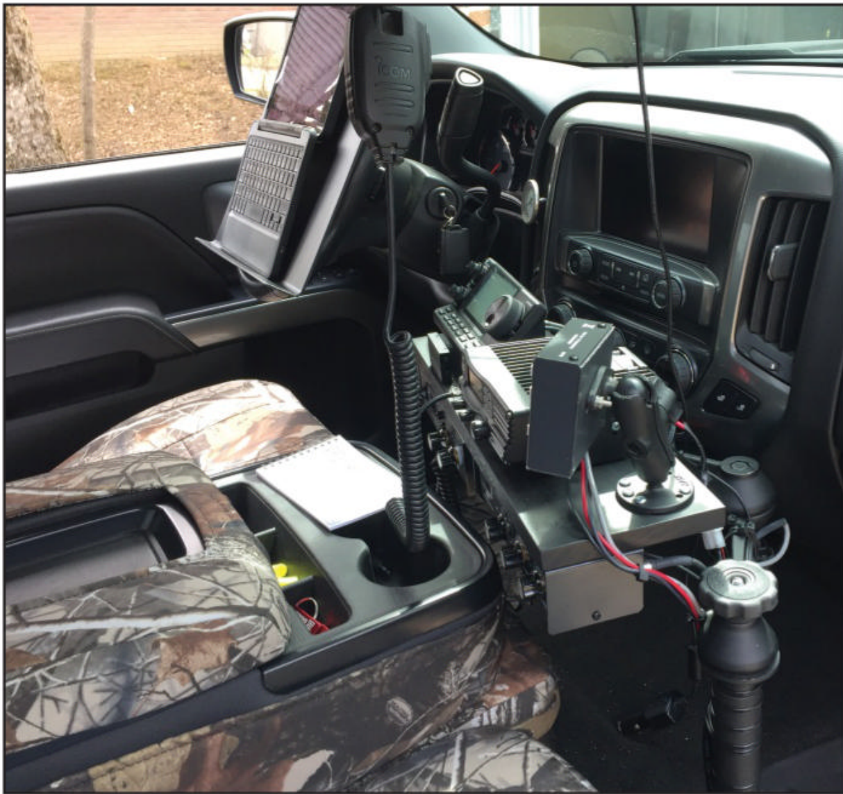
Photo H. Gary Marks, WD8ICX, has installed an Icom IC-7100 and Icom V-800, with tuners and the control for his Tarheel antenna, using a RAM mount system. Gary operates multiple modes from his driver seat position. His laptop is resting on a support that is attached to the steering wheel of his Chevy Silverado.
