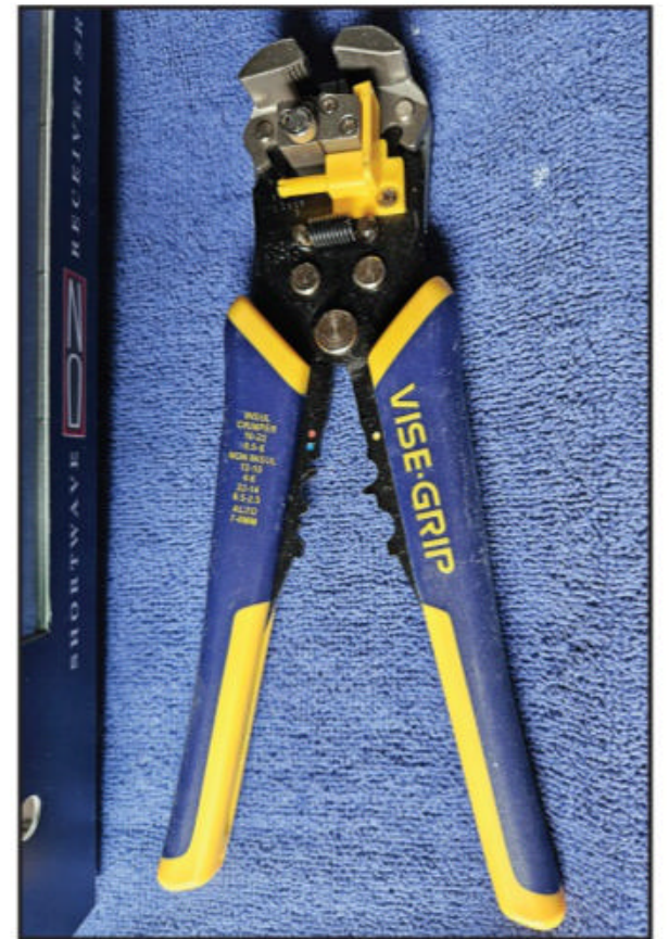
Photo H. The Irwin Vise-Grip automatic wire stripper was very useful in preparing the many wires in this kit.
