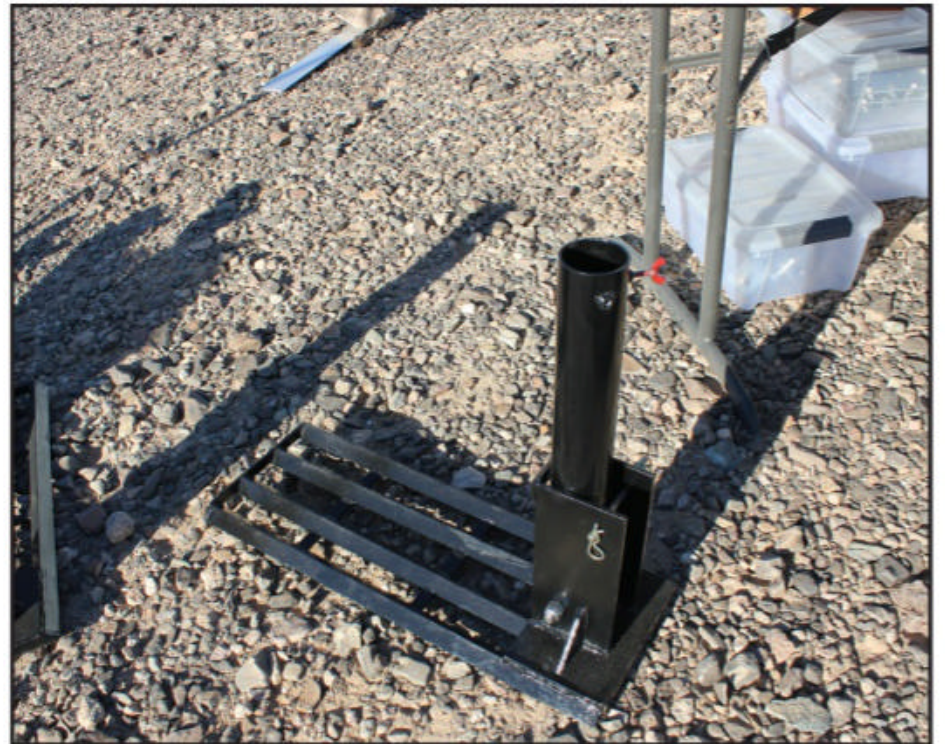
Photo F. An idea for a portable antenna mount. Drive over the flat part, holding the mount in place with the vehicle tire. The tilt-over vertical mast support makes erecting and working on the antenna relatively easy.
