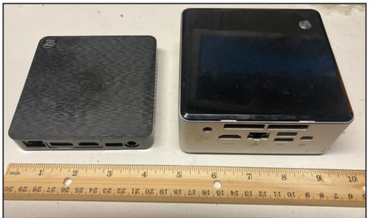
Photo A. Two small 12VDC-powered logging computers you might consider as part of a battery-powered effort on Field Day. On the left is the Beelink T4; on the right is the Intel NUC.
