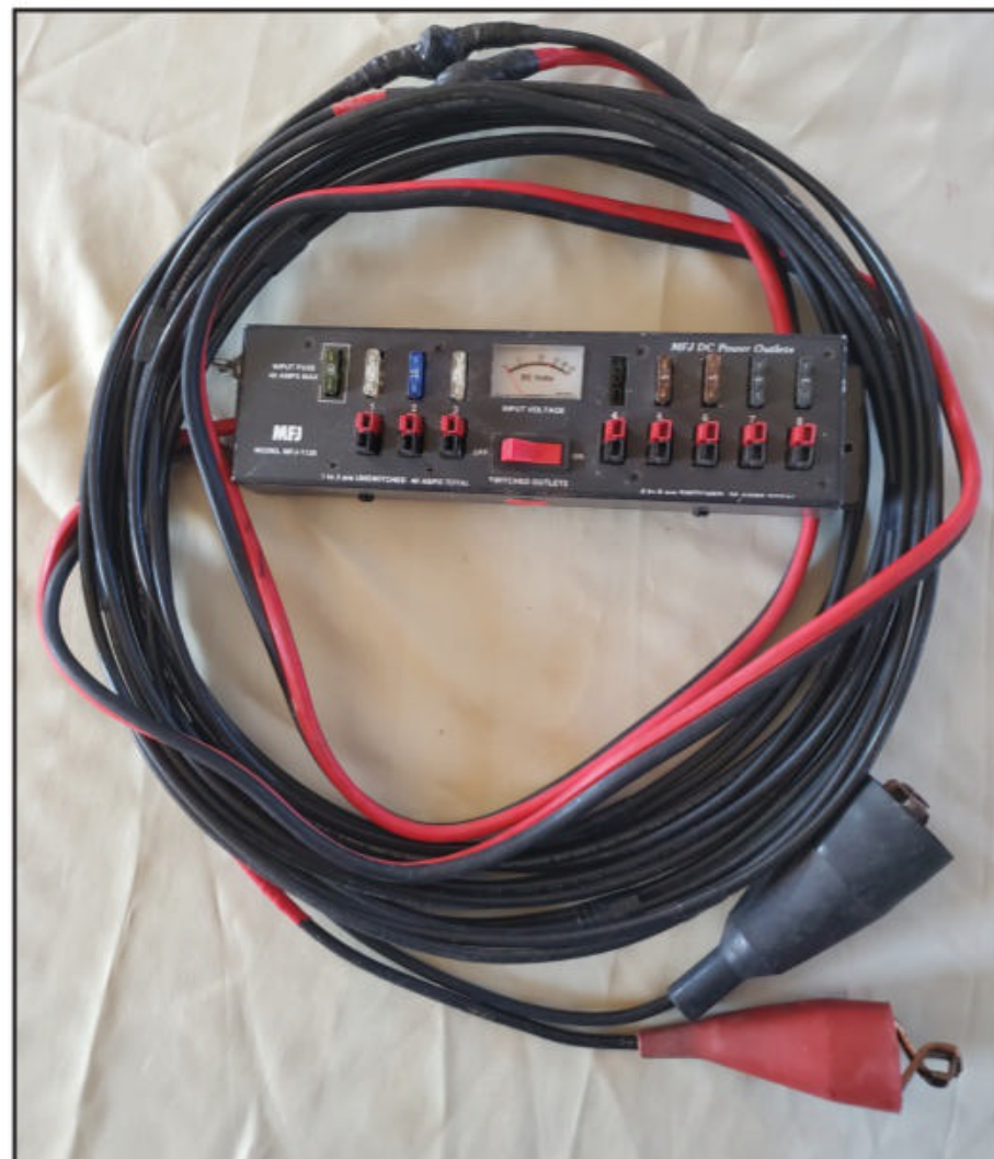
Photo E. Power Pole distribution with # 8 wire and big clips
