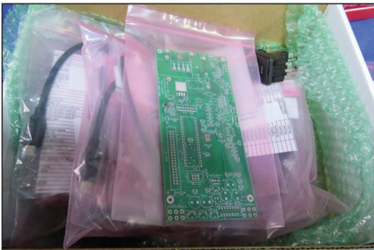
Photo B. A box of many of the parts needed for assembly, packaged in labeled antistatic bags.
