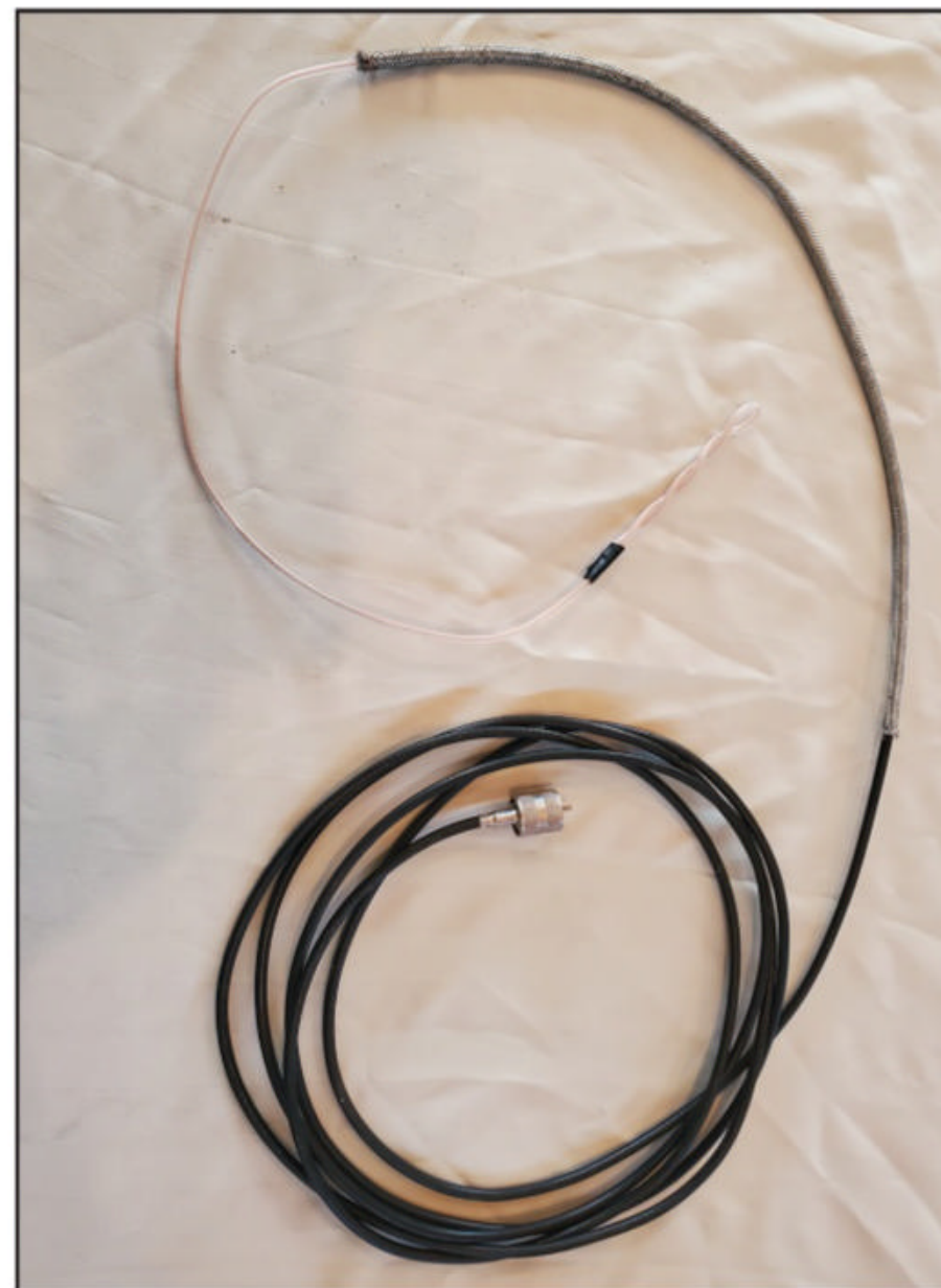
Photo F. Coaxial dipole comprised of RG 58/U and a coax connector
