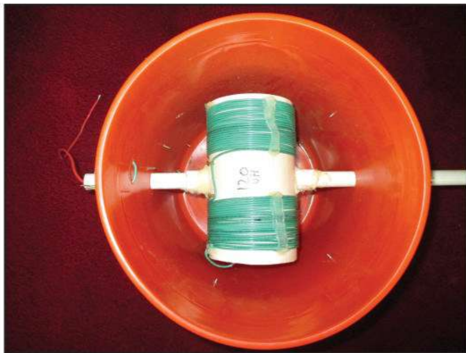
Photo C: Here is an image of the nested coil of a variometer. In this position the coil provides minimum inductance. The number of turns on the nested coil also determines the rate of change of inductance. Input and output for the nested coil are accomplished via the shaft that is used to adjust its orientation. (Courtesy WA3ETD)
