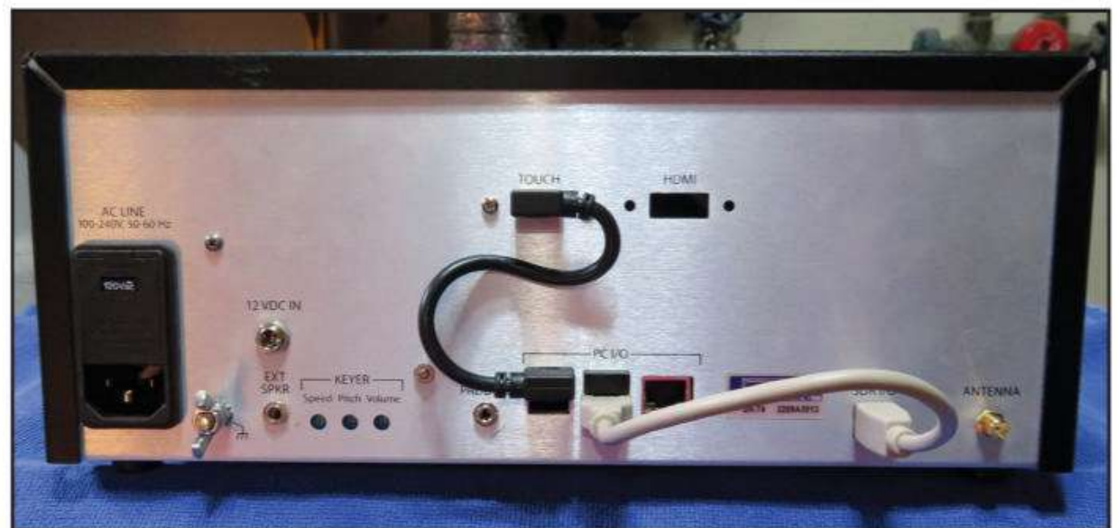
Photo B. The rear panel of the Saguario has the connections to the Raspberry Pi as well as audio output and a paddle input for the built-in code practice keyer.
