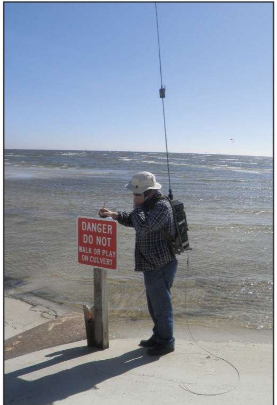
Photo E: Note the trailing drag wire (counterpoise) for the author's backpack-mounted vertical antenna.
