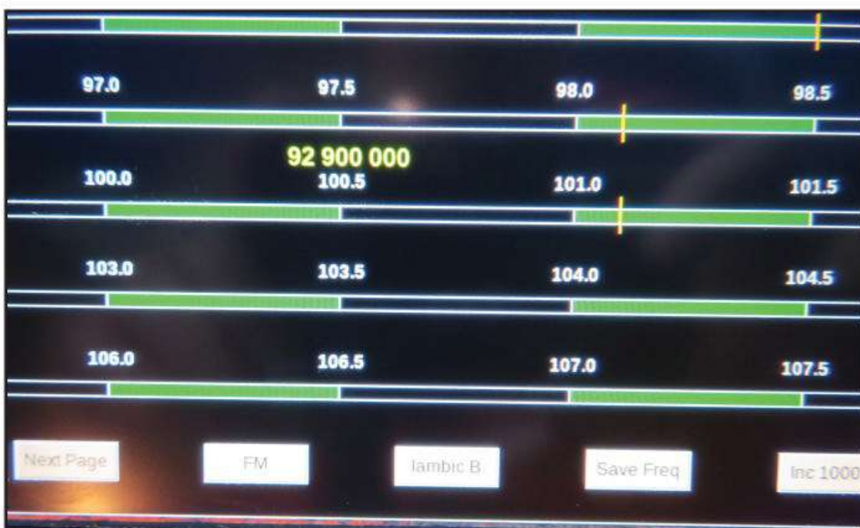
Photo D. Frequencies as high as the FM broadcast band are received. This is tuned to KTGL, a local FM station. For higher frequencies up to 2 GHz, CUBIC SDR software is included on the Pi software SD card but must be accessed using a keyboard and mouse.
