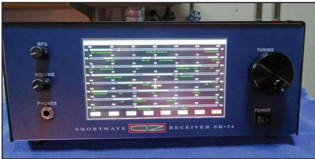
Photo C. The case is finally closed and the receiver is working and tuned to WRM1 5.050 MHz.
