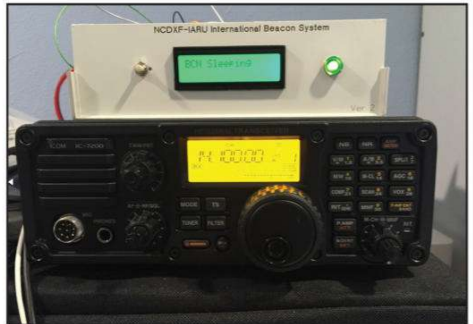
Photo A: International Beacon Project stations use a specialized beacon controller to assure that they transmit on the proper time sequence. (Photos from NCDXF/IARU IBP website)
