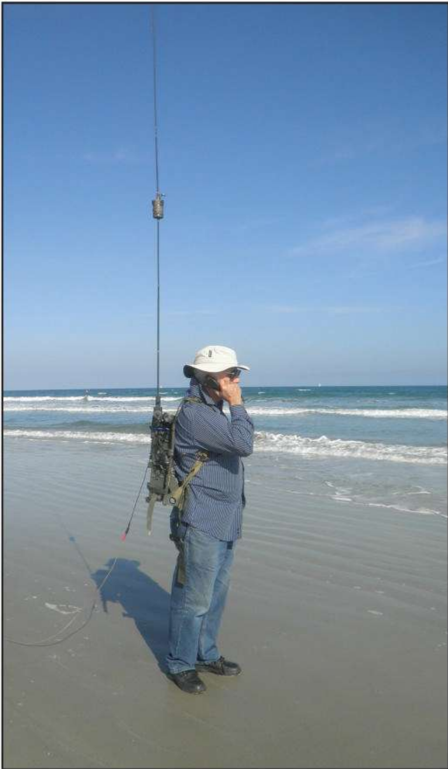
Photo D: Getting out on the beach with salty sand beneath your feet results in immediate signal improvements, both on receive and transmit.
