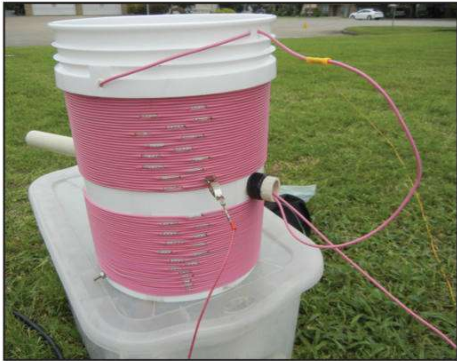
Photo B: This is a variometer that is commonly used to resonate 630- and 2200-meter antennas. It is two coils in series, a fixed outer coil and another that is rotatable inside of the bucket. RF is applied to one of the taps, selected experimentally using an antenna analyzer to find where reactance goes to zero, thus resolving the resonant point. The top of the coil feeds into the shaft of the nested coil and then returns through the same shaft with the returning wire going to the antenna.
