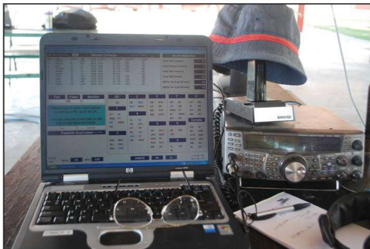
Photo F: FD logging program. A good logging program networked with other FD operating stations is a tremendous work saver. It also allows club members new to Field Day a chance to actively participate. Today's logging programs are intuitive and easy to operate. Pictured is N3FJP's FD logging program on the laptop screen.
