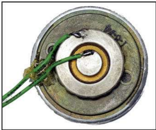
Photo A: Solder connections to a T1 carbon mic element from an old telephone.
