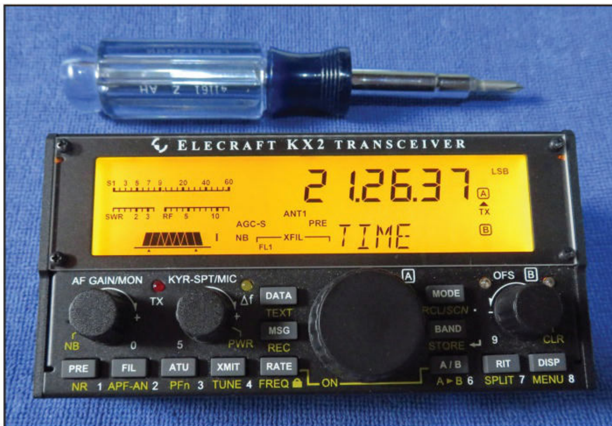
Photo H: The radio is reassembled and the new real-time clock is activated as well as the internal charging function. The charging rate is a bit slower than using the dedicated outside charger, but you no longer have to open the radio to charge the battery.
