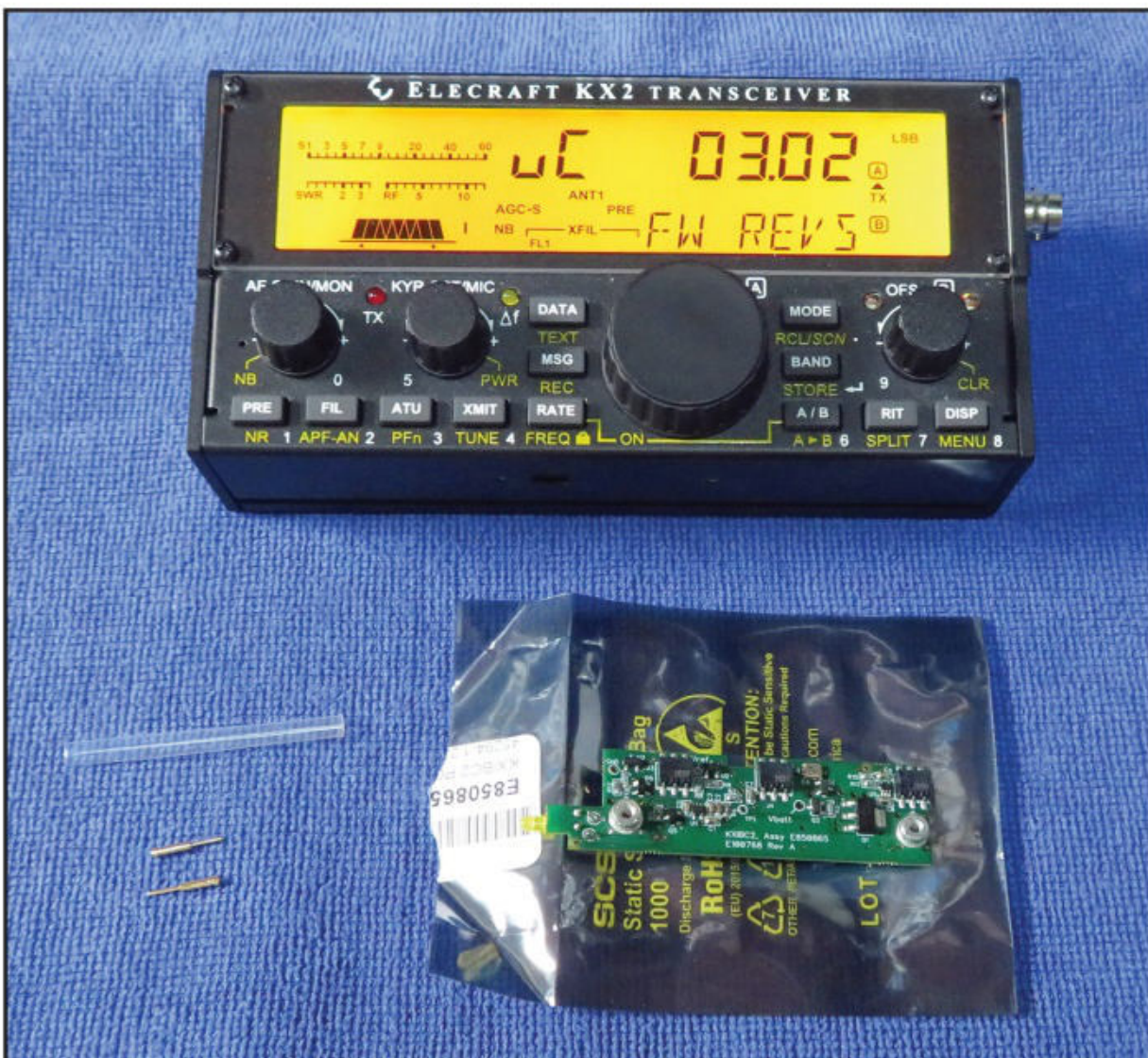
Photo E: After updating the firmware on the Elecraft KX2, the radio is now ready to be opened and the internal charging kit installed.
