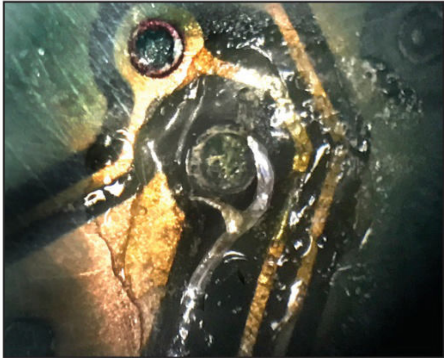
Photo B: This via pad carries the receive audio (RXA) signal directly from the radio's discriminator circuit out to the TNC. Despite extreme care and my 20x stereo microscope, this trace was badly damaged in the attempt, being broken and lifted from the board.
