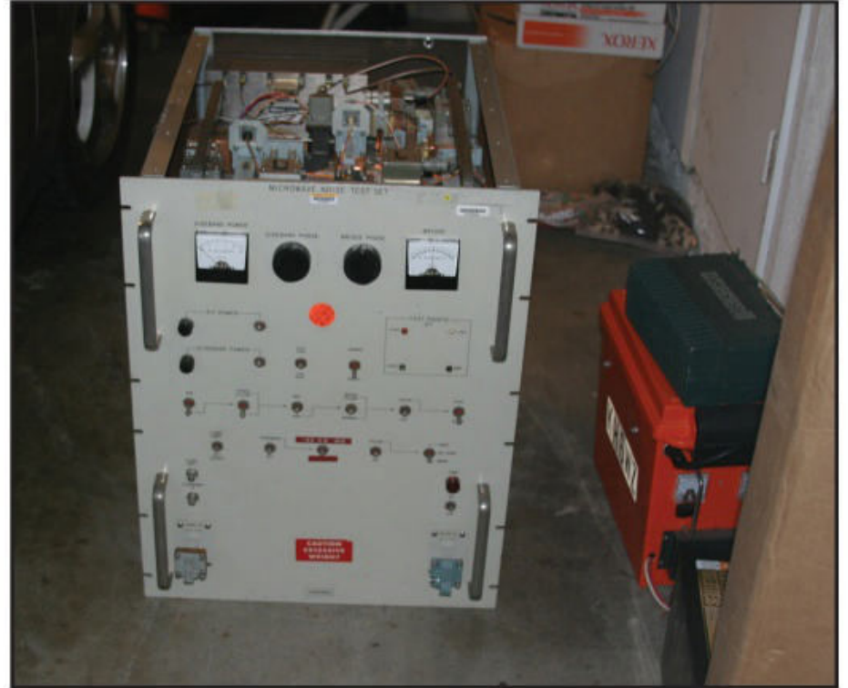
Photo H: This "Microwave Noise Test Set," filled with tons of 10 GHz components and assemblies, is another one of my most amazing surplus discoveries.
