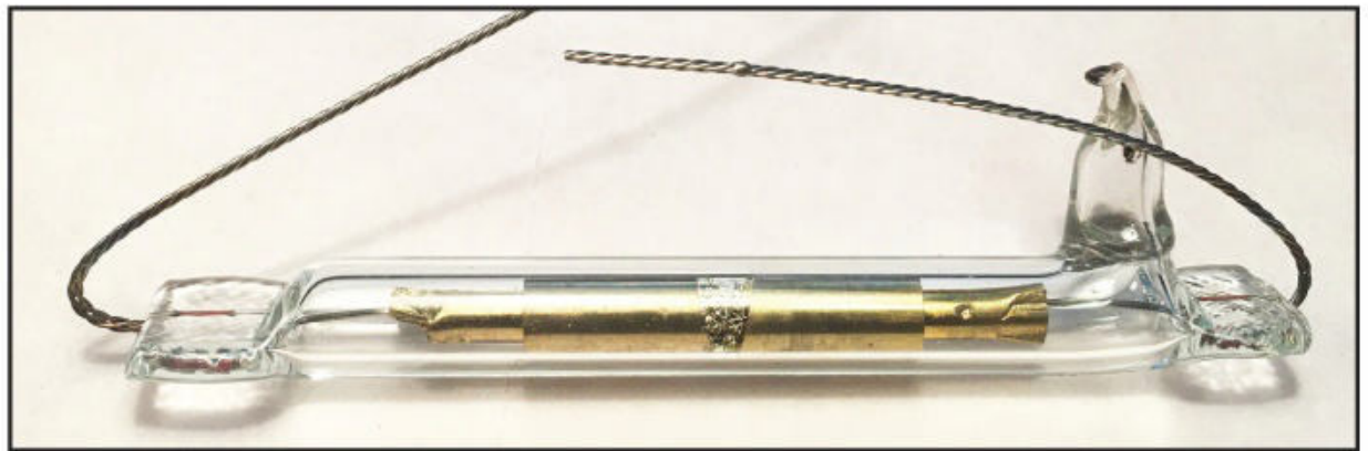
Photo A: Branly coherer with brass powder. (Photos by the author)
