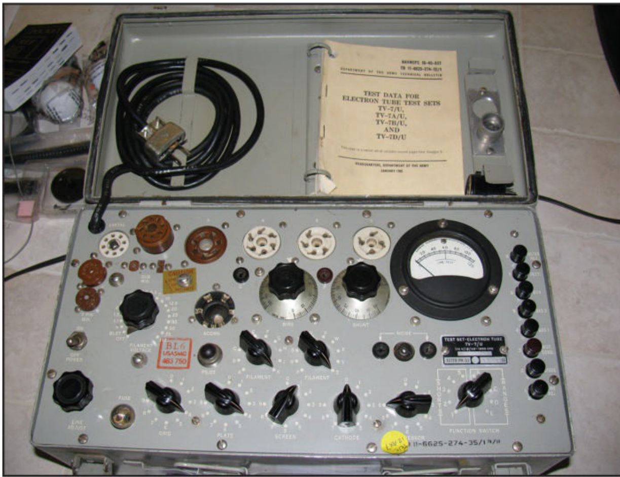
Photo C: A US Army TV-7/U tube tester, purchased on eBay, is a great tool for testing old tubes.
