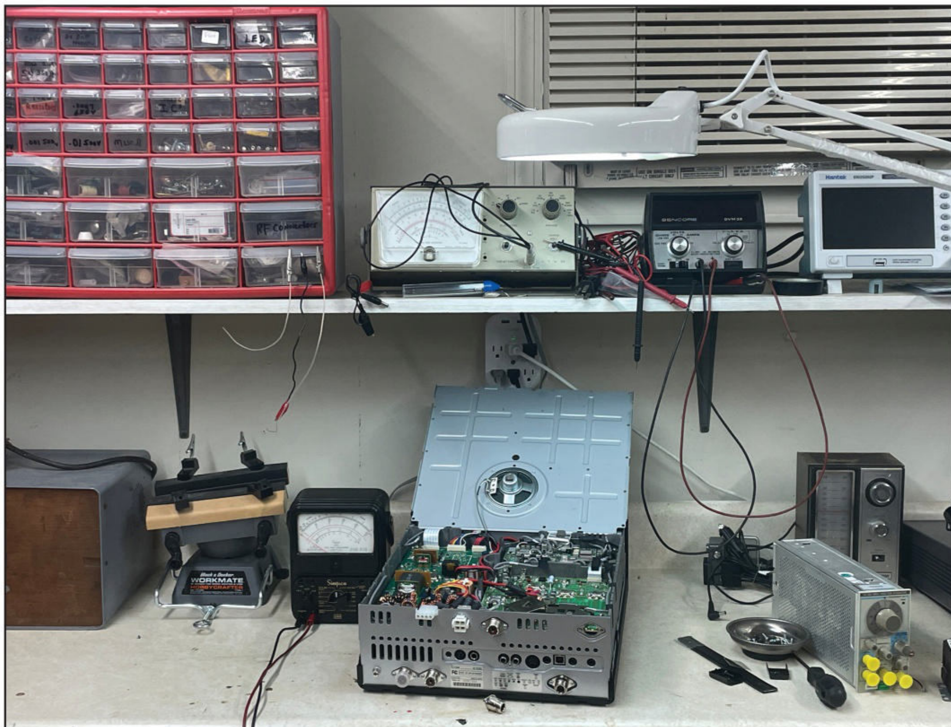
Photo B: New workspace for N4DTF showing IC-9100 undergoing 432 MHz connector repair.
