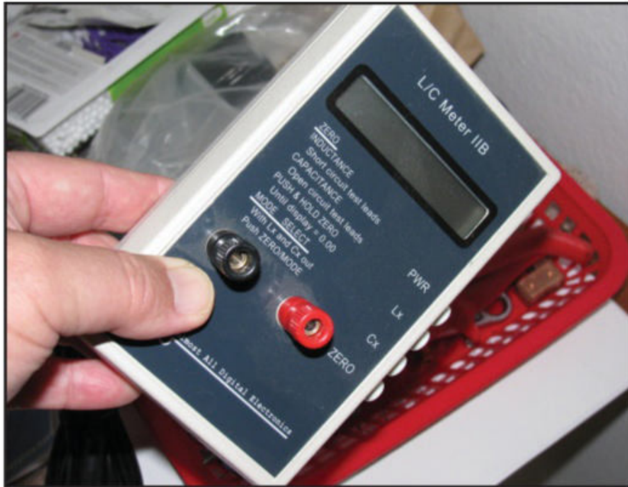
Photo D: A capacitor and inductor tester should be in your tool kit if you build and test your own gear. This unit has been discontinued, but many modern multi-testers include a capacitance function.
