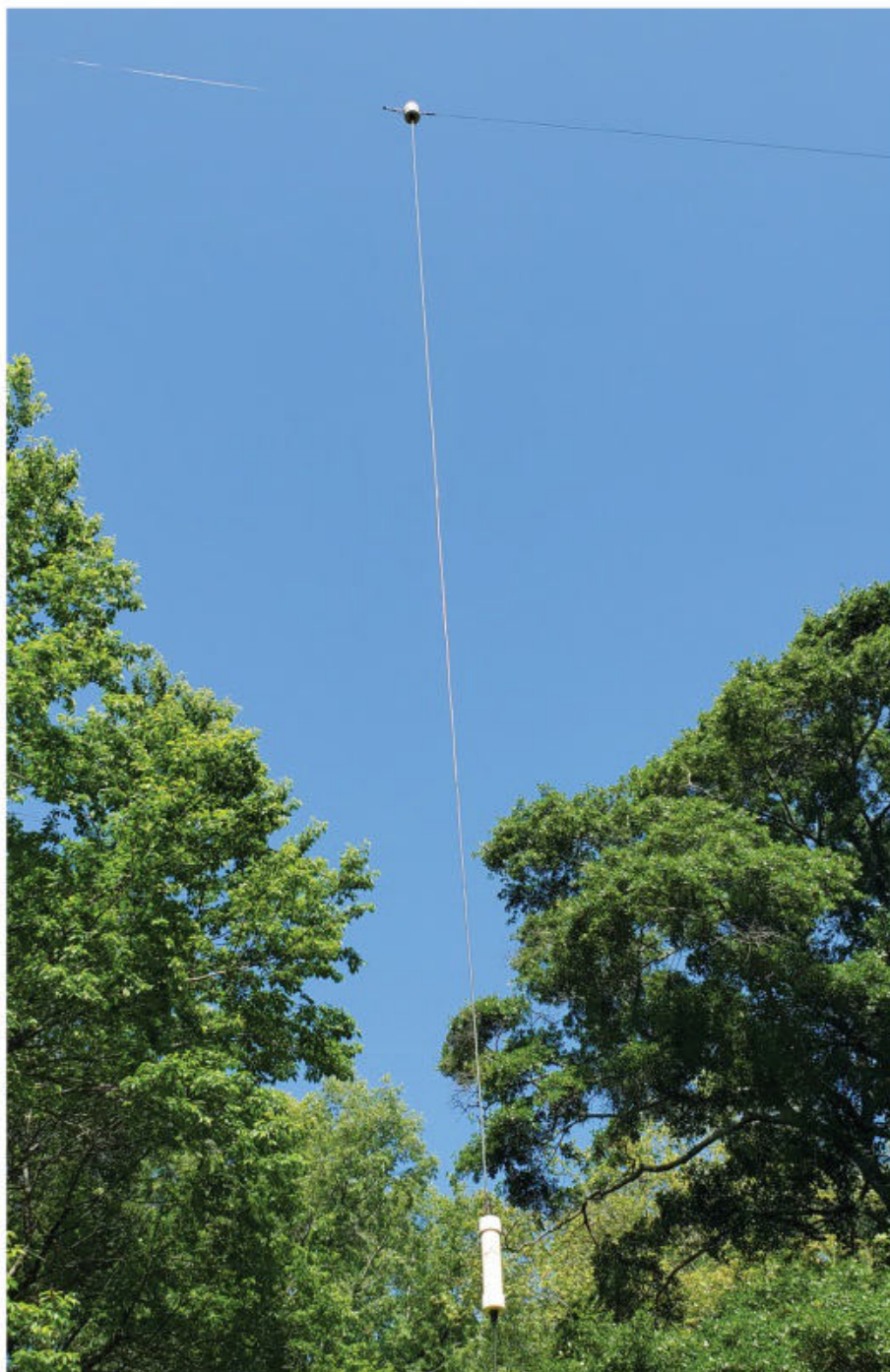
Photo D. Feed for the Carolina Windom 160® showing the OCF balun, the 22-foot vertical section and the 1:1 isolating balun for connection to the feedline.
