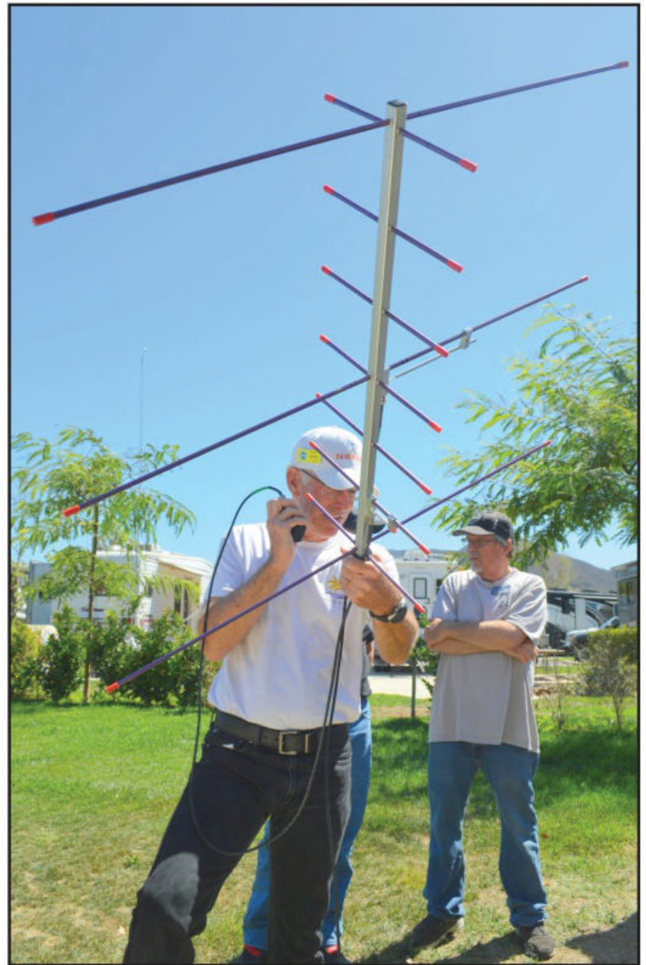
Photo C: This simple Yagi is all you need to work other hams through the repeater on the space station.
