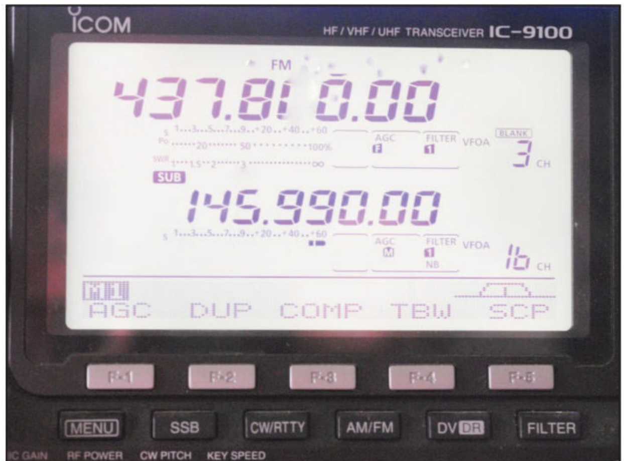
Photo B: 437.810 MHz is where you will first hear signals coming up from the International Space Station's cross-band repeater as it begins a pass over your location.
