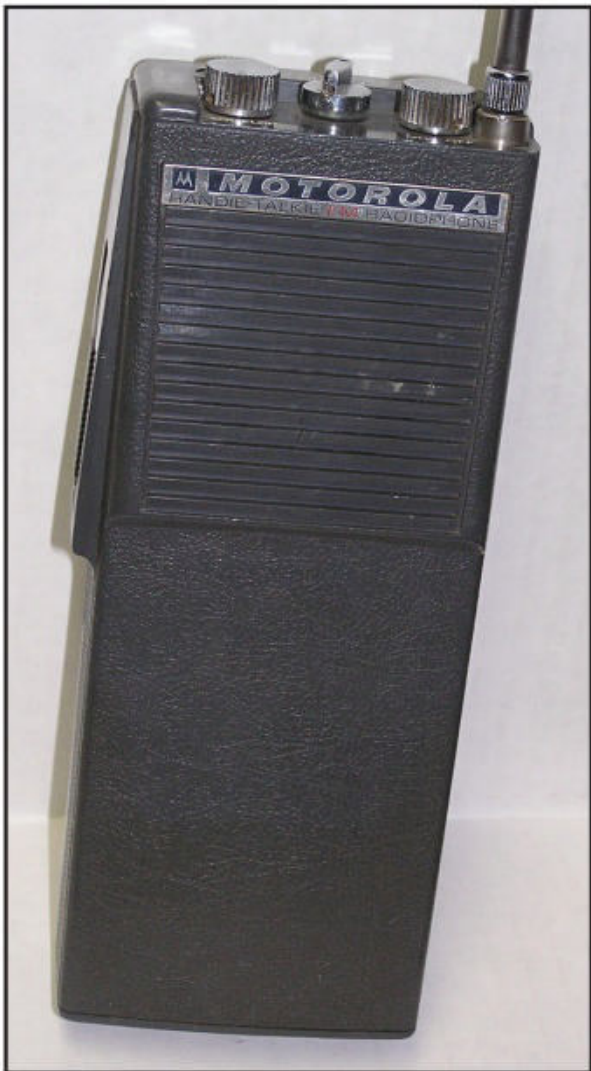
Photo C: The Motorola HT-200 "brick" handheld could be tuned to operate on mobile phone frequencies. It didn't matter that you couldn't dial with it, as calls had to be placed through the mobile service operator.
