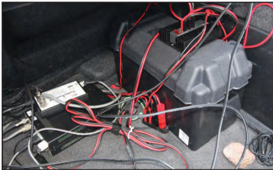
Photo A. Power installation in the trunk of NS6X's Toyota Avalon hybrid. Vehicle battery is in the compartment behind the battery box. The West Mountain Radio IsoPower is mounted on top of the battery. The IC-7100 radio is beneath the TurboTuner2 for the Little Tarheel II antenna. The power distribution comes from the IsoPower to the PowerPole block and then to the IC-7100, FT-7900 and a PowerPole block in the passenger compartment.
