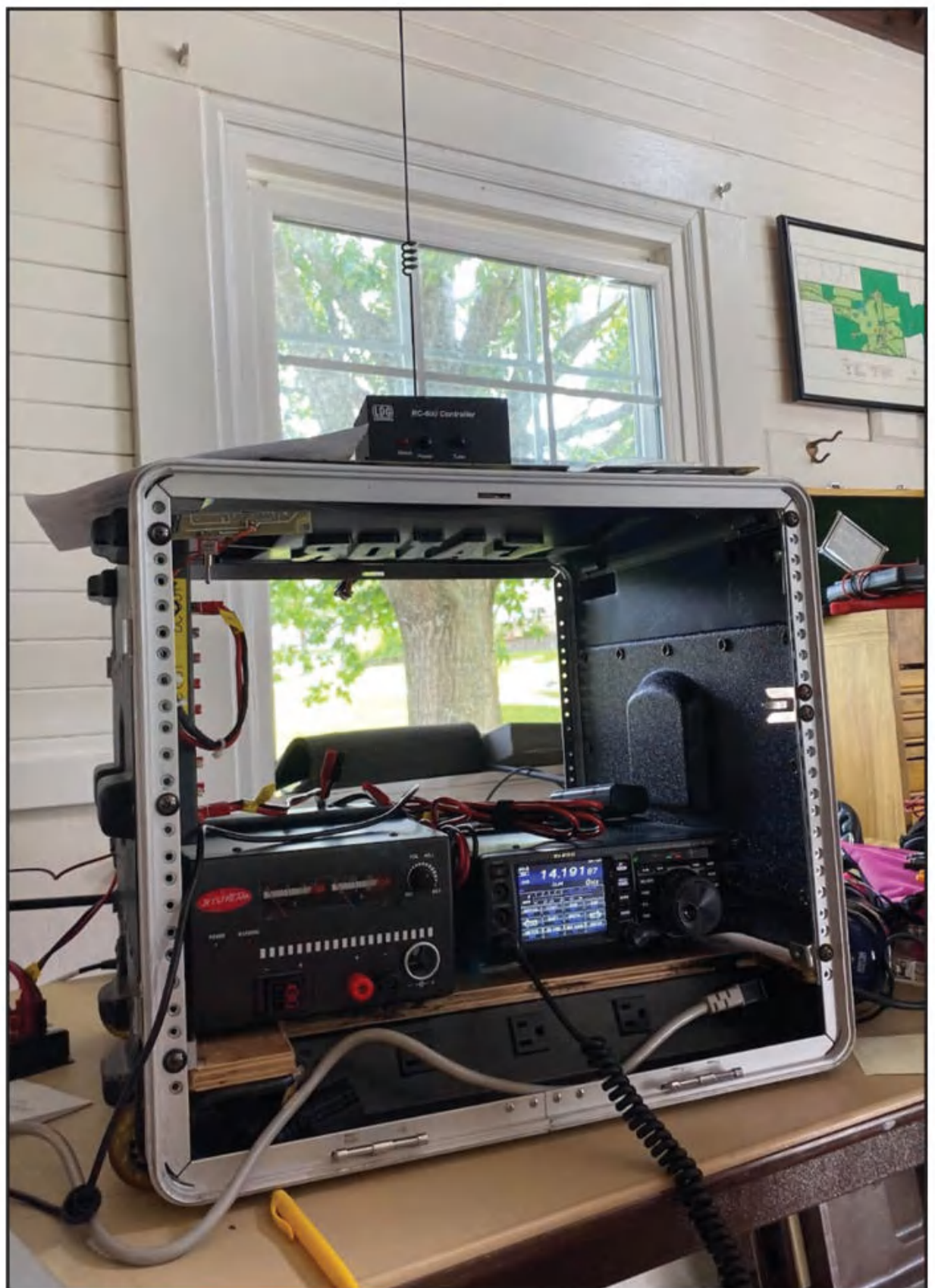
Photo A. W8EDU Go Box with Yaesu FT-991a operating on one of the DXE-135 dipoles.
