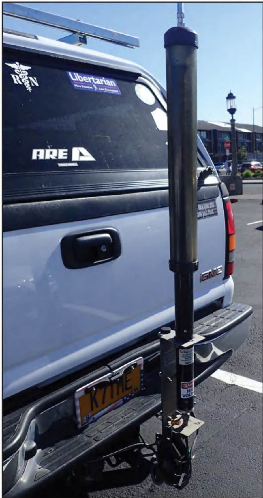
Photo E. The Big Tarheel antenna would work better than the Little Tarheel II when on a hitch mount. This Tarheel mount, on a truck belonging to Larry Bever, K7TME, also has more ground clearance to help with not bottoming out. Larry's QERZ.com site has some gorgeous photos of his apparently remote home.
