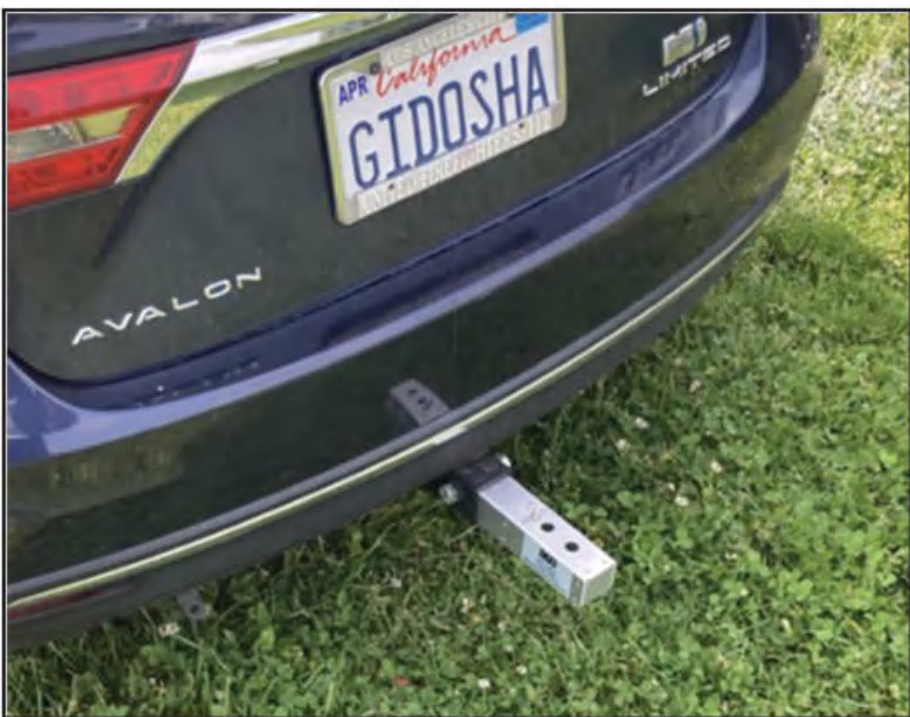
Photo C. The MFJ hitch receiver mount that had a few issues with the lower-slung car, The car would bottom out, causing the antenna mount to drag, damaging the coax and coax connector. (See Photos E and F for more on this.)
