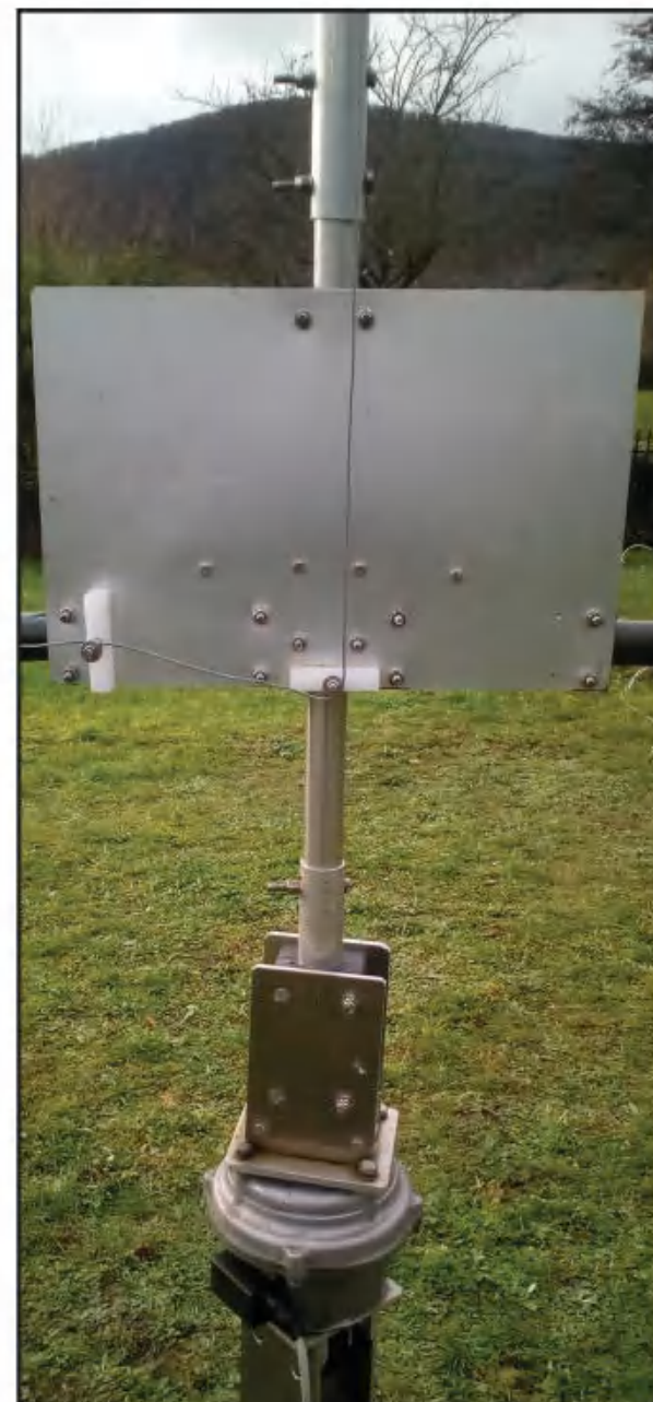
Photo B: Isolating the antenna wire at the central point.
