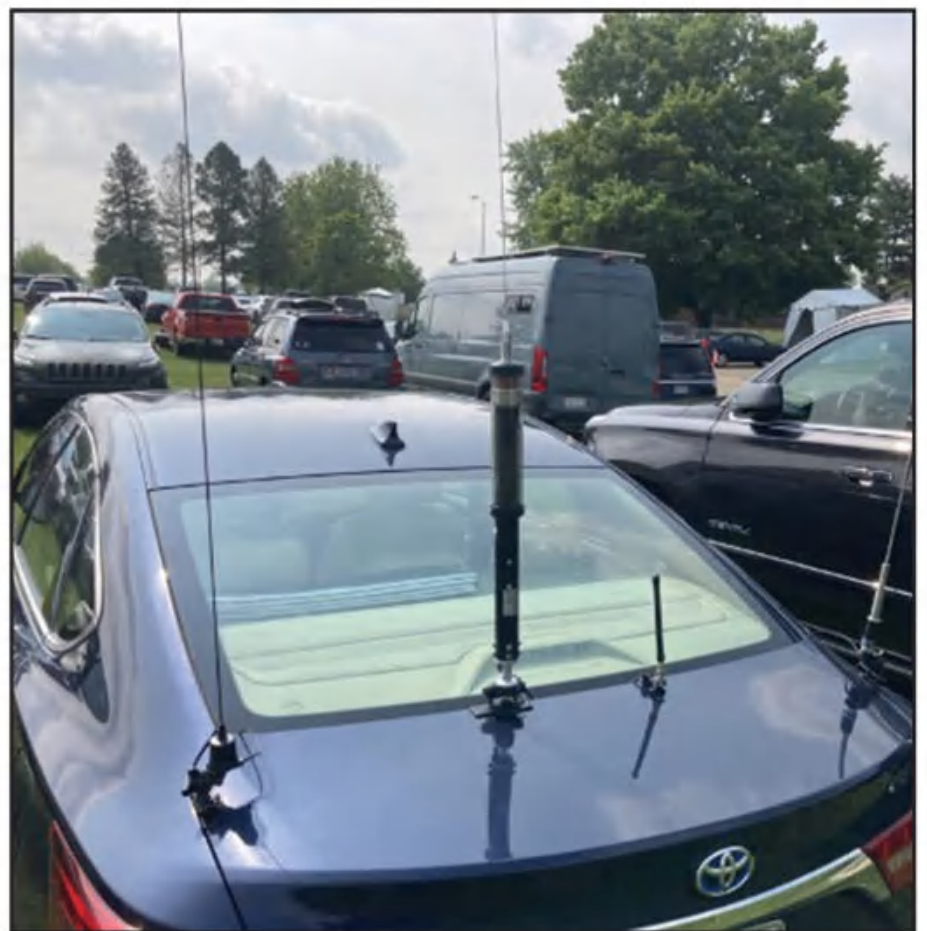
Photo B. The Toyota Avalon hybrid ride of The Lost Boys, W6RH, AA6JR and NS6X. Two VHF/UHF antennas, packet antenna and the Little Tarheel II HF antenna.
