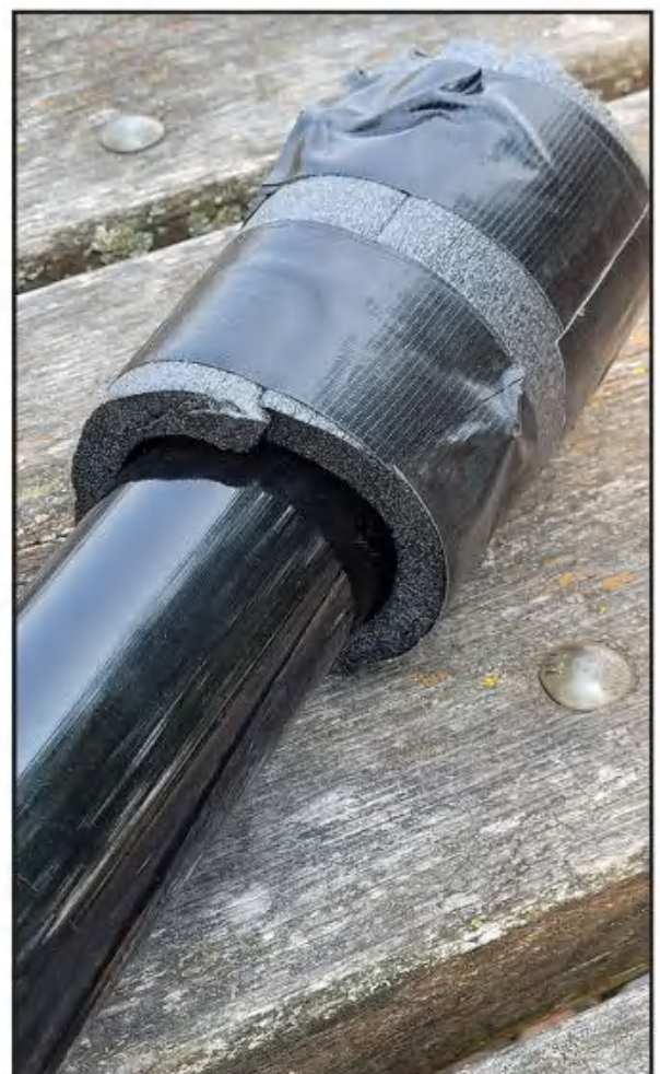
Photo D: Closeup showing pieces of pipe insulation wrapped around and fastened to the base of the Spiderbeam telescopic pole.
