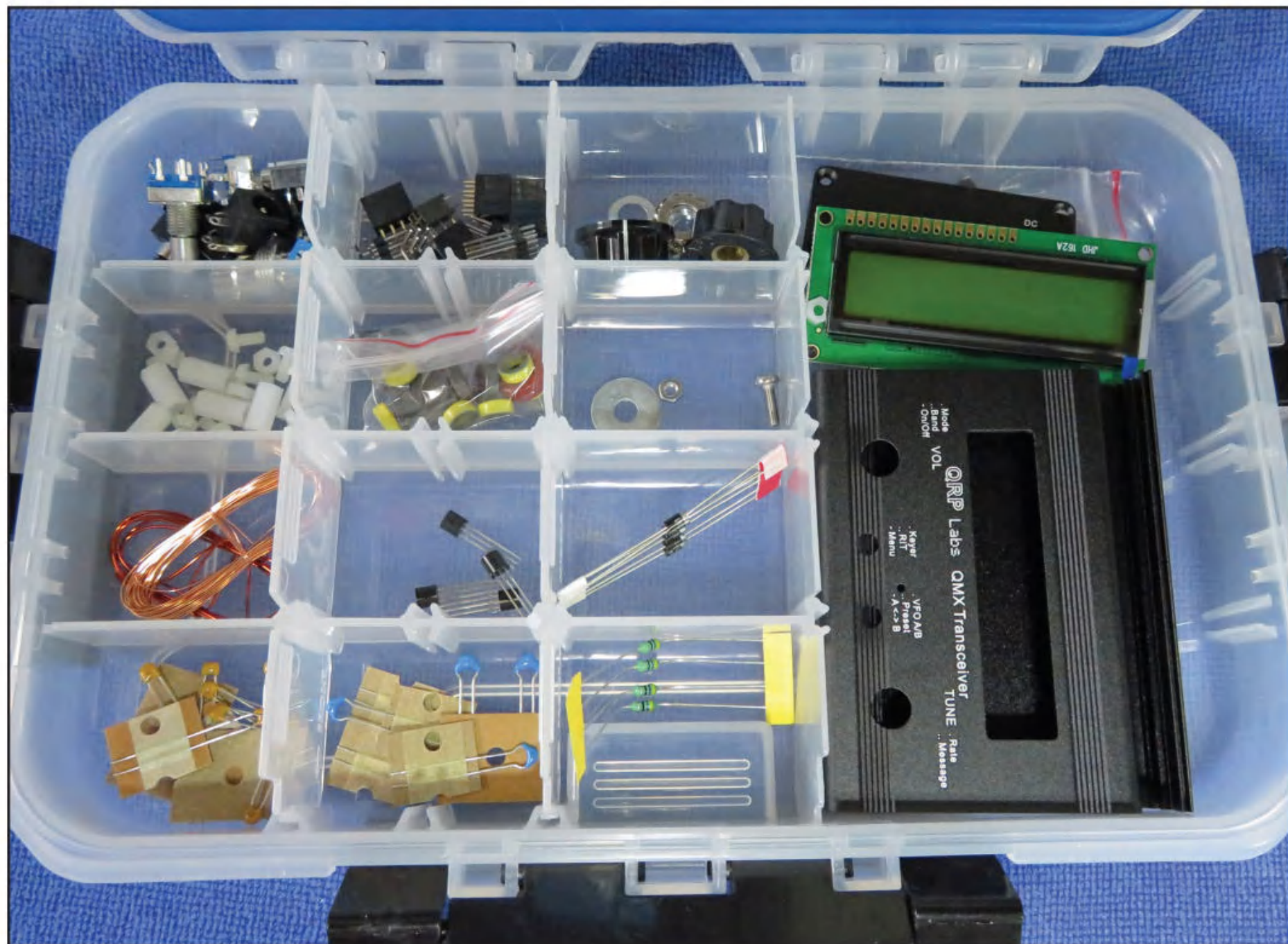
Photo C: The QMX parts are sorted and ready to begin assembly. Other than a trimpot, there are no resistors to mount!
