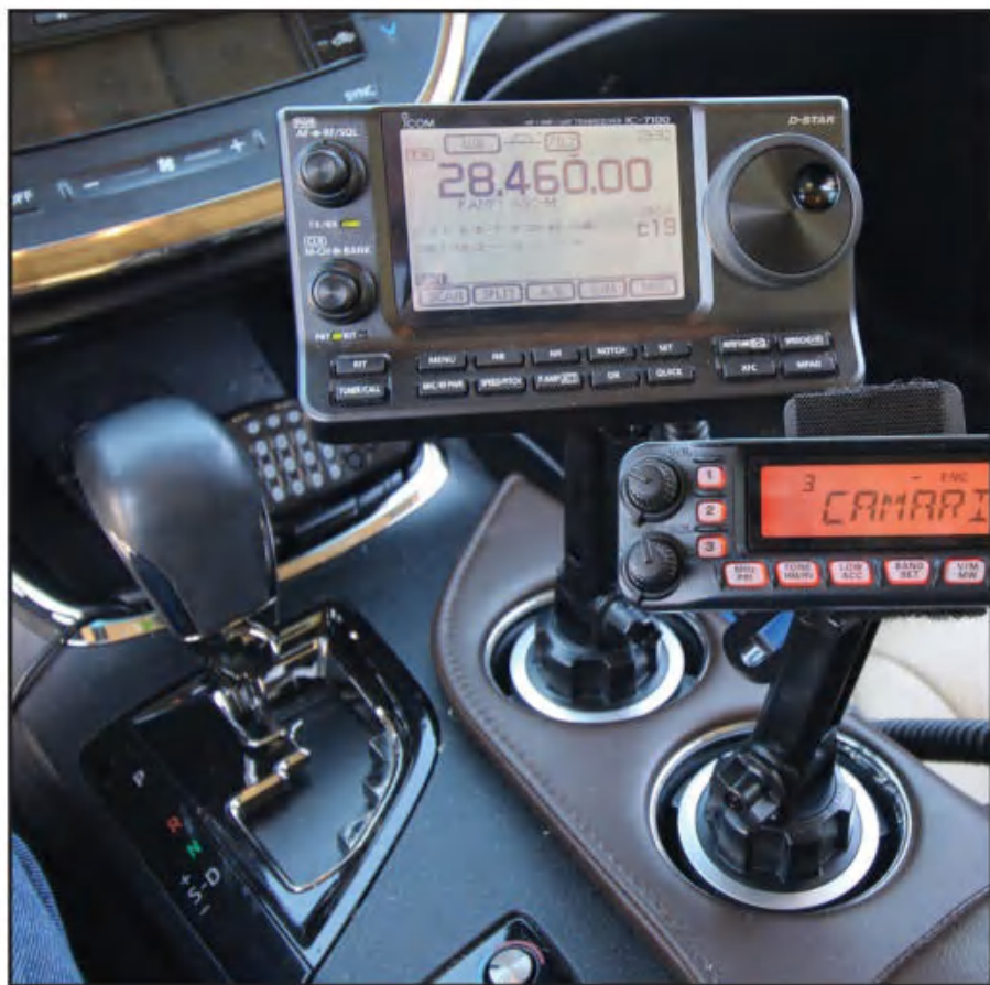
Photo D. The IC-7100 and FT-7900 control heads are mounted on Lido Products cupholder mounts that fit snugly into the vehicle's cupholders.
