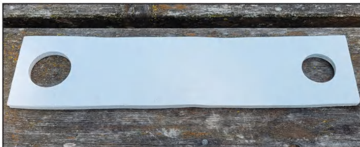
Photo B: The wooden mount for securing the telescopic pole to the operating position.
