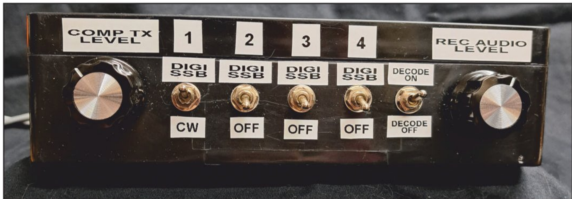
Photo C. Front view of the completed interface box
