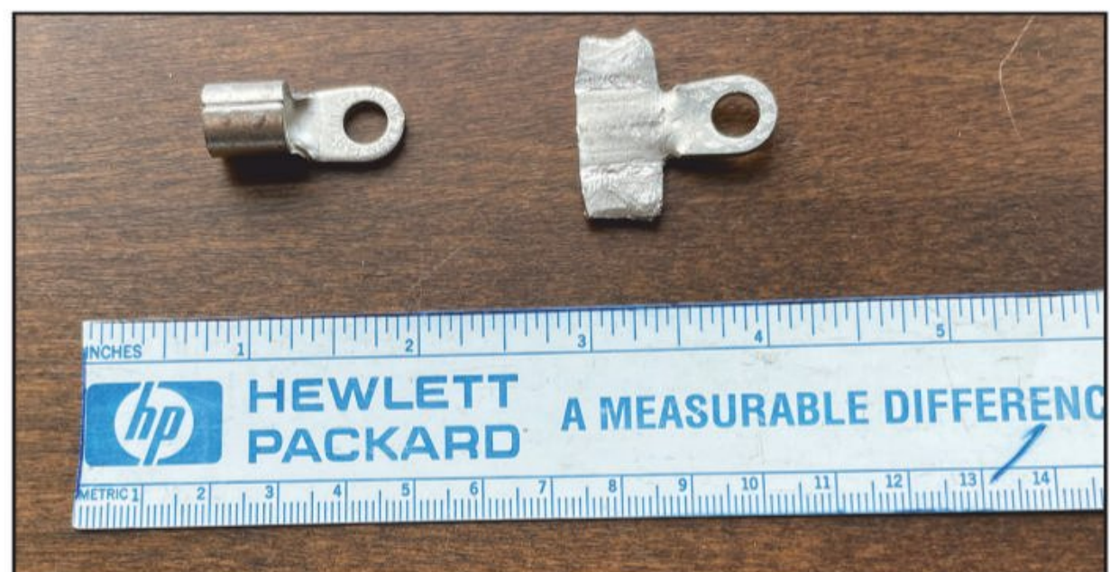
Photo E. Electrical terminals locators before and after
