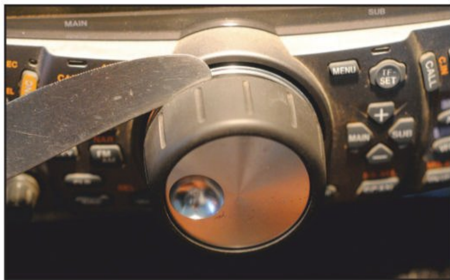
Photo B. The first step is to gently remove the rubber outer ring on the tuning knob.
