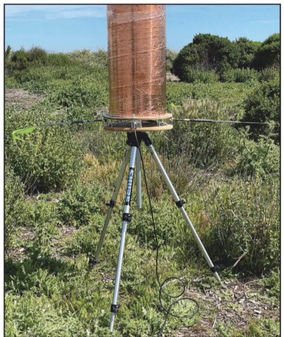
Photo B. The bottom part of the antenna is made from a 12-inch diameter cardboard construction form covered with adhesive copper tape. Also note the tuned radials, which are actually Hustler resonators.
