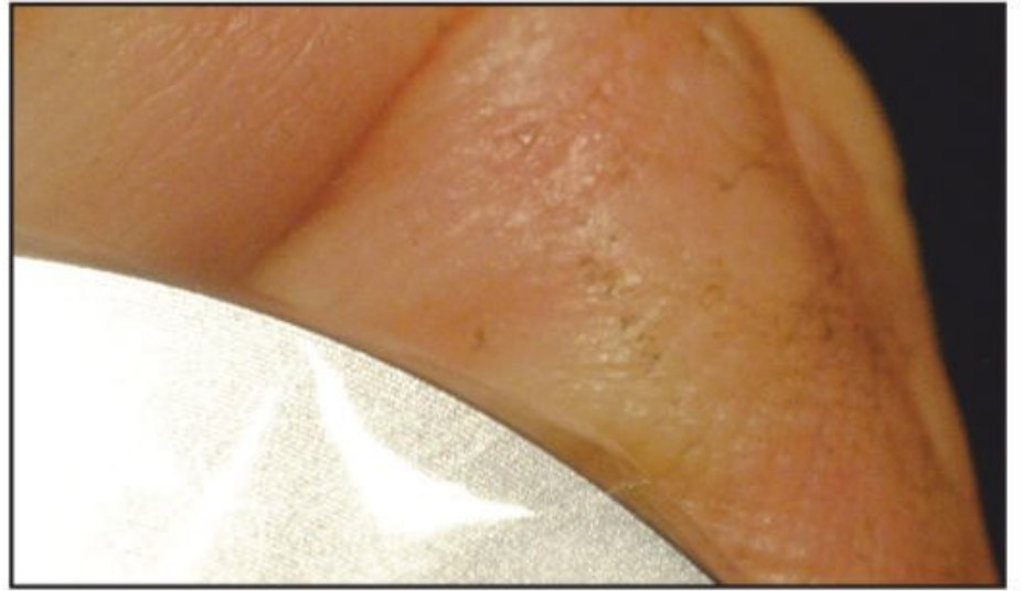
Photo H. There should be a thin plastic film on the back of the knob, which will likely be starting to come loose (and is generally the cause of your tuning dial problem). Peel it off with your fingertip.
