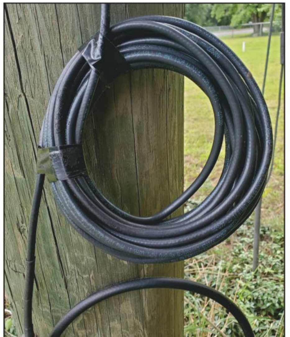
Photo E. An ugly but effective RF choke on the feedline
