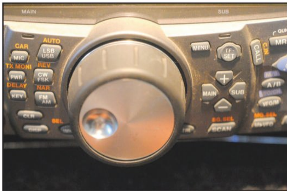
Photo A. The main tuning dial on the Kenwood TS-2000 can get "sticky" after years of use. Very often, the fix is easy, as long as you're careful.
