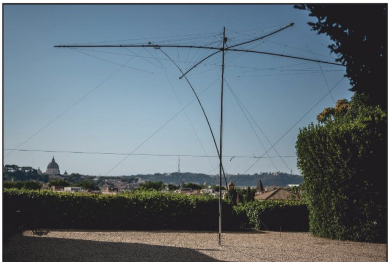
Photo J. The 5-band Spiderbeam Yagi on the terrace of Magistral Villa (Photo by IZ4AKS)
