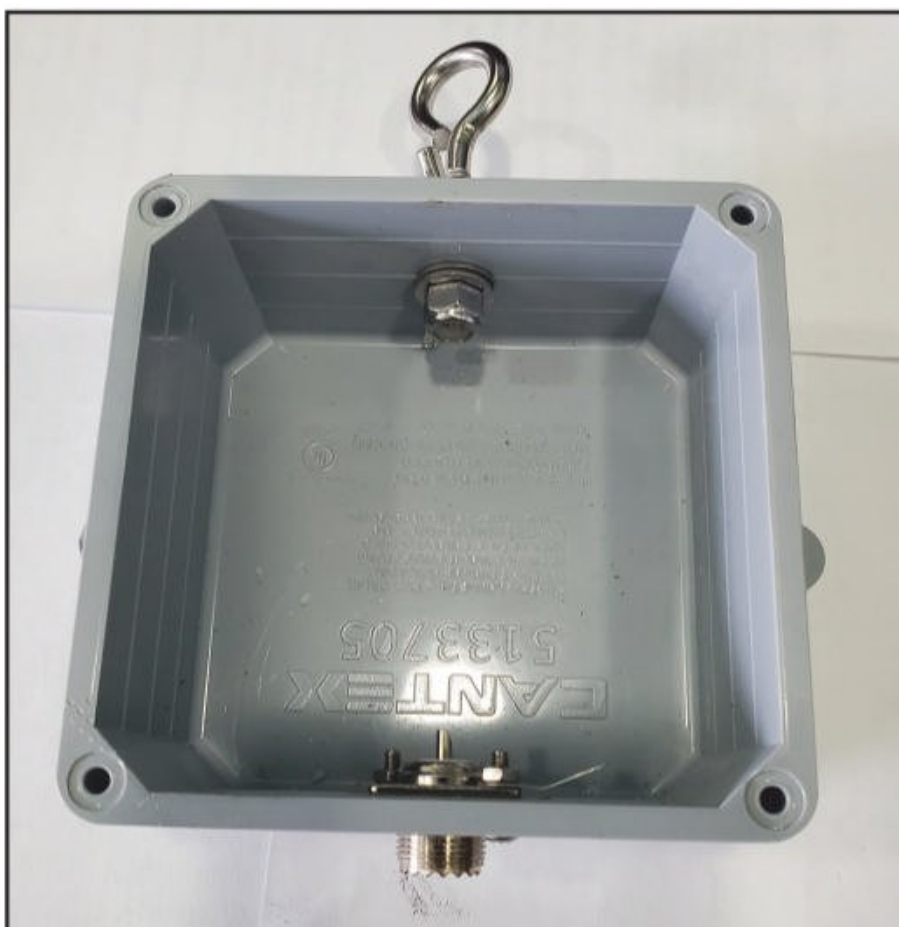
Photo A. Unun enclosure with hardware
