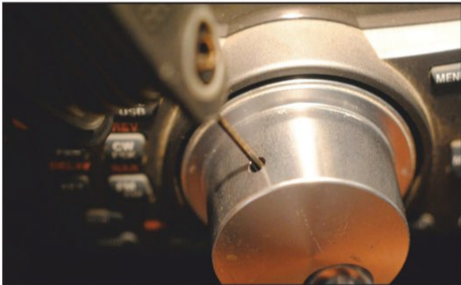
Photo F. Loosen the set screw with your metric Allen wrench, and ...
