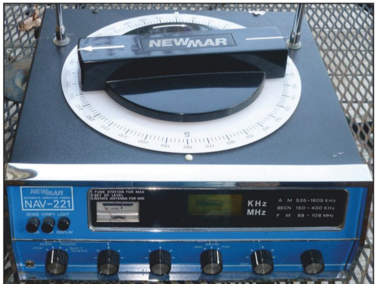
Photo B. Ferrite rod antenna in a direction finder
