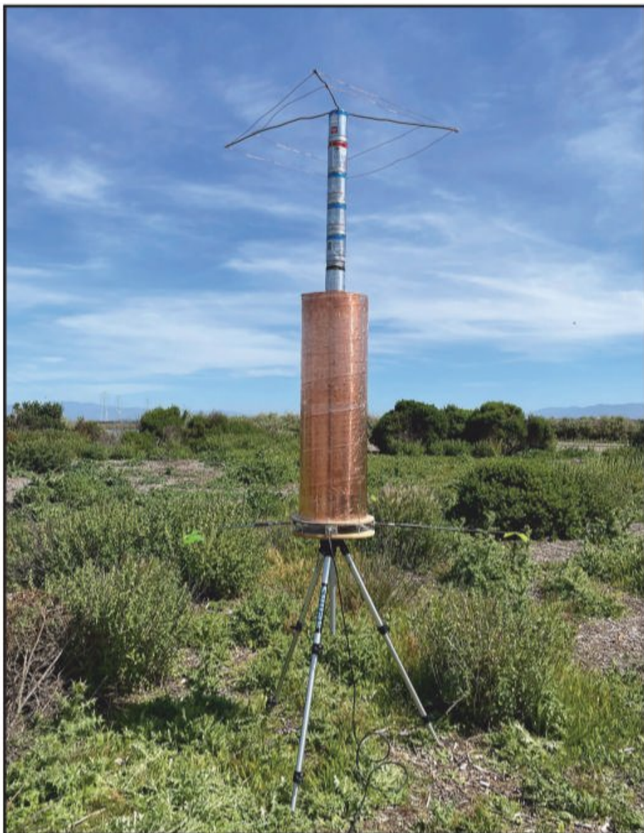
Photo A. AH6CY's asymmetric vertical dipole works on any three bands between 20 and 10 meters.
