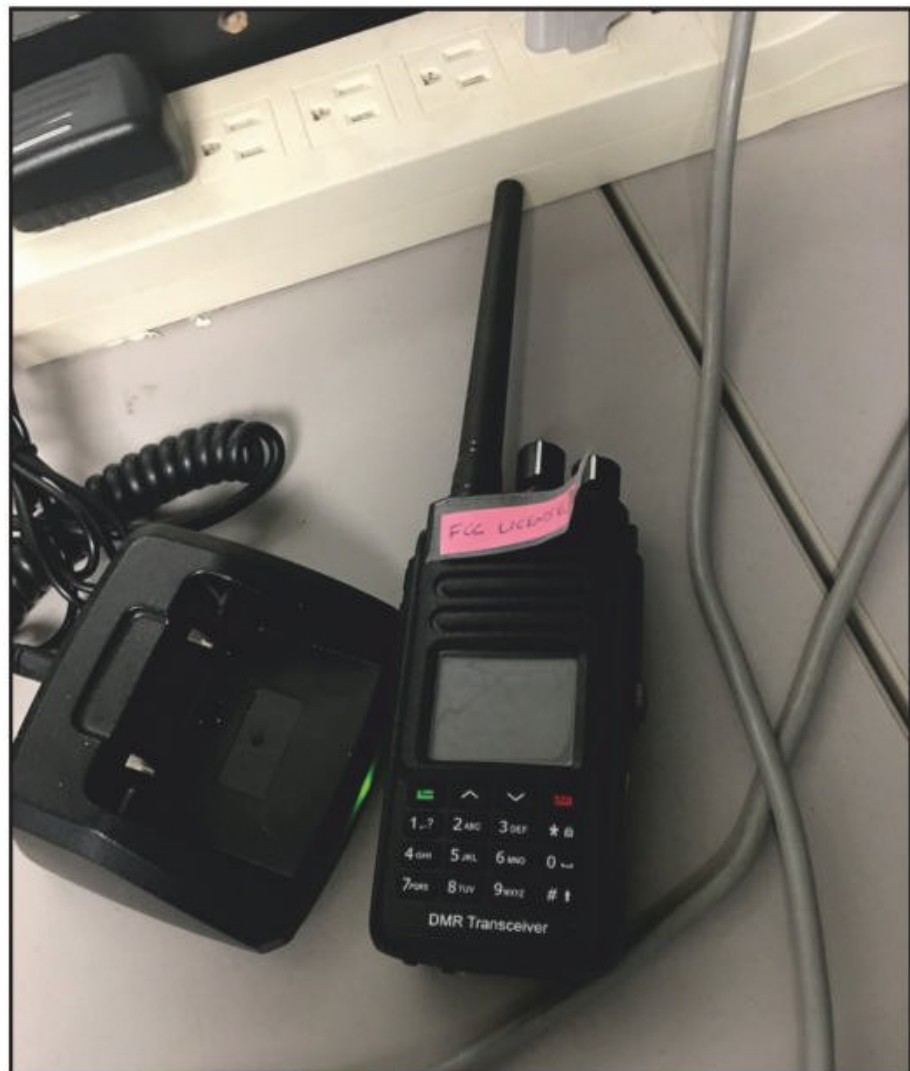
Photo L. DMR is another vital communications tool for Memphis NWS. The advantage is that geographical groups within the CWA can give storm reports with clear reception as long as there is a reliable internet connection or DMR repeater coverage back to the Memphis NWS office.
