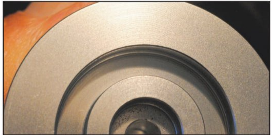
Photo I. Make sure the back of the knob is clean and smooth after you've removed the plastic.
