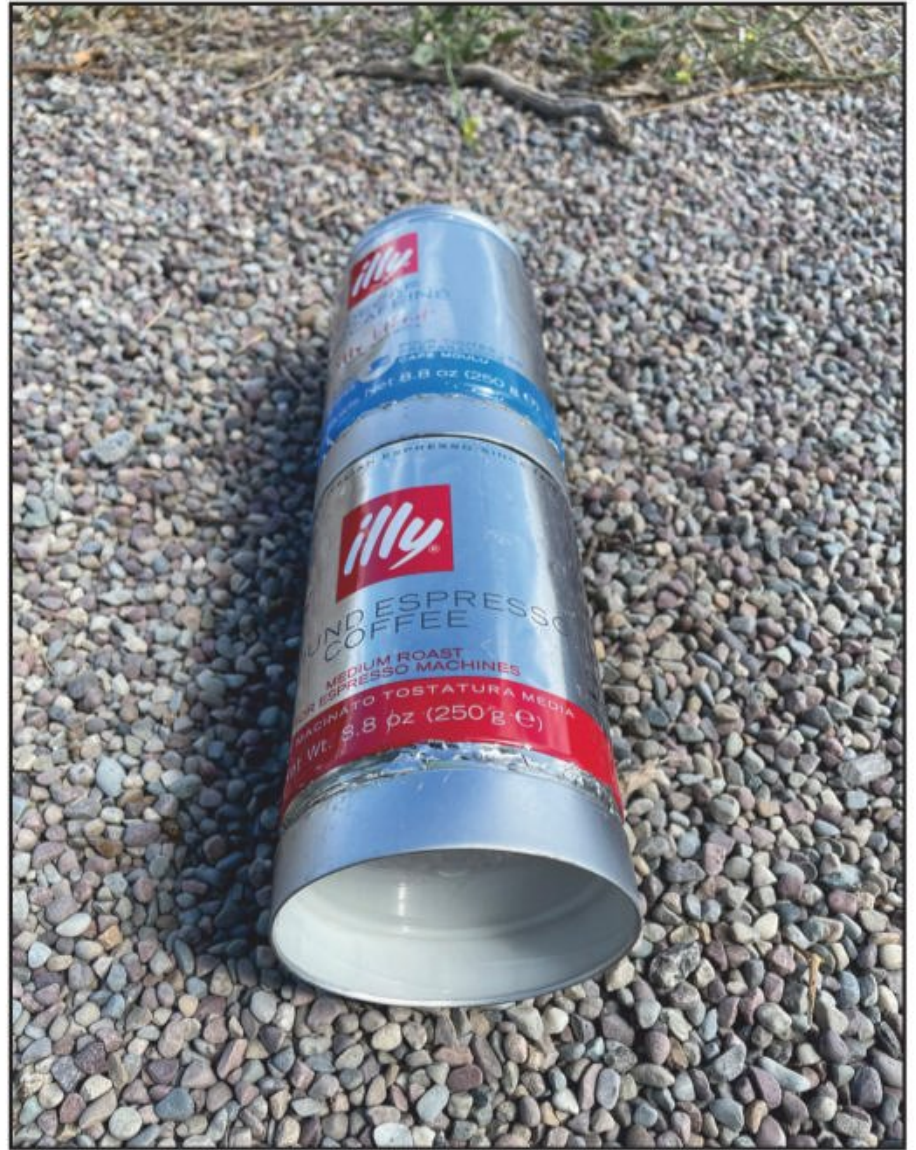
Photo D The modified coffee cans may then be screwed together to form a stable stack.
