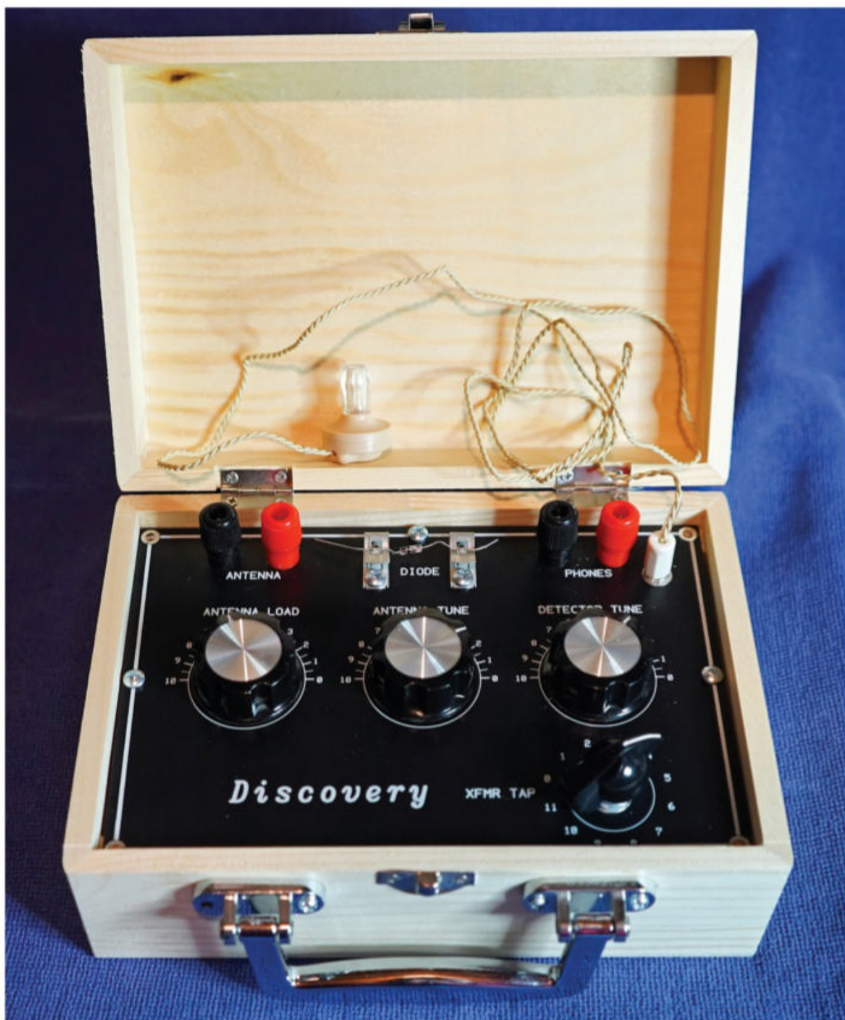
The finished Discovery crystal set in the Hobby Lobby wooden case.
