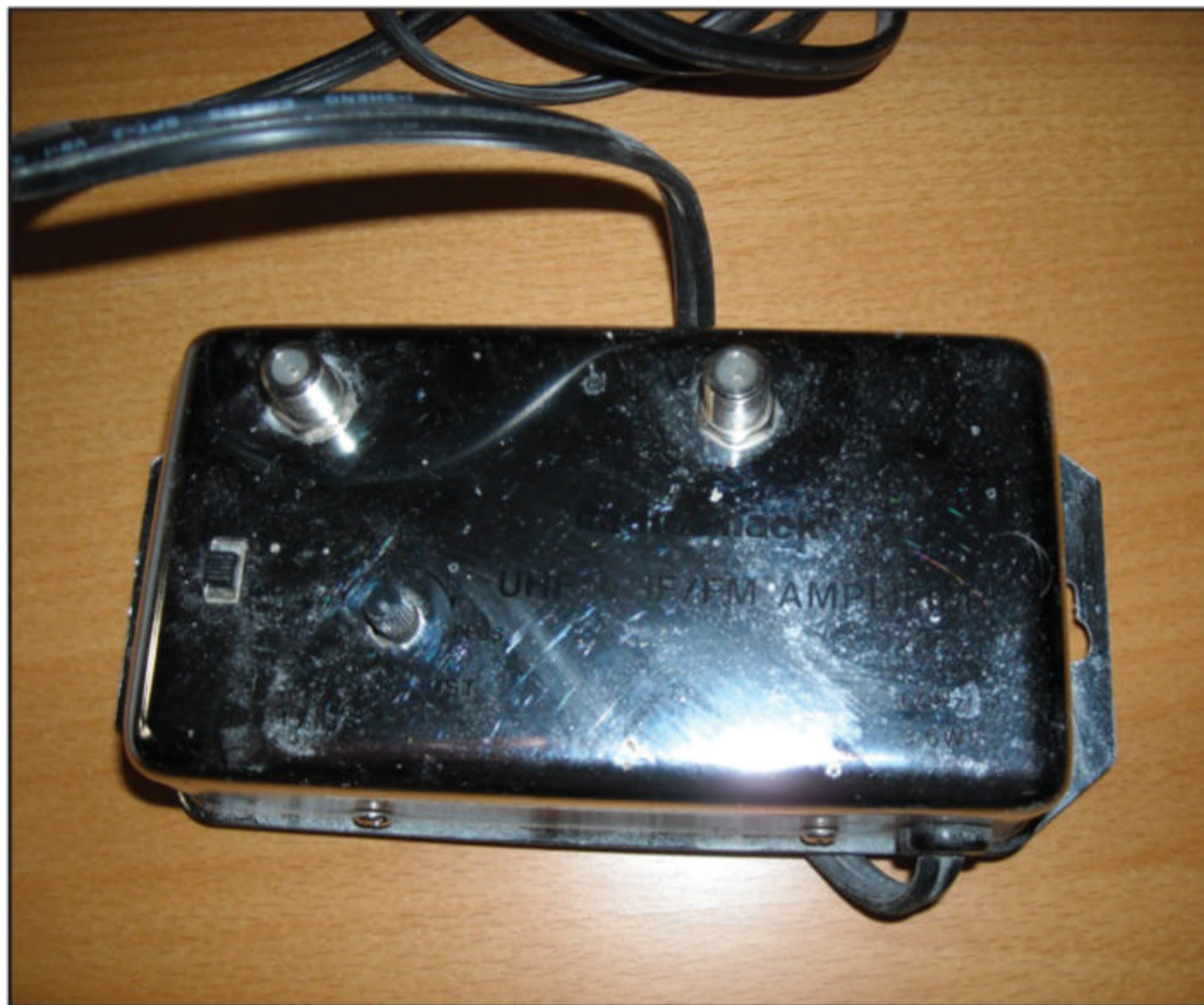
Photo C. A VHF/UHF TV/FM preamplifier provides broadbanded amplification over the VHF and UHF portions of the spectrum where most scanner listening takes place. With the advent of digital TV and the market dominance of cable and satellite TV systems, look for these at bargain prices at hamfests and even yard sales.
