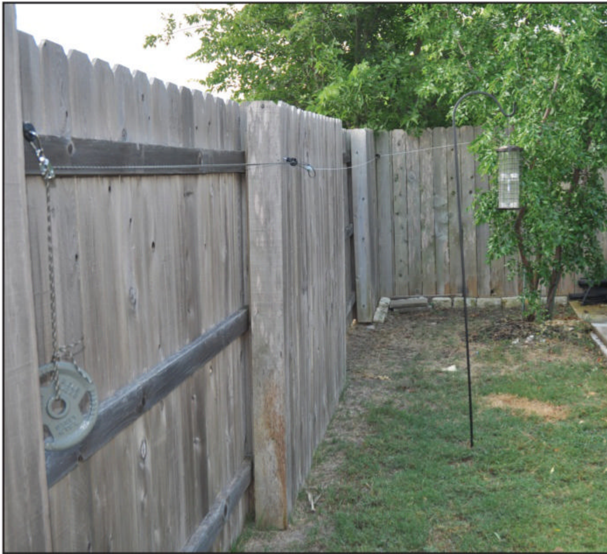
Photo B. The left leg of the dipole, bent at the fence corner and held by a 2.5-pound weight.
