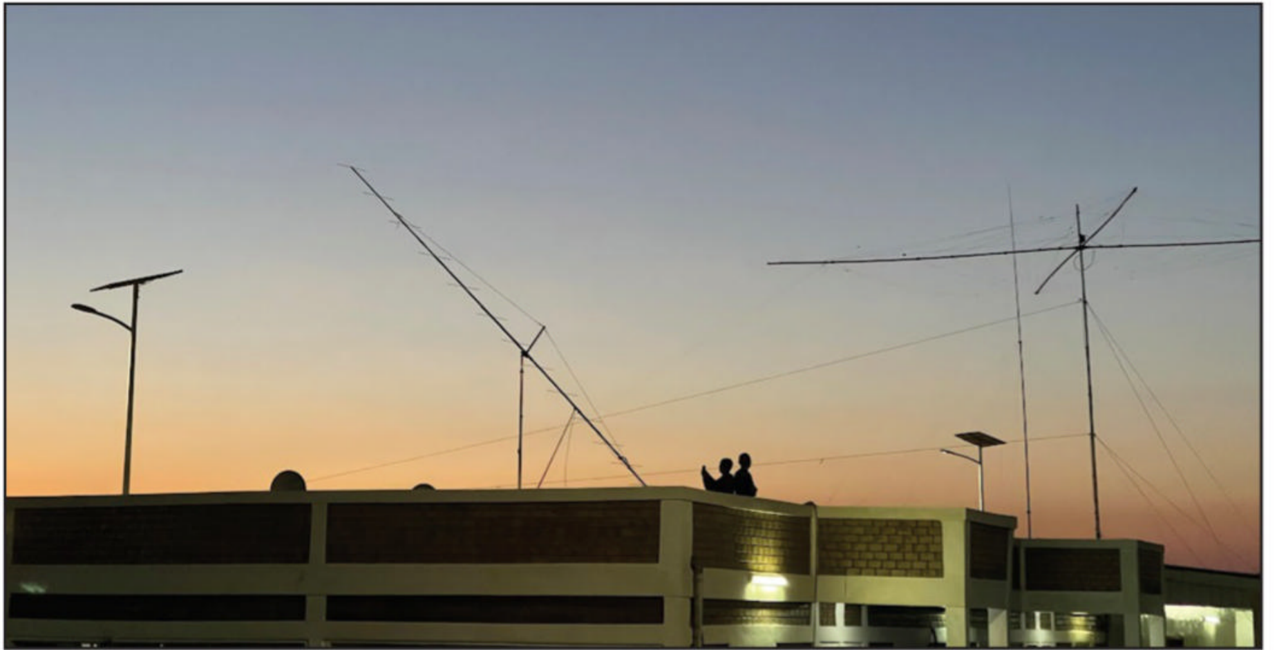
Photo H. EME antenna, 80-meter vertical, and wire beam antennas in the sunset.
