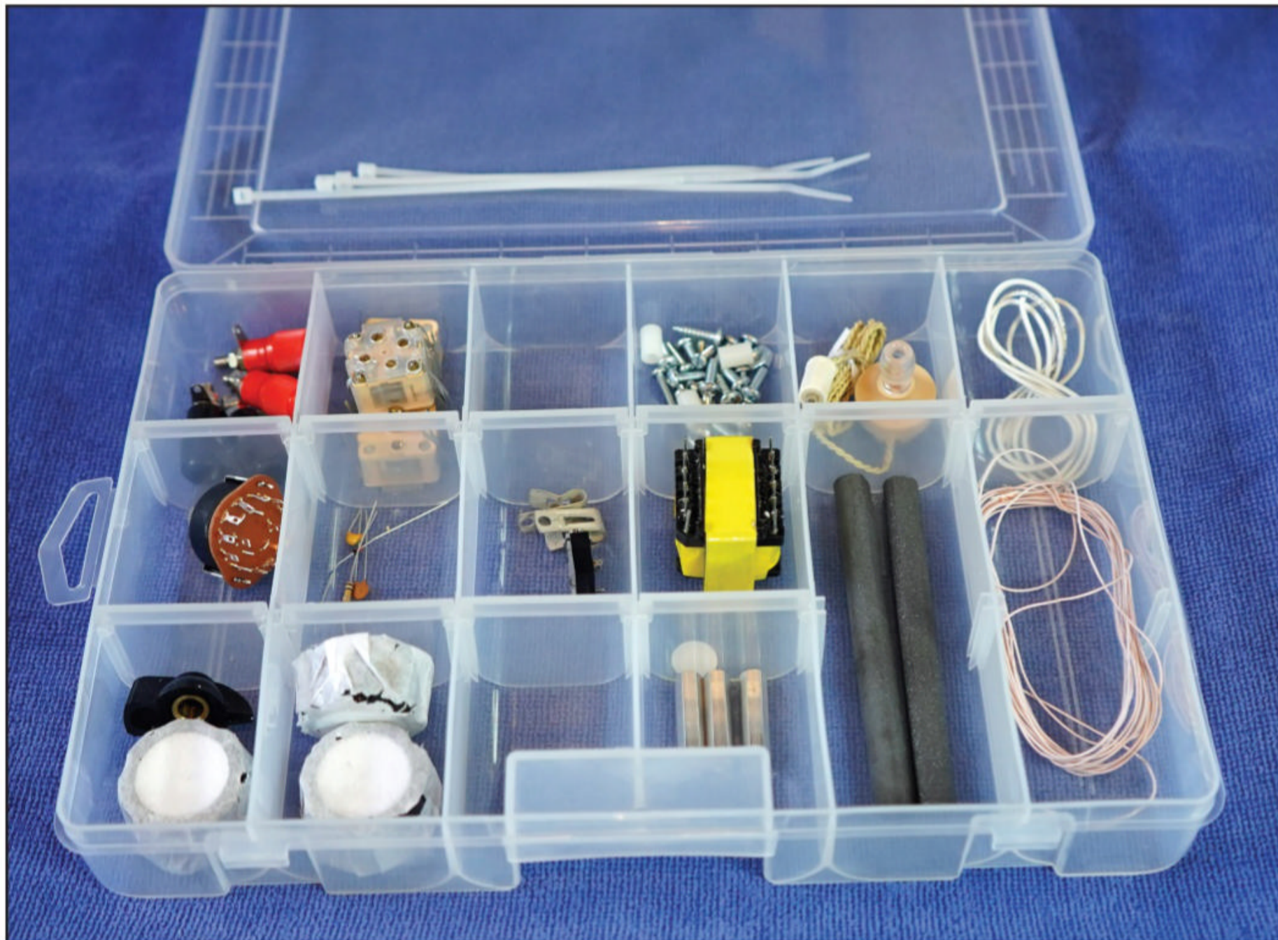
The parts for the Discovery crystal set kit all sorted and ready for assembly.
