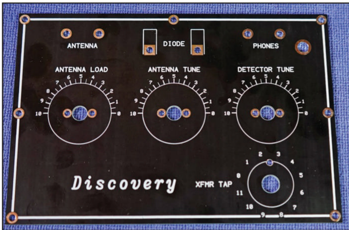
The front panel side of the main PC board before assembly.
