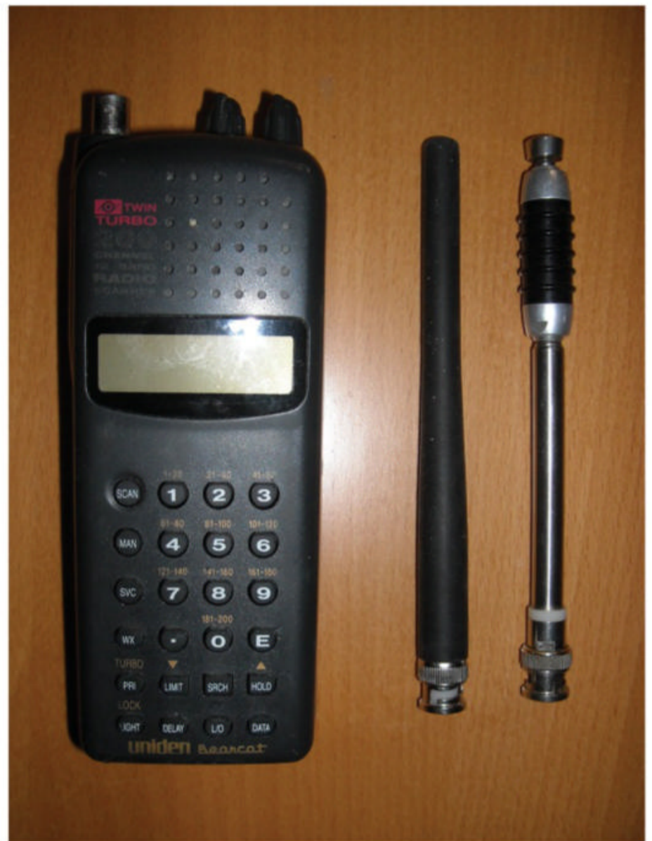
Photo A. An easy way to increase the range of a handheld scanner is to replace the “rubber duck” antenna (center) with an extendable whip (right). (Photos by the author)
