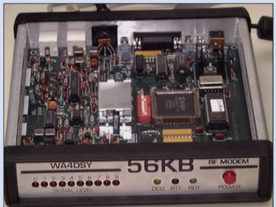
One of Dale's major contributions to amateur radio digital technology was his 56-kilobaud GRAPES radio modem, the fastest amateur radio modem of its day.
