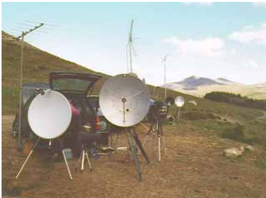
At Mynydd Garnguwch, GW8OZP, 2m Yagi, 3cms TX and large dish, RX LNB and Offset dish
