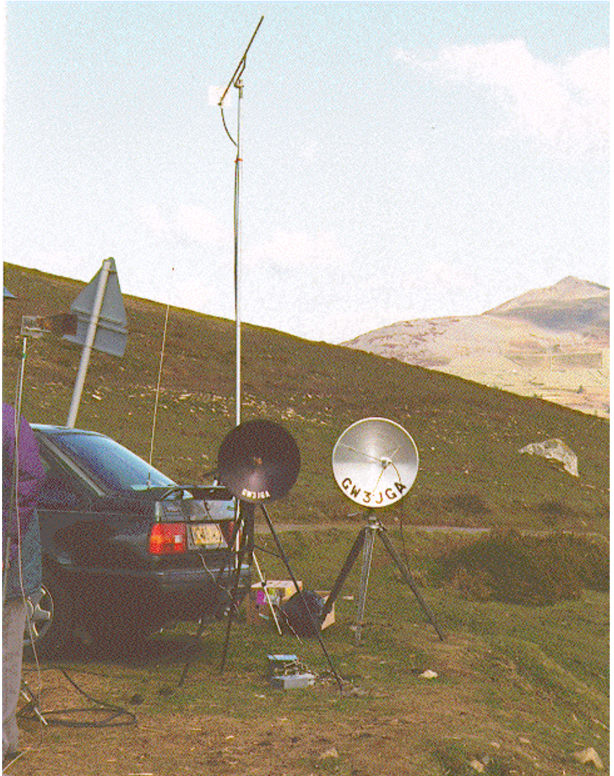
At Mynydd Garnguwch, GW3JGA, 24cm Loop Yagi, 3cms TX, Penny Feed Dish, RX LNB and Dish
