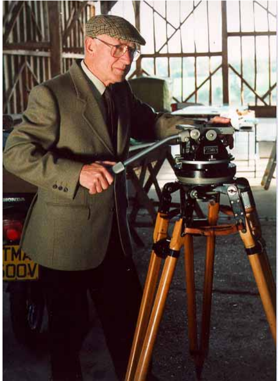
Bill Vinten with a pristine example of a model 'J' pan and tilt head, inertia flywheel drag
