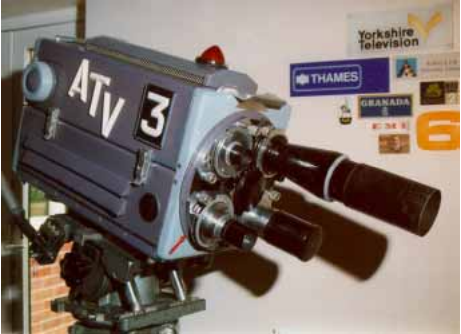
The Pye MkIII 3 inch image orthicon camera. (1956)
