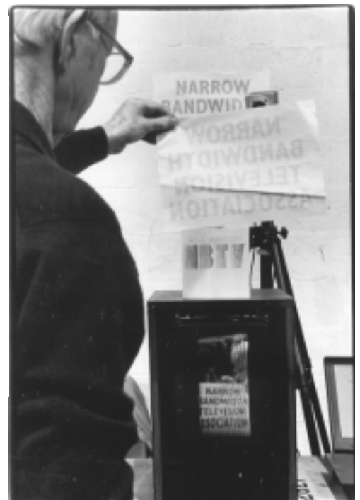
Above, right:- Doug Pitt dangles a rather creased paper poster before the camera. A rigid caption card with the camera properly focused would have given better results of course. All the same, the legibility is quite good when you consider that the minimum criterion for recognition of a 625 line picture is just four digits (BATC contest rules) (Photos by Jeremy Jago)
