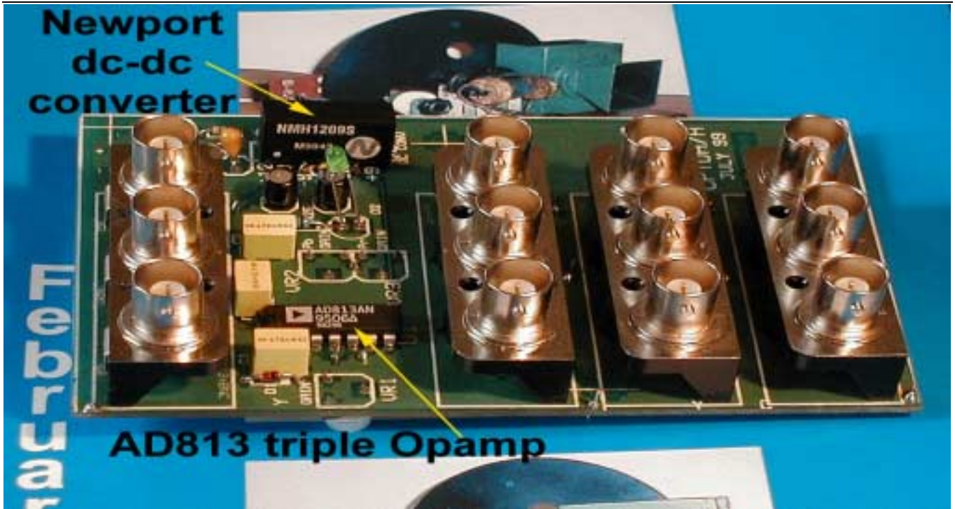
Figure 3 - Component DA pcb
