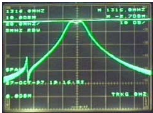
Passband of two sections with notch filter
