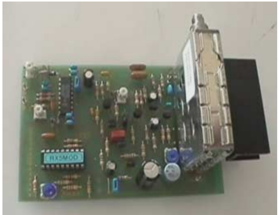
The receiver before the LCD and rotary encoder fitted.
