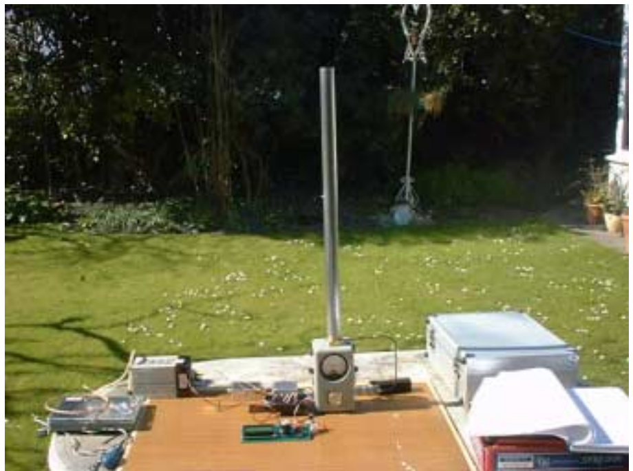
Fig. 1. Testing Alford Slot for GB3TM
