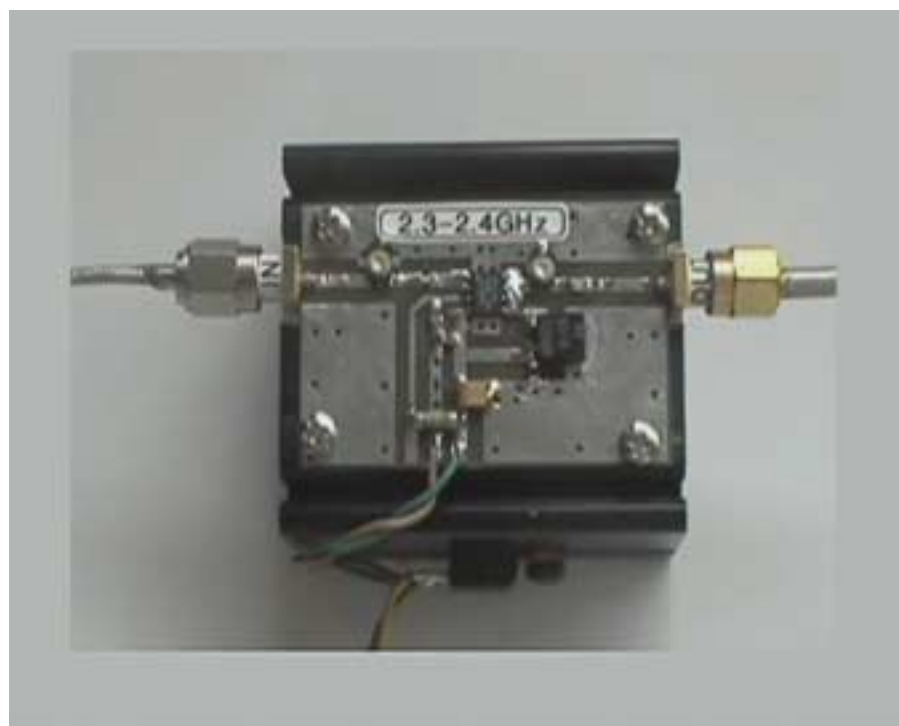
The latest offering from F1GE, a single stage 13 cm amplifier
