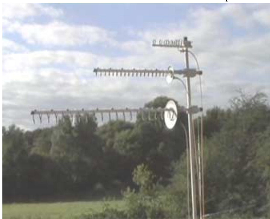
Top; Directive Systems 13 cm 9element loop yagi; Middle Sandpipers 13 cm 20 turn helix; bottom the 23/24cm cousin of the one above. In the background all of those tree dBs!
