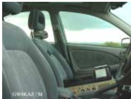
Picture 3 - Shows the equipment plus the video camera firmly held by the headrest.
