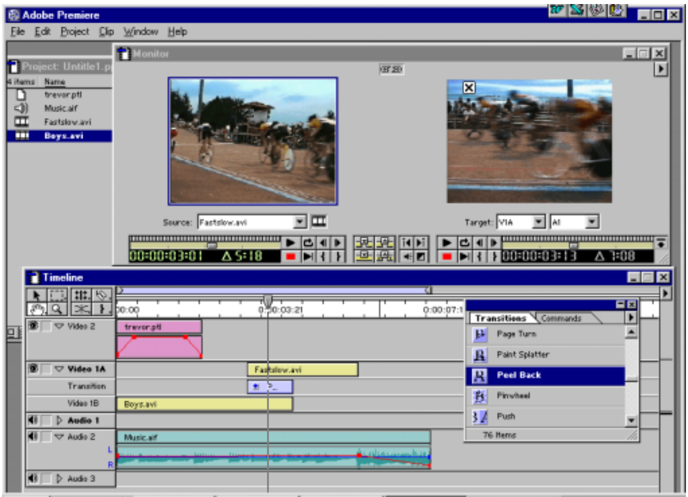
Figure 1 shows a caption set to fade in and out, two video clips with a transition and a sound track with fade out. The mauve bar sets the preview and the scrub pointer can be seen along with Transitions menu PV and TX monitors.
