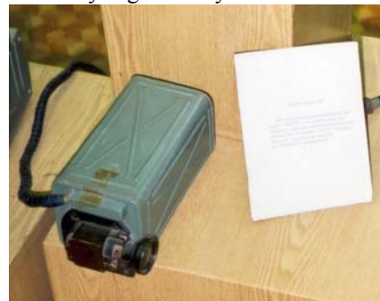
Gagarin's 100 line Television Camera with description alongside.
