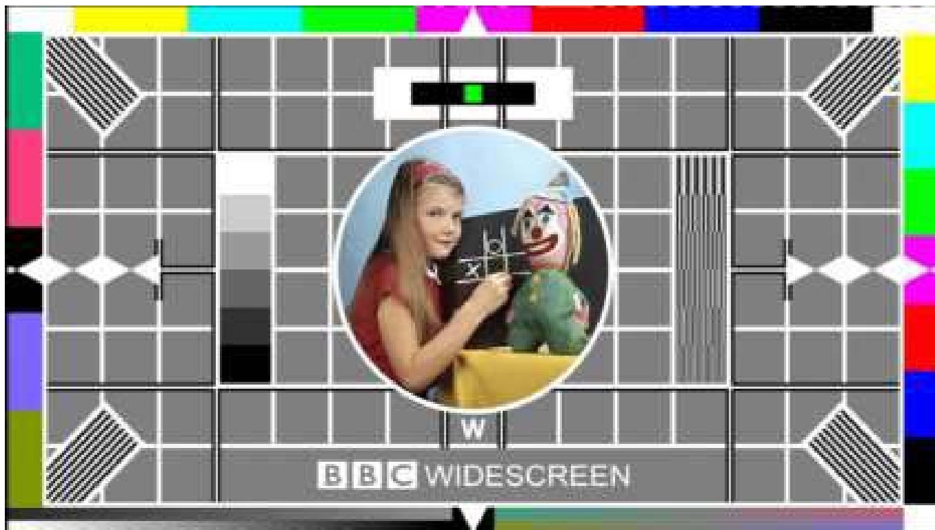
4:3 picture in a 16:9 coded frame
