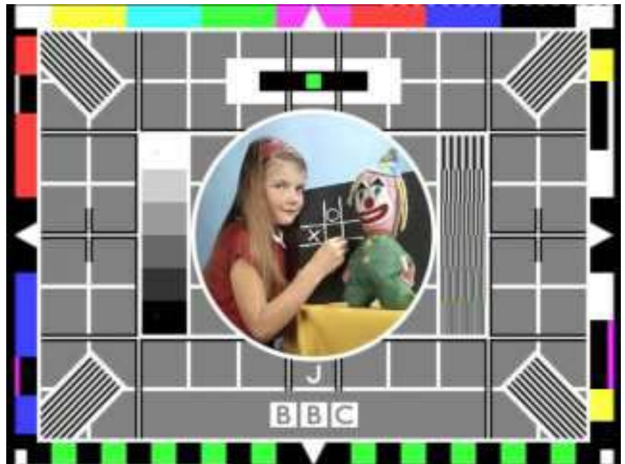
4:3 picture in a 4:3 coded frame
