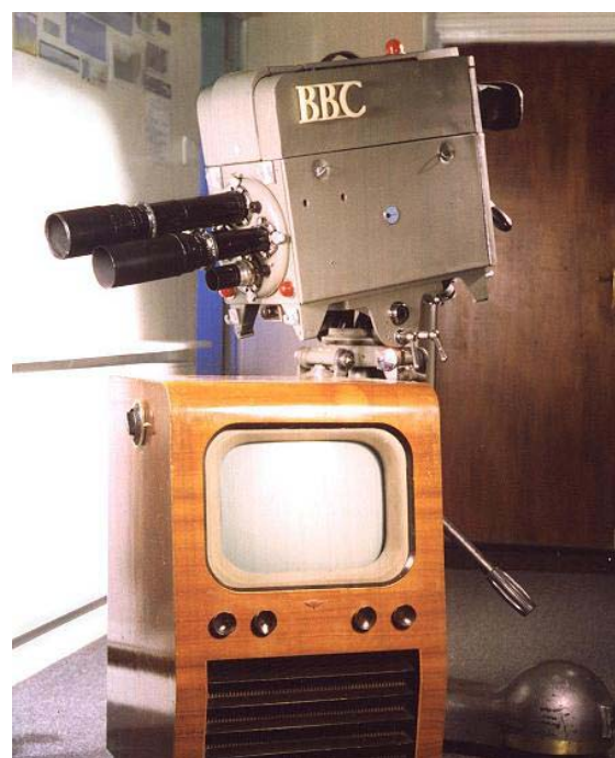
iBOTH ENDS OF THE CHAIN. A Marconi Mk II, the type used at the Coronation in 1953. A Kolster Brandes console tv set, the type used to view the Coronation in 1953. (From The Dicky Howett collection)
