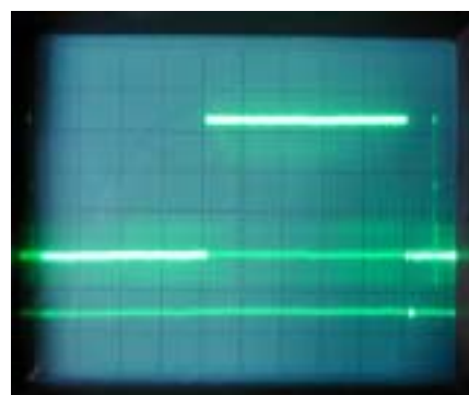
Received 50Hz square wave on scope (Field rate)
