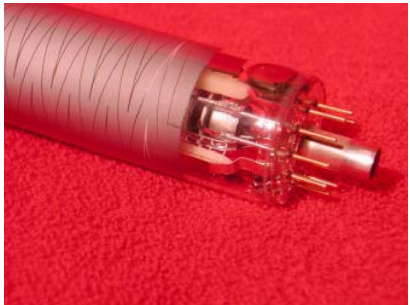
Figure 7 Zigzag Deflection plates (From the author’s collection)
