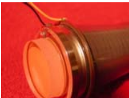
Figure 9 Target and Mesh Contacts (From the author's collection)
