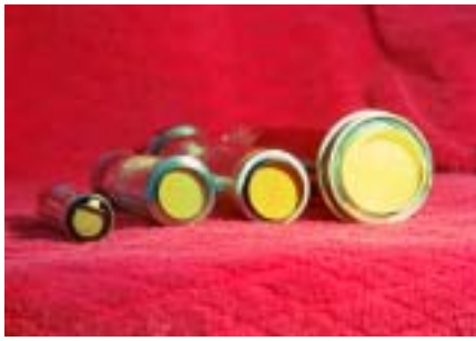
Figure 8 Plumbicons (L to R) 18mm (2/3in), 25mm (1in), 30mm, and 45mm Plumbicon tubes. (From the author's collection)
