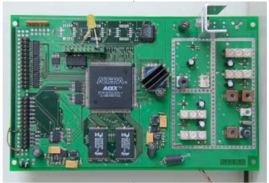
The Transmitter board
