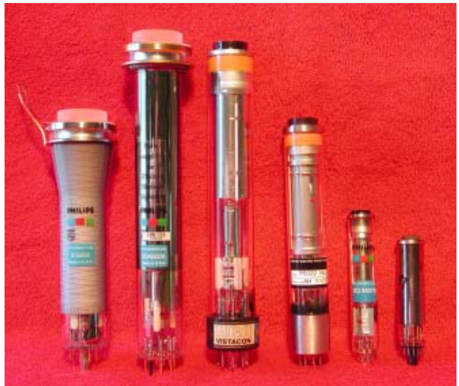
Figure 11 Camera Tubes. (L to R) 45mm Philips XQ5002 MS (Medical), 45mm Philips XQ4502 MM (Medical), 30mm RCA Vistacon BC4592/L MM, 25mm (1in) EEV P8022HG MM, 18mm (2/3in), Philips XQ3457B MM, 18mm (2/3in) Sony CT2332 MS. (From the author's collection)
