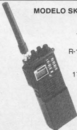
Transceptor FM 2 metros R-140 a 164 MHz, 3/7 W. RA - 142 a 175 MHz, 3/7 W.
