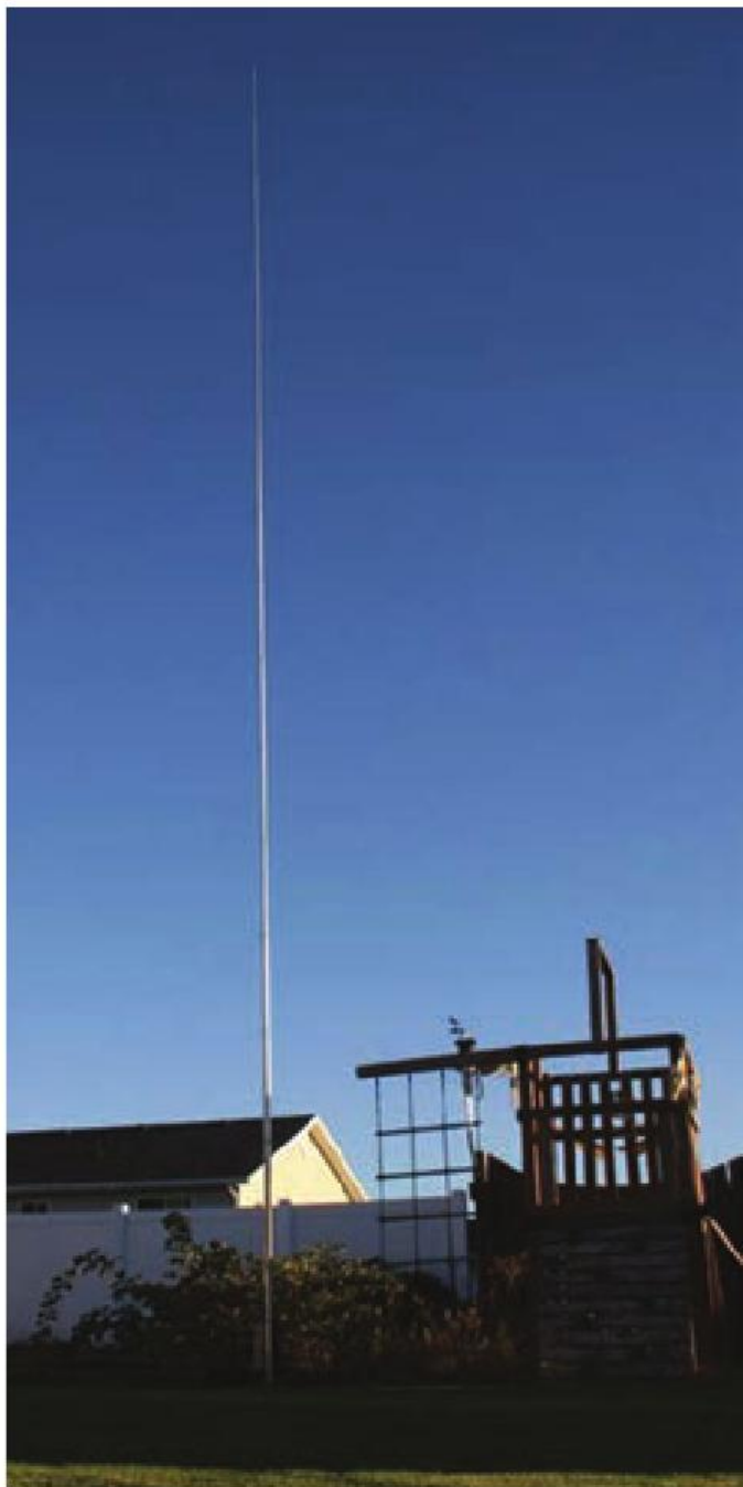
Gary Roberts, AG1T, utiliza esta vertical MBV-1 de DX Engineering de 13 metros (43').
