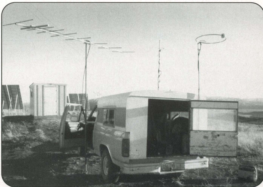
NC7K's rover station in a recent photo. The loop antennas cut down range somewhat, but minimize set-up and tear-down time.
