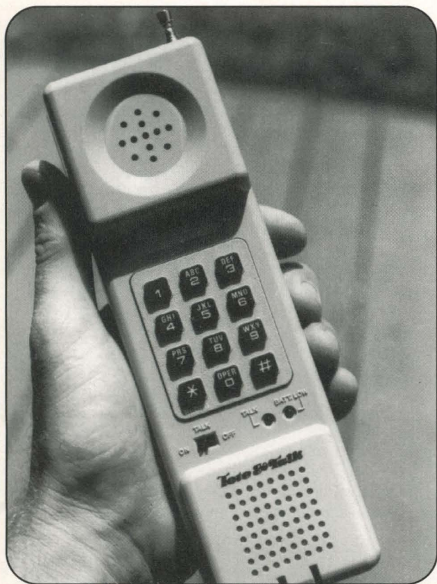
Cordless phones are actually low-power transceivers. And the new 900-MHz models can put "birdies" on 2 meters.
