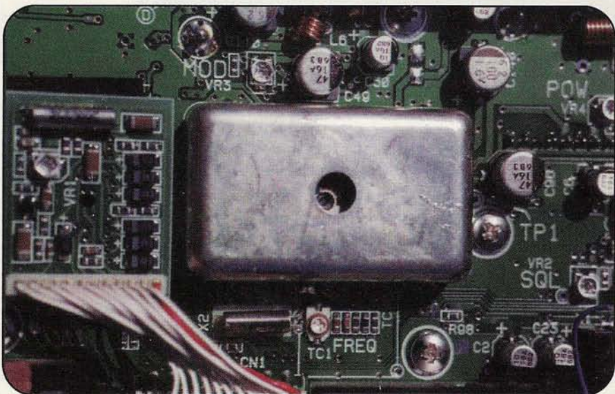
The CTCSS decode unit is installed at the left of the silver can and plugs in easily. It's an extra-cost option, but it's worthwhile.
