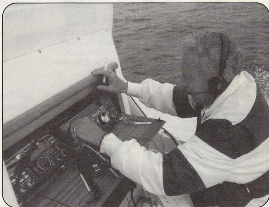
Accessories such as a headset mic (a Heil "Pro-Micro" in this case) helped quiet engine noise on both transmit and receive during this marine VHF DXpedition.
