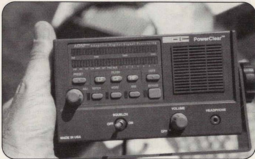
Serious VHF weak-signal operators are learning the benefits of outboard DSP (Digital Signal Processing) units, such as SGC's "PowerClear."
