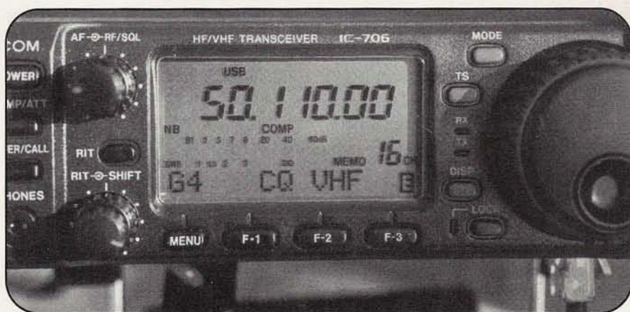
You'll need a multimode rig capable of SSB and CW operation—such as the popular ICOM IC-706 pictured here—to make use of the "exotic modes" discussed in this article.
