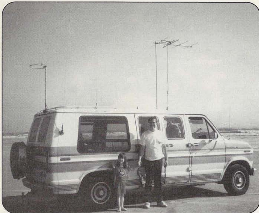
It's easy to go mobile with weak-signal VHF. Here, Mark Casey, NILZC, and his daughter, April, pose in front of Mark's van on the beach in Florida (in February!). The beam above Mark's head is for 2 meters, as is the omnidirectional loop on the back of the van. (Courtesy NILZC)
