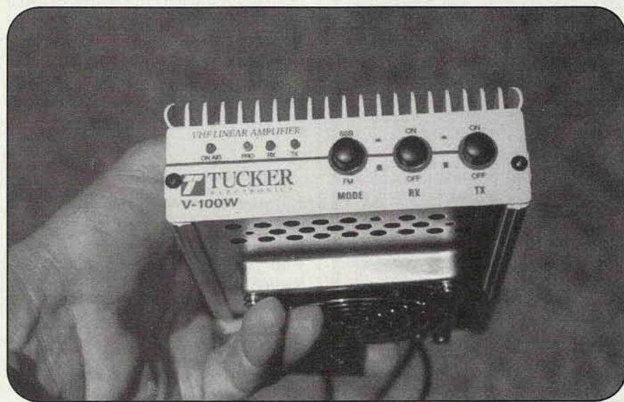
Several manufacturers offer amplifiers to boost the 3 to 5-watt output power of the typical HT. This is the Tucker V-100W.
